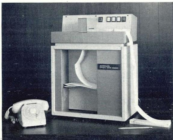
The Automata OMR 8421, an optical mark reader which can read pencil marks from fan-fold forms at a rate of 400 marks per second.
