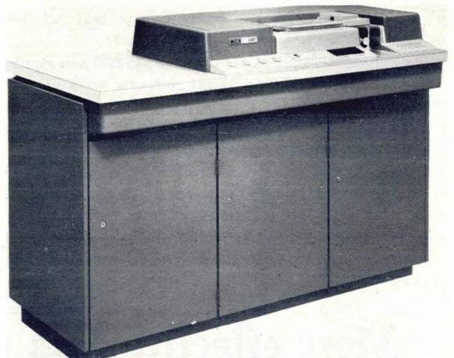
NCR's 420-2 optical journal tape reader, capable of reading 52 lines per second from the paper tape outputs of adding machines, cash registers, and accounting equipment.
