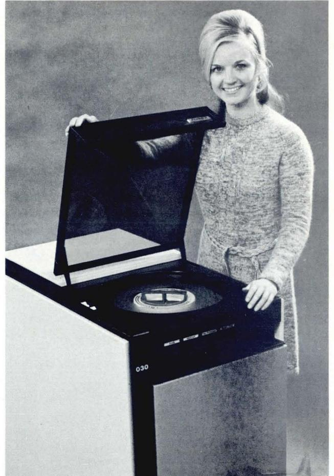
Fig. 3. The DM-312 drive of Ampex, a plug-to-plug compatible for the 2312 drive.
