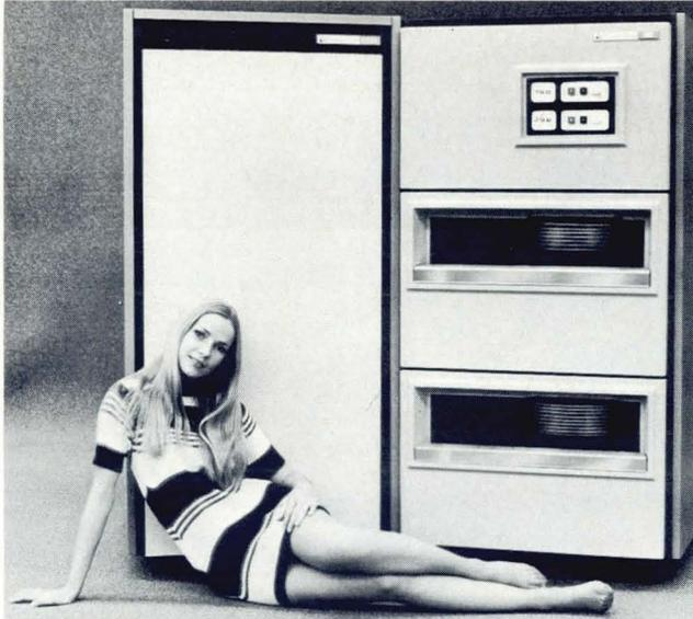
Fig. 2. Century Data's CDS 214 drive and CDS-1014 A controller, plug-to-plug compatibles for the 2318 drive and 2314 controller.
