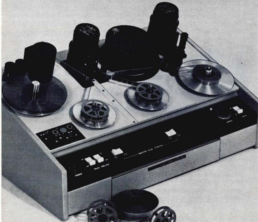
The new Canon Roll Duplicator 800 produces ready-for-use microfilm duplicates at the astonishing rate of 85 feet per minute. Without tying up an expensive Computer-Output-Microfilm system for simple film duplication.
