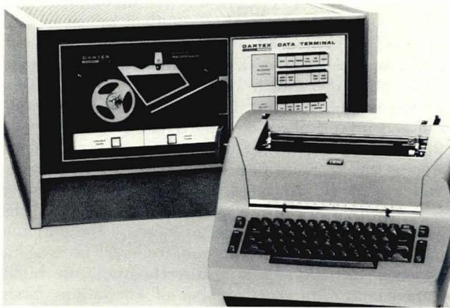
Fig. 3 Free-standing typewriter/cassette system (IBM Selectric and Talley Corp. "Dartex" terminal).
