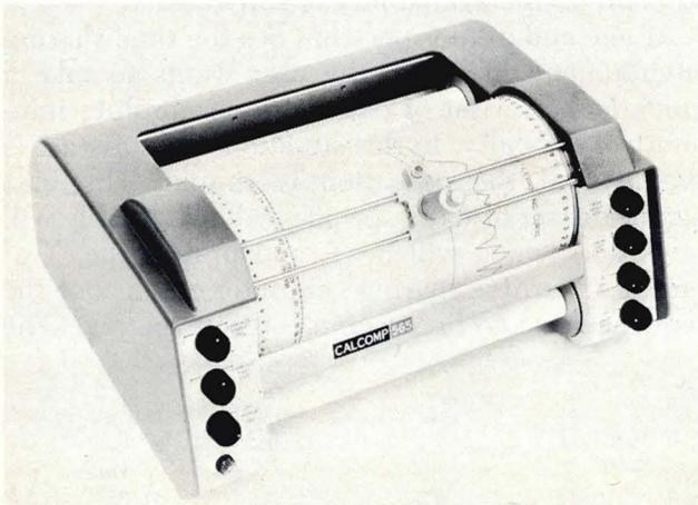
Fig. 3 California Computer Products Model 565 Drum Plotter
