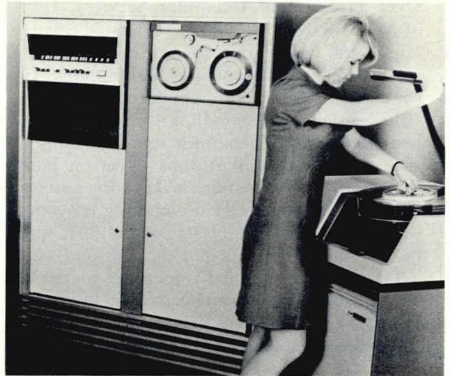
Fig. 4 Central collection and control key-to-disk-to-tape system. (Logic Corp. LC-720.)
