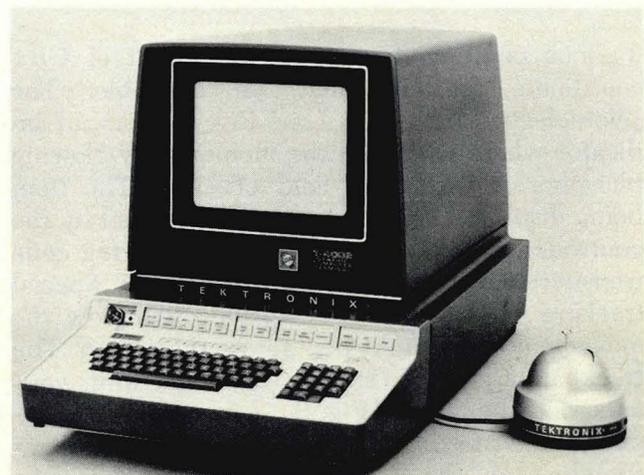
Fig. 2 Tektronix Trackball with T-4002 Terminal
