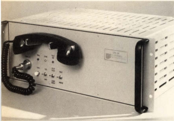
Reduced. E-Systems' LPC-24 speech processor knocks about $2,000 to $3,000 off the price of older generation military units.
