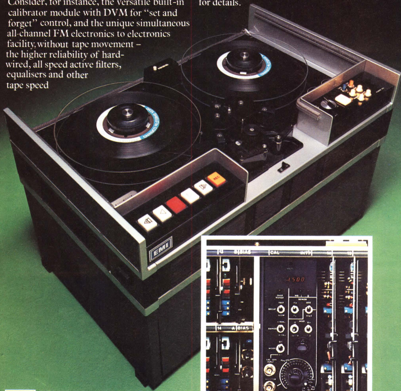
SE 7000M — the only wideband portable with built-in 14 channel electronics to electronics FM calibration and pre-record checkout.
