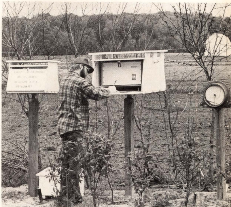
1. Apple protector. This movable, microprocessor-controlled instrument, shown in an orchard, predicts severity of fungus attacks on apple trees. Manual instruments for measuring temperature and humidity are grouped about the new unit, which replaces them.
