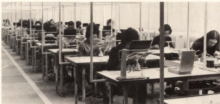
On the line. Hungarian women at the Videoton factory in the ancient town of Székesfehérvár work on printed-circuit boards intended for the firm's line of data-processing equipment.
