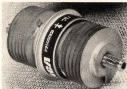
Heat-piped. RCA's 250-ampere rectifier weighs 12 ounces, occupies less than 14 in. 3
