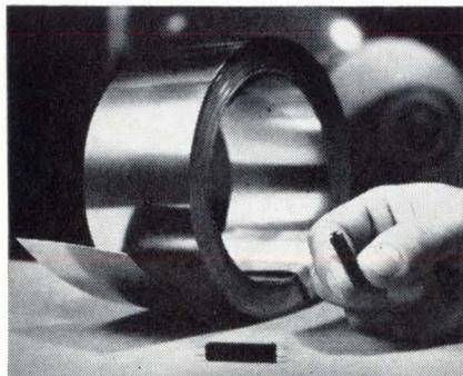
**MAGNETIC MATERIAL.** Remendur, latest member of a large family of high-performance magnetic materials developed at Bell Laboratories, is shown here in sheet form and as element of new telephone switch. A malleable, ductile cobalt-iron-vanadium alloy, Remendur has a remanence of 21,500 gauss.
