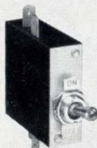
Here, a relay-trip breaker is paired with a NTC thermistor to protect semiconductor circuits in a computer from over-heating. Temperature rise in ventilating air will drop thermistor resistance, raise breaker coil voltage, and cause instantaneous tripping. Breaker contacts open power lines to semiconductor circuits, prevent burnout. Design was chosen as the most economical means of providing high-temperature cutoff with manual reset.
