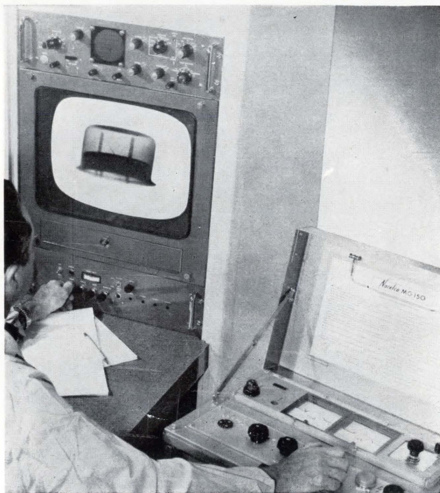
Technician checks transistor on vidicon x-ray television image enlargement system—a product of Philips Electronic Instruments. Diagram at right shows the complete system.
