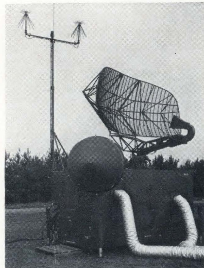
Long-range search radar (AN/TPS-35) which detects and identifies aircraft by displaying range and bearing information on remote scopes. Developed for the 482L system, it will be used in the 407L.
