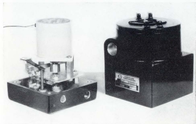
Digital-pneumatic transducer with its cover removed. The stepping motor changes digital signals from the control computer into pneumatic signals of 3 to 15 pounds per square inch by controlling an air nozzle.
