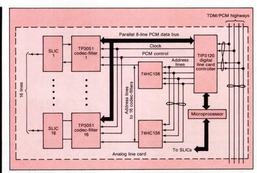
5. An eight-line parallel data bus running between codecs, the line card controller, and TDM/PCM (time-division multiplexing/pulse-code modulation) highways permits the controller chip to handle 16 lines at high speed.
