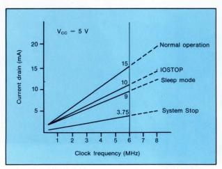
3. At a 6-MHz clock rate and 5-V dc supply, the processor draws 15 mA dc. However, the Sleep mode reduces the current drain to 9 mA, helping to conserve power for battery- and solar-powered applications. IOSTOP, by suspending all I/O functions, cuts current drain to 10 mA. System Stop suspends CPU functions as well, dropping current to 3.75 mA.
