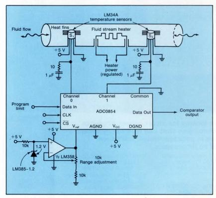
4. The ADC0854 teams up with two thermal sensors to measure the flow rate of a liquid. A differential temperature-measuring circuit enables preset limits to be detected in either direction.
