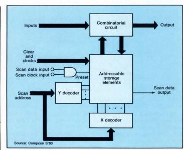
5. A random scan method developed by Fujitsu places all storage elements of a sequential circuit into an addressable array. As each element is serially addressed, test data is scanned in. An important advantage of this technique is that when data is scanned out, the internal states of the circuit are not changed.
