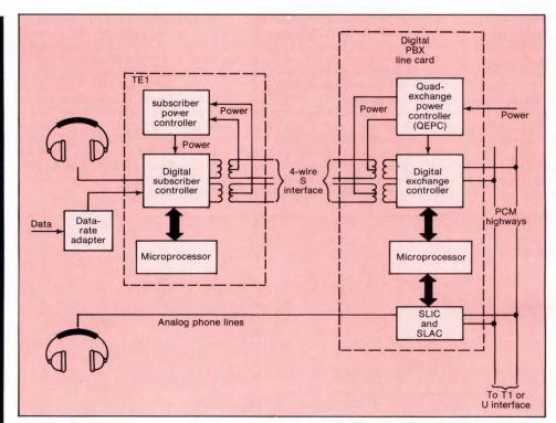
8. In an ISDN-compatible PBX, two chips route the audio signal from the handset to the TDM/PCM highway. The digital subscriber controller chip converts sound into a digital signal suitable for the S interface, and the digital exchange controller puts the digital signal on the highway.
