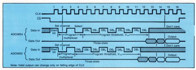
2. In operation, the system microprocessor activates Chip Select (logic 0) and then uses the Data In line to choose first the multiplexer channel (program multiplexer) and then the comparator's threshold value. After 14 clock pulses for the 14-pin device (13 for the 8-pin version), the on-chip logic activates the comparator. Toggling CS through one on-off cycle is enough to ready the comparator for reprogramming.
