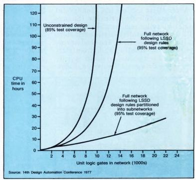
4. Partitioning a complex circuit for test purposes, even when it has been designed for testability, greatly reduces the CPU time needed to generate test programs. In this study concluded by IBM, CPU time rises linearly with gate count when an LSSD design is also partitioned. By contrast, both the unconstrained and full network LSSD designs rapidly reach points where CPU time becomes pronibitive.
