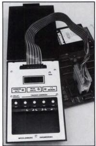
Dackaged in the form of a breakout box, a microprocessor bus-monitoring instrument is a useful debugging aid for real-time control software. since it does not affect the operation of the system under test. The Model 08 is available for use with a variety of 8-bit microprocessors. With some additional parts, the system can be easily reconfigured to accommodate 6502, 6809, 8085, and Z80 de-
