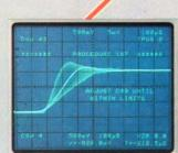
**Envelope Mode.** Displays upper and lower tolerance limits to simplify production testing and calibration. **System:** R7603 with 7D20 Programmable Digitizer.
