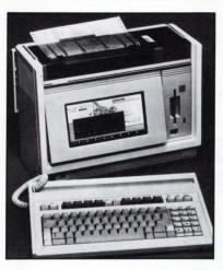
storage. A 25-lb unit 13 in. wide, 16 in. high, and 7 in. deep, it includes a 9-in. electroluminescent display driven by a proprietary
