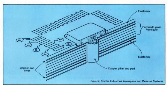
7. With power dissipation increasing, substrates reinforced with copper-clad invar supply an effective way of matching temperature expansion coefficients while still drawing away large amounts of heat from the circuit.
