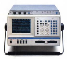
standard general purpose analyzer, now with T12 remote communicator. Allows off-site remote diagnostics.
