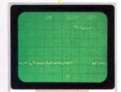
Differential Measurements. High gain differential amplifier captures 5mV signals. System: 7834 with 7A13 Differential Comparator Amplifier.
