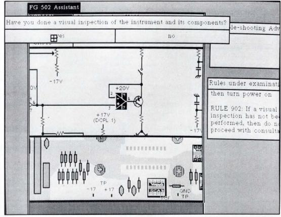
3. Intelligent assistants will soon simplify troubleshooting of electronic equipment. By tying schematic and physical layout together and interpreting test data, such an expert system can multiply a technician's effectiveness.
