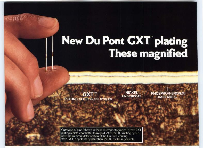
Tests also show the GXT plating system is better than gold in solderability, porosity, bend ductility, and corrosion resistance. Yet GXT can reduce costs as much as 20%.
