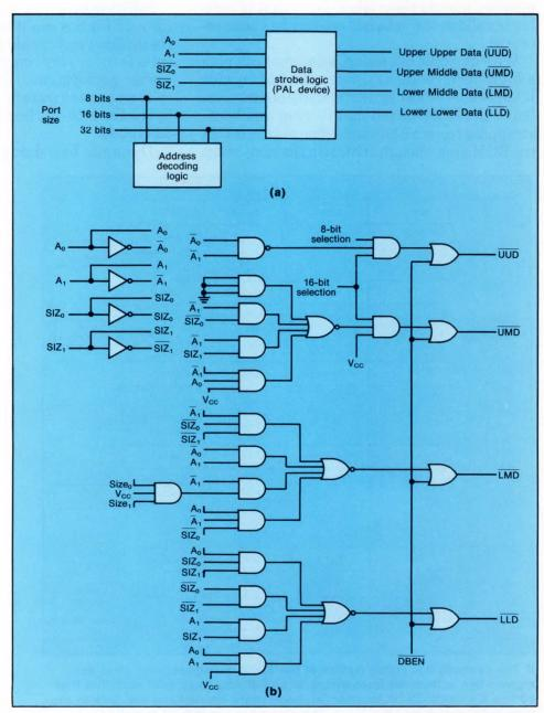
3. The processor must generate up to four separate data strobe signals when fewer than 32 bits are sent out at a time. The strobe signals tell a peripheral or memory device when a byte or word of data is ready. Normally, a single AND-OR-INVERT logic array could generate the four strobes (a), but when high speed requirements prevail, six TTL gates can do the job faster (b).
