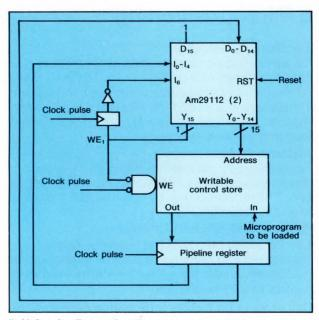
5. Using its Force Continue mode on pin I<sub>6</sub>, the sequencer generates sequential addresses for a writable control store. That permits data to be written into the store faster.
