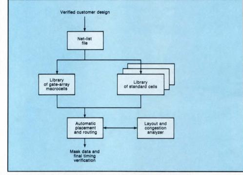
Software makes the best choice between standard cells and gate arrays once a circuit's net list has been created. In either case, the designer gets the benefits of a channelless structure, which yields dense wiring and thus extremely compact chips.
