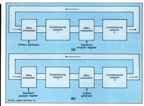
7. Using Bilbo (built-in logic block observation) subsystems, tester functions can be incorporated as part of a chip. In this example, one subsystem supplies pseudo-random test signals to network 1, while the other subsystem acts as a multiple input signature analyzer to gather test results (a). By reversing the functions of the subsystems with control signals, network 2 can be tested also (b).
