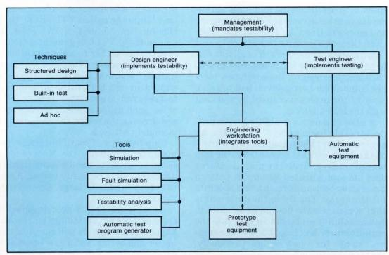
1. The engineering workstation is destined to aid testability by uniting all the elements in the design-test cycle. Important links involving designers and test personnel which are just starting to appear are indicated by the dotted lines.
