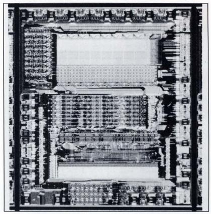
2. The support circuits for the 8086 or 8088 can be constructed on a single chip using both new and existing standard cells. This configuration cuts the pin count to 68, from the over 100 pins associated with discrete components.
