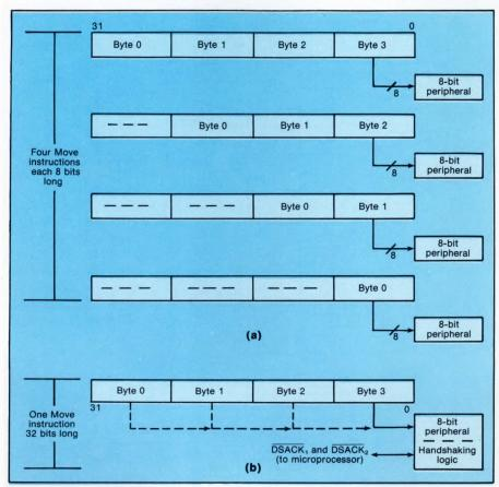
2. The dynamic bus sizing feature of the 32-bit microprocessor gives designers two options for transferring 32 bits of data to an 8-bit port. The first option, a pseudo-32-bit transfer (a), takes more instructions and time to execute but requires less hardware. The second is a true 8-bit transfer (b), meaning that 32 bits are transferred with a single instruction. Additional handshaking logic is needed to generate DSACK<sub>1</sub> and DSACK<sub>2</sub>.
