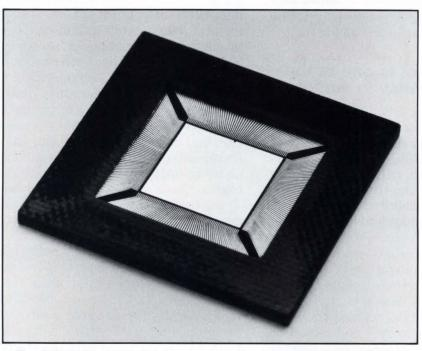
4. The Epic chip carrier from Tectonic and British Telecom breaks away from the traditional use of plastic and ceramic for IC packages. It comes in a range of sizes: 84 pads on 50-mil centers, 132 pads on 25mil centers, and here a 20-mil package with 256 pads.
