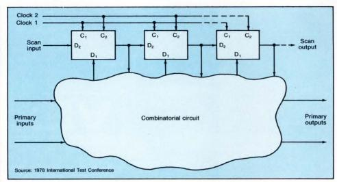
2. In the scan-path technique implemented by NEC, the storage elements have auxiliary data (D2) and clock inputs (C2). During test, the element form a shift register for scanning test vectors in, and test results out using clock 2. Thus, a sequential circuit is transformed into a combinatorial one for test purposes.
