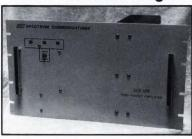
wo rf power amplifiers, the SCA100 and the SCA100V provide output power levels of up to 150 W at 136 to 174 MHz and up to 100 W at 406 to 512 MHz, respectively. The rf drive capability for the SCA100 is 10 W: for the SCA100V, rf drive is 30 to 40 W. A massive heat sink permits cool operation in hot environments, even under 100% continuous-duty conditions. The units come in standard 19-in. rack-mounted enclosures.
