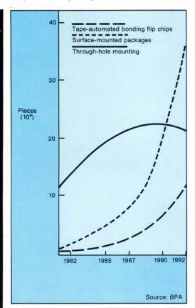
Surface-mounting technology is indeed on the rise, but that does not tell the whole story. The circuits inside the packages will also use the latest semiconductor technologies. DIPs, however, will tend to stay with the older technologies.
