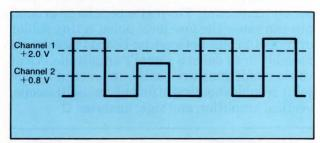
3. To find low-amplitude pulses, the vertical amplifier's NOT CH1 AND CH2 function triggers on any pulse that remains within the TTL transition area (0.8 to 2 V) longer than the period defined by the trigger filter.
