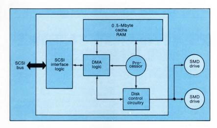
he first SMD drive controller board containing a cache memory of 0.5 Mbyte speeds up data accesses by an order of magnitude or more over other controllers. The ASC-800, from Advanced Storage Concepts, uses 64-kbit dynamic RAMs for the cache; future versions will use 256-kbit chips to provide 4 MBytes of cache memory.
