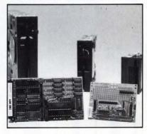
single-board computer with an on-board video controller interfaces directly with a TTL or composite video monitor, eliminating the need for a terminal. The module also includes a 6-MHz Z80B CPU, 64 kbytes of RAM, a floppy-disk controller, and serial and parallel I/O-all on a board that is only 4 by 6 in. The package is supplied with a copy of CP/M 2.2, complete with a customizable BIOS, CP/M utilities, and source code.
