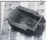
esigned for testing bare substrates on test centers down to 0.010 in., a probe module contains flexible wire contacts in a dedicated housing that matches test points. The wire contacts provide a full travel range of 0.030 in. and have a minimum contact force of 0.5 oz (1.25 oz maximum). The module
