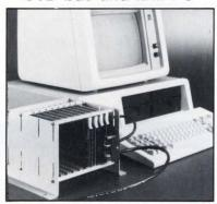
Based on the WD2840 LAN controller chip, a LAN interface card connects the IBM PC with the STD bus for industrial control applications. The card, designated the NETPC/STD, implements a token bus protocol that is similar to Arcnet, but with higher throughput rates (1 Mbit/s) and greater noise immunity. Lengths of up to 1000 ft between daisy-chained nodes are permitted, with a maximum total distance of 10,000 ft.
