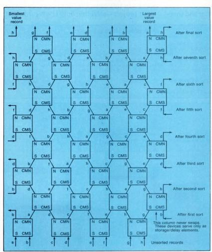
3. The array chip compares the values "a, b, c . . ." along the bottom of each row of processor elements and then rearranges them in the desired rank until the proper values reach the top.
