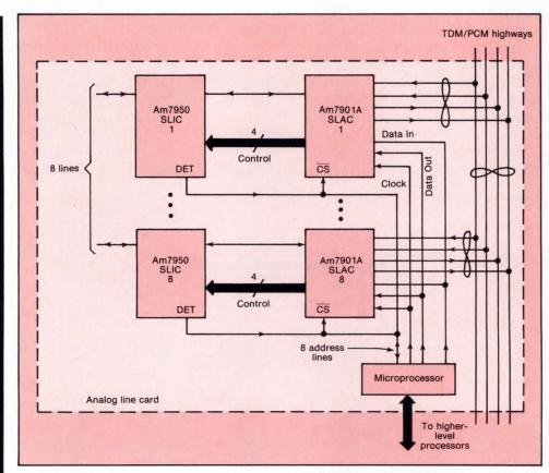
Under the guidance of a microprocessor, eight codecs—actually subscriber line audio processing circuits, or SLACs—can be connected to the TDM/PCM highways without a line card controller. Time slots are stored in each SLAC's memory.
