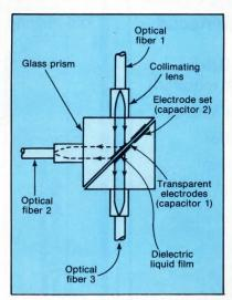
The laser beam being switched is guided by an optical fiber, terminating with a collimating lens, to one side of the first prism. When the liquid dielectric is placed in the path of the incoming light beam, the beam passes ultimately to the optical fiber.
