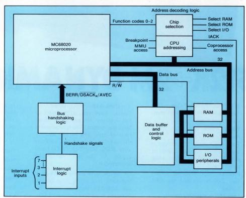
4. A simple yet powerful microcomputer system centers on the 68020. Both RAM and ROM sections are implemented as 32-bit-wide memories, with data transfers under the control of the data buffer and control logic. The peripherals, however. use a simple 8-bit bus, because they are accessed relatively infrequently compared with the memory devices.
