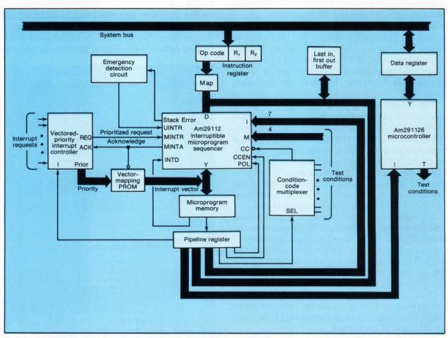
4. A single-level pipelined system, designed around the Am29112 and the Am29116 16-bit microcontroller, allows one microinstruction to be executed while the next instruction's address is generated and accessed. The Am20112 generates the microprogram memory addresses for the next microprogram to be executed.
