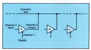
2. Bus contention occurs when two or more devices try simultaneously to drive a common bus. The vertical amplifier generates a trigger whenever the device's output does not match its input after it has been enabled. A special filter in the amplifier prevents inadvertent triggering caused by propagation delay through the buffer.
