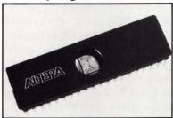
Designed with CMOS EPROM technology, a reprogrammable logic device has 1200 gates and more than 14,000 reprogrammable bits. Designated the EP1200, the array features dedicated latchable inputs, local and global communications, product-term sharing, buried registers, and programmable I/O structures. The device-which comes in a windowed 40-pin ceramic DIP—is capable of operating at speeds above 16 MHz, while dissipating only 400 mW in the active mode. Standby power dissipation is only 15 mW.
