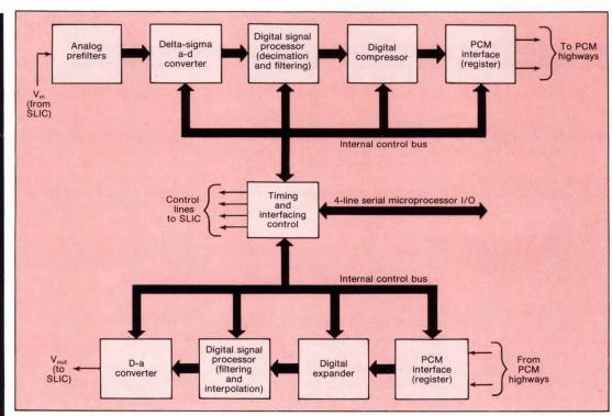
7. A SLAC tackles virtually all normally analog functions in an on-chip digital signal processor. Its functions include filtering and companding the signal after it has passed through the analog-to-digital converter.
