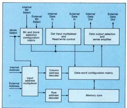
To make the memory as flexible as possible, decoding logic is programmed during metalization. The logic determines the word width and the widths of the memory core's on- and off-chip interfaces.
