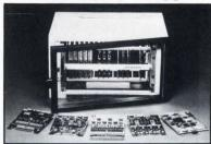
Operating as a stand alone process computer or as a remote front end for distributed control and/or data acquisition, the Safe 8000 replaces program-
