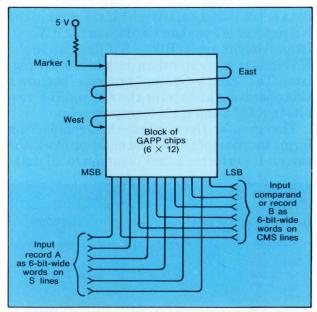
2. The chip can accept and process input record A, which comes from memory, and the comparand or input record B. If it cannot complete the processing in one pass, the signal can be wrapped around and run through again.
