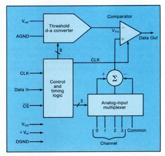
1. Timing and control logic in the 14-pin ADC0854 and the 8-pin ADC0852 comparator ICs offloads a system microprocessor of most of its analog control functions. Nevertheless, the processor is still responsible for initially setting both the comparator threshold (via the digital-to-analog converter) and the channel multiplexer. The 8-pin device unites COM and the two ground lines, omits channels 2, 3, and  $V^{+}$ , and combines  $V_{\rm ref}$  with the  $V_{\rm CC}$  line.
