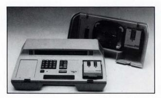
universal programmer allows an engineer to program over 99% of all existing programmable logic devices, including PROMs and PAL and IFL (integrated fuse logic) devices. The Model 60A, made by Data I/O, is available with a handler interface for programming parts in production quantities.
