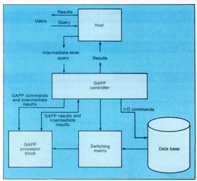
5. Systolic array chips can be called into duty in a data-base management system, forming a processor block, a controller, and a switching matrix. The matrix prepares data for array processing.
