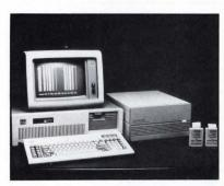
Costing less than most standalone logic analyzers, the MicroAnalyst workstation integrates the power of an IBM PC AT with the Series 2000 logic analyzer and a Lotus-based general-purpose software package. Five software functions—spreadsheet, data base, word processing, graphics, and communications—allow the user to perform complex data analysis.
