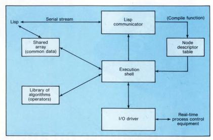
1. A front-end package adds real-time capabilities to a Lisp-based system through a communicator, an execution shell, and an I/O driver. Each processing point, or node, is listed within a descriptor table, and a library of algorithms contains the C code for the system's basic operators.
