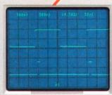
Counter/Timer. Oscilloscopecontrolled counter/timer permits measurements to counter accuracy on displayed waveforms. **System:** R7603 with 7D15 Universal Counter/Timer.
