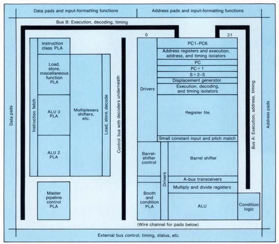
4. One of the first dedicated RISC processor chips, from MIPS, replaces much of the usual memory-fetch logic with registers. The chip halves the number of transistors on a 68000 yet delivers the same processing power.
