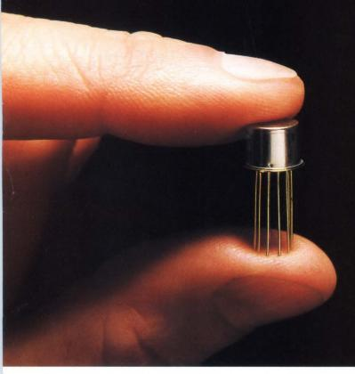
Our little magnetic latching TO-5 relay simply never forgets. Once it's set with a short pulse of coil voltage, Teledyne's Maglatch TO-5 will retain its state until reset. Even if system power fails or is shut off.
