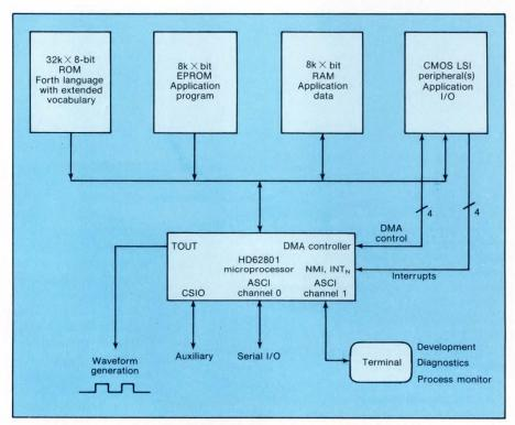
4. A Forth-language computer fabricated entirely in CMOS serves as an industrial controller with built-in development capability. A 32k-by-8-bit ROM holds the language itself; an 8k-by-8-bit EPROM stores the application program; and an 8k-by-8-bit RAM holds data. Using byte-wide memories ensures rapid matching of application requirements.
