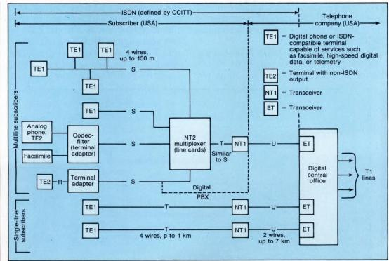
2. A complete ISDN line transmits signals on two voice or data channels at 64 kbits/s full duplex. An additional 16-kbit/s packet-switching data channel carries control and signaling information.
