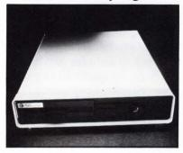
nabling users of stand-alone CP/M-based computers to enter a multi-user, multitasking environment while protecting their hardware and software investments is the MC-186, a dual-processor computer capable of handling both 8- and 16-bit programs. When networked to the MC-186, IBM PC-compatible computers can run both CP/M and PC-DOS programs.
