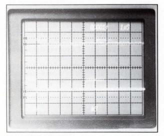
4. The vertical amplifier snares a low-amplitude pulse out of a busy data stream.
