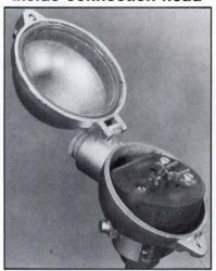
A remote conversion unit for potentiometers and sensors fits into standard industrial connection heads and takes its power from the signal voltage. The LP01 standard model is designed for potentiometers with a total resistance of 2 to 5  $k\Omega$ , with units for other resistances available on request. It converts the potentiometer setting into a standard 4-to-20-mA signal. A fault in the potentiometer will cause the output signal to fall below 4 mA or to rise above 20 mA.
