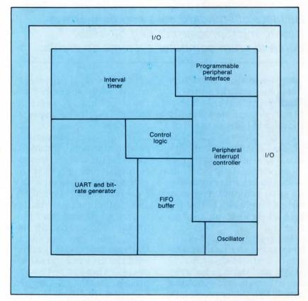
1. Using NCR's standard-cell library, including its recently introduced CMOS 6502 microprocessor core, a semicustom chip—complete with analog functions, I/O, and all the components necessary for running the microprocessor—fits onto a single 50,000-mil<sup>2</sup> chip.
