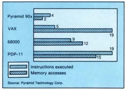
3. The ratio of instructions executed to memory accesses is higher for a reducedinstruction-set computer (in this case the Pyramid 90x) than for a VAX, a 68000, and a PDP-11. The smaller number of memory accesses means fewer procedure calls and parameter returns.
