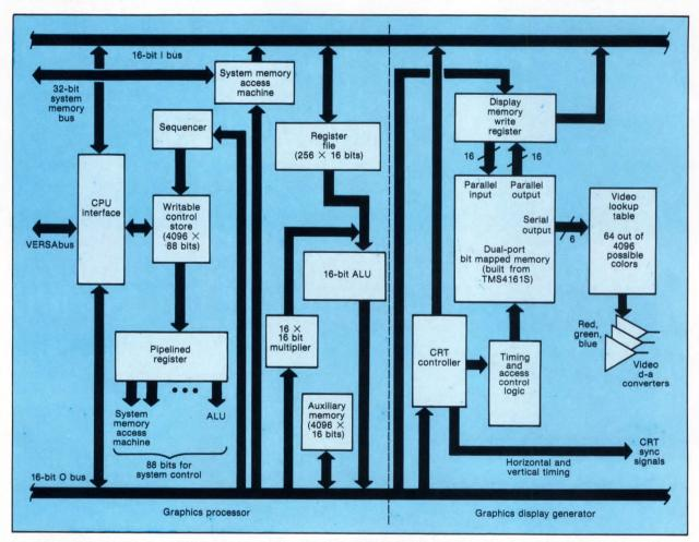
An internally pipelined multiprocessor and multiple-bus architecture helps the graphics and display subsystem of a graphics accelerator handle 400,000 clipping operations and transformations each second. At that speed, images can be manipulated almost instantaneously.
