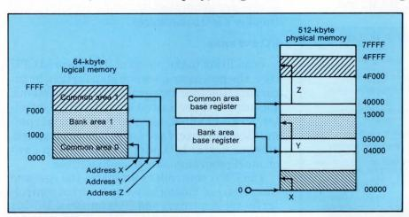
2. The on-chip memory management unit eliminates the 64-kbyte address limit associated with 8-bit microprocessors. Using it, a designer defines three areas within the 64 kbytes of addresses and maps two of them-the bank area and common area 1-into a 512-kbyte address space. The starting address of each mapped area is set by a base register, and boundaries are established at 4-kbyte intervals.
