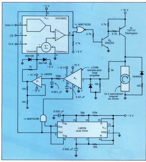
5. In an application for which it is particularly suited, the ADC0852 controls the speed of a dc motor. A sensing loop in the controller detects back EMF, ensuring that the circuit remains insensitive to changes in line voltage and loading.
