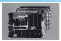
6809 Single Board Computer. 6809 MPU, 2 serial ports, 4 parallel ports, RAM, EPROM, real-time clock, watchdog timer, 44-pin 4.5" × 6.5" PCB. EXPANSION MODULES: RAM, EPROM, CMOS RAM/battery, analog I/O, serial I/O, par-allel I/O, counter/timer, IEEE-488, EPROM programmer, floppy disks, cassette, breadboard, keyboard/display. Wintek Corporation, 1801 South Street, Lafayette, IN 47904-2993. (317) 742-8428.
