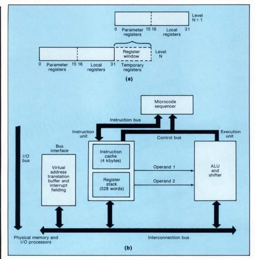
1. Overlapping the register windows on the Pyramid 90x allows data to pass from a temporary register to the top of a stack without a memory-access cycle (a). The machine's instruction bus ensures that fetches and executions proceed rapidly and independently of each other (b).
