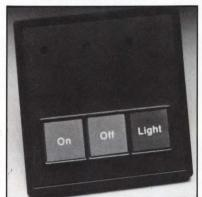
ermanently molded into a bezel for front-panel mounting, a control-display module contains a user-specified number of dome switches, LED indicators, electronic components, and a pin connector. The dome switches are actuated through auxiliary external circuitry to deliver up to 10 mA at 24 V dc to the terminals of the built-in connector. Actuation of the switches also illuminates the respective LED indicator. The normally open SPDT switch contacts have a resistance of less than  $100 \Omega$ .
