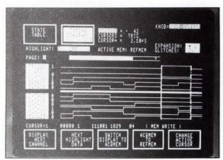
5. The logic analyzer's ability to display pretriggering data comes to the fore in pinpointing an intermittent fault. When a low-amplitude pulse is detected by the scope, it sends a trigger pulse to the logic analyzer to initiate data acquisition. The events leading up to the scope trigger are displayed on the analyzer's screen.
