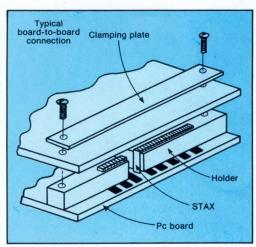
3. In yet another instance of using elastomerics as connectors, Flexicon Systems' alternate conductive and nonconductive strips squeeze up to 250 connections into an inch. Once the bolts are inserted, the connectors are self-aligning.
