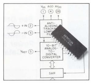
or the first time a monolithic a-d converter does not require a supporting anti-aliasing filter chip. The RT5640, a 10-bit device from EG&G Reticon, incorporates a high-performance switchedcapacitor filter that is tunable over the range of 20 Hz to 15 kHz (ELECTRONIC DESIGN, Sept. 6, p. 205). Thus it serves handily the needs of 8- and 16-bit microprocessors undertaking the complex signal processing necessary for such applications as speech recognition and sonar.
