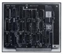
ne of the fastest encryption devices currently available, the WD2200 data security board allows personal computer users to control or prohibit access to data files. The board, which is based on the NBSapproved WD2001 data encryption chip, operates at a data transfer rate of 1.3 Mbits/s.
