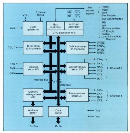
1. The HD62801 combines an enhanced central processing core (compatible with the Z80) and four major I/O subsections. The core's memory management unit expands a logical address space of 64 kbytes into one of 512 kbytes. The I/O features include a DMA controller, high-and low-speed serial ports, and dual counter-timers.
