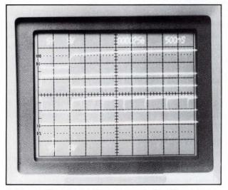
1. The oscilloscope, when connected to three control lines and to the strobe output of a microprocessor system, reveals normal logic levels. No crosstalk or ringing is evident.
