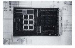
**68008 Single Board Computer.** 100 by 160mm Eurocard. 3 RAM/EEPROM/EPROM sockets for 2K-64K byte devices (2K RAM included). 6 8-bit Bi-Dir I/O ports with handshake and individually vectored interrupts. 4 16-bit timers. Dual async serial RS232 ports. 256b nvRAM. Diagnostics LEDs. Multitasking kernal option. \$295/unit. Quantity discounts available. Heritage Systems Corporation, P.O. Box 10588, Greensboro, NC 27404. (919) 274-4818.
