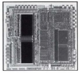
ased on the popular 8-bit 8051, the Am 9761H contains 64 kbits of EPROM, the largest amount of EPROM storage available on a single-chip microcomputer and twice the amount on the EPROM version of the 8051, the 8751. Consequently, it can take on new and larger control applications while saving the designer 12 to 16 weeks' lead time over a standard ROM-based implementation.
