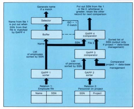
4. A configuration of parallel processor building blocks can tackle data-base tasks. Here four chips search through two files to find the names of workers involved in a data-base management project.
