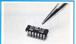
CMOS IC GENERATES CALL PROGRESS TONES. Generate audible ringing and other callrouting tones such as dial, busy and reorderwith just one chip. Teltone's M-991 produces combinations of seven standard frequencies using one 5V supply and a 3.58 MHz crystal. As the only tone generator on the market, it joins Teltone's family of telecommunications generators, detectors, receivers and relays. 1-800-227-3800, ext. 1130. Teltone Corporation, P.O. Box 657, Kirkland, WA 98033.
