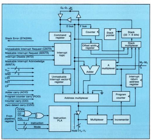
1. The Am29112 interruptible microprogram sequencer chip is a mixture of conventional and new logic functions. To improve its ability to handle interrupts, the chip carries enhanced interrupt logic and a very deep stack—33 levels—that allows nesting of interrupts and subroutines.
