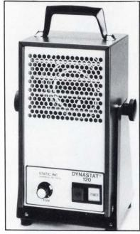
Smaller and lighter than most units, the Dynastat 120 series of ionizing air blowers incorporates a fixed or adjustable 100-cfm fan that provides a smooth flow of ionized air to control static electricity. Adjustable fan speeds range from 50 to 100 cfm.
