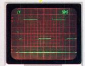
Glitch Capture Application. Unique logic triggering solves problems caused by abnormal pulses. System: 7834 with 7A42 Logic-Triggered Vertical Amplifier, 7D11 Digital Delay Unit.
