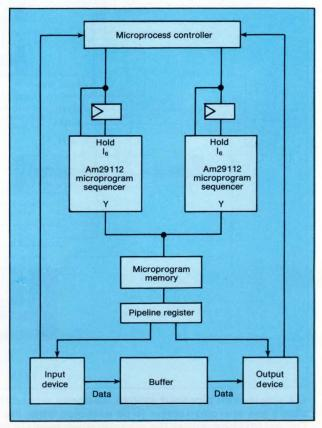
3. Two AM29112s can process in parallel through a buffer. In such a system, one sequencer is active, while the second is on hold. Time multiplexing enables one sequencer to handle input operations; the other is responsible for outputs.
