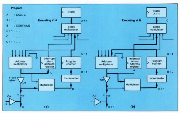
2. While the microprogram sequencer is executing the instruction CALL C at program location A (a), an interrupt enters and redirects execution to the instruction CONTINUE at program location B (b). The return address (A+1) of the interrupted routine is saved on the stack, but the first instruction (B:CONTINUE) of the interrupting routine must not use the stack, which is being preempted by the return address already pushed onto it.
