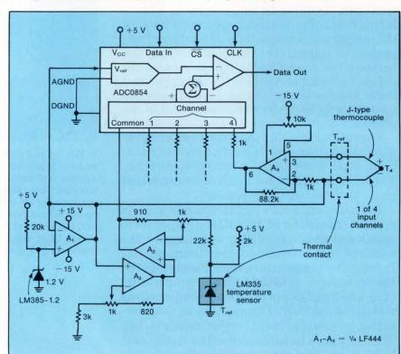
3. One comparator IC can monitor up to four compensated thermocouples in a system that detects whether an oven or refrigerator is operating below or above a certain temperature. Each sensor can be assigned its own trip point within the range of 0° to 300°C.
