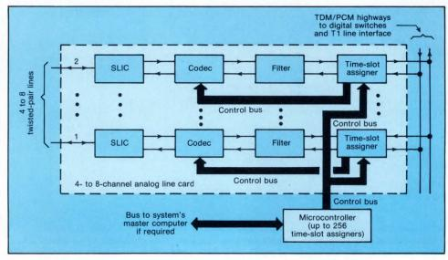
3. Analog line cards convert telephone signals into time-division-multiplexed, pulse-code-modulated (TDM/PCM) signals at central offices and in PBXs.
