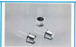
MIL SOLID STATE AC/DC RELAY Teledyne's M640-1W features AC/DC switching up to 40V, & low on resistance (2 ohms typ), Transformer coupling provides 1000VAC isolation & low offstate leakage. Hybrid microcircuit assembly to MIL-883B in TO-5 case. MIL P/N M28750/5-001 on QPL. The M640-1W is used as data coupler, isolated line driver, current loop switch, analog & transducer signal switching. \$38 ea for 500 pcs. Teledyne Solid State Products, 12525 Daphne Ave., Hawthorne, Ca, 90250 (213) 777-
