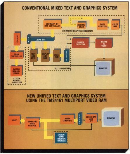
**Major reductions** in system component count and board area are achieved by using the TMS4161 Multiport Video RAM in the unification of graphics and text into a totally bit-mapped system.
