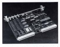
is turned off while the display is being built up) with an average writing speed of 900,000 dots/s. It holds in ROM 95 eight-byseven-dot ASCII characters, the sizes of which are programmable from 1 to 16 dots in each direc-
