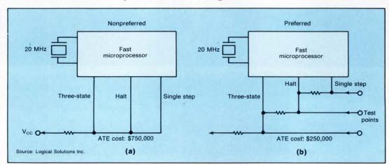
8. Something as simple as tying a microprocessor's control lines to V<sub>CC</sub> or ground can cause testability problems. A high-speed functional tester must be used when the microprocessor cannot be controlled (a). Bringing out test points for control purposes allows a lower-cost static functional tester to be used (b).
