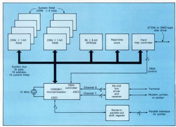
5. In a desktop or rack-mounted setting, the microprocessor, standard NMOS 256k-by-1-bit dynamic RAMs, and a banked operating system form the foundation of a small high-performance computer. The 6-MHz clock yields a minimum instruction cycle of 500 ns. To serve multiple users a UART can be added for each extra terminal.
