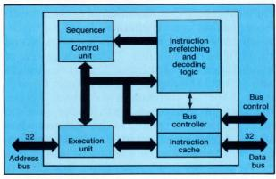
1. The MC68020's interface dramatically simplifies the designer's job. The 32-bit-wide data and address buses prove invaluable, and they get assistance from logic that dynamically controls the width of the bus. Also, an instruction cache helps reduce the number of external bus cycles overall.
