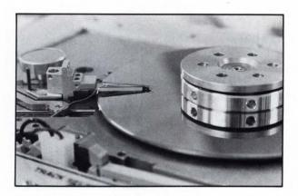
write heads is one of the first to meet the needs of advanced hard-disk drives having densities in excess of 1200 tpi. The 1200 series, an addition to Read-Rite's RR-1212 line, will handle a data track width as thin as 250 µin.
