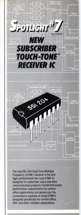
The 14-pin SSI 204 is a complete DTMF. It detects all 16 standard digits, with excellent speech immunity and no front-end filtering. To operate the 204, the only externally required components are an inexpensive 3.58-MHz frequency reference crystal and a bias resistor. The 204's 5-volt power requirement and 3-state outputs make it ideal for microprocessorbased systems.
