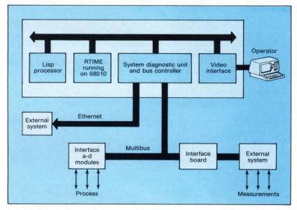
2. RTIME is designed to run on a 68010 coprocessor, which is part of the Lambda machine. It allows users to program real-world events in Lisp. The package interfaces with sensors and process controllers through the Multibus, with a host system through Ethernet.
