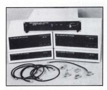
Comprising four Token/Net interface modules, a translator head-end, and broadband cabling, a local area network starter system allows the evaluation of an IEEE-802.4 broadband token-bus network. The Token/Net interface module (TIM) contains a 5-Mbit/s rf modem, a media-access unit that implements the token-passing access method, and a
