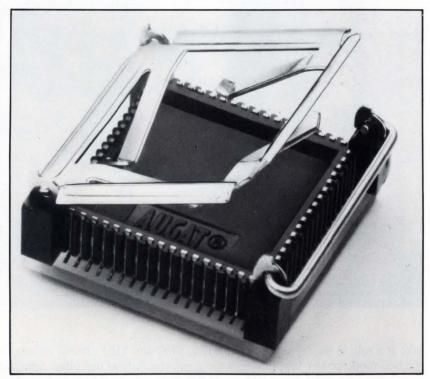
6. A more conventional socket for leadless chip carriers, this one from Augat Components, has an open-side insulator for good heat dissipation and for inspection of the solder joints.
