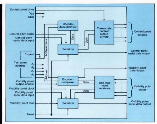
6. The Turino (Totally Universal Reset, Initialization and Nodal Observation) circuit has been proposed by Logical Solutions to interface the control and visibility points of a circuit to a standard testability bus. All connections to the circuit other than the control point outputs and visibility point inputs, are for the testability bus.
