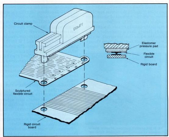
2. One of the first surface-mounted edge connectors, developed by Dowty Electronic Interconnect, shuns current approaches and instead uses elastomeric pressure pads to make contact between the board and the flexible circuit.
