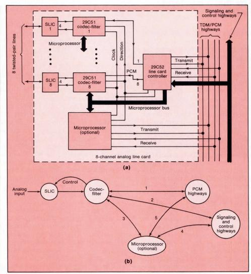
4. Third-generation line cards combine codec-filter functions on one chip and put eight time-slot assigners on a line card controller (a). A microprocessor on the card adds local control. The overall architecture equips the card with five separate signal and control paths (b).
