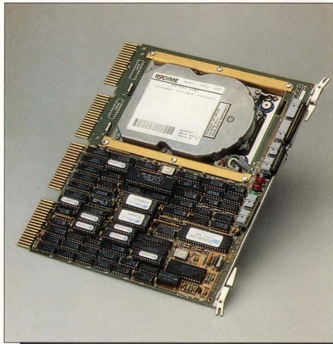
**The CMD hard card. The drive projects three slots on the other side of the card. A second drive can connect to the edge connectors, but must get power elsewhere.**
