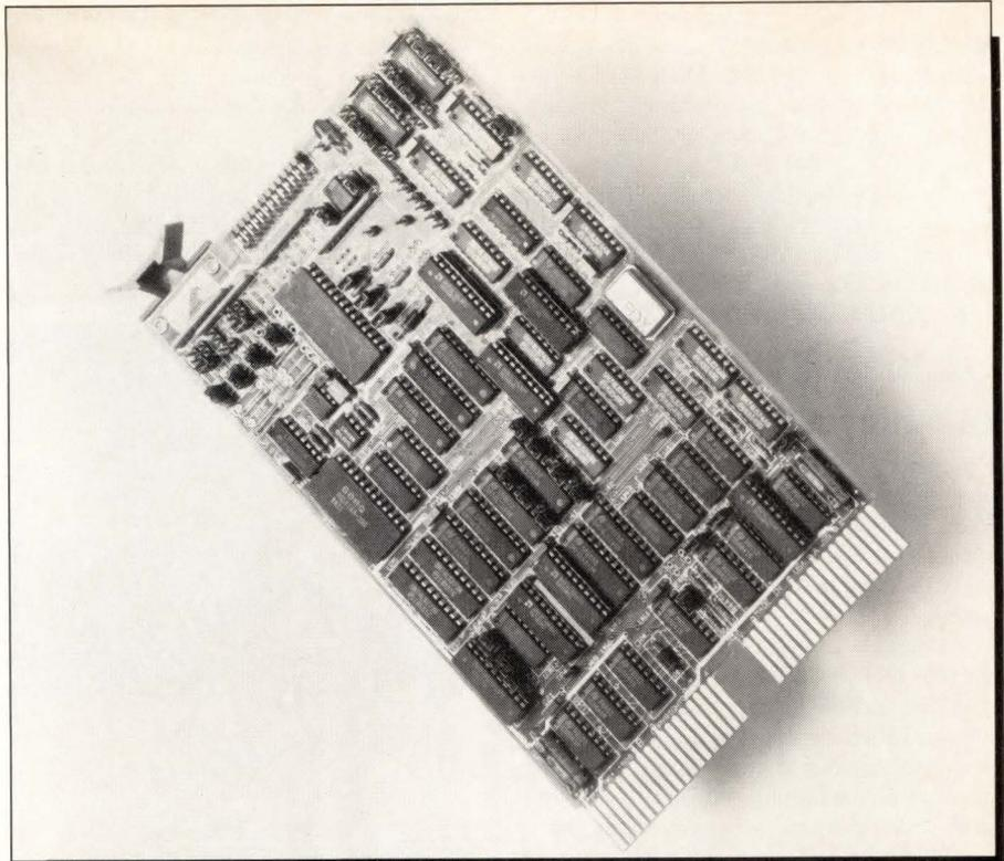
*Codar Technology's Model 190 System Channel Monitor provides 16 channels of high-speed 8-bit A/D to MicroVAX/Q-bus users.*
