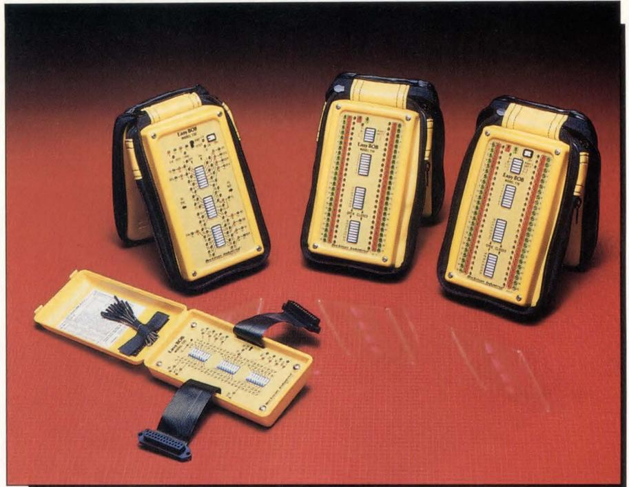
*The breakout box line from Beckman Industries, Brea, California, is the 100 LED-type enabling all 25 lines on both sides of the interface to be monitored.*
