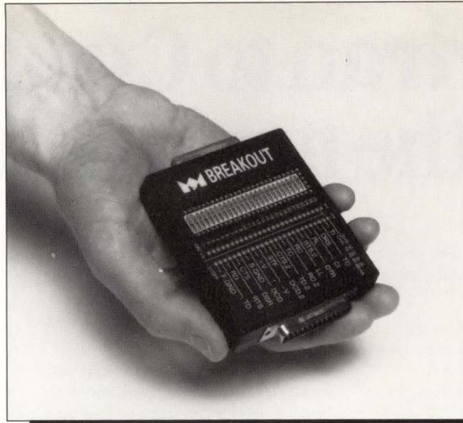
*M-Breakout — a complete RS-232/V24 interface troubleshooter can break and cross-patch all 25 lines from M-Test Equipment, San Francisco, California.*
