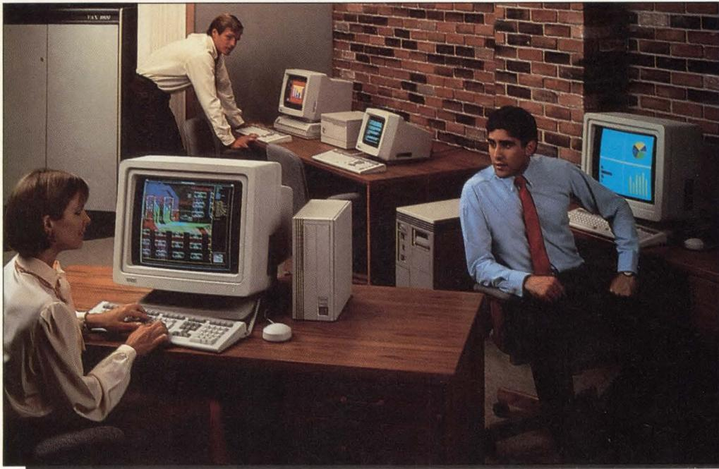
*Both the VAXSTATION 2000 workstation (foreground) and the MICROVAX 2000 system (man standing) can be integral links in DEC's Local Area VAXcluster environment. Work group users are able to cluster and share resources with other DEC workstations (VAXSTATION II/GPX system, right) and larger VAX systems (VAX 8800 system, far left).*
