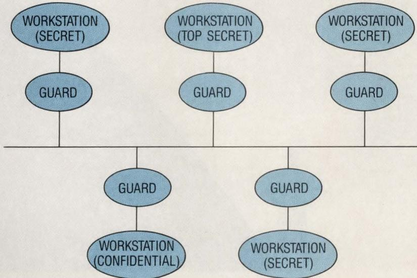
*A Secure LAN. Information doesn't flow from a workstation with a low classification to one with a higher level.*
