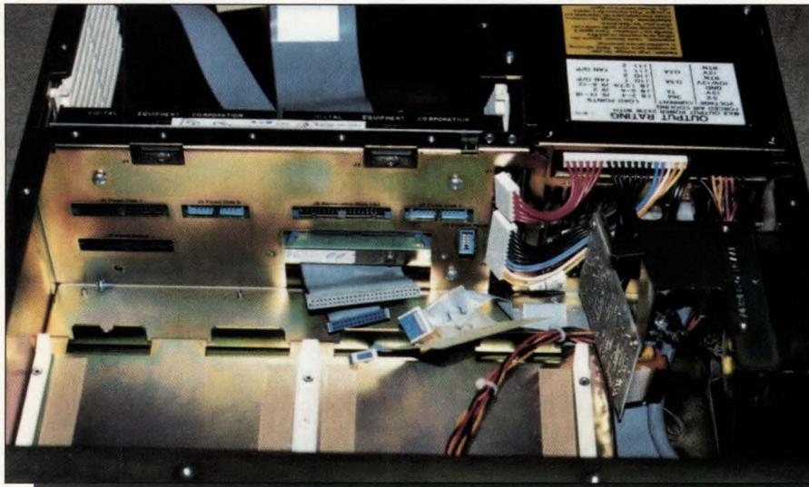
*Replacing the backplane means almost total disassembly of the BA23 components. Here, all CPU cards and disk drives are out and all that remains is the disk cable distribution panel.*
