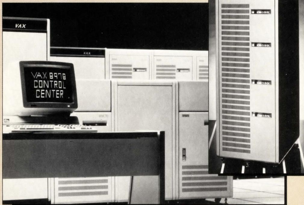
*DEC's new VAX 8978 provides 50 times the power of the 11/780 and includes DEC's highest capacity storage subsystem, the SA482.*
