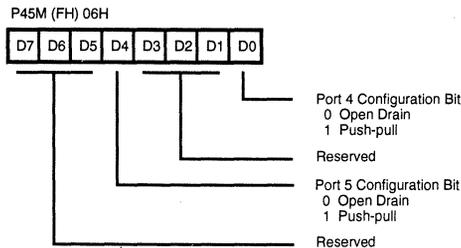
Figure 19. Port 4 and 5 Configuration Register (F) 06H [Write Only]
