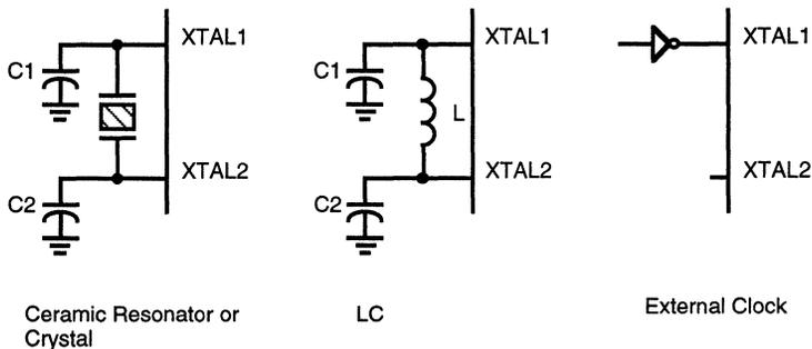
**Figure 16. Oscillator Configuration**
