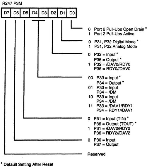
Figure 72. Port 3 Mode Register (F7H:Write Only)
