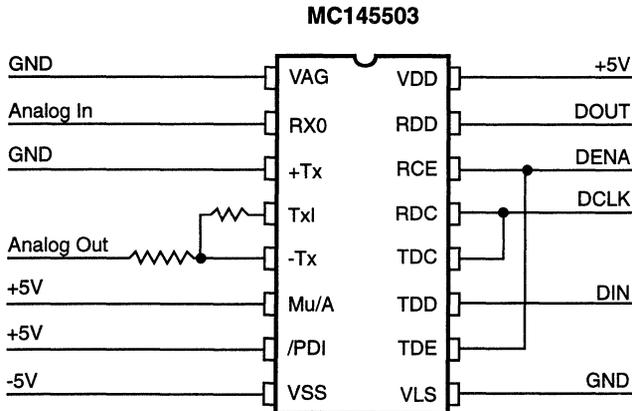
**Figure 26. Connecting TCM29C18 and MC145503 to Z89C67/C68**
