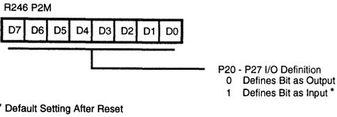
Figure 71. Port 2 Mode Register (F6H: Write Only)
