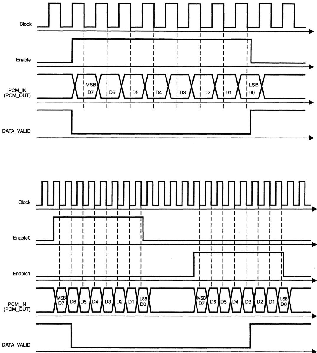
Figure 27. Timing Diagram of Codec Interface
