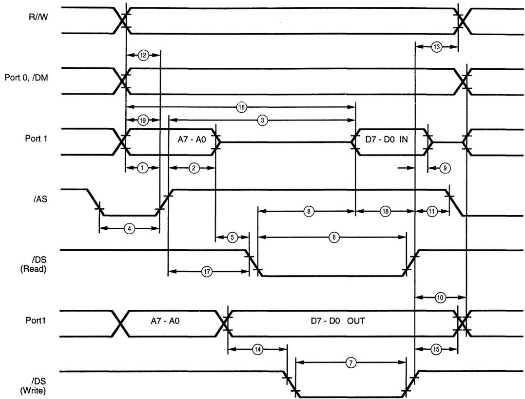
**Figure 37. External I/O or Memory Read/Write Timing**
