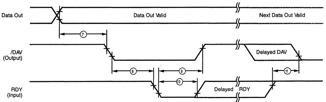
**Figure 36. Output Handshake Timing**
