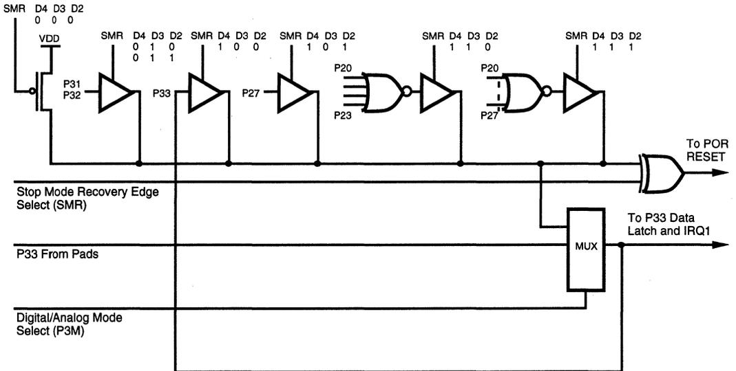
Figure 21. Stop-Mode Recovery Source
