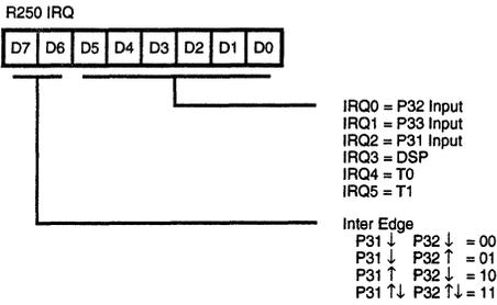
**Figure 75. Interrupt Request Register (FAH:Read/Write)**
