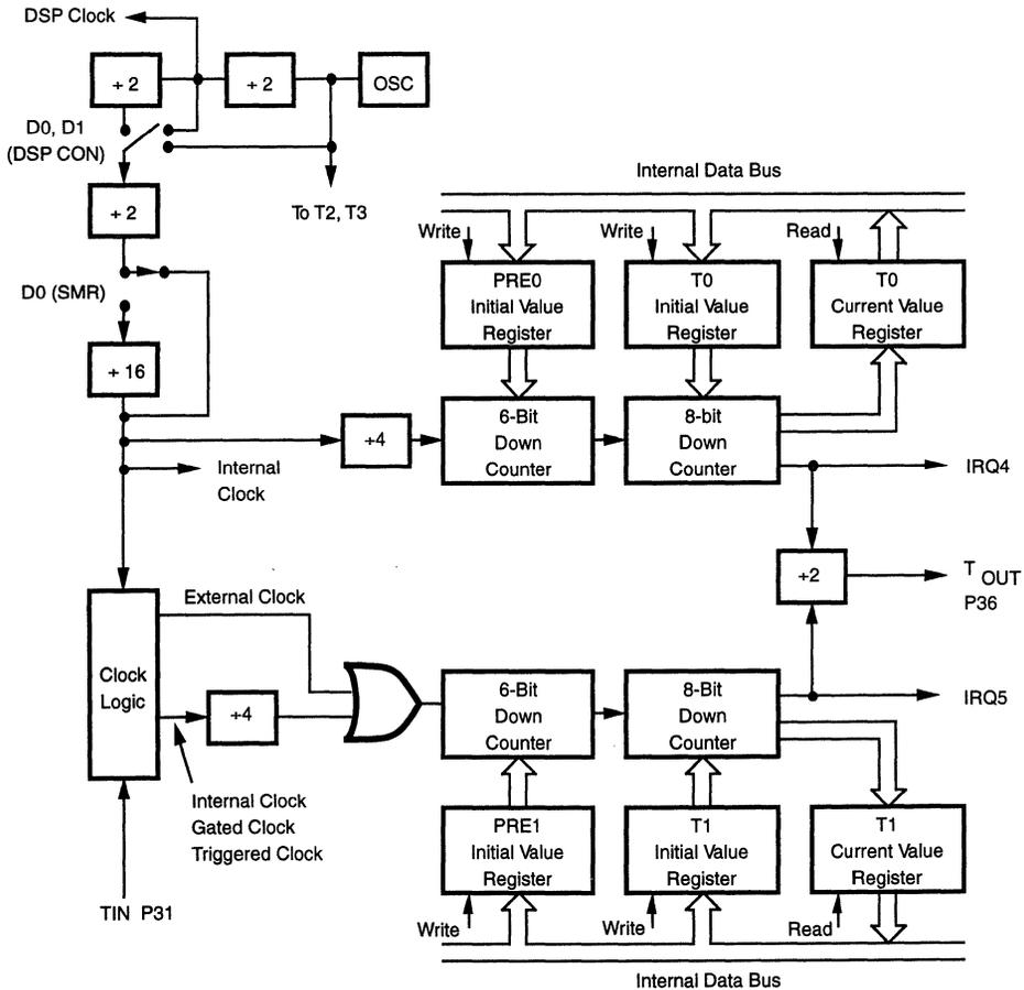
Figure 17. Counter/Timer Block Diagram
