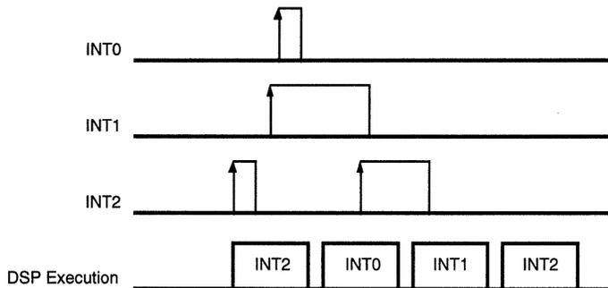
Figure 23. DSP Interrupt Priority Structure
