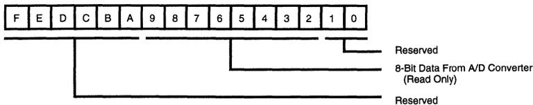
**Figure 29. EXT5 Register A/D Mode Definition**
