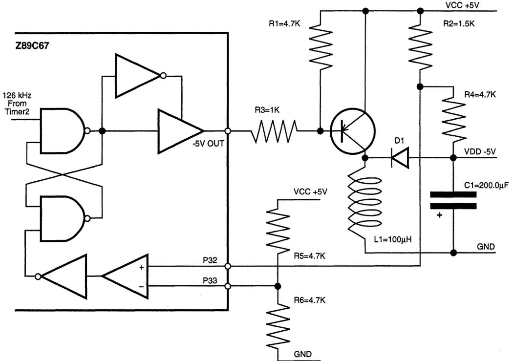
**Figure 29. Circuit Diagram for  $-5V$  Generation**
