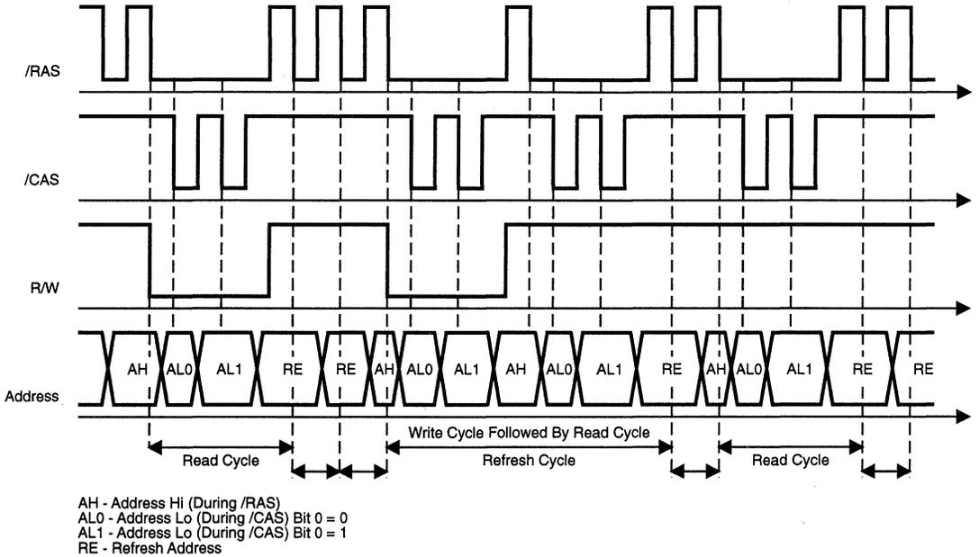
**Figure 30. Timing Diagram for ARAM Interface**
