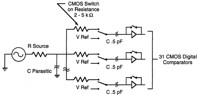
Figure 35. Input Impedance of ADC
