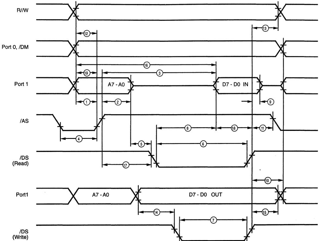
**Figure 33. External I/O or Memory Read/Write Timing**
