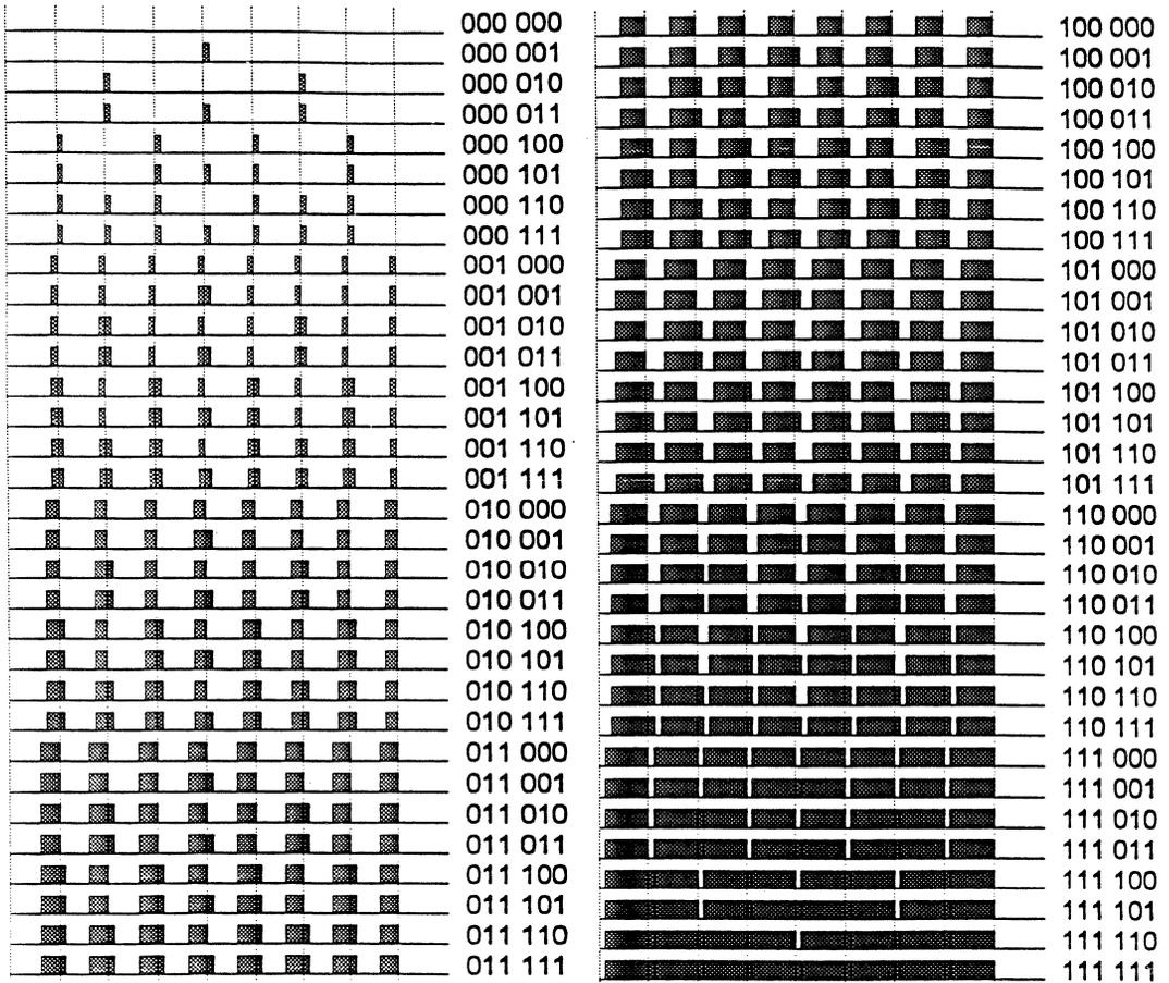
Figure 25. PWM Waveform of the Active Region
