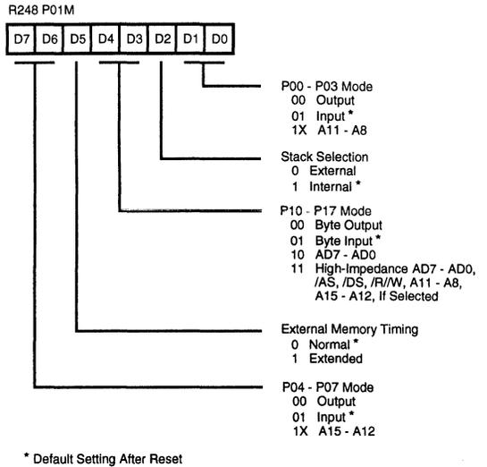
Figure 73. Port 0 Mode Register (F8H:Write Only)
