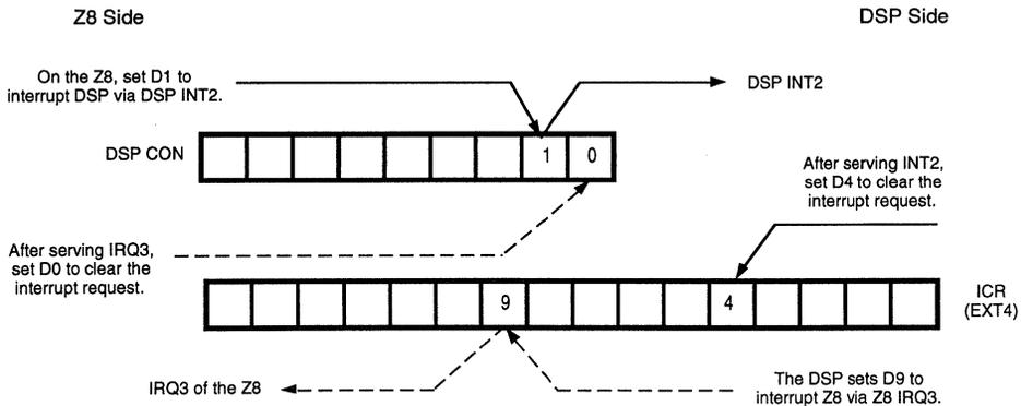
Figure 27. Interprocessor Interrupts Structure
