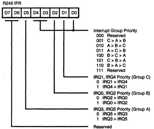
Figure 74. Interrupt Priority Register (F9H:Write Only)
