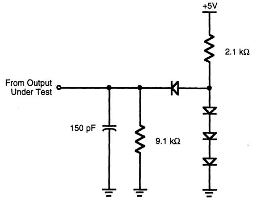
Figure 36. Test Load Diagram
