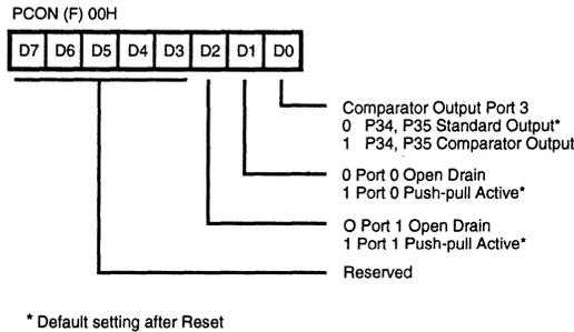
Figure 18. Port Configuration Register (PCON)
