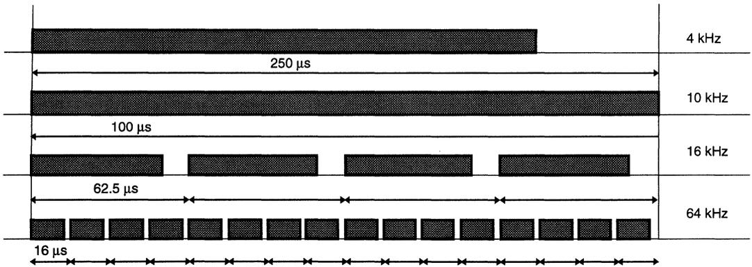
Figure 24. PWM Waveform (shaded area shows the active region)
