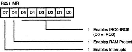
**Figure 76. Interrupt Mask Register (FBH:Read/Write)**
