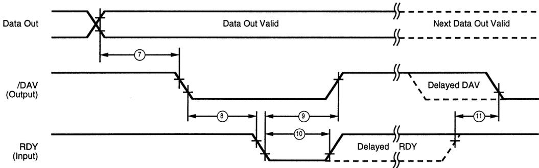
**Figure 40. Output Handshake Timing**
