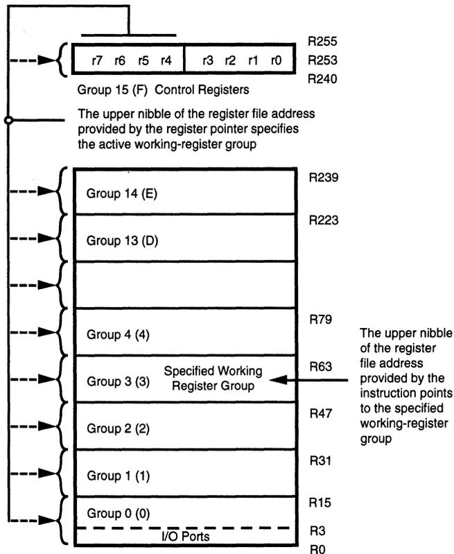
**Figure 13. Register Pointer**
