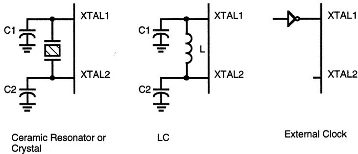
**Figure 16. Oscillator Configuration**
