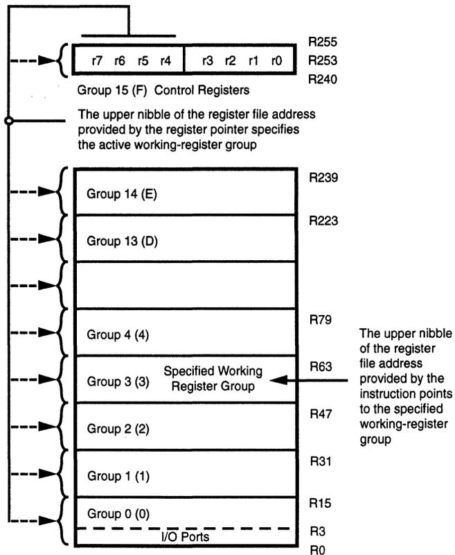
**Figure 13. Register Pointer**
