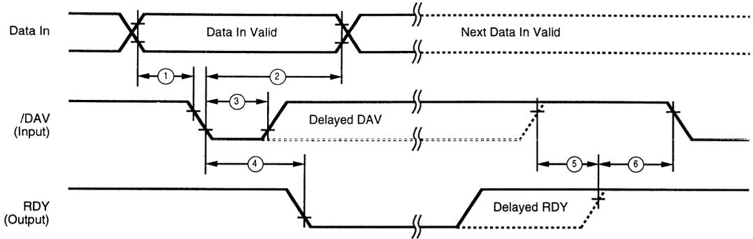
**Figure 39. Input Handshake Timing**
