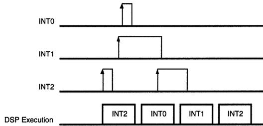
Figure 26. DSP Interrupt Priority Structure
