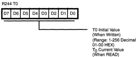
Figure 27. Counter/Timer0 Register (F4H: Read/Write)
