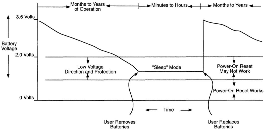
**Figure 4. Low Voltage Detection and Protection**
