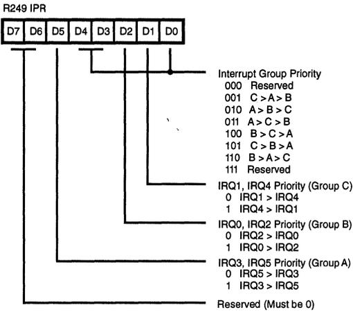
Figure 32. Interrupt Priority Register (F9H: Write Only)
