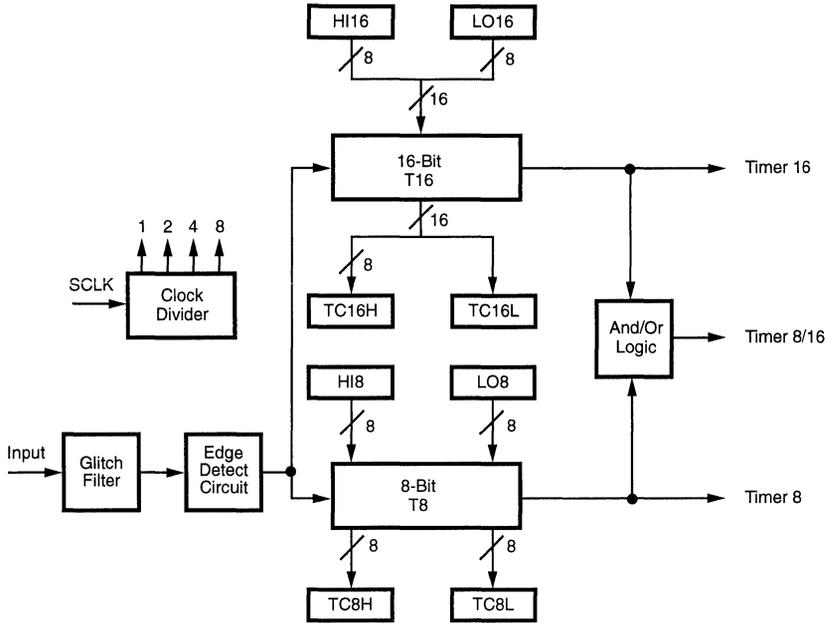
Figure 1. Counter/Timer Block Diagram
