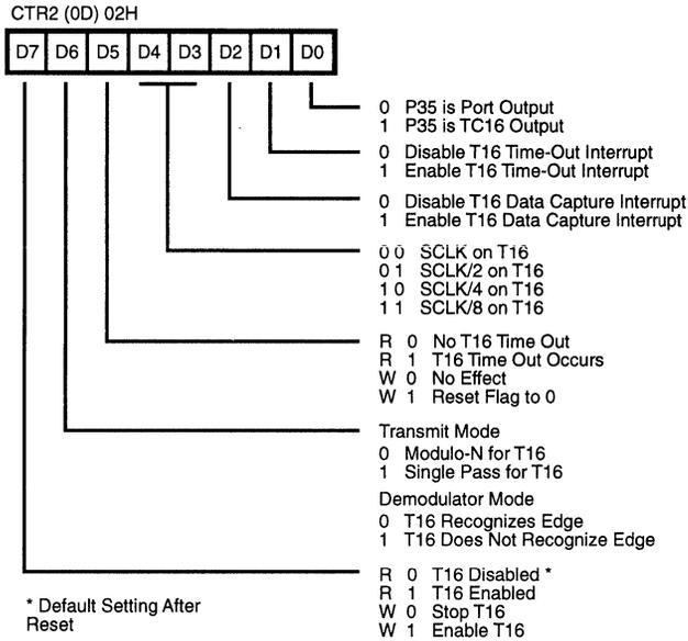
**Figure 49. T16 Control Register**
