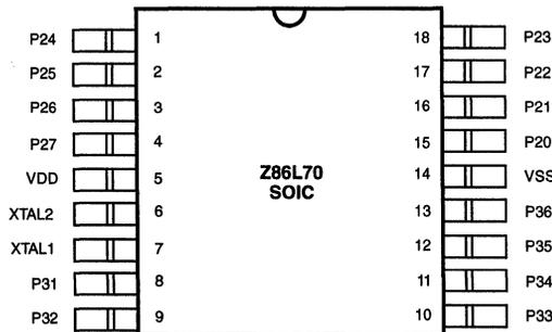
**Figure 6. 18-Pin SOIC Pin Assignments**
