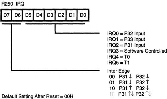
Figure 33. Interrupt Request Register (FAH: Read/Write)
