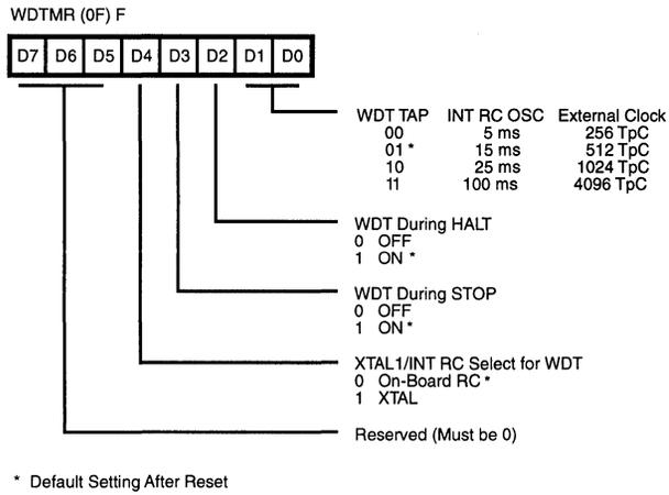
**Figure 52. Watch-Dog Timer Mode Register ((F) 0FH: Write Only)**
