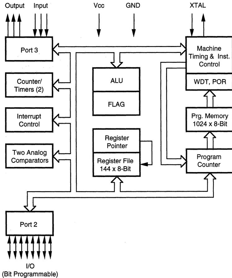
**Figure 1. Z86L06 Functional Block Diagram**
