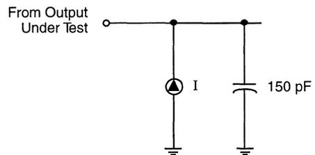
**Figure 19. Test Load Configuration**
