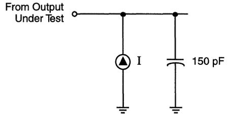
Figure 42. Test Load Diagram
