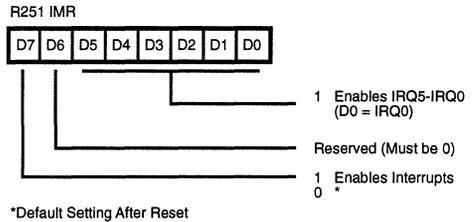
Figure 34. Interrupt Mask Register (FBH: Read/Write)
