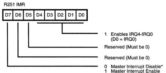
**Figure 58. Interrupt Mask Register ((0)FBH:Read/Write)**
