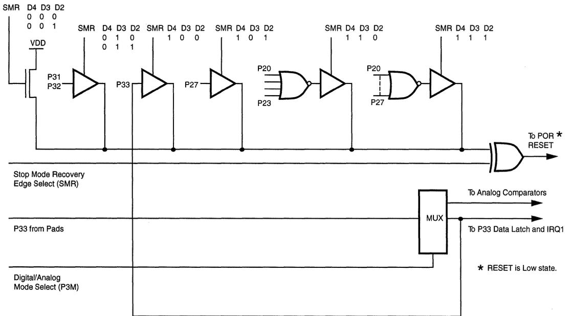
**Figure 15. Stop-Mode Recovery Source**
