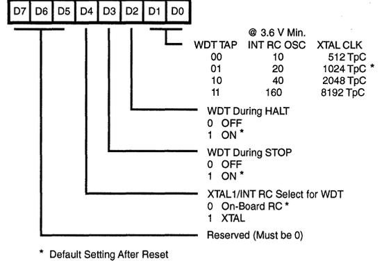
Figure 22. Watch-Dog Timer Mode Register ((F) 0FH: Write Only)
