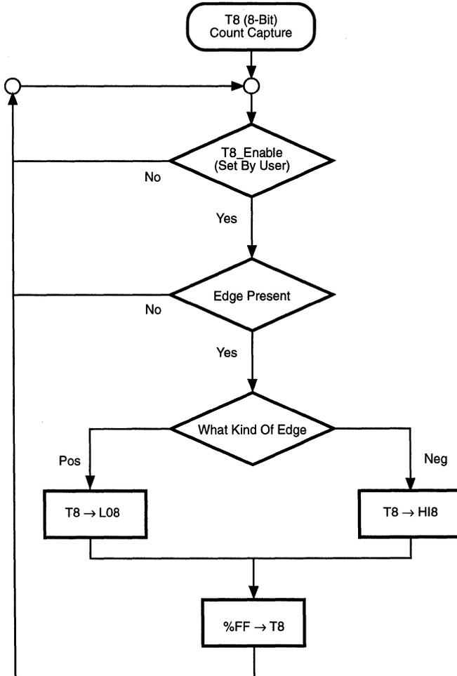
**Figure 24. Demodulation Mode Count Capture Flowchart**
