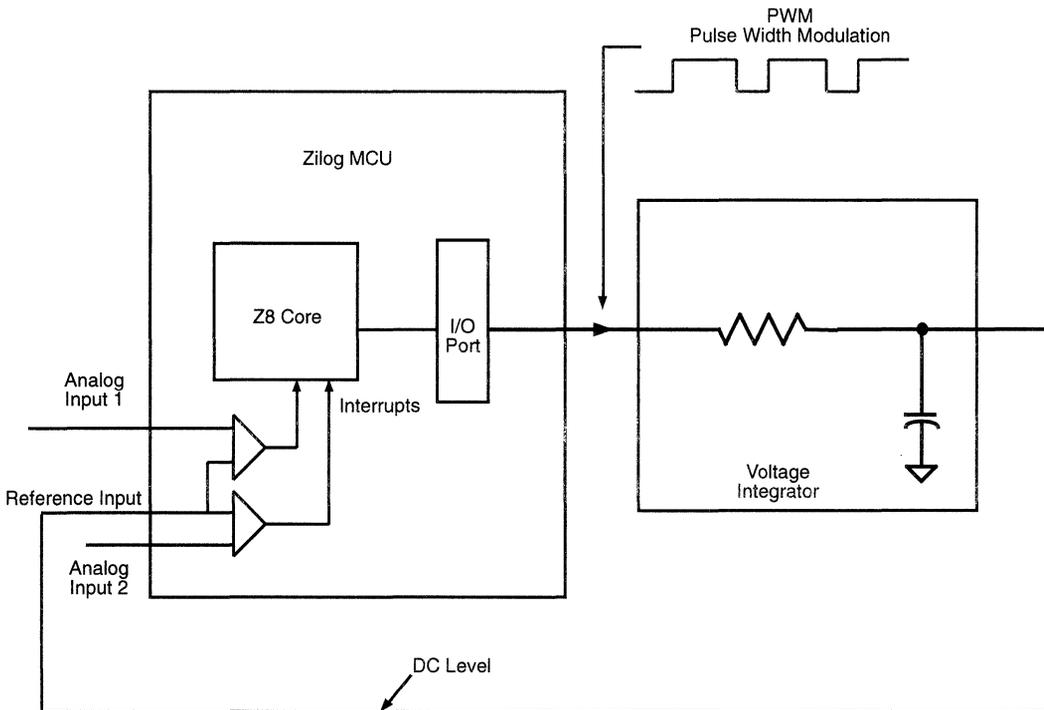
Figure 6. On-Board Comparators
