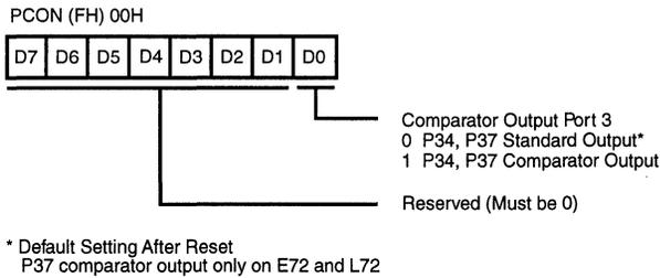
**Figure 53. Port Configuration Register (PCON) ((0F) 0H: Write Only)**
