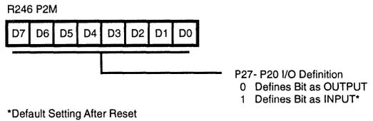
Figure 29. Port 2 Mode Register (F6H: Write Only)
