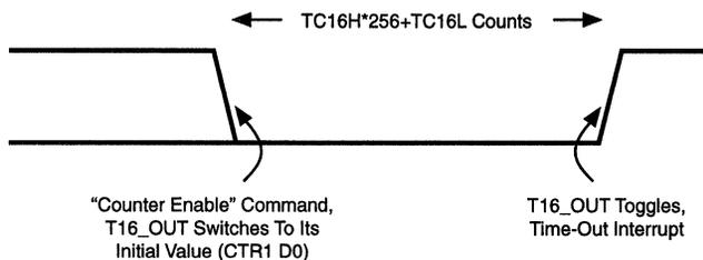
**Figure 28. T16\_OUT in Single-Pass Mode**
