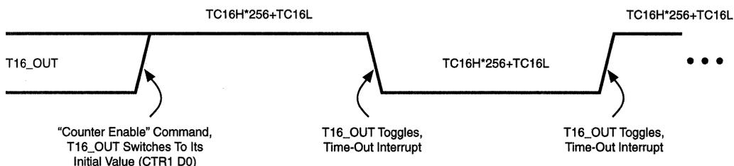
**Figure 29. T16\_OUT in Modulo-N Mode**
