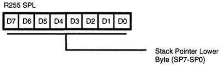
**Figure 38. Stack Pointer**
