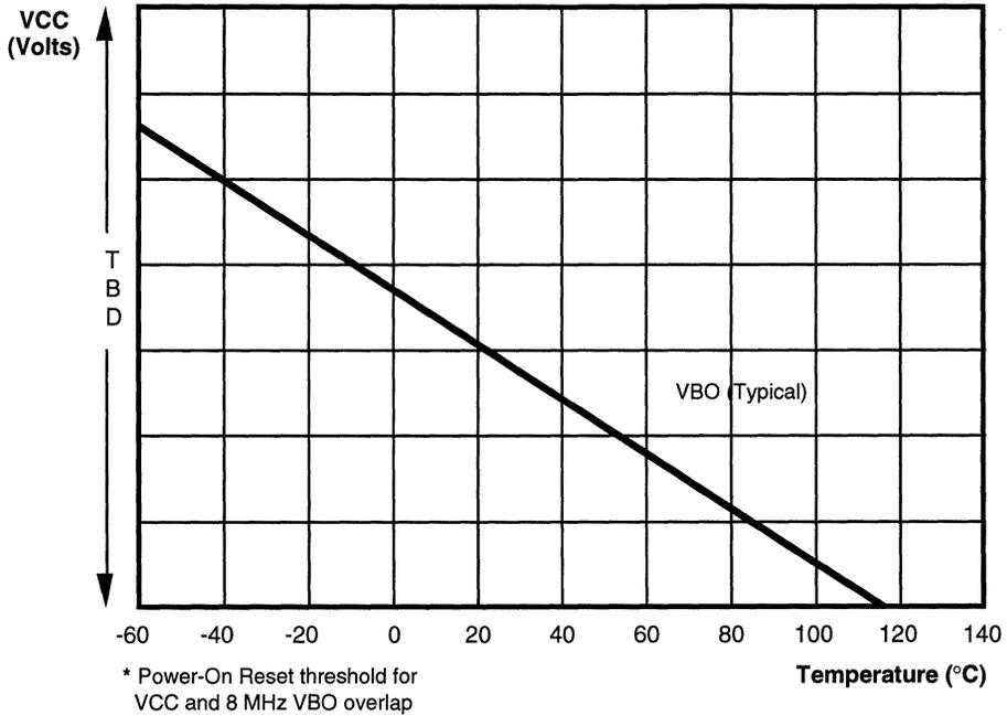
Figure 18. Typical Z86L29  $V_{BO}$  Voltage vs Temperature
