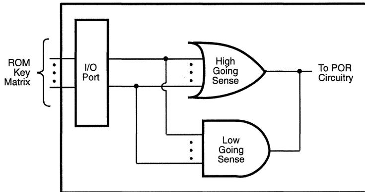
Any high-going or low-going change on the I/O port triggers the on-board POR circuitry.
