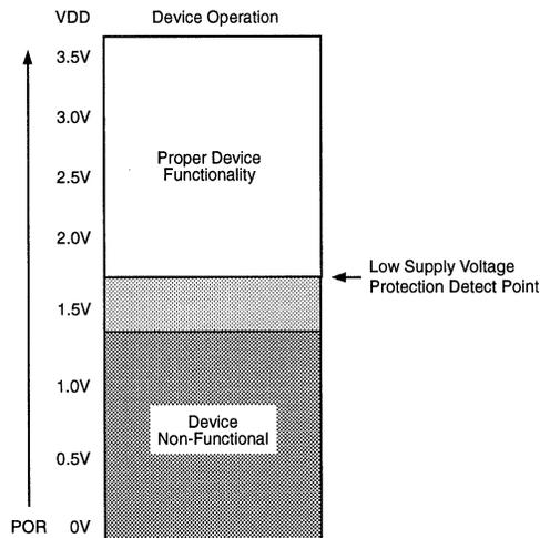
Figure 3. MCU Device Operation vs Supply Voltage
