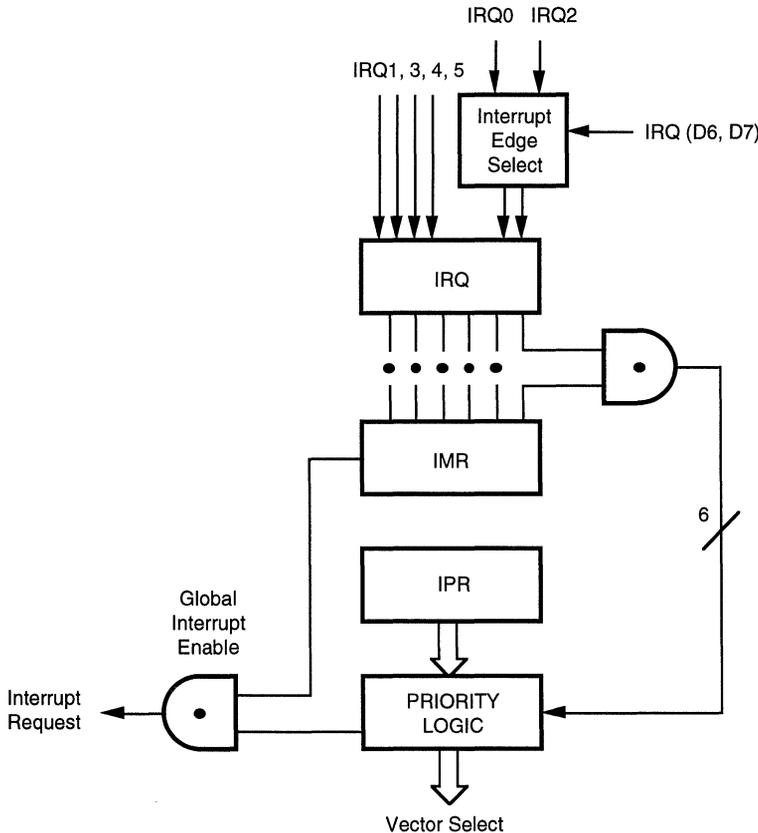
**Figure 12. Interrupt Block Diagram**
