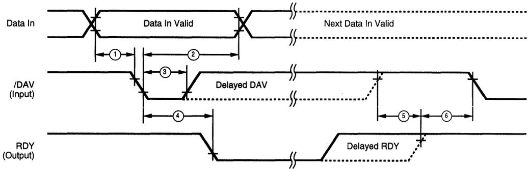
**Figure 45. Input Handshake Timing**
