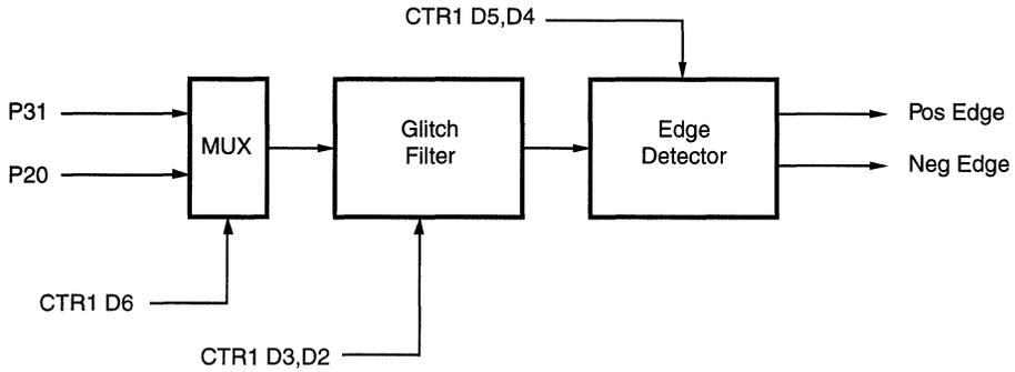
**Figure 20. Glitch Filter Circuitry**
