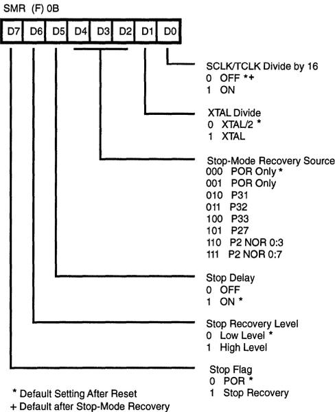
Figure 20. Stop-Mode Recovery Register (Write Only, except bit 7)
