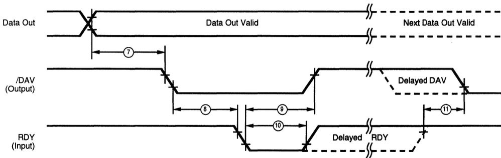
**Figure 46. Output Handshake Timing**
