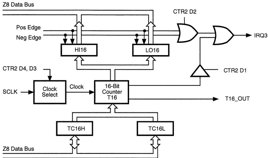
Figure 27. 16-bit Counter/Timer Circuits
