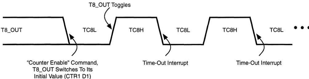
Figure 23. T8\_OUT in Modulo-N Mode
