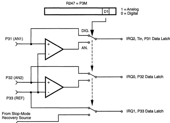
Figure 4. Port 3 Comparator Configuration
