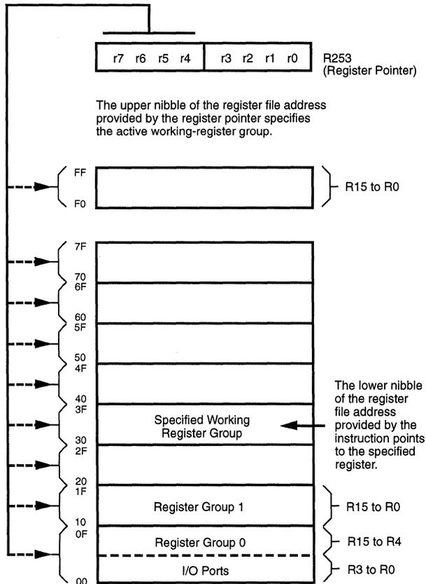
Figure 10. Register Pointer
