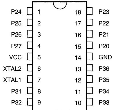
**Figure 2. 18-Pin DIP and SOIC Configuration**
