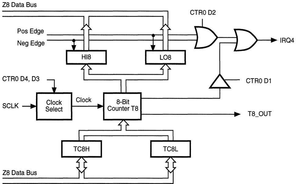
**Figure 21. 8-bit Counter/Timer Circuits**
