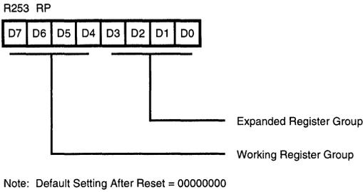
**Figure 8. Register Pointer Register**
