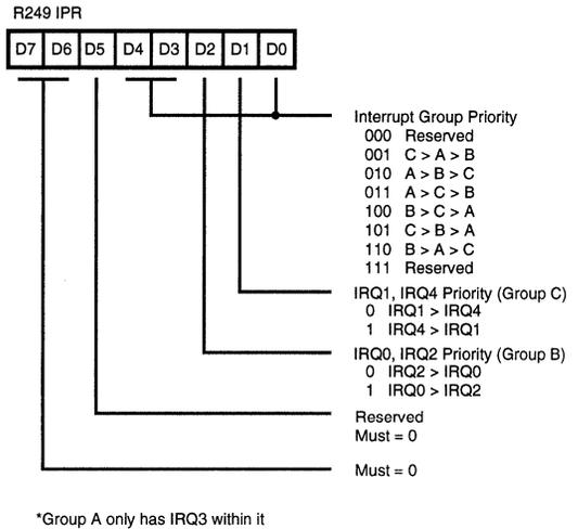
**Figure 56. Interrupt Priority Registers ((0)F9H:Write Only)**
