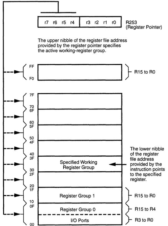
**Figure 9. Register Pointer**
