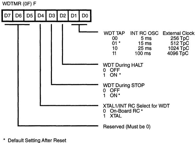
**Figure 39. Watch-Dog Timer Mode Register (Write Only)**
