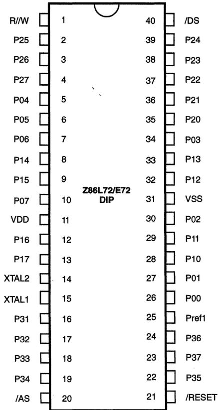
**Figure 3. 40-Pin DIP Pin Assignments**
