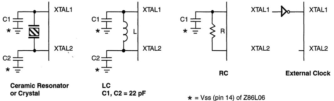
Figure 13. Oscillator Configuration
