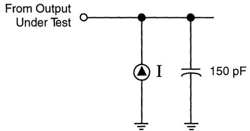
**Figure 18. Test Load Configuration**
