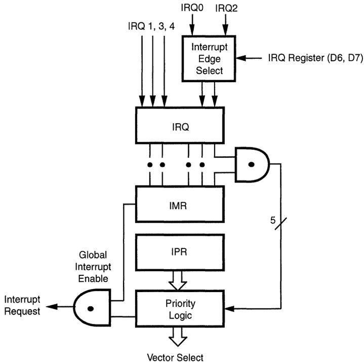
Figure 33. Interrupt Block Diagram
