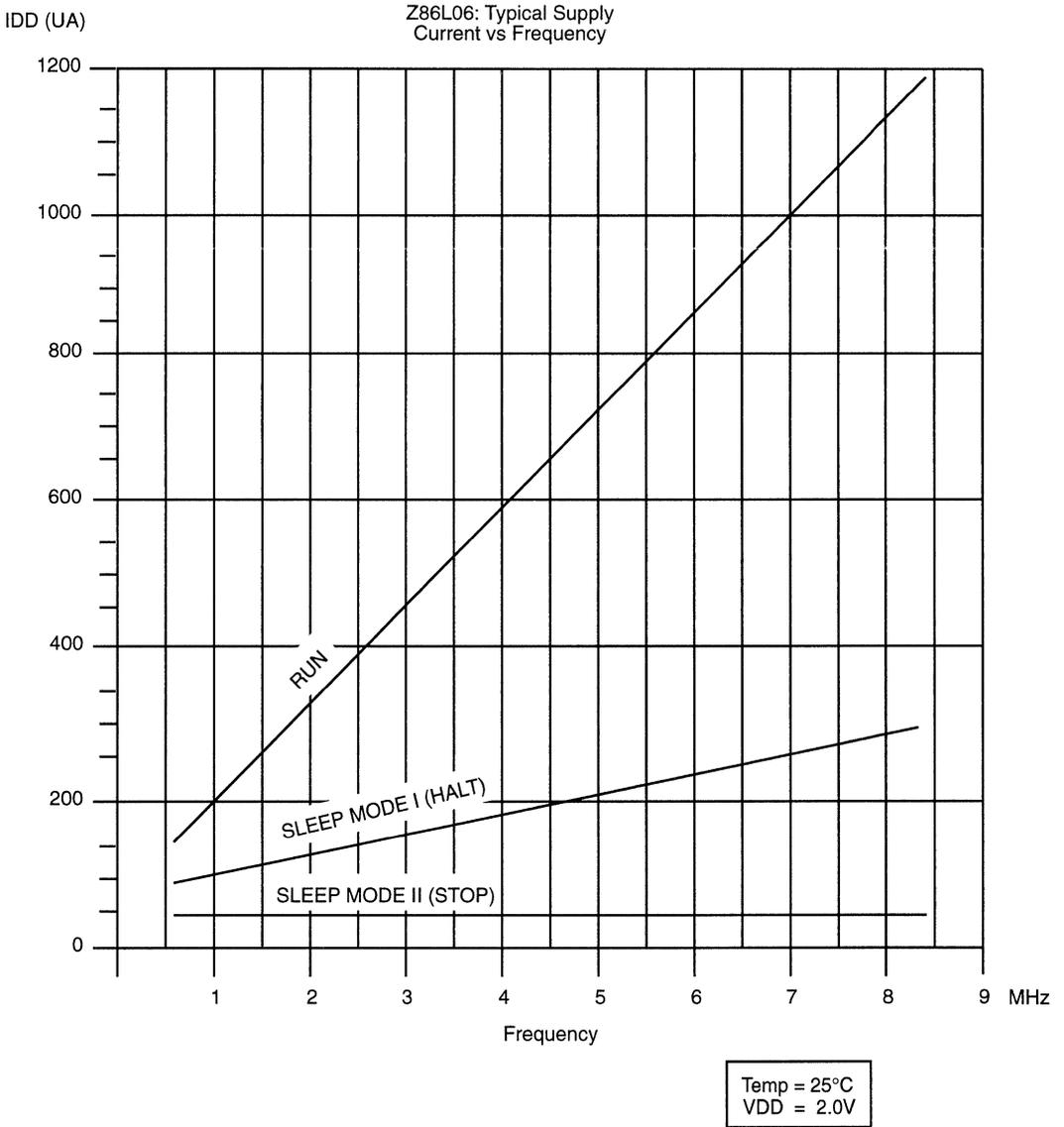
Figure 2. Typical Supply Current vs Frequency
