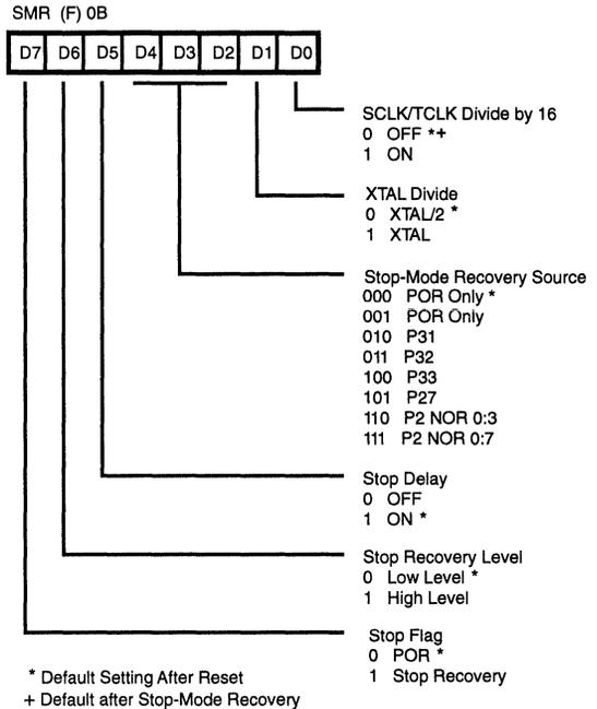
**Figure 14. Stop-Mode Recovery Register (Write Only, except bit 7)**
