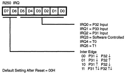
Figure 33. Interrupt Request Register (FAH: Read/Write)
