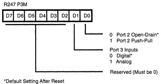
Figure 30. Port 3 Mode Register (F7H: Write Only)
