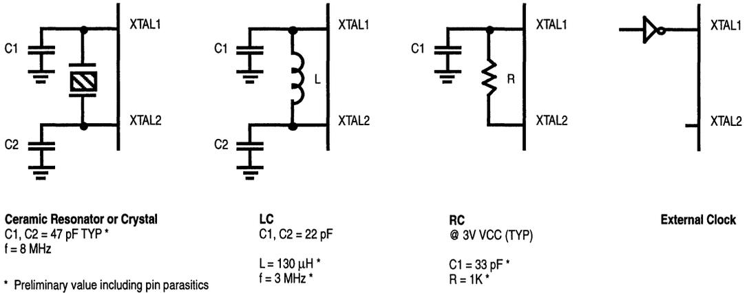
**Figure 34. Oscillator Configuration**
