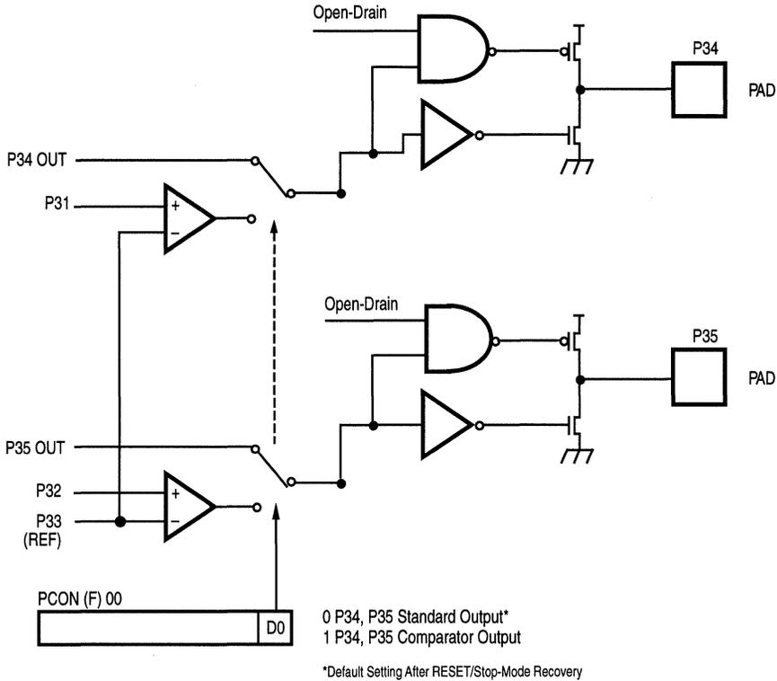
Figure 5. Port 3 I/O Configuration
