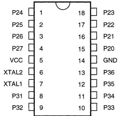
Figure 2. DIP and SOIC Pin Configuration
