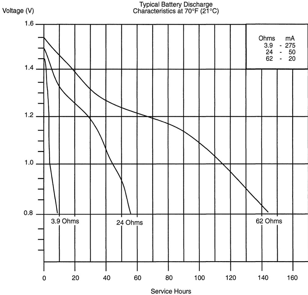
Figure 1. Typical Battery Discharge
