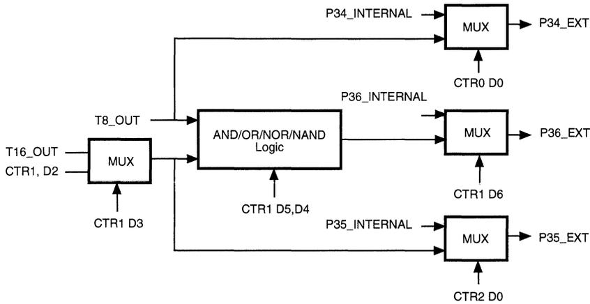
Figure 32. Output Circuit
