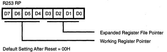
Figure 36. Register Pointer (FDH: Read/Write)
