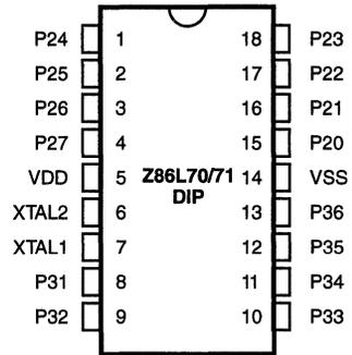
**Figure 4. 18-Pin DIP Pin Assignments**
