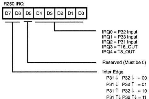
**Figure 57. Interrupt Request Register ((0)FAH:Read/Write)**
