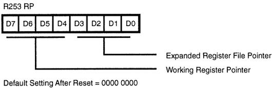
**Figure 60. Register Pointer**
