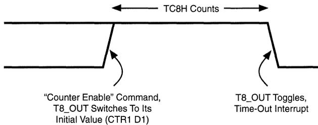
Figure 22. T8\_OUT in Single-Pass Mode
