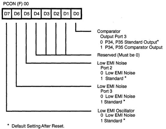
Figure 22. Port Control Register (Write Only)
