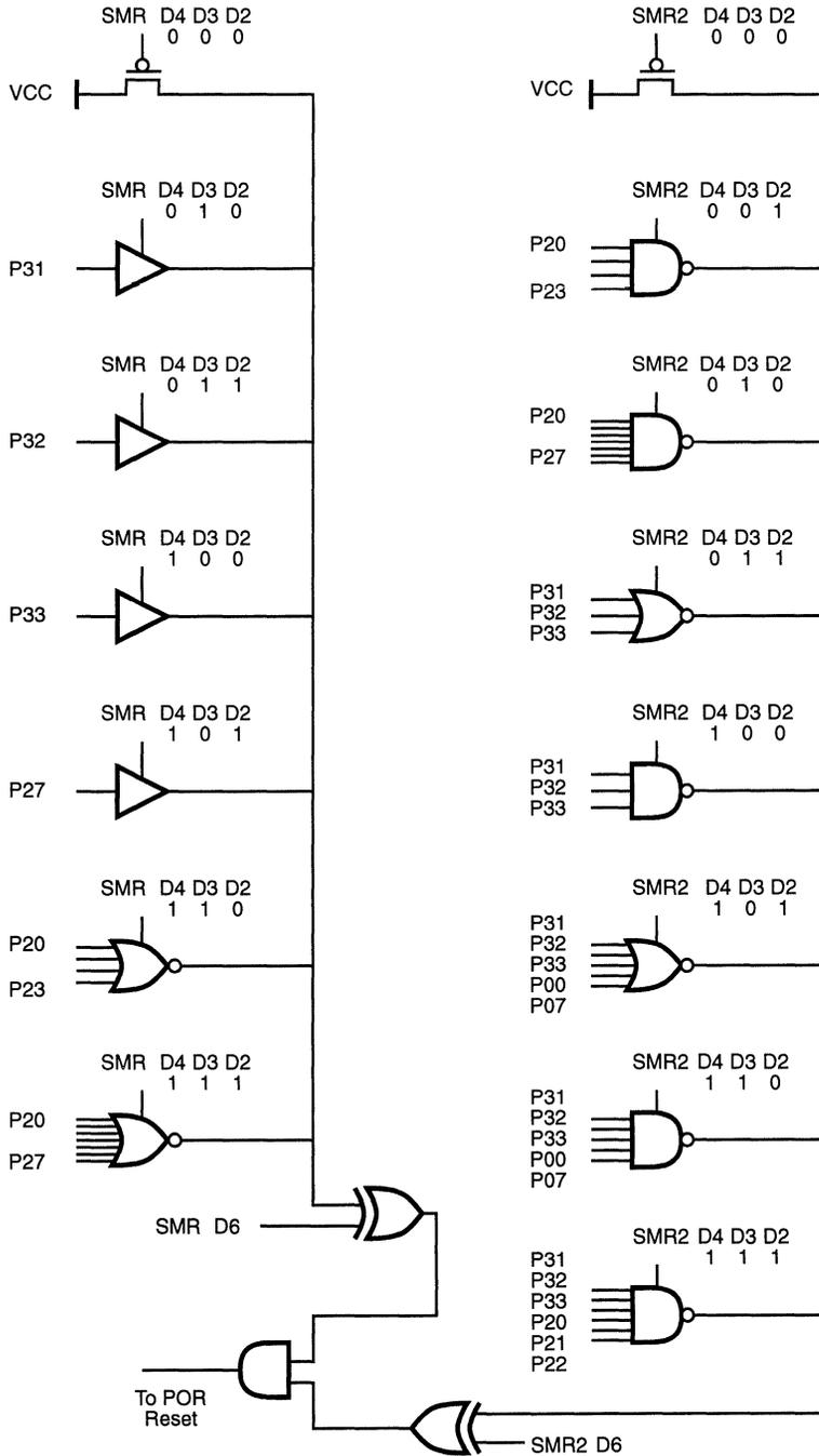
Figure 38. Stop-Mode Recovery Source
