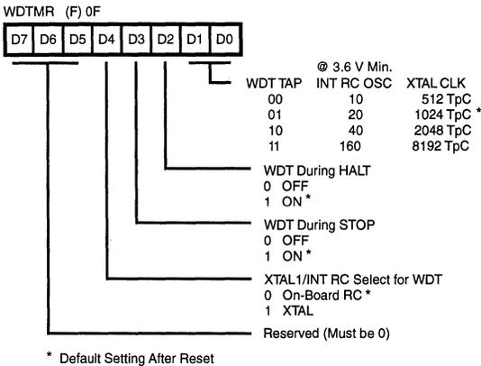
Figure 21. Watch-Dog Timer Mode Register (Write Only)
