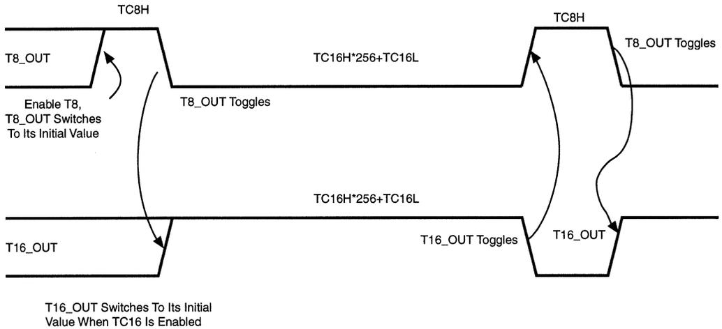
**Figure 31. T8\_OUT and T16\_OUT in Ping-Pong Mode**
