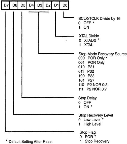
Figure 21. Stop-Mode Recovery Register ((F) 0BH: Read Only)
