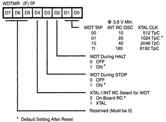
Figure 16. Watch-Dog Timer Mode Register (Write Only)
