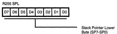
Figure 38. Stack Pointer (FFH: Read/Write)
