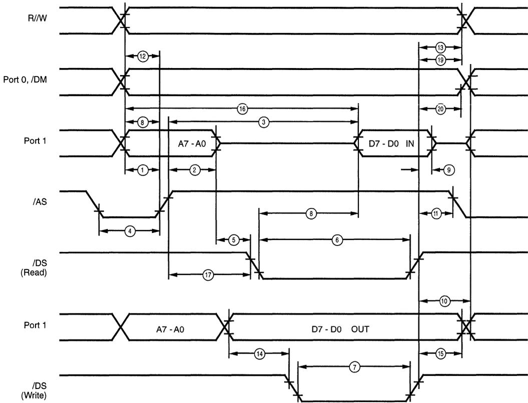
**Figure 43. External I/O or Memory Read/Write Timing**
