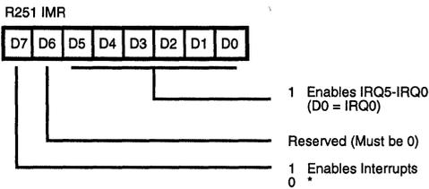
Figure 34. Interrupt Mask Register (FBH: Read/Write)
