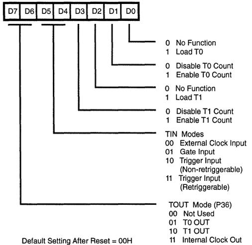
Figure 24. Timer Mode Register (F1H: Read/Write)
