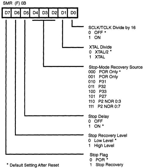
**Figure 13. Stop-Mode Recovery Register**
