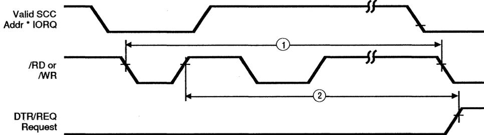
Figure 76. SCC External BUS Master Timing
