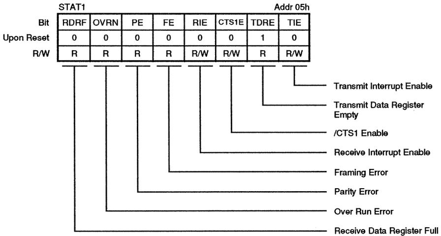
Figure 12. ASCII Status Register (Ch. 1)
