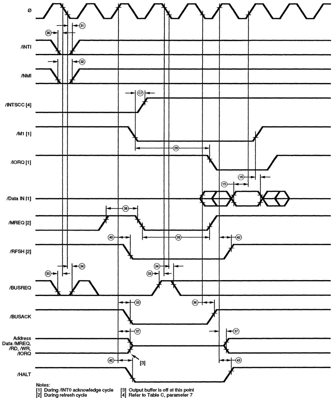
**Figure 61. CPU Timing**
