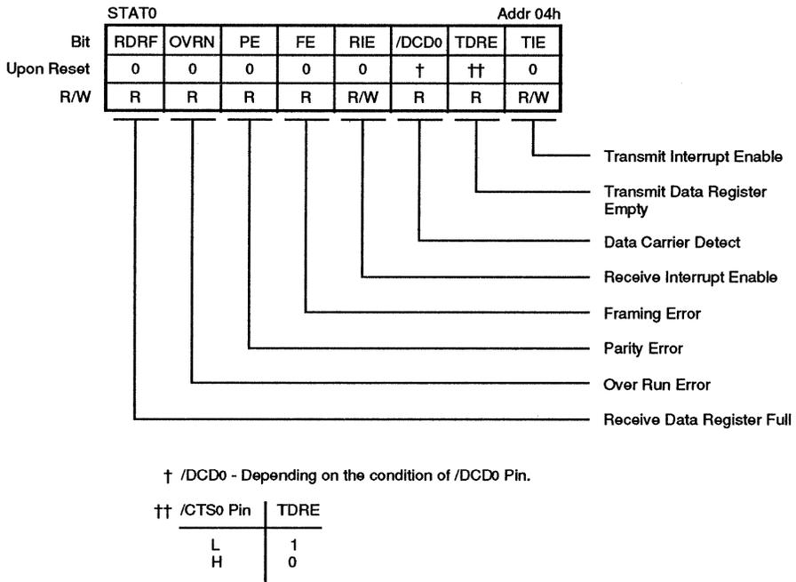
Figure 11. ASCII Status Register
