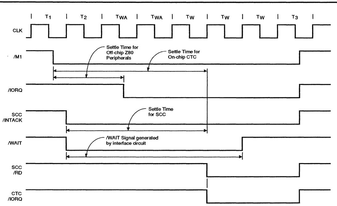
Figure 78. Interrupt Acknowledge Cycle Timing
