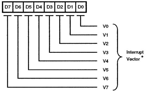
\* Modified if VIS bit in Write register 9 is set.
