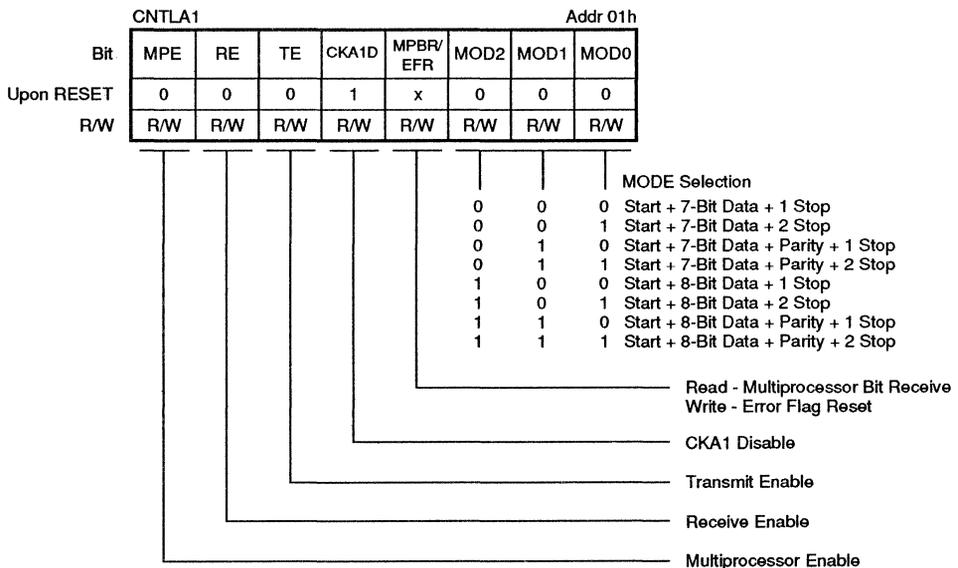
Figure 8. ASCII Control Register A (Ch. 1)
