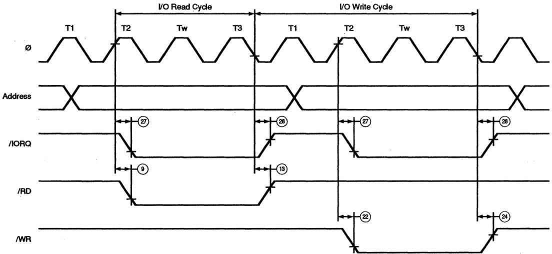
**Figure 62. CPU Timing** ( $\text{I/O} = 0$ )
