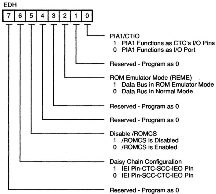
Figure 58. System Configuration Register
