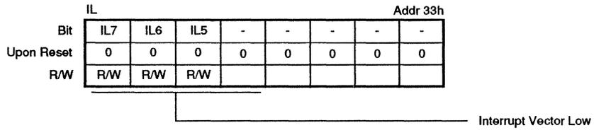
Figure 41. Interrupt Vector Low Register
