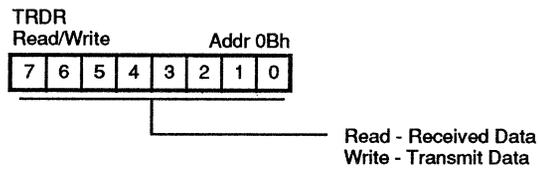
Figure 18. CSI/O Transmit/Receive Data Register
