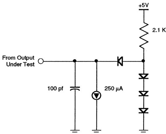
Figure 59. Standard Test Circuit
