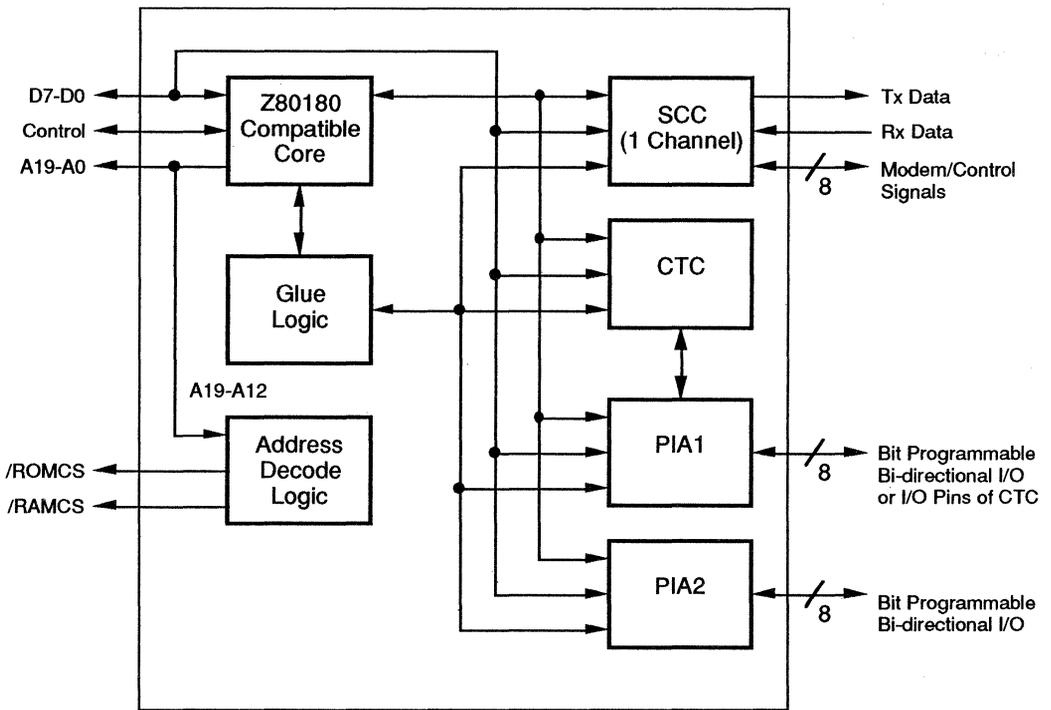
$$\text{Z80181} = \text{Z180} + \text{SCC} + \text{CTC} + \text{PIA}$$
