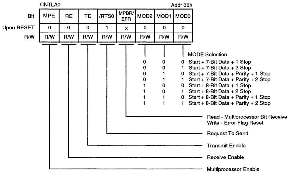
Figure 7. ASCII Control Register A (Ch. 0)
