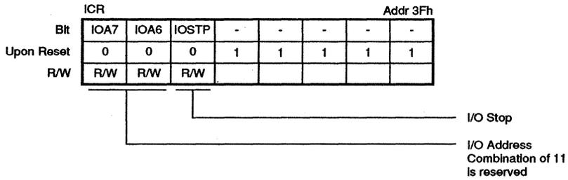
**Figure 45. I/O Control Register**
