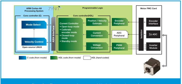
Figure 2 — The motor control system model includes two primary subsystems.
