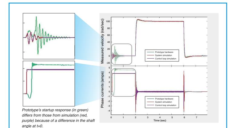
Figure 4(b) — Comparison of results from hardware prototype and simulation
