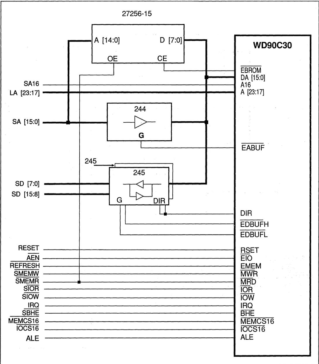
FIGURE 15. 16-BIT PC AT INTERFACE WITH 8-BIT BIOS
