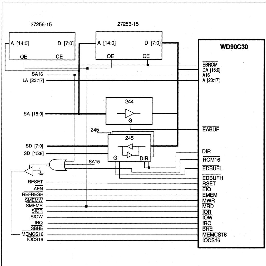
**FIGURE 16. 16-BIT PC AT INTERFACE WITH 16-BIT BIOS**
