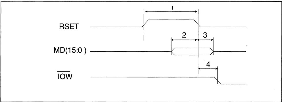
FIGURE 5. RESET TIMING
