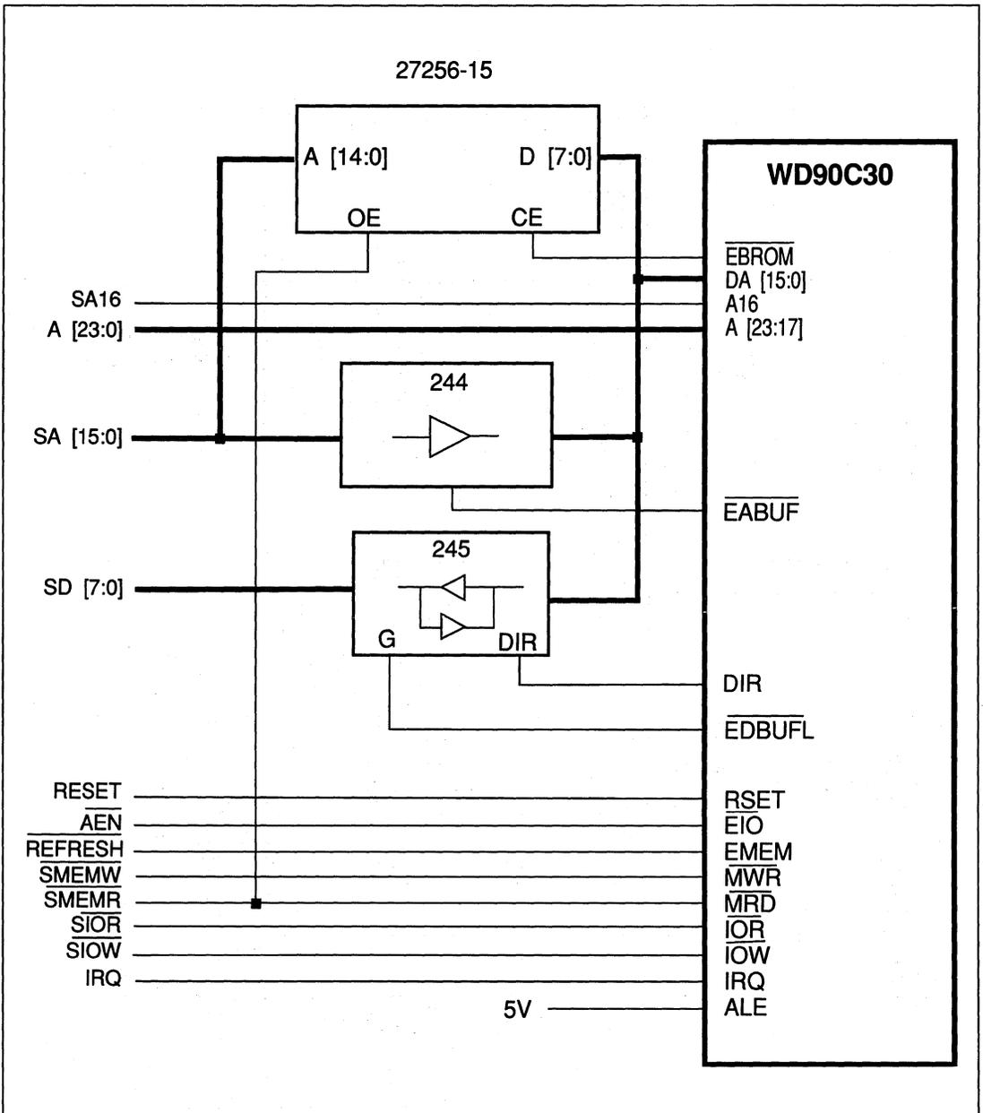
**FIGURE 14. 8-BIT PC AT INTERFACE WITH 8-BIT BIOS**
