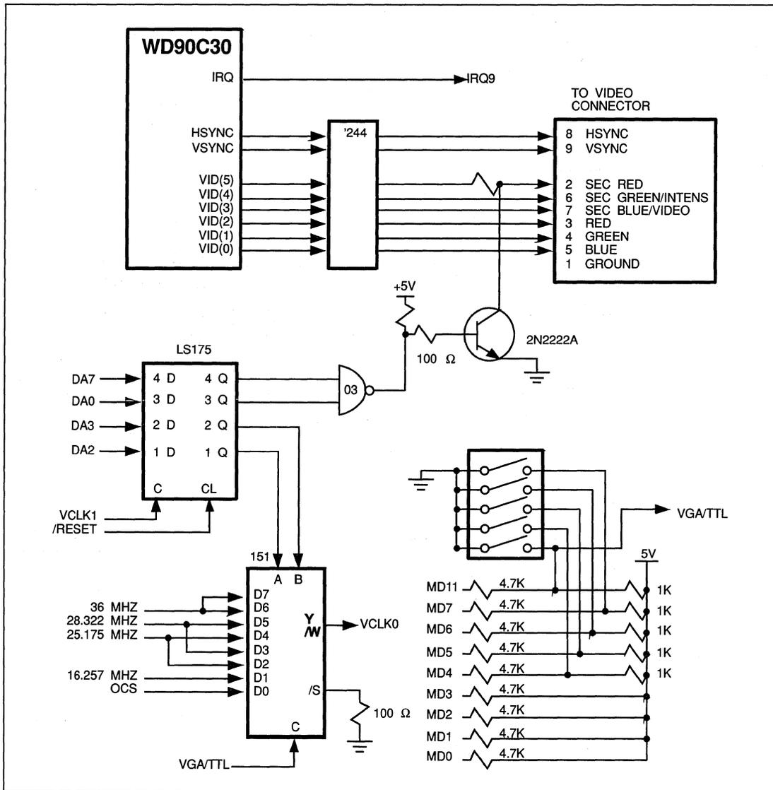
**FIGURE 22. WD90C30 AND TTL MONITOR CONNECTIONS**
