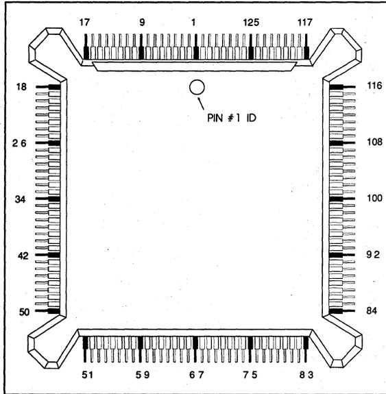
FIGURE 3. 132-PIN JEDEC PACKAGE
