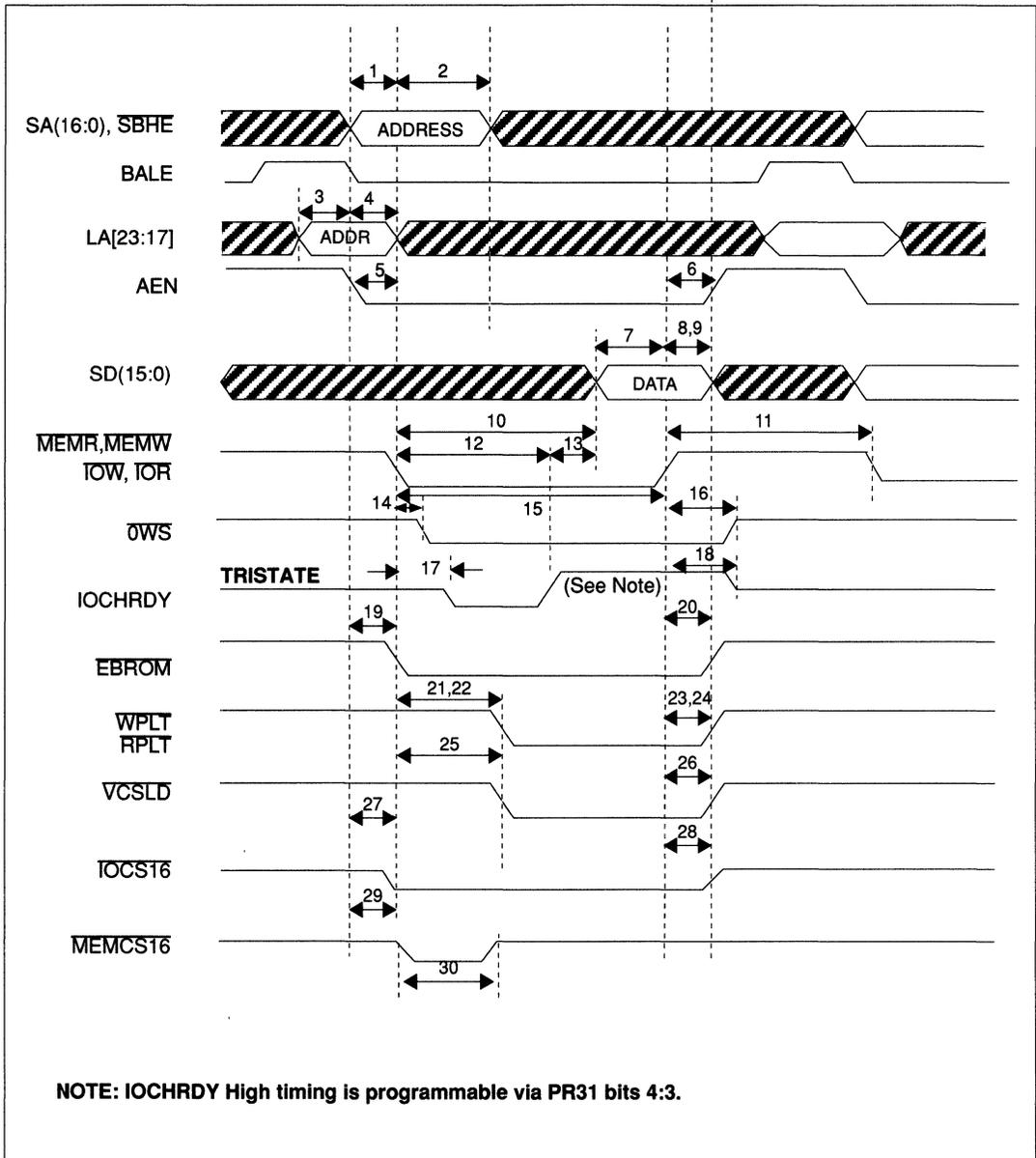
FIGURE 11-3 I/O AND MEMORY READ/WRITE ISA (AT) MODE TIMING
