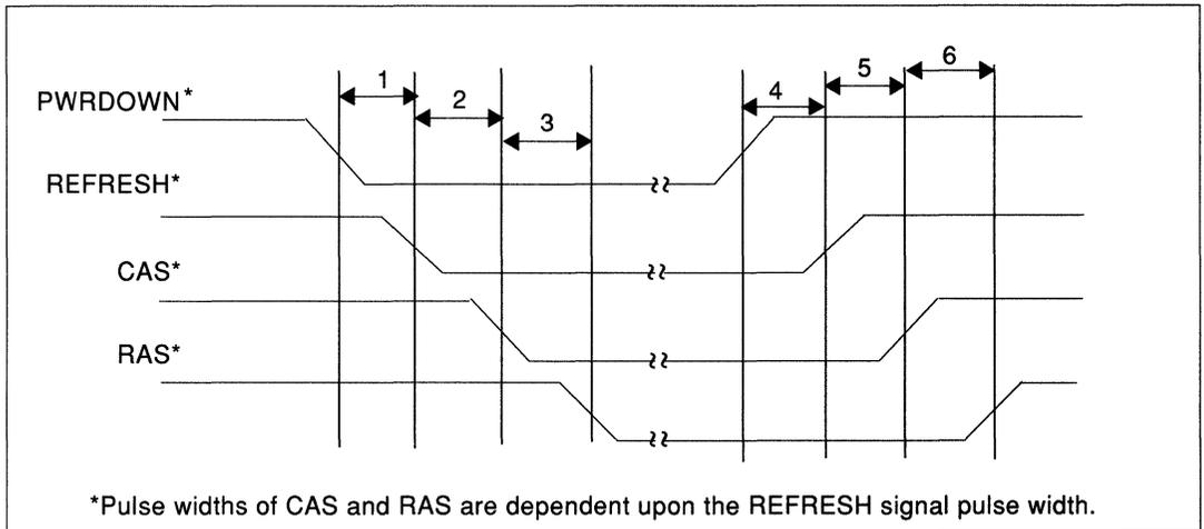
FIGURE 11-13 SELF-REFRESH TIMING, SLEEP/DISPLAY IDLE MODES
