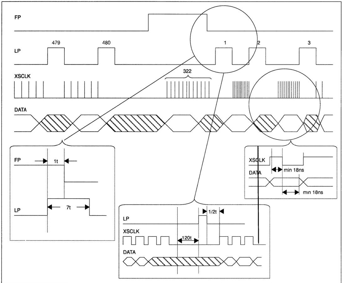
FIGURE 11-7 STN COLOR LCD INTERFACE FUNCTIONAL TIMING
