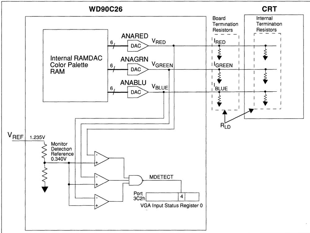
**FIGURE 6-28 MONITOR DETECTION CIRCUIT FOR INTERNAL RAMDAC**
