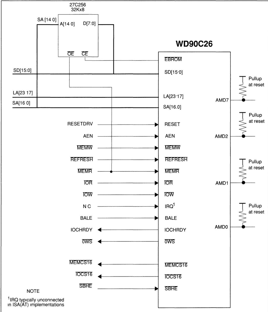
FIGURE 6-6 16-BIT ISA BUS (AT) INTERFACE
