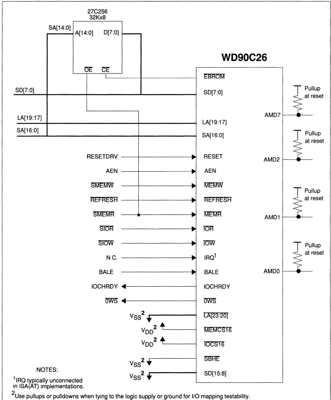
**FIGURE 6-5 8-BIT ISA BUS (AT) INTERFACE**
