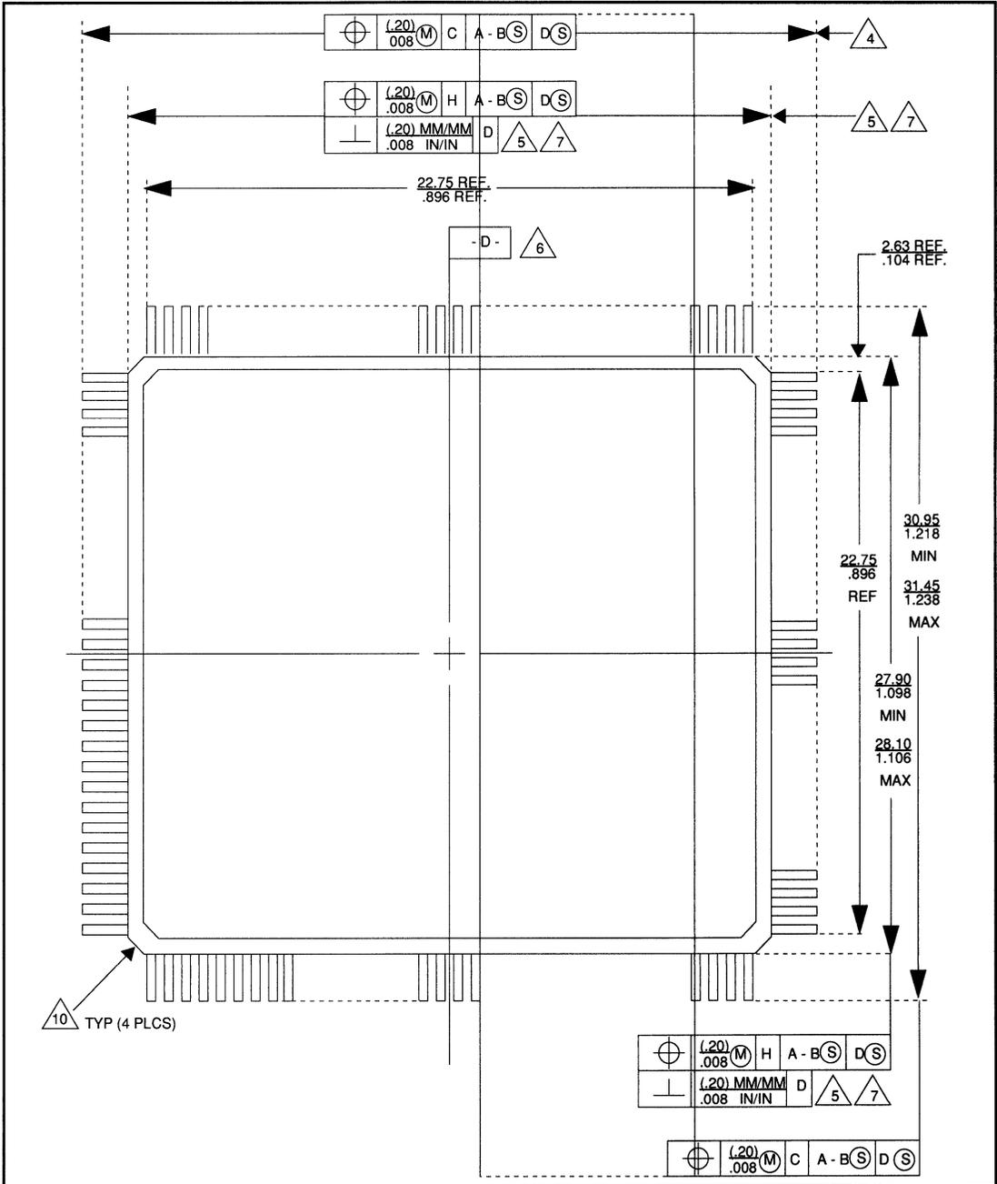
FIGURE 12-1 WD90C26 144-PIN MQFP PACKAGE MECHANICAL DRAWING
