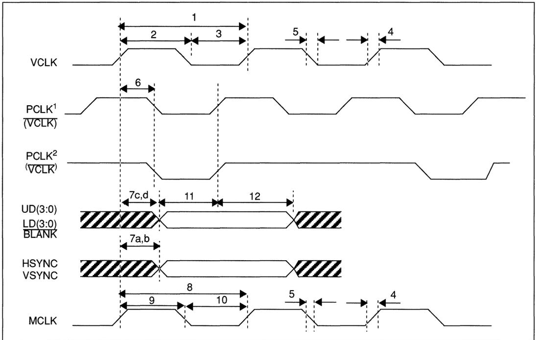
FIGURE 11-1 CLOCK AND EXTERNAL RAMDAC TIMING
