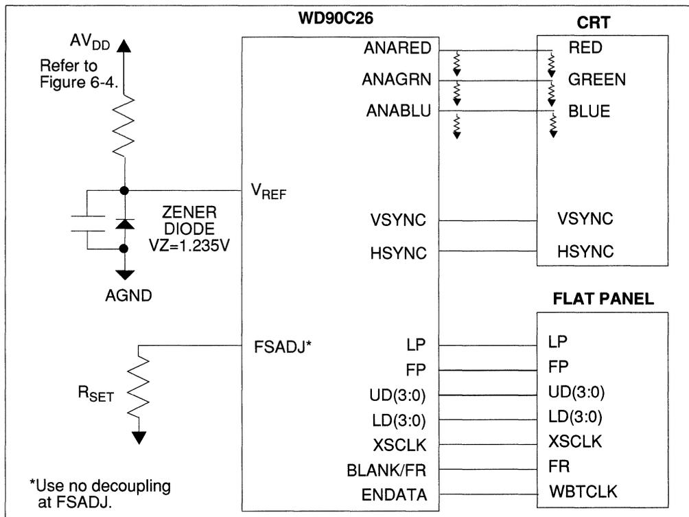
FIGURE 6-27 EXAMPLE OF CRT INTERFACE SHOWING V<sub>REF</sub> AND FSADJ CIRCUITS
