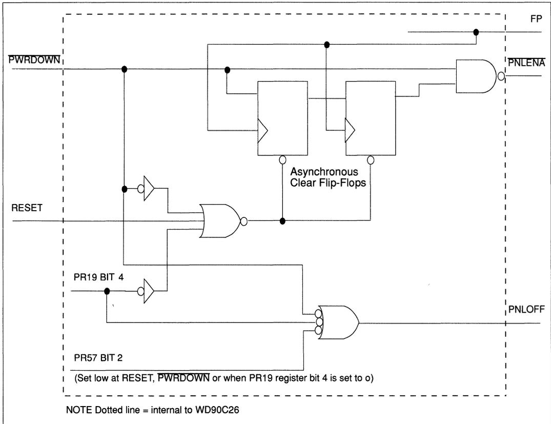
**FIGURE 6-12 PNL $\overline{EN}$ A AND PNLOFF PANEL PROTECTION SIGNALS**
