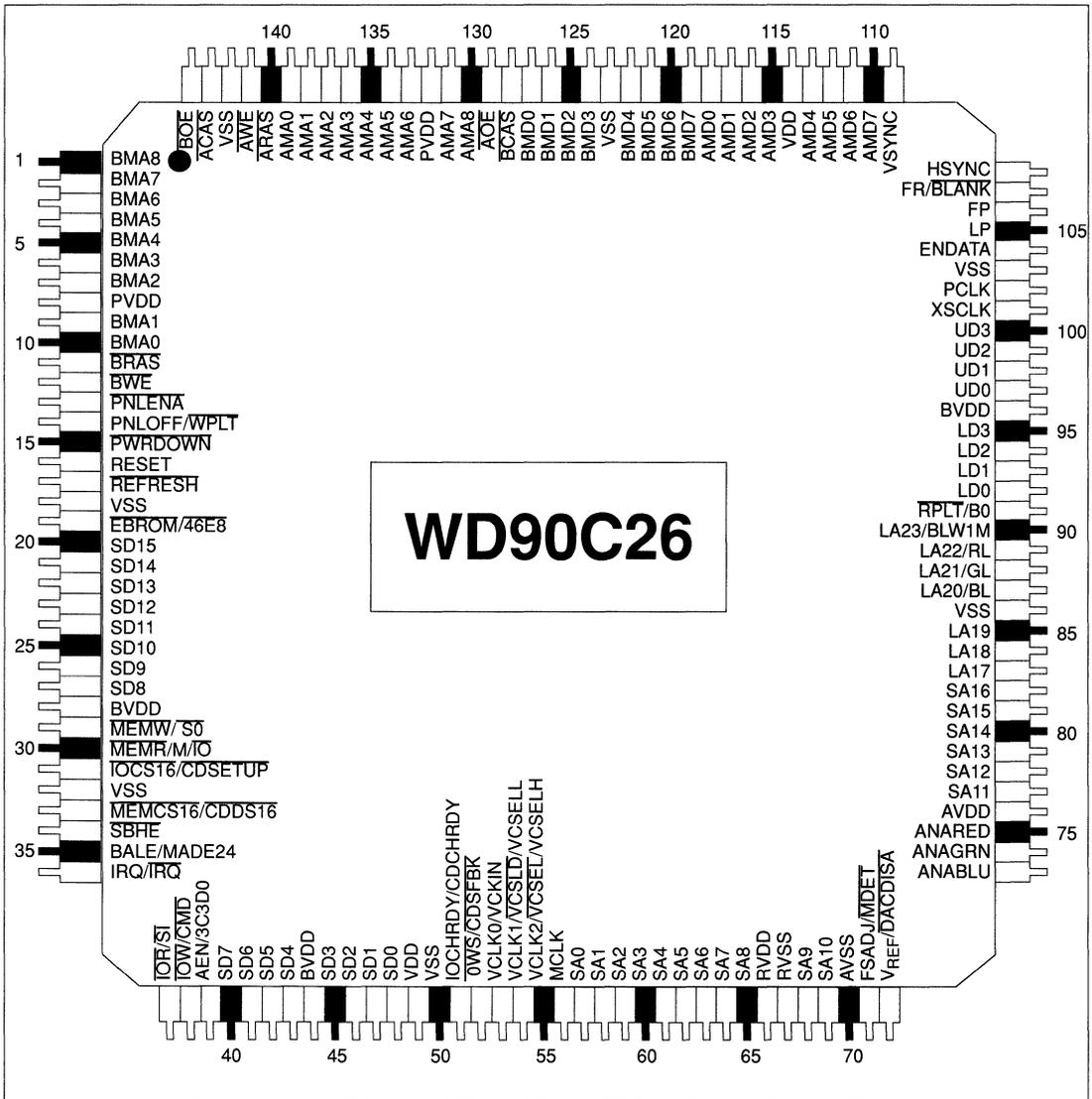
FIGURE 4-1 WD90C26 PIN DIAGRAM, 144 PIN JEDEC MQFP PACKAGE
