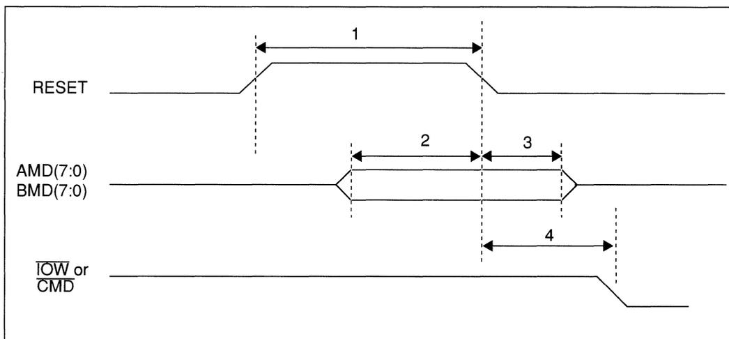
FIGURE 11-2 RESET TIMING
