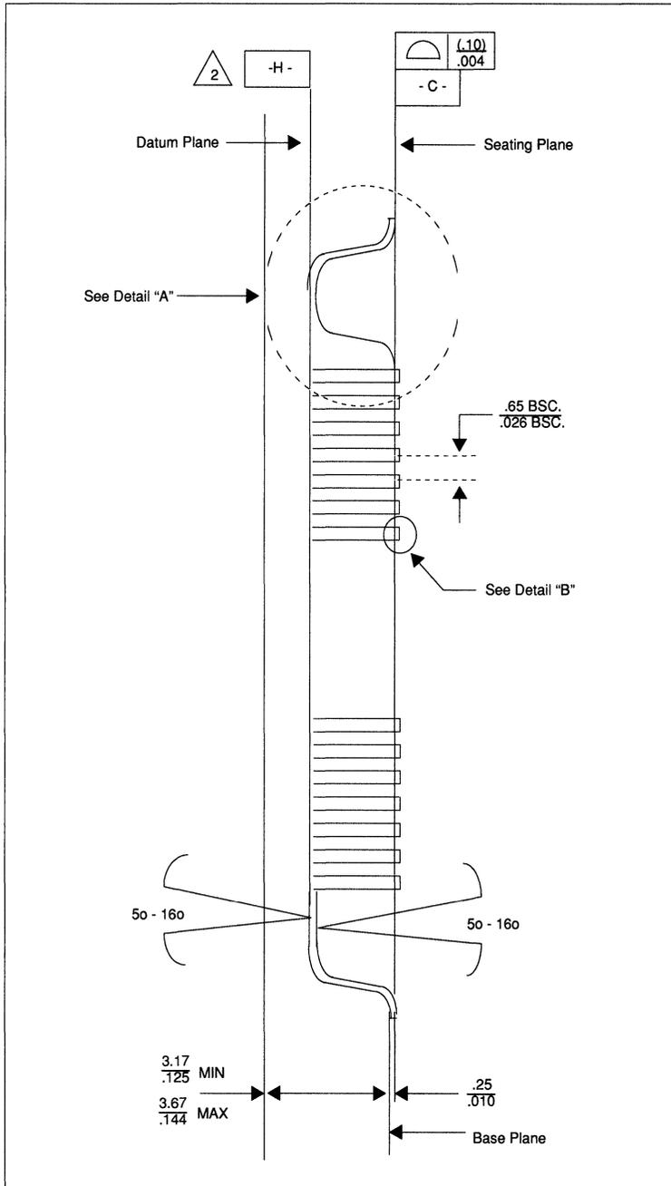
FIGURE 12-1 WD90C26 144-PIN MQFP PACKAGE MECHANICAL DRAWING
