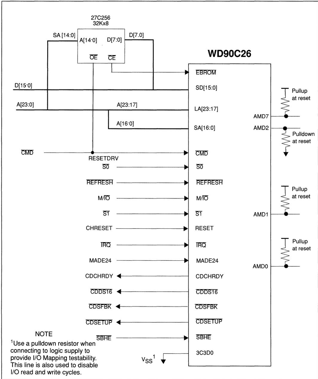
**FIGURE 6-7 16-BIT MICROCHANNEL BUS INTERFACE**
