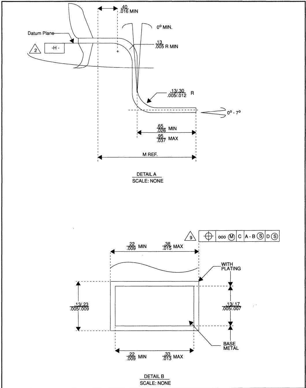
FIGURE 12-1 WD90C26 144-PIN MQFP PACKAGE MECHANICAL DRAWING
