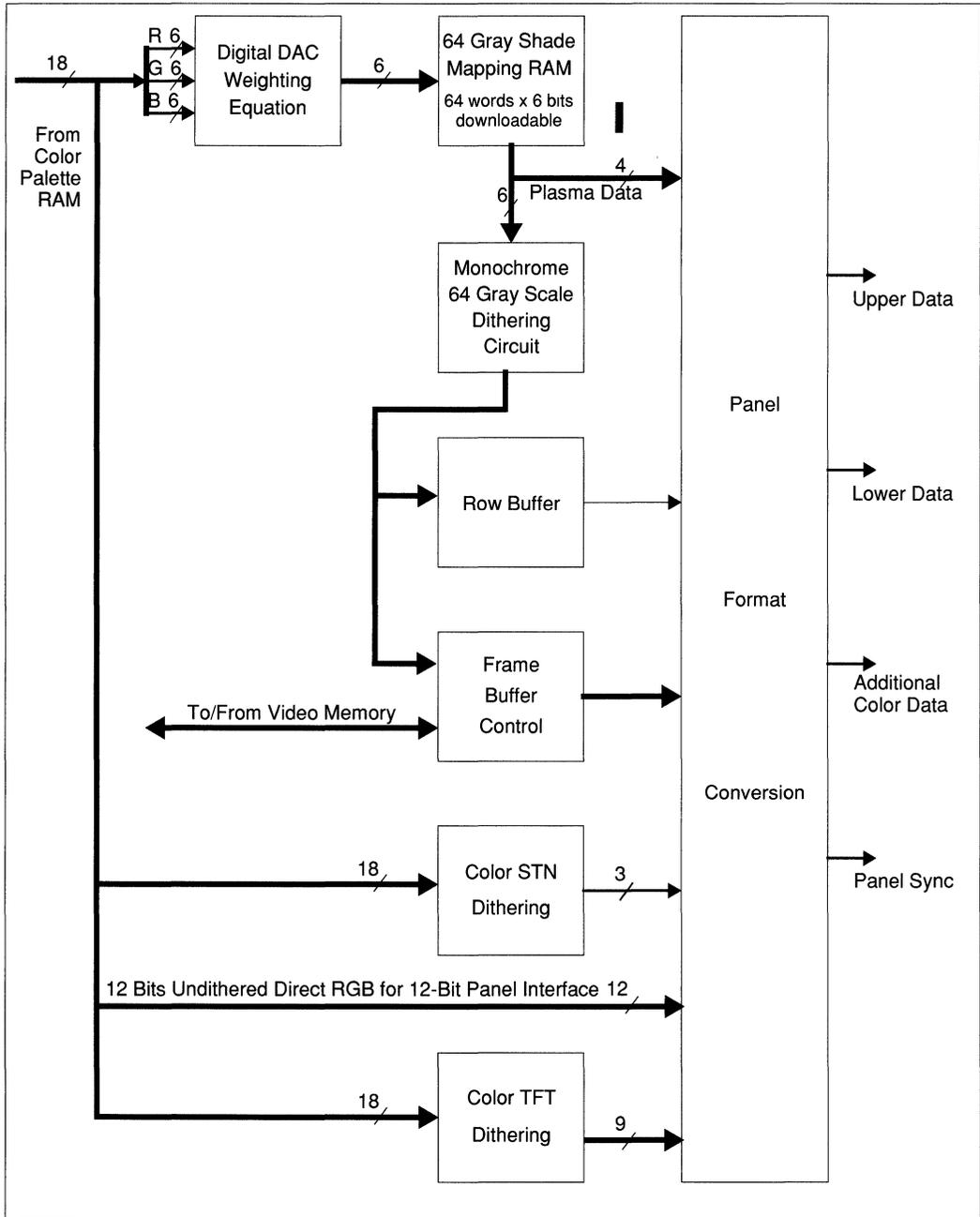
FIGURE 2-2 FLAT PANEL ADAPTER SECTION BLOCK DIAGRAM
