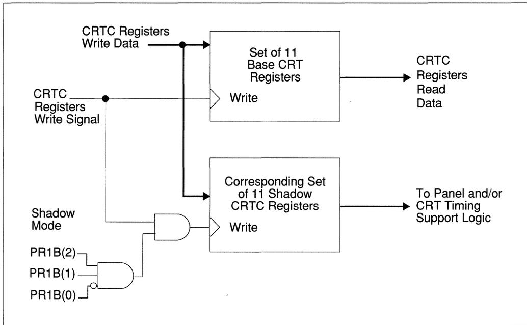
**FIGURE 6-13 RELATIONSHIP BETWEEN SHADOW AND BASE CRTC REGISTERS**
