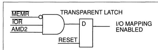
**FIGURE 6-30 ENABLING I/O MAPPING ON THE WD90C26**
