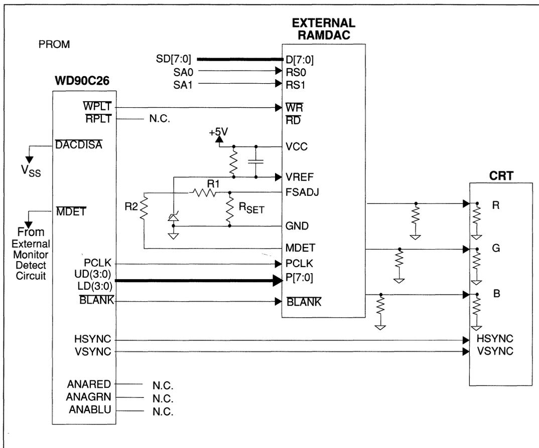
FIGURE 6-29 WD90C26 WITH EXTERNAL RAMDAC INTERFACE
