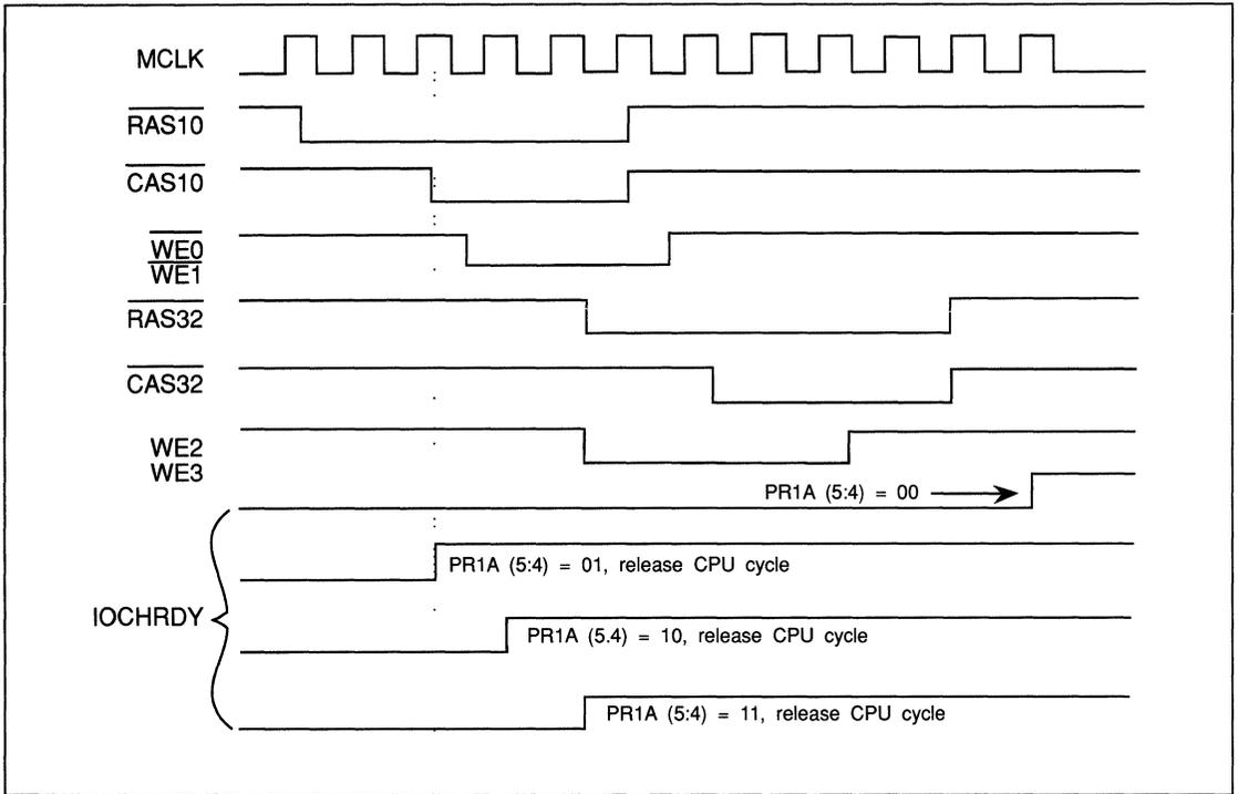
FIGURE C-21. IOCHRDY RELEASE TIMING IN MEMORY WRITE CYCLE
