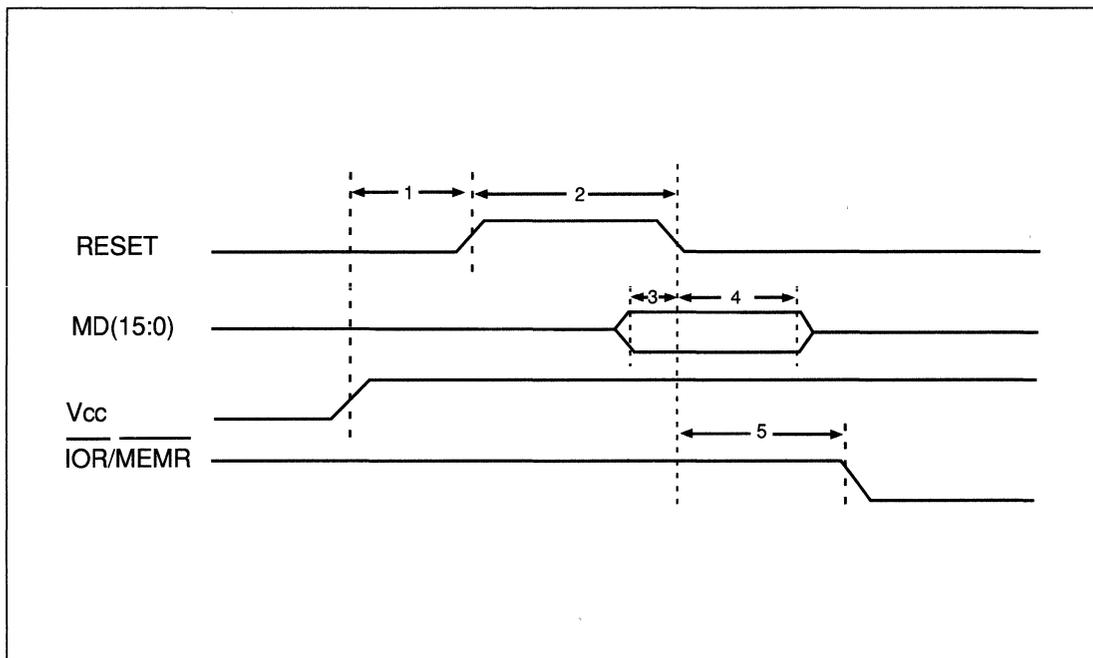
FIGURE C-15. RESET TIMING
