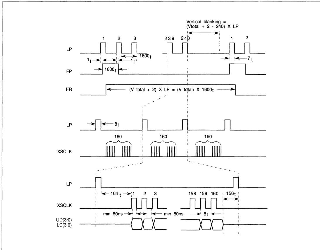
FIGURE C-12. WD90C22 LCD TIMING DIAGRAM ( $t=VCLK$ )
