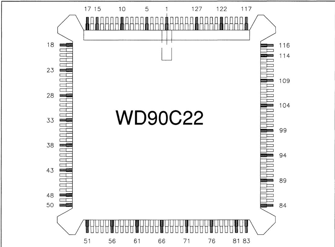
FIGURE 4-1. 132-PIN PQFP PIN ASSIGNMENTS
