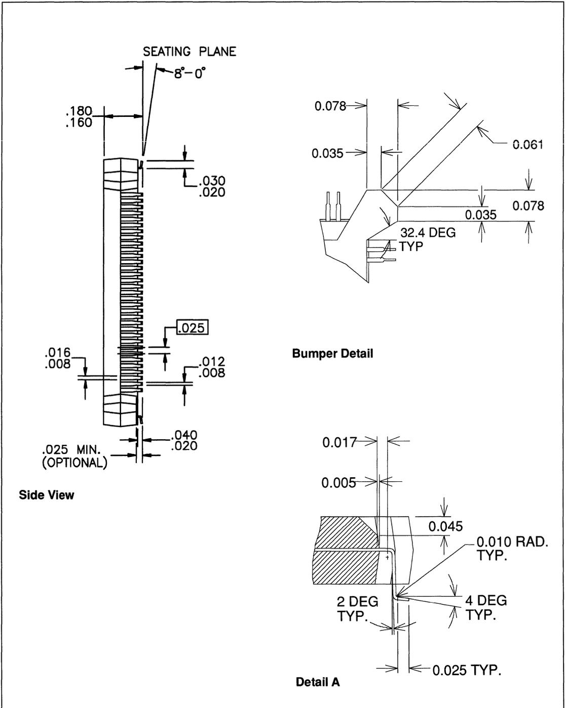
FIGURE D-1. 132-PIN PQFP PACKAGE DIMENSIONS (CONTINUED)
