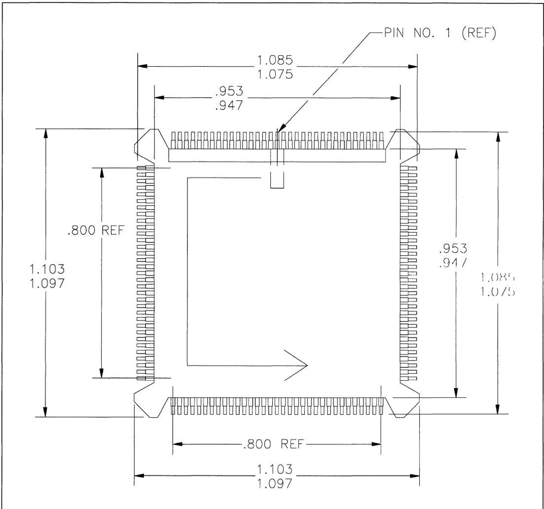
FIGURE D-1. 132-PIN PQFP PACKAGE DIMENSIONS
