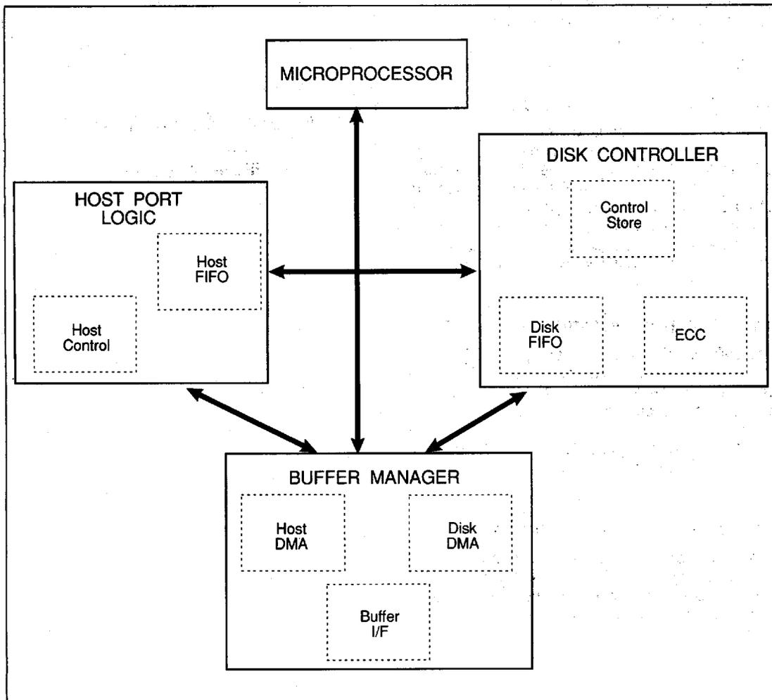
FIGURE 2-1. BLOCK DIAGRAM OF THE WD61C40A
