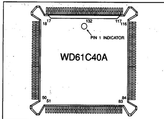
FIGURE 4-1. 132-PIN PQFP
