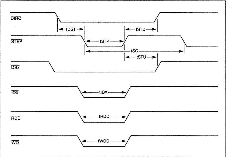
FIGURE 12. DISK DRIVE TIMING
