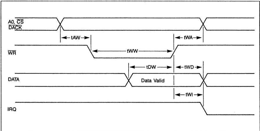
FIGURE 8. WRITE TIMING
