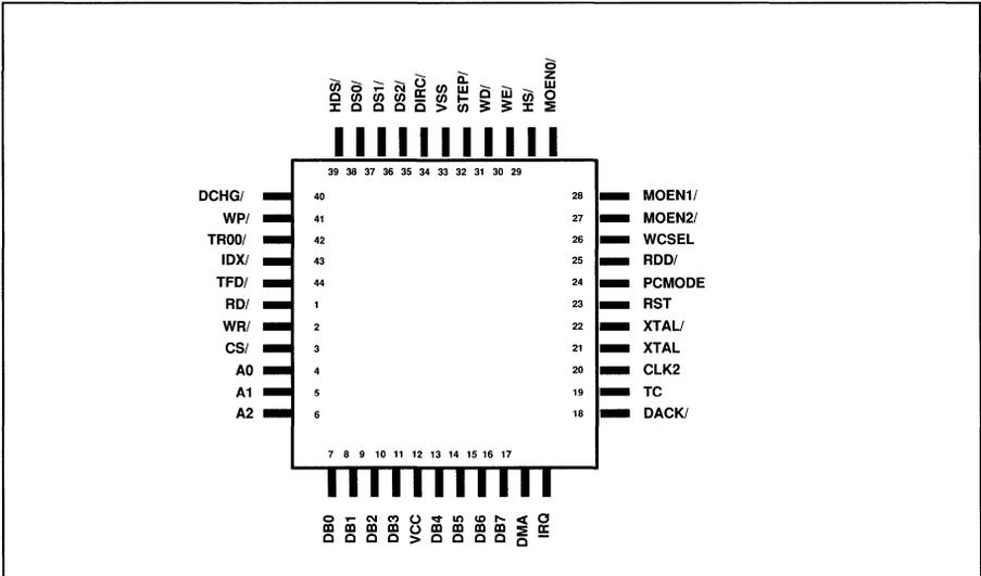
FIGURE 5. WD57C65 44-PIN PLCC
