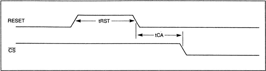
FIGURE 11. RESET TIMING
