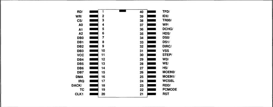
FIGURE 4. WD57C65 40-PIN DIP
