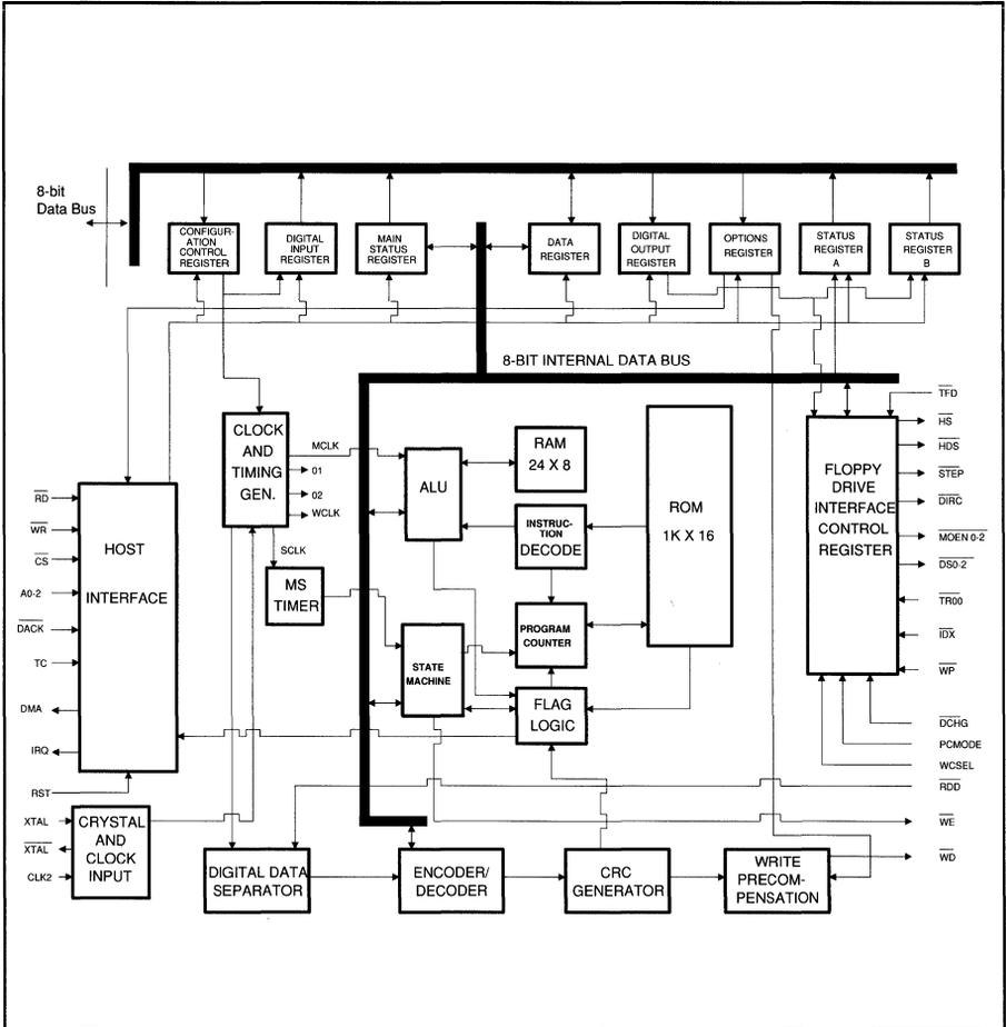
FIGURE 1. WD57C65 BLOCK DIAGRAM
