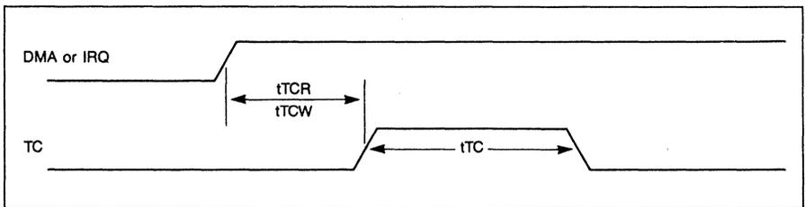
FIGURE 10. TERMINAL COUNT TIMING
