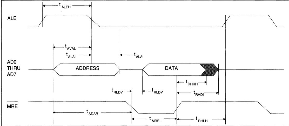
**FIGURE 21. MICROPROCESSOR READ TIMING (INTEL BUS)**
