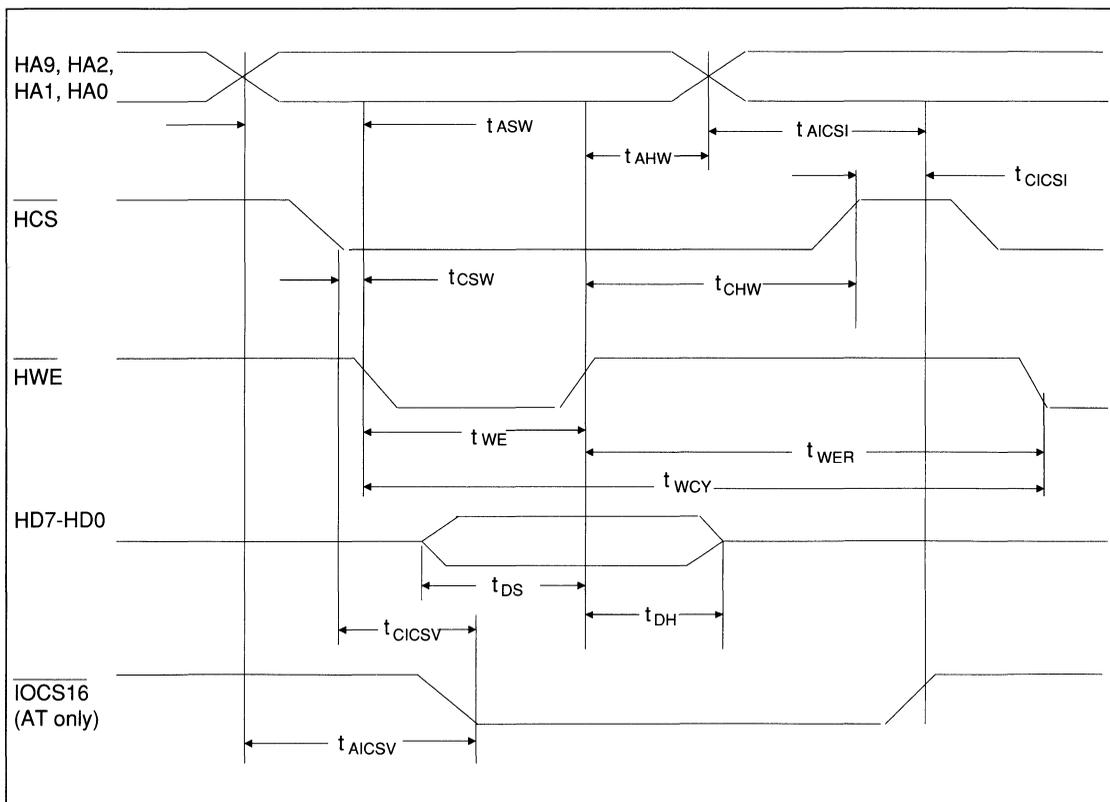
FIGURE 8. AT/XT HOST PROGRAMMED I/O WRITE TIMING
