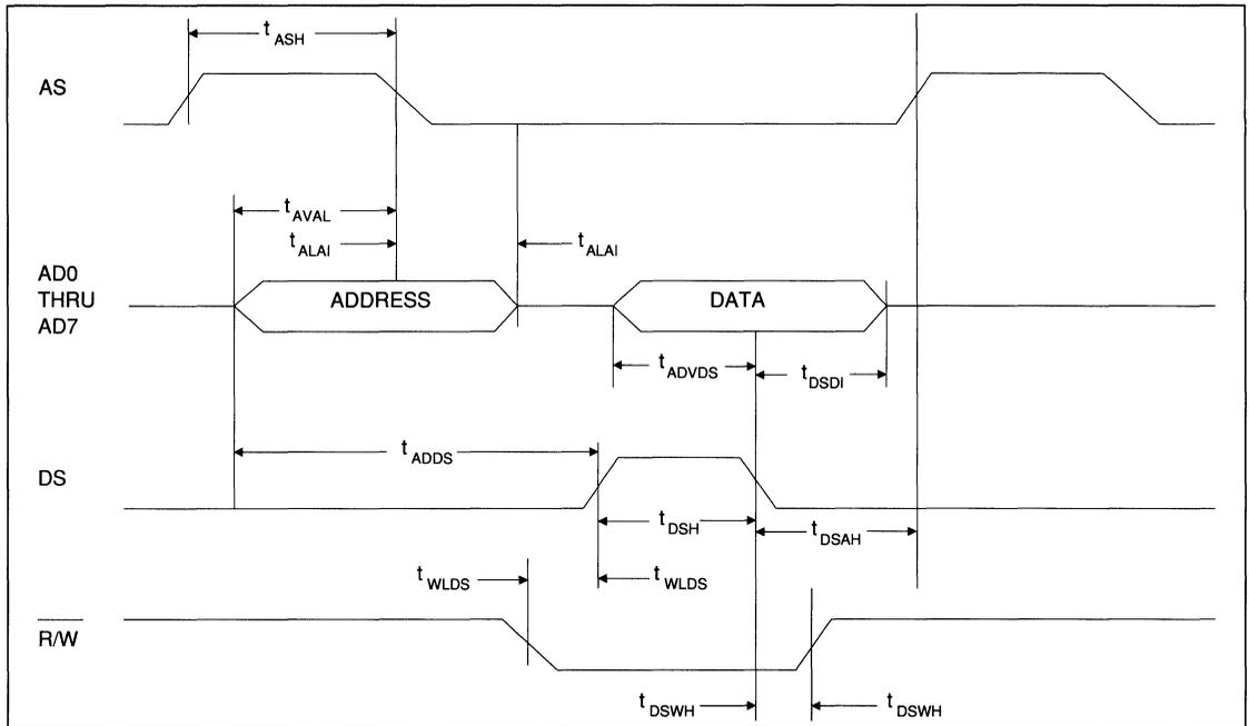
FIGURE 20. MICROPROCESSOR WRITE TIMING (MOTOROLA BUS)
