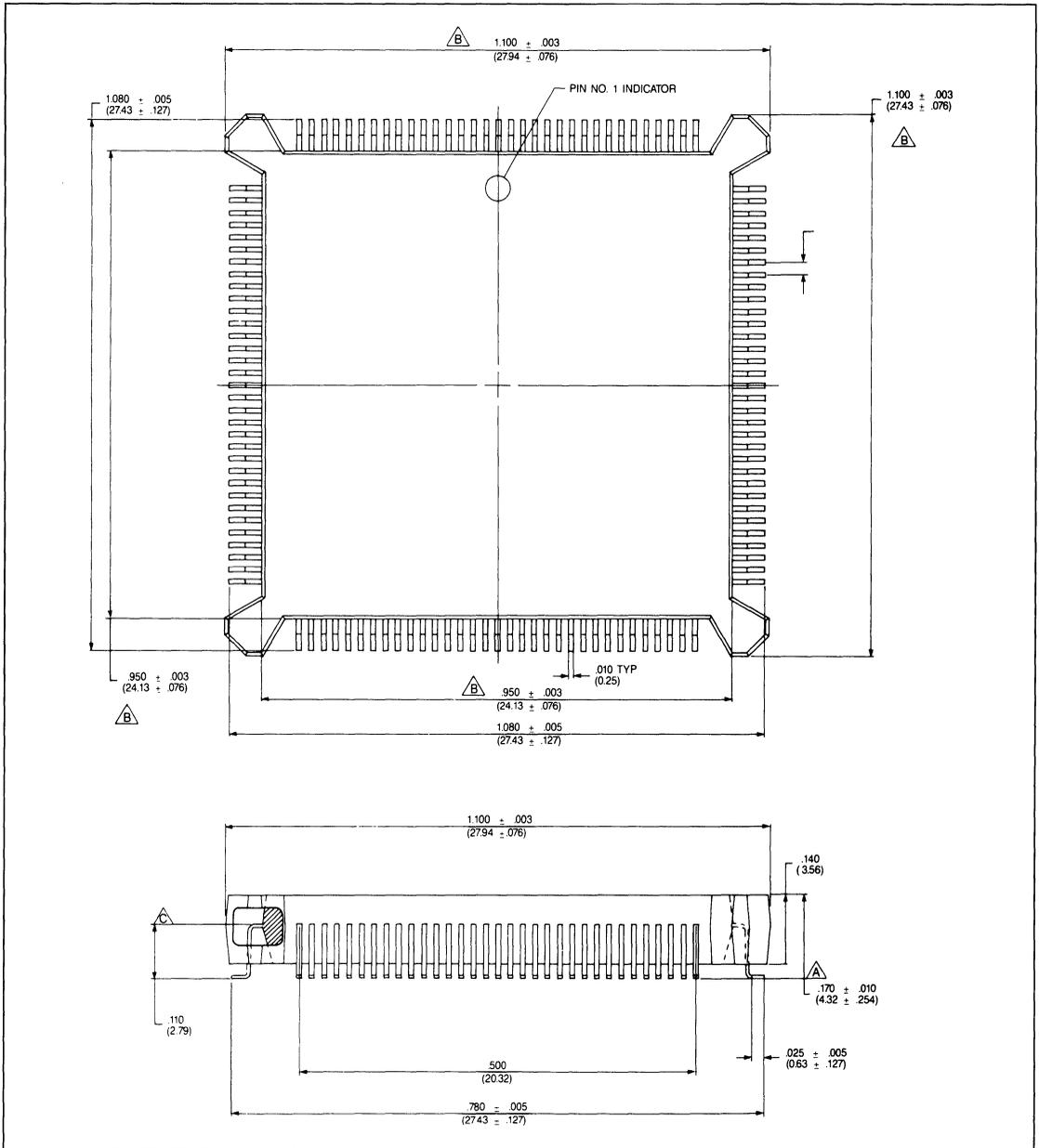
**FIGURE 35. 84 LEAD PQFP**
