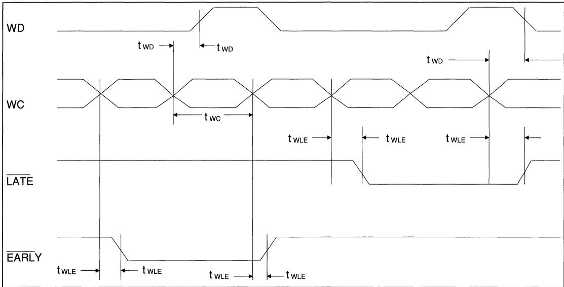
**FIGURE 23. WRITE DATA TIMING (MFM/RL MODE)**
