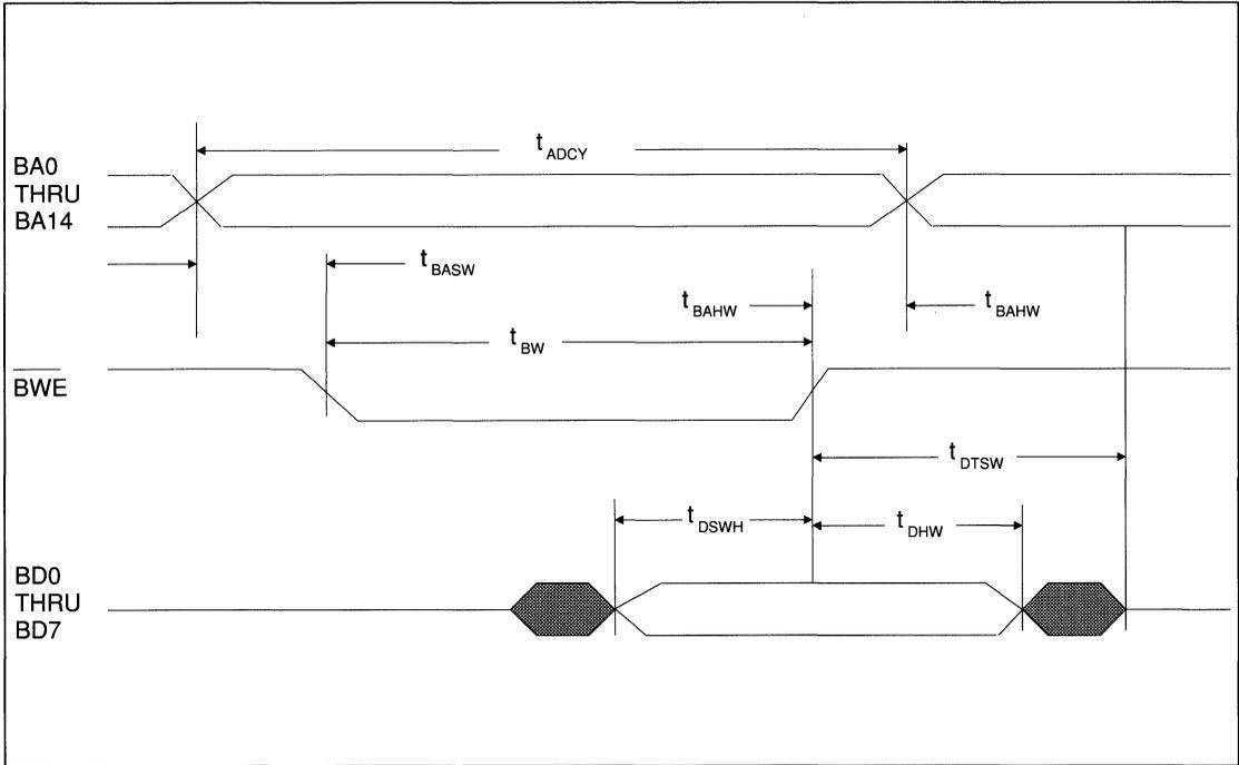
**FIGURE 17. BUFFER RAM WRITE TIMING (EXTERNAL OSCILLATOR)**
