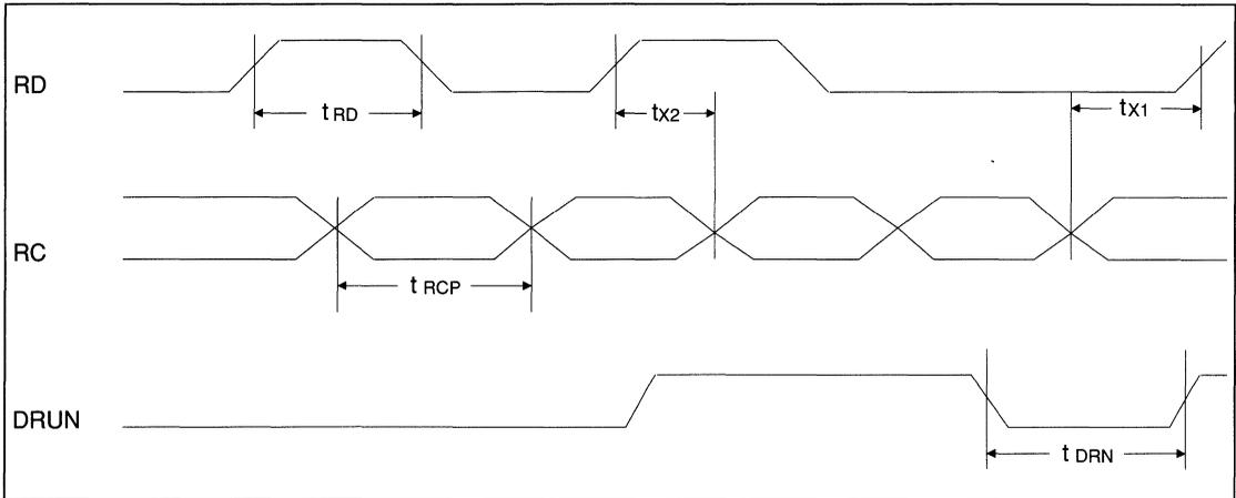
FIGURE 25. READ DATA TIMING (MFM/RLI)
