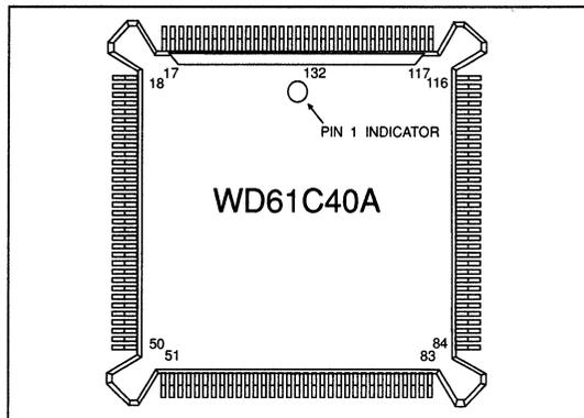
FIGURE 4-1. 132-PIN PQFP
