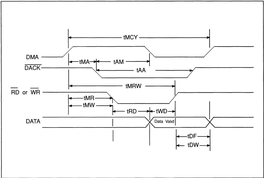
FIGURE 5-3. DMA TIMING
