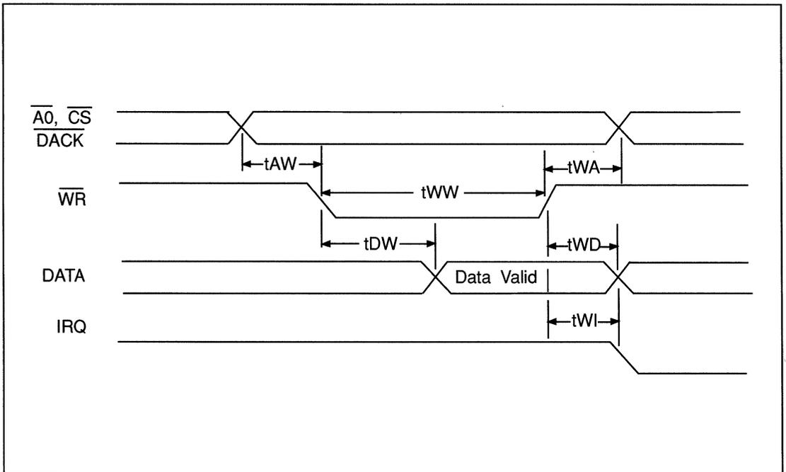
FIGURE 5-2. WRITE TIMING
