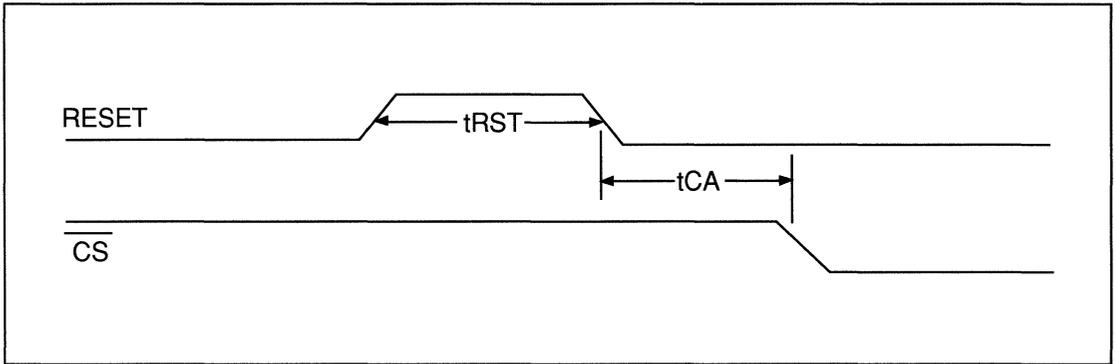
FIGURE 5-5. RESET TIMING
