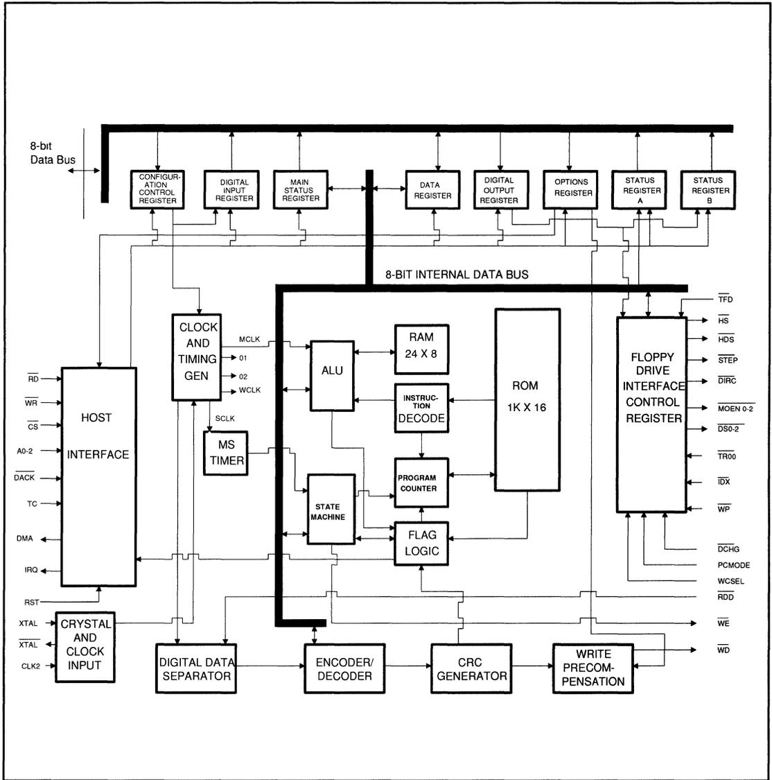
FIGURE 2-2. WD57C65 BLOCK DIAGRAM
