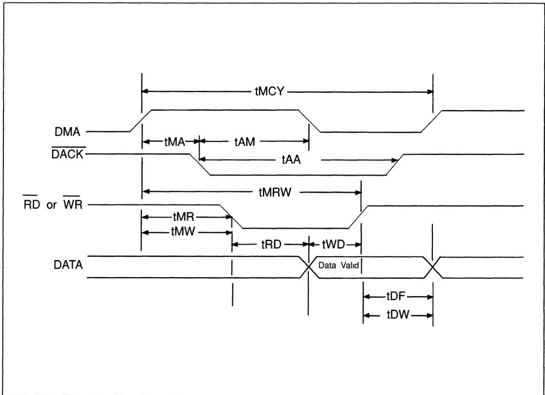
FIGURE 18-3. DMA TIMING
