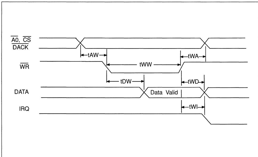
FIGURE 18-2. WRITE TIMING
