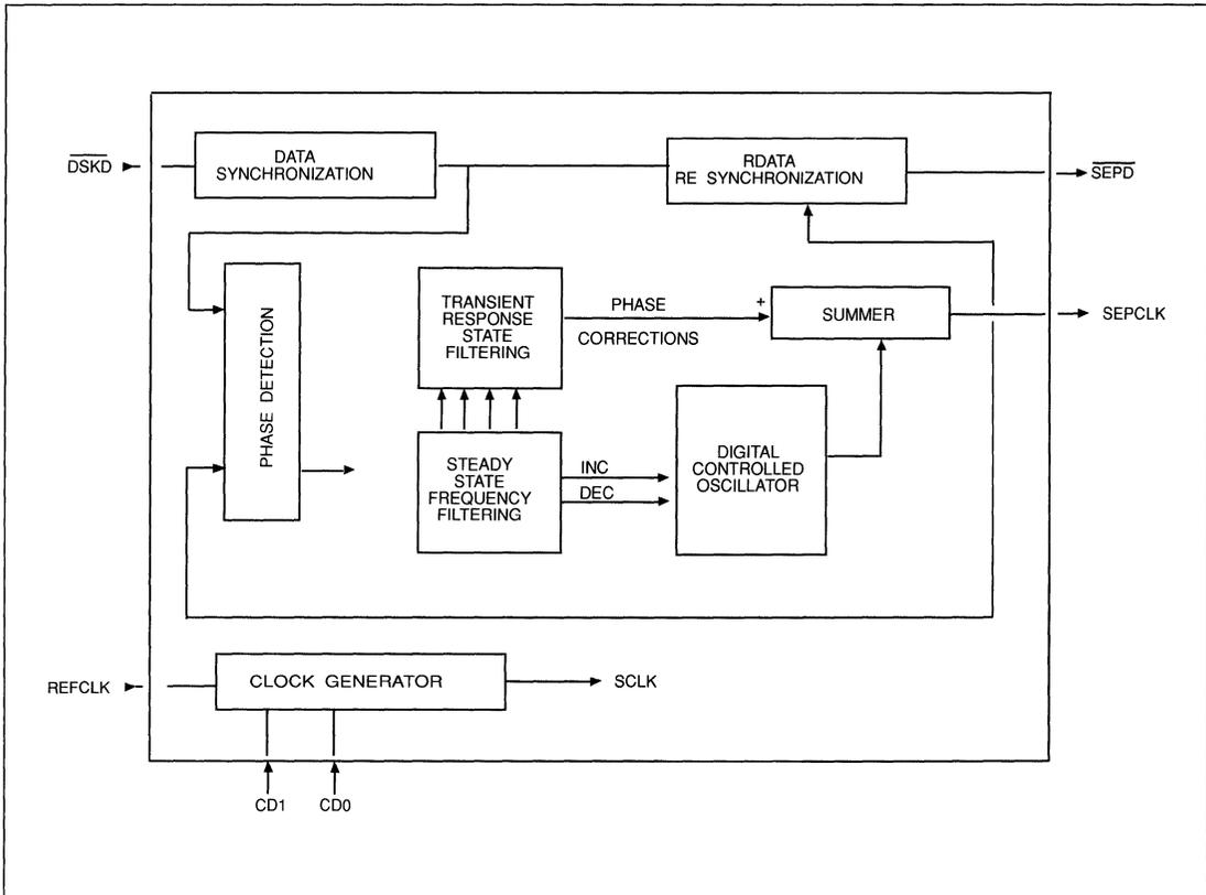
FIGURE 13-1. WD92C32 SIMPLIFIED BLOCK DIAGRAM
