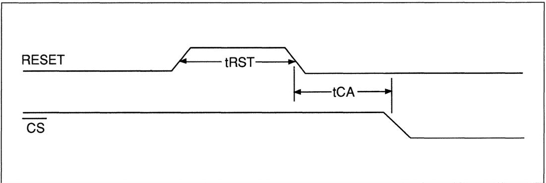
FIGURE 18-5. RESET TIMING
