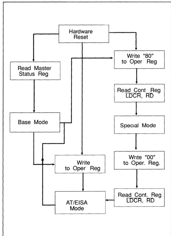
FIGURE 9-1. FLOW DIAGRAM BASE, SPECIAL & AT/EISA MODES
