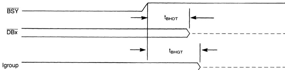
NOTE: Igroup = signals driven by an Initiator =  $\overline{ATN}$ ,  $\overline{ACK}$
