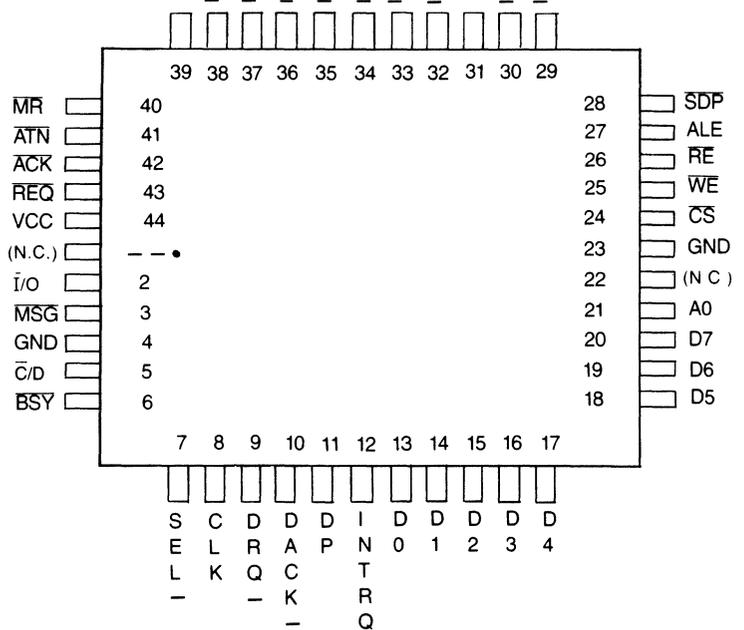
NOTE: Pin labeled N C. should be left not connected.
