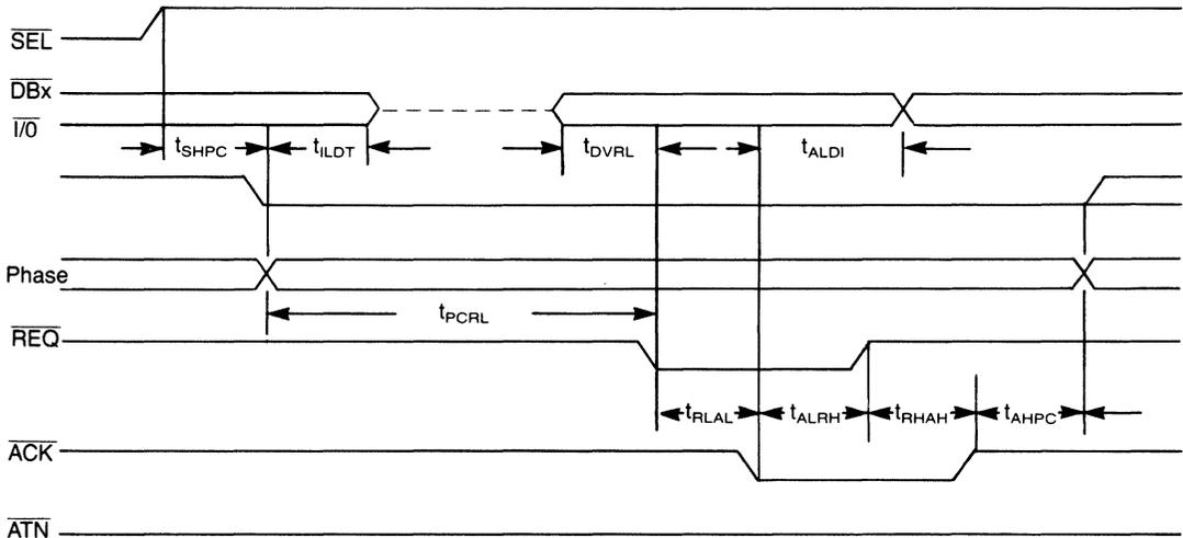
NOTE: Phase = signals that define the bus phase  $\overline{C/D}$ ,  $\overline{MSG}$
