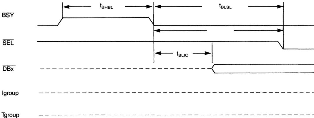
NOTE: Tgroup = signals driven by a Target =  $\overline{I/O}$ ,  $\overline{C/D}$ ,  $\overline{MSG}$ ,  $\overline{REQ}$
