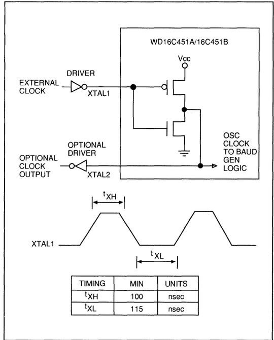
**FIGURE 6-1. EXTERNAL CLOCK INPUT (8.0 MHz MAXIMUM)**
