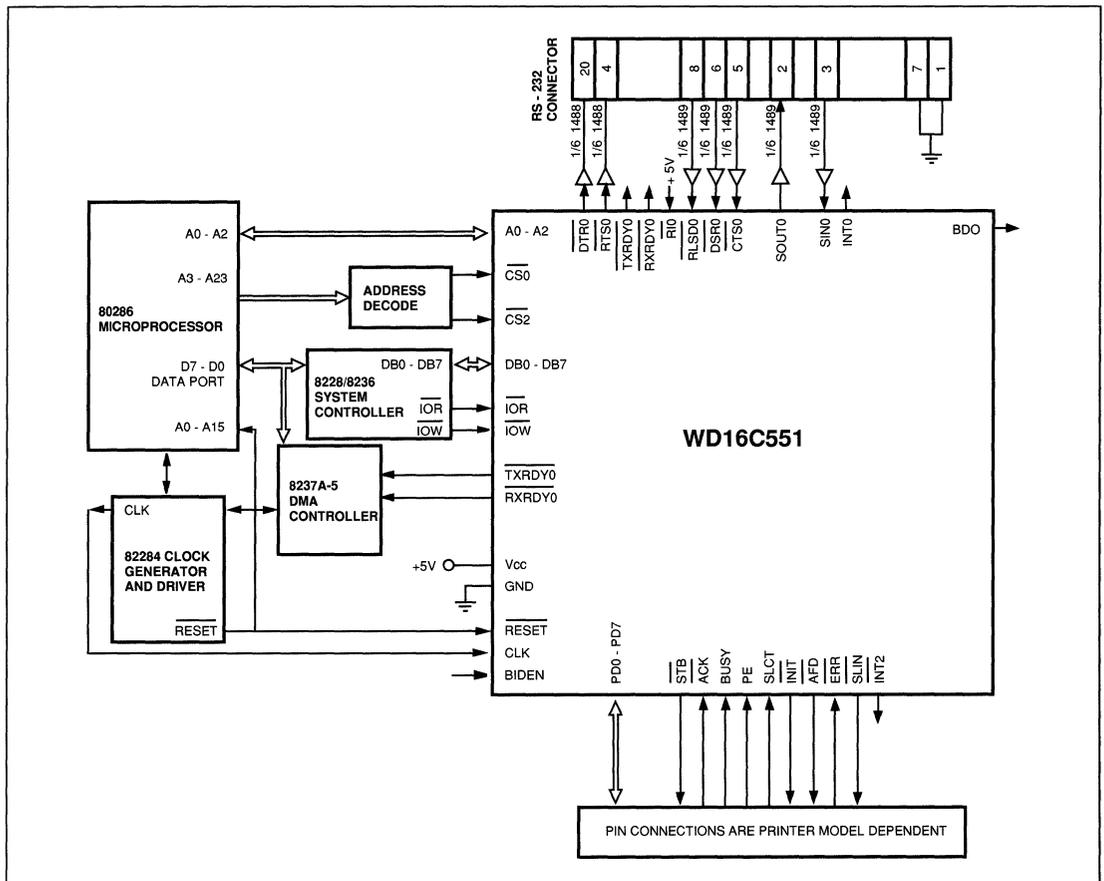
FIGURE 5-2. TYPICAL 16-BIT MICROPROCESSOR/RS-232 TERMINAL INTERFACE USING THE WD16C551
