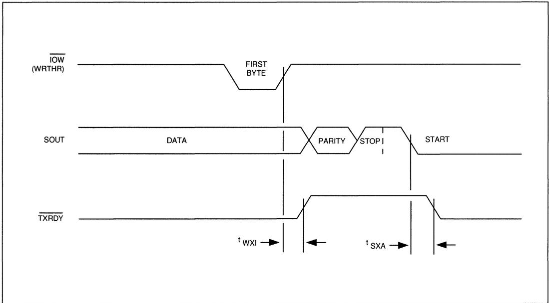
**FIGURE 7-10. TRANSMITTER DMA MODE 0 TIMING**
