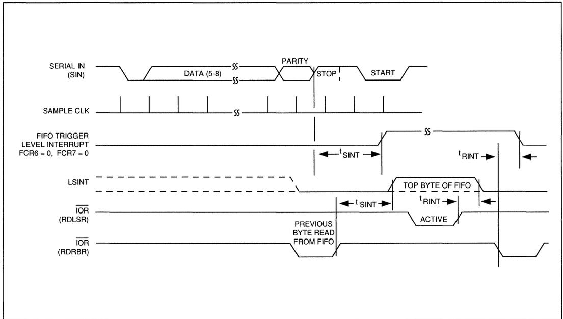
FIGURE 7-7. RCVR FIFO SIGNALING TIMING AFTER FIRST BYTE (RBR Already Set)
