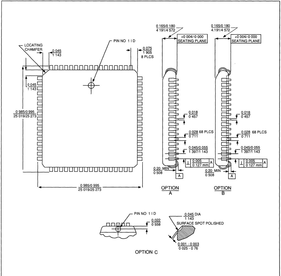
FIGURE 8-1. 68-PIN PLCC PACKAGE DIMENSIONS
