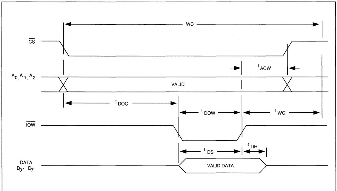
FIGURE 7-5. WRITE CYCLE TIMING
