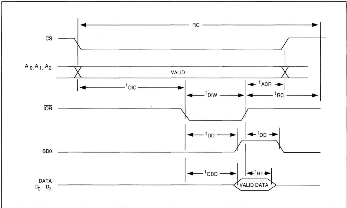
FIGURE 7-4. READ CYCLE TIMING
