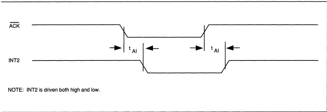
FIG. 7-13. WD16C451/WD16C451A PARALLEL PORT INTERRUPT TIMING
