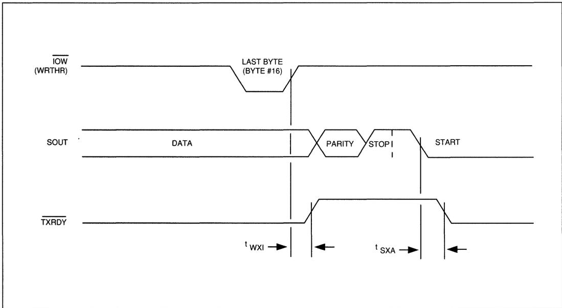
**FIGURE 7-11. TRANSMITTER DMA MODE 1 (FCR0 = 1 and FCR3 = 1)**
