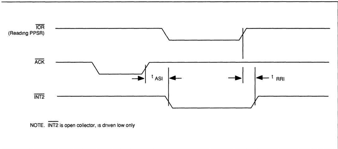
FIG. 7-14. WD16C551/WD16C451B PARALLEL PORT INTERRUPT TIMING
