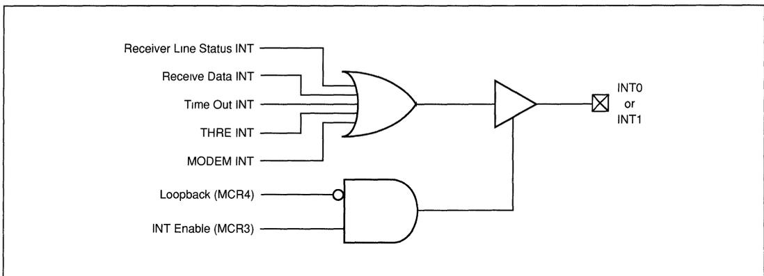
FIGURE 3-1. INTERRUPT SIGNAL LOGIC
