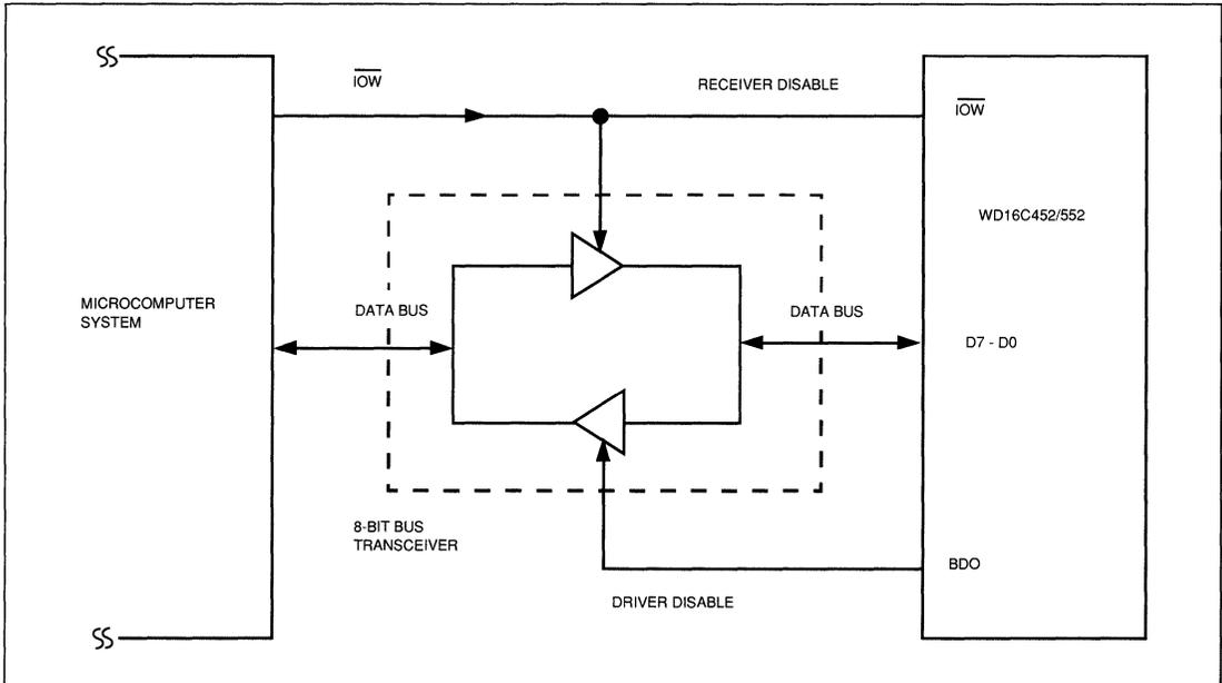
FIGURE 5-1. TYPICAL INTERFACE FOR A HIGH-CAPACITY DATA BUS
