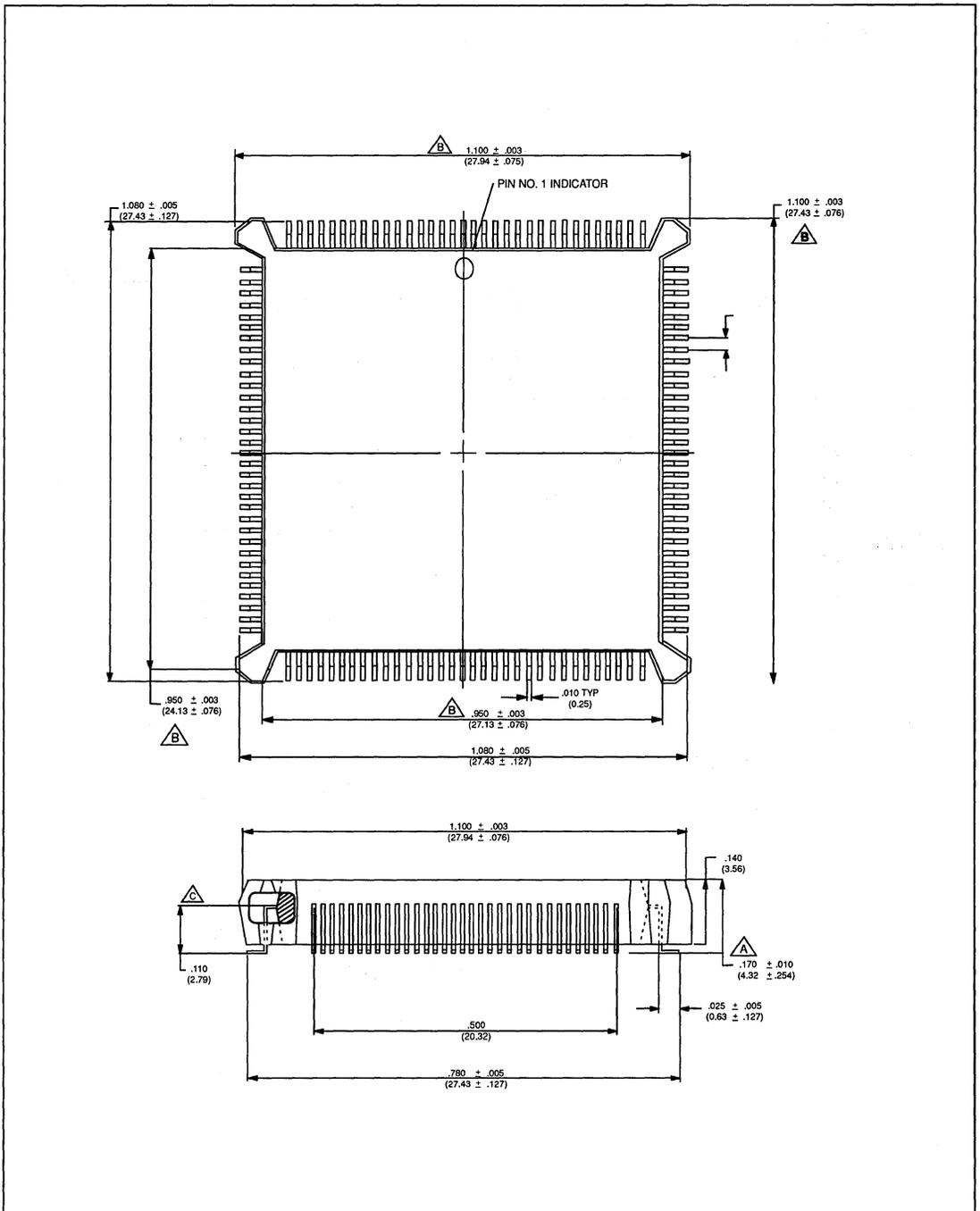
FIGURE 36. 84 LEAD PQFP
