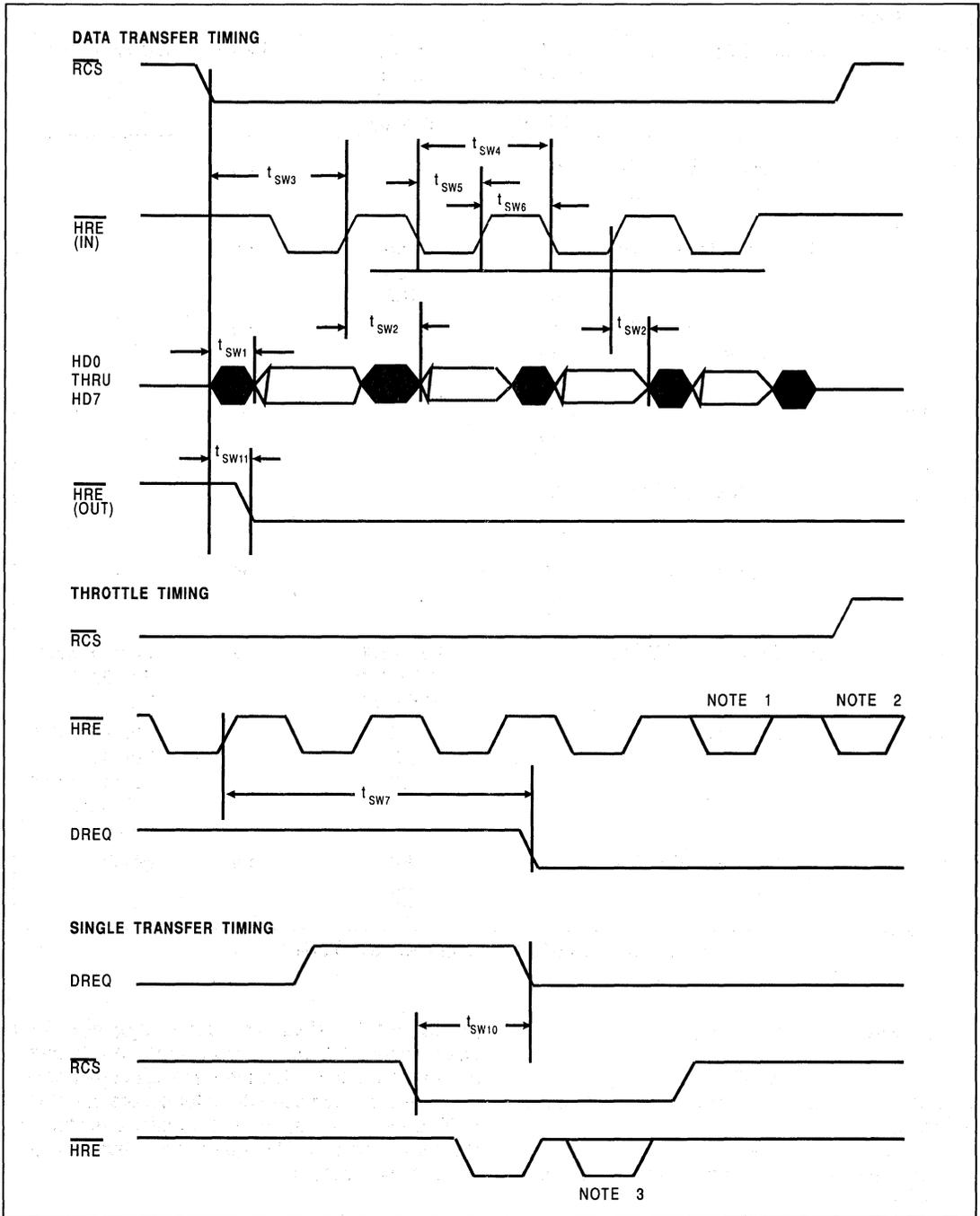
FIGURE 15. SLAVE HOST DMA READ TIMING
