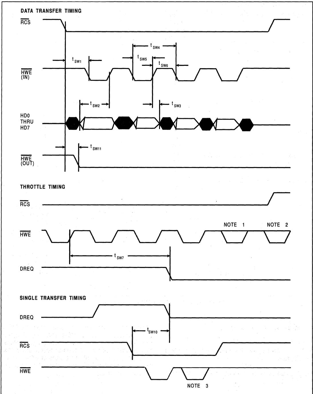
FIGURE 14. SLAVE HOST DMA WRITE TIMING
