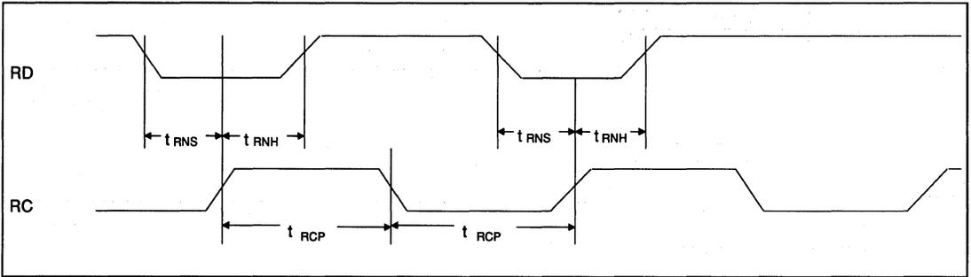
FIGURE 27. READ DATA TIMING (NRZ MODE)
