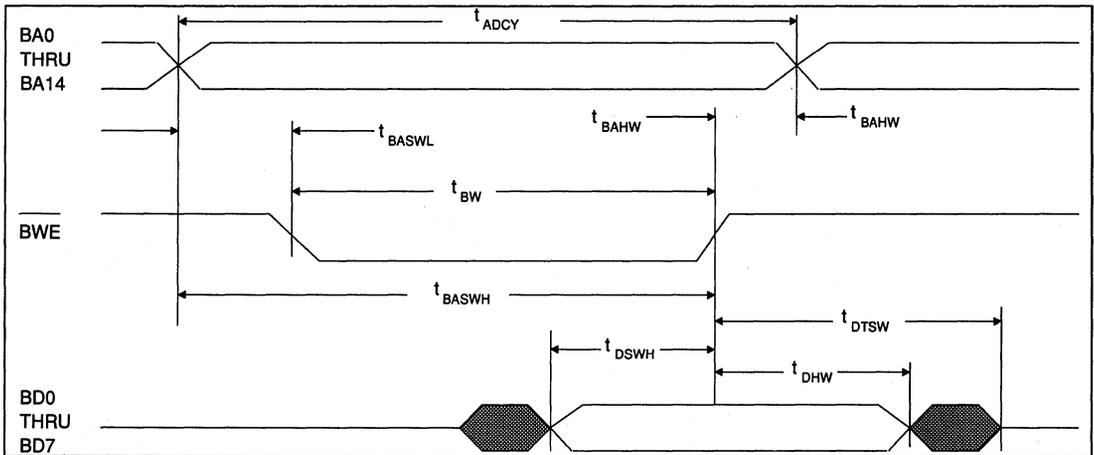
**FIGURE 16. BUFFER RAM WRITE TIMING (INTERNAL OSCILLATOR)**
