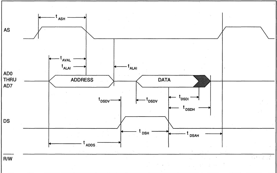
FIGURE 23. MICROPROCESSOR READ TIMING (MOTOROLA BUS)
