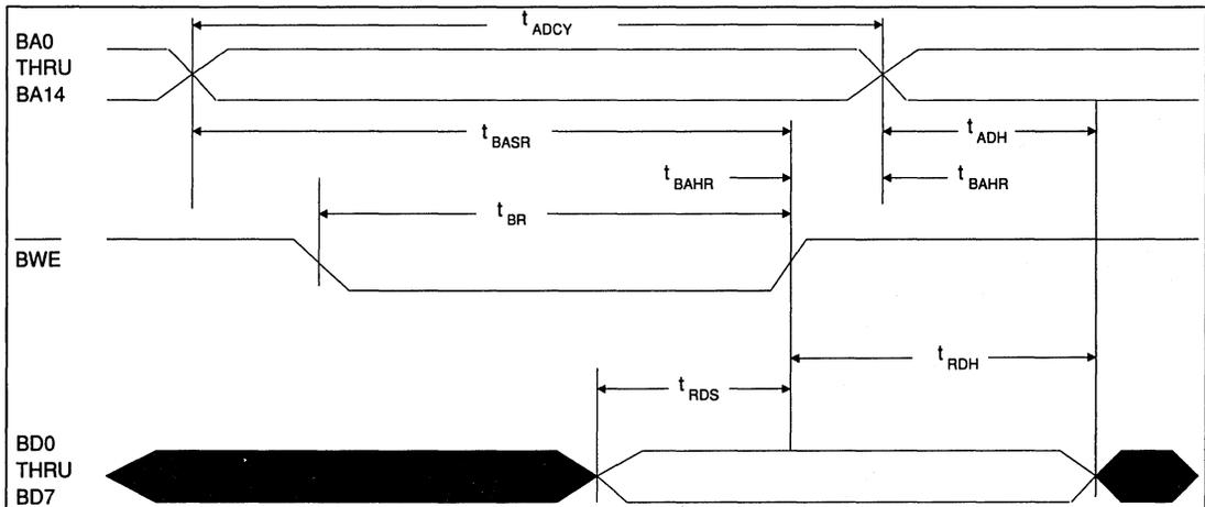
FIGURE 17. BUFFER READ TIMING (INTERNAL OSCILLATOR)
