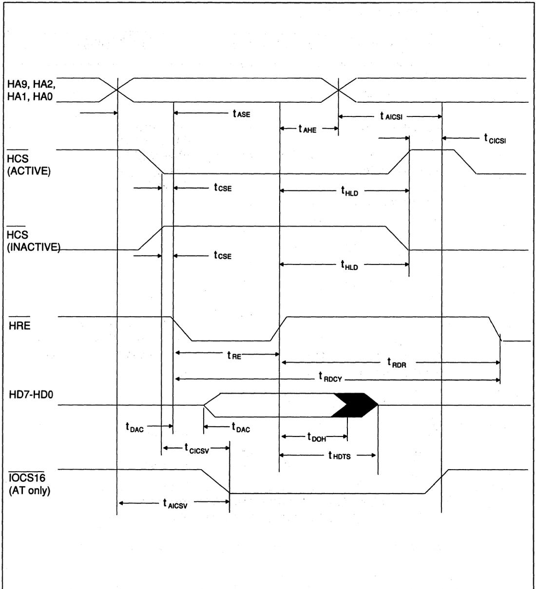
FIGURE 9. AT/XT HOST PROGRAMMED I/O READ TIMING
