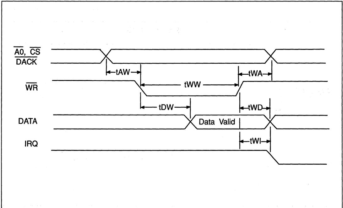
FIGURE 18-2. WRITE TIMING
