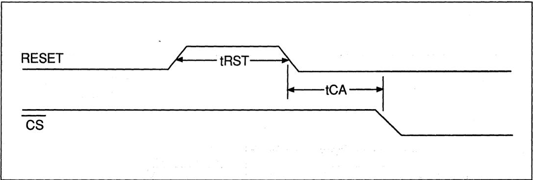
FIGURE 18-5. RESET TIMING
