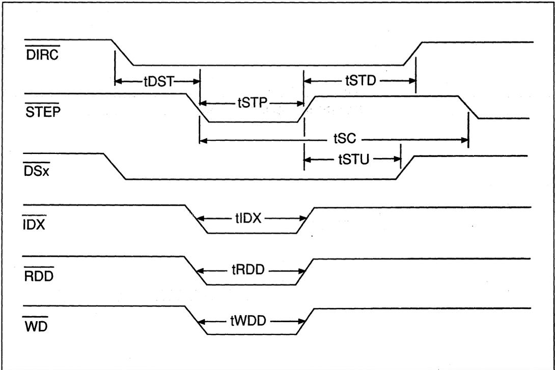
FIGURE 18-6. DISK DRIVE TIMING
