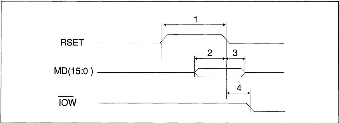
FIGURE 7-1. RESET TIMING
