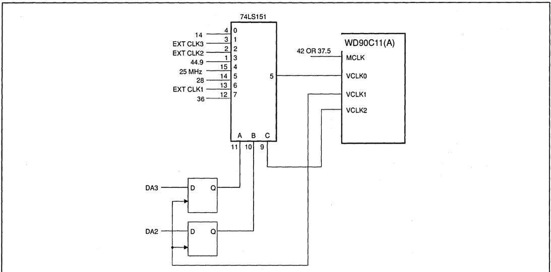
FIGURE A-10. EXTERNAL VIDEO CLOCK MULTIPLEXING
