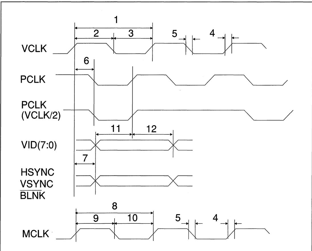
FIGURE 7-2. CLOCK AND VIDEO TIMING
