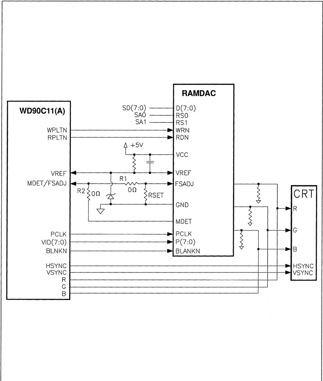
FIGURE A-7. WD90C11(A) WITH RAMDAC INTERFACE
