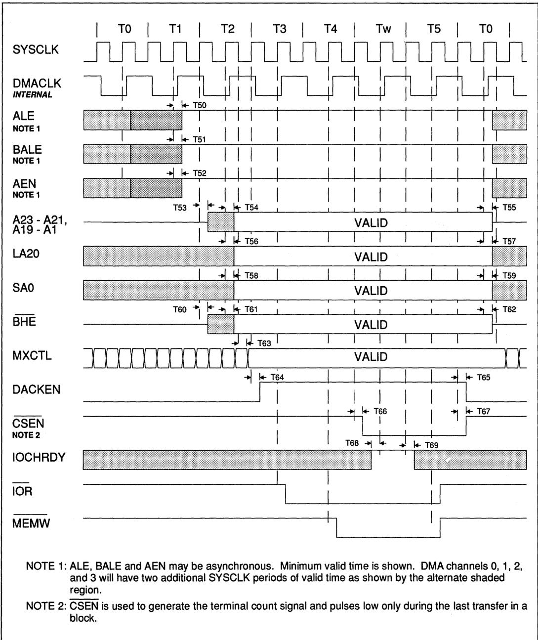
FIGURE 12-42. BASIC DMA CYCLE, DEFAULT TIMING
