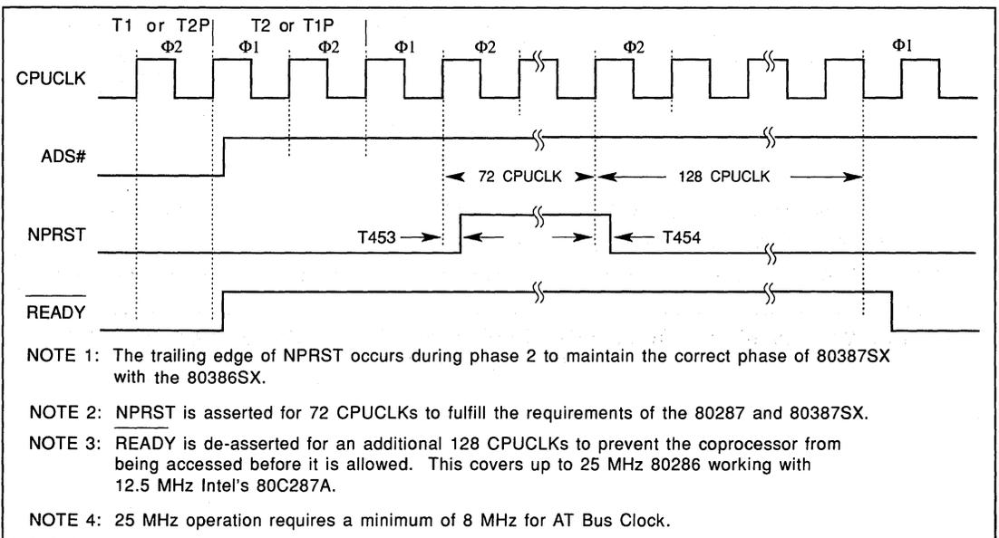
FIGURE 12-56. 80386SX - COPROCESSOR RESET (NPRST) INITIATED BY I/O TO PORT F1
