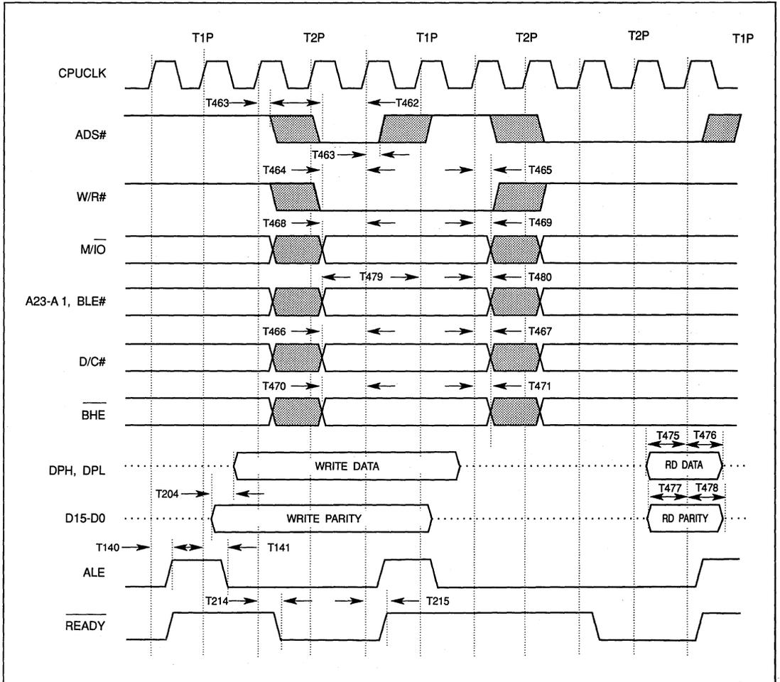
FIGURE 12-60. 80386SX - MISCELLANEOUS TIMING
