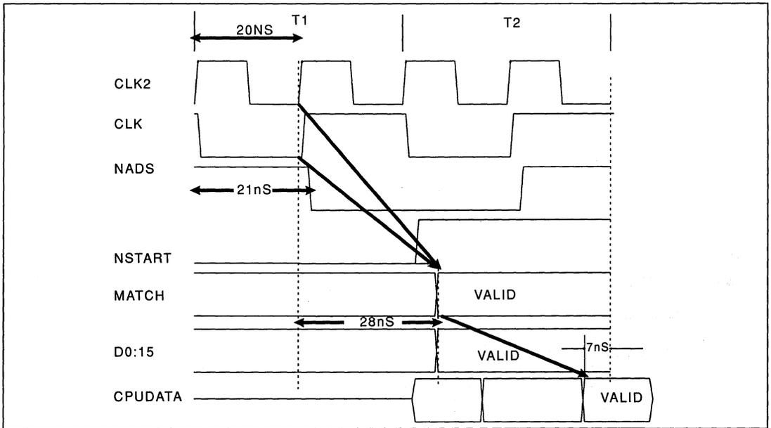
FIGURE 12-67. TAG RAM AND DATA RAM TIMING
