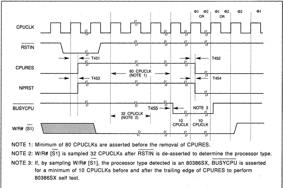
FIGURE 12-55. 80386SX - CPURES AND NPRST DURING POWER UP
