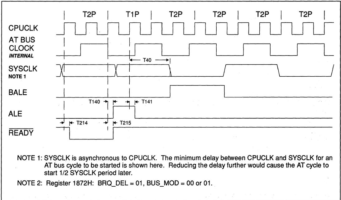
FIGURE 12-35. 80386SX CPU - BREQ DELAY = 1/2 CLOCK
