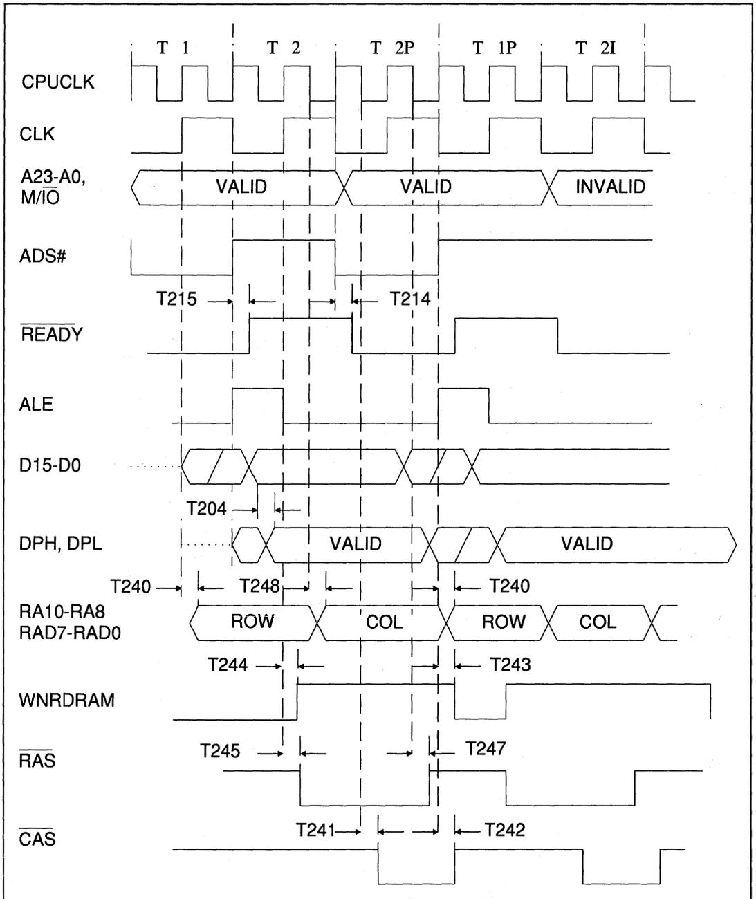
FIGURE 12-21. 80386SX - NON-PAGE MODE 01, 0 WAIT STATE READ (PIPELINE)
