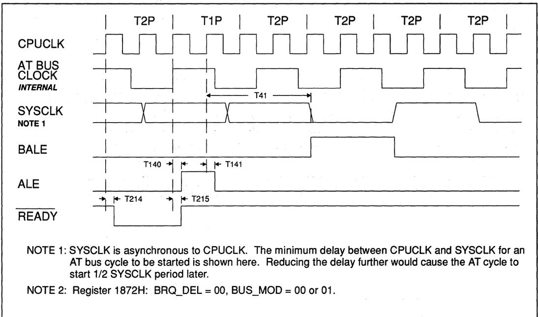
FIGURE 12-36. 80386SX - BREQ DELAY = 1 CLOCK
