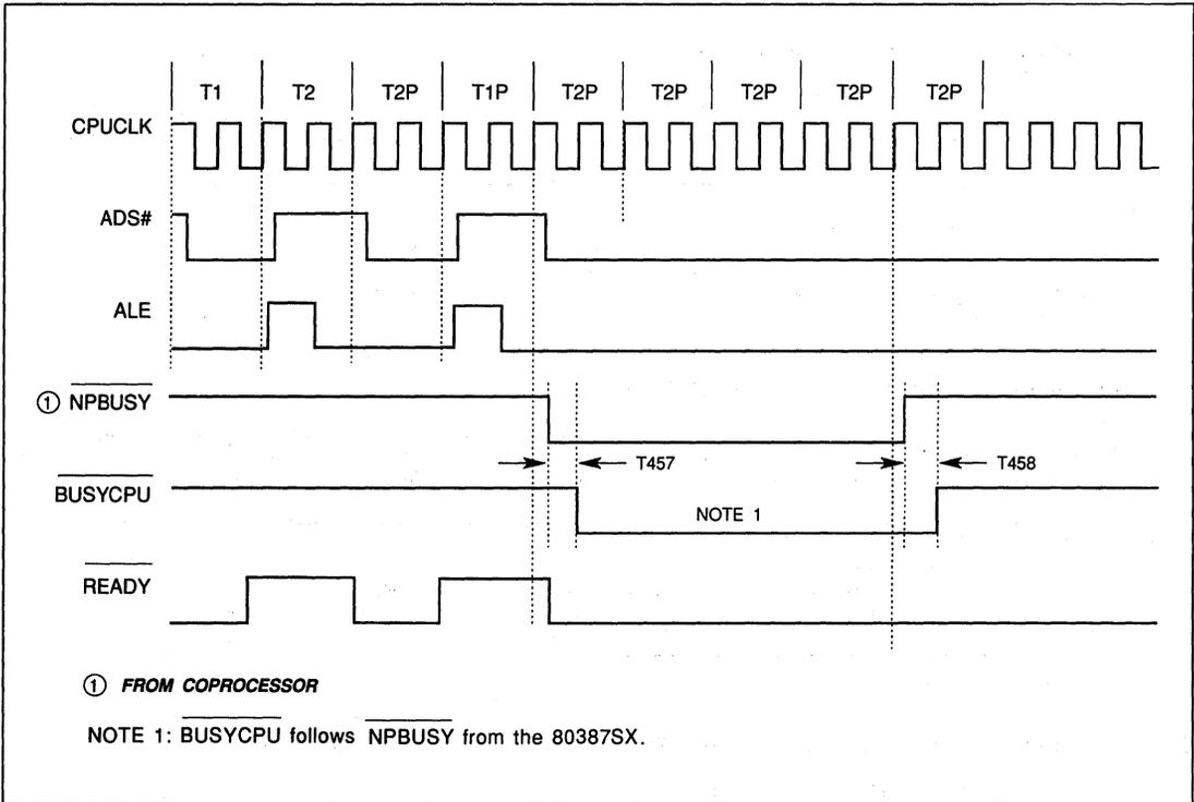
FIGURE 12-58. BUSYCPU ASSERTION DURING COPROCESSOR ACCESS
