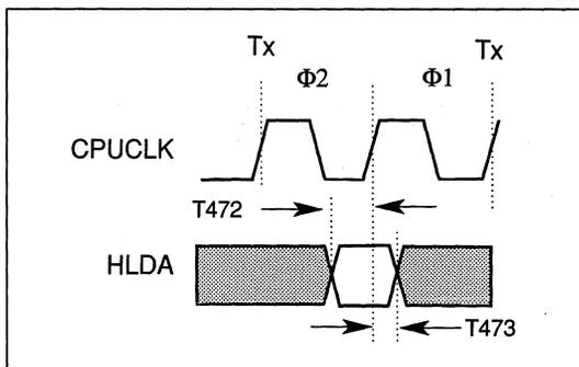
FIGURE 12-61. 80386SX - INPUT SETUP AND HOLD TIMING
