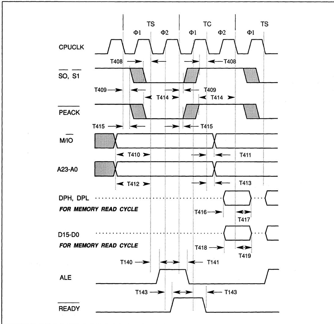
FIGURE 12-54. 80286 - MISCELLANEOUS TIMING
