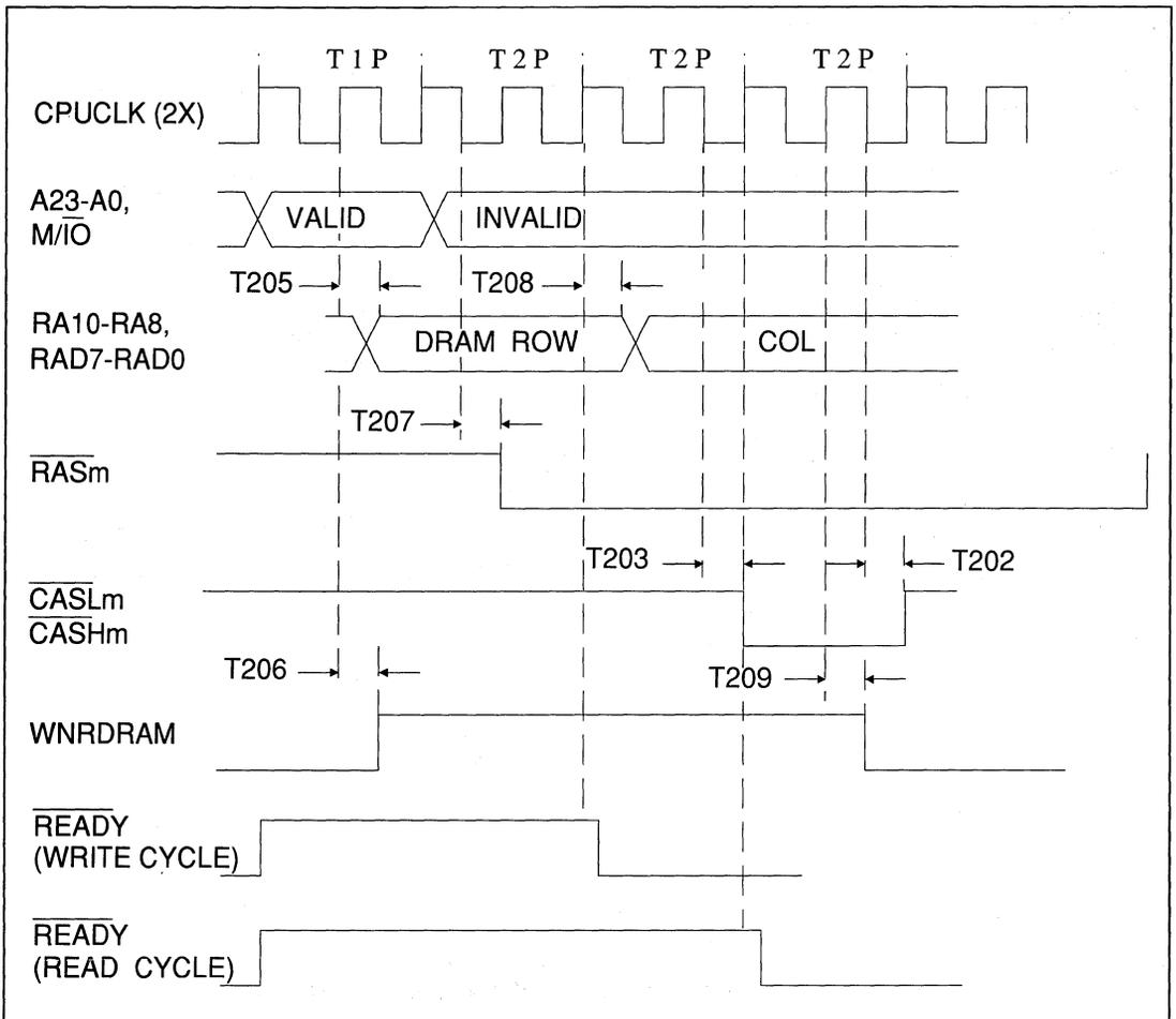
FIGURE 12-12. 80386SX - PAGE MODE, FIRST ACCESS READ/WRITE
