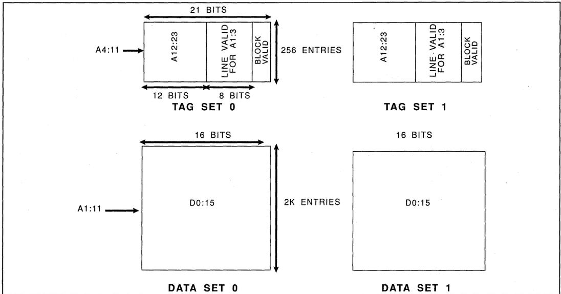
FIGURE 7-2. TAG RAM AND DATA RAM STRUCTURE
