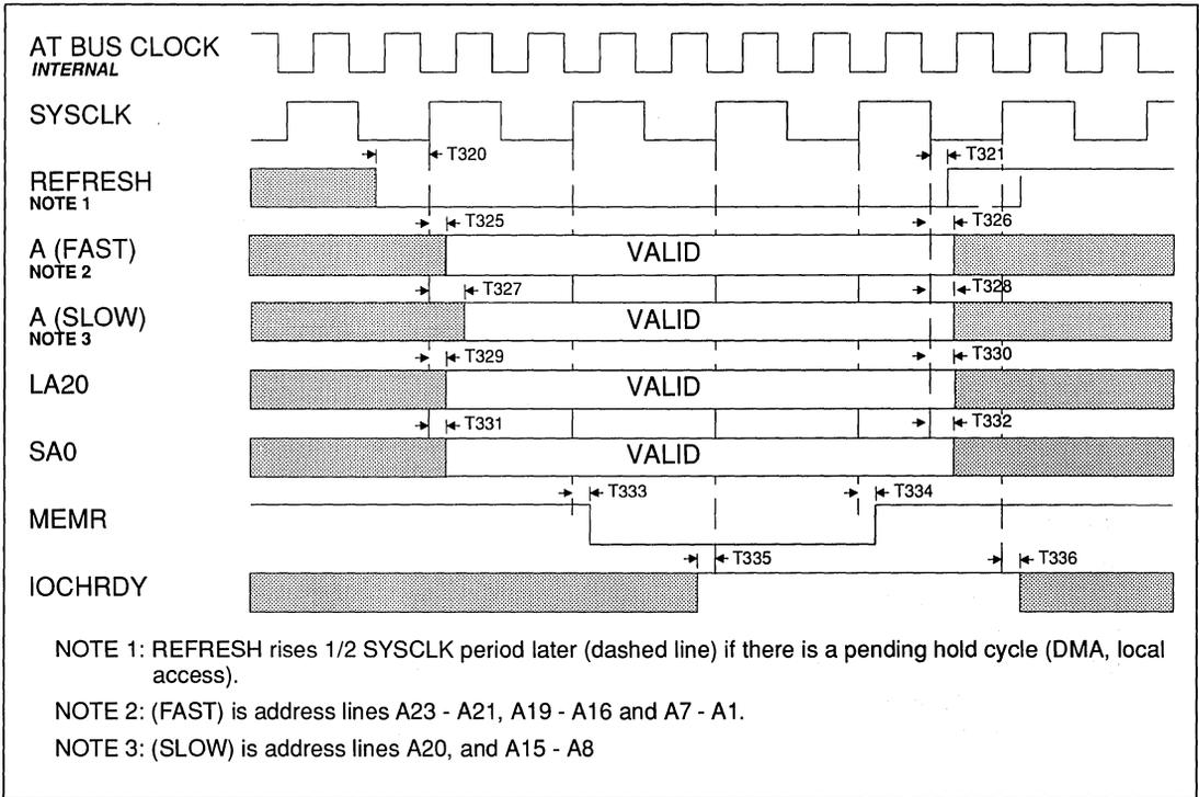
FIGURE 12-48. AT BUS REFRESH CYCLE, DEFAULT TIMING
