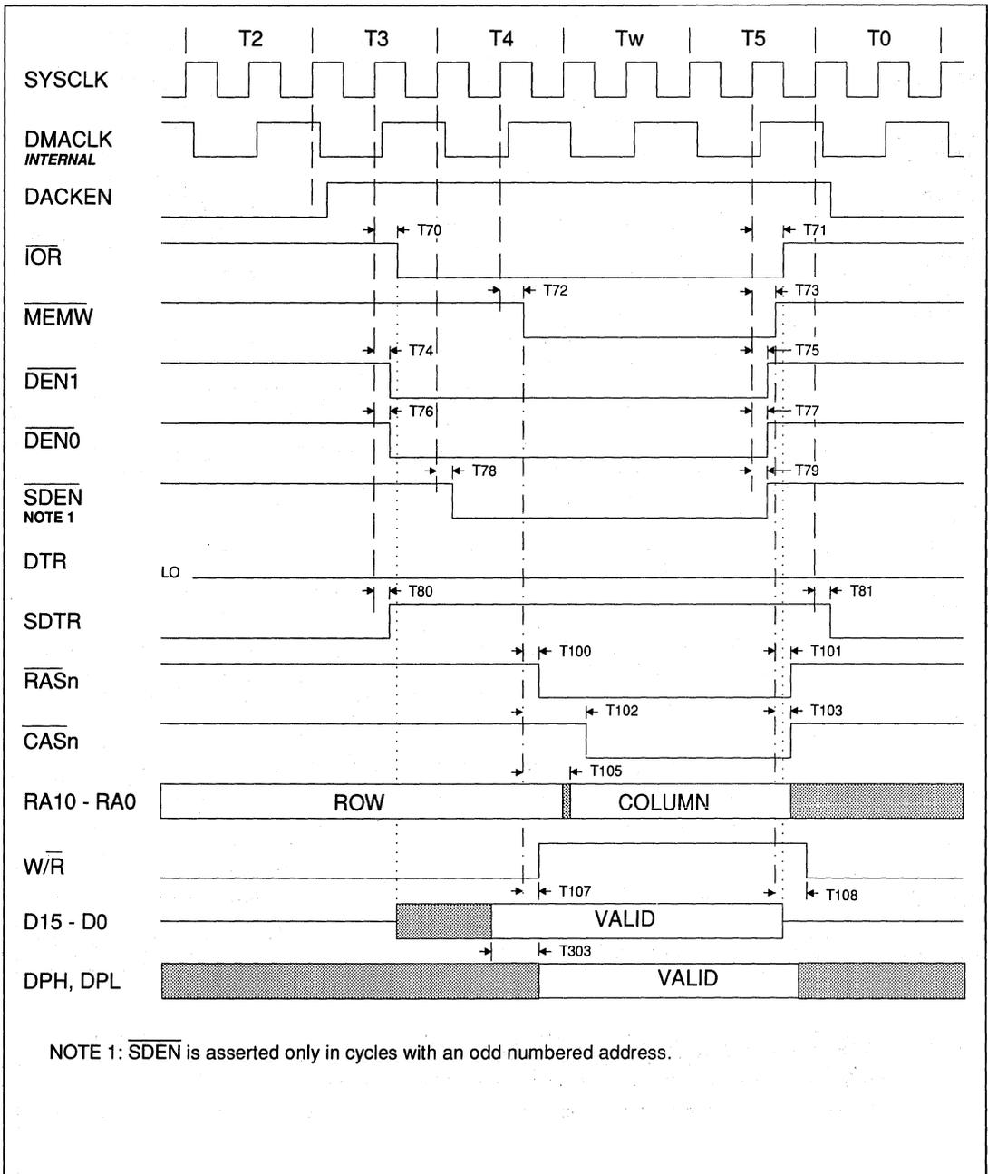
FIGURE 12-43. DMA CYCLE, 8-BIT I/O TO ON-BOARD MEMORY
