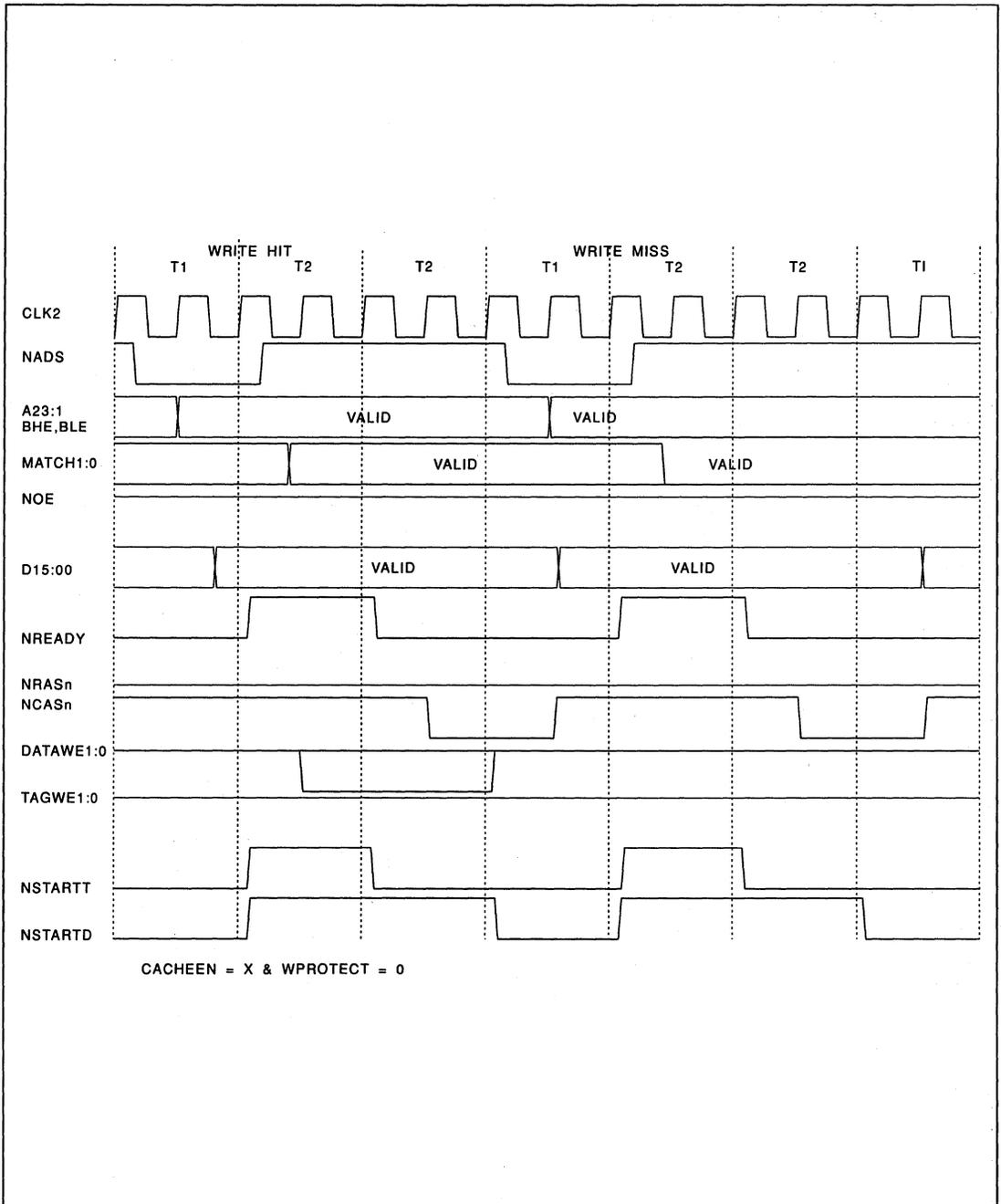
FIGURE 12-64. WRITE HIT/WRITE MISS CYCLE
