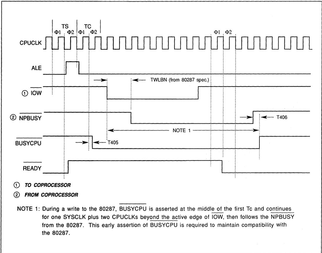
**FIGURE 12-52. 80286 - BUSYCPU ASSERTED DURING COPROCESSOR ACCESS**
