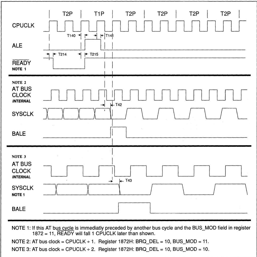
FIGURE 12-37. 80386SX CPU - SYNCHRONOUS CPUCLK TO SYSCLK
