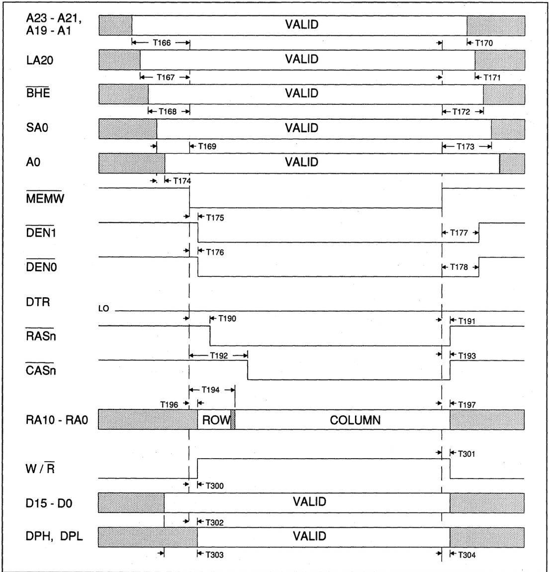
FIGURE 12-46. AT BUS MASTER, WRITE TO ON-BOARD MEMORY
