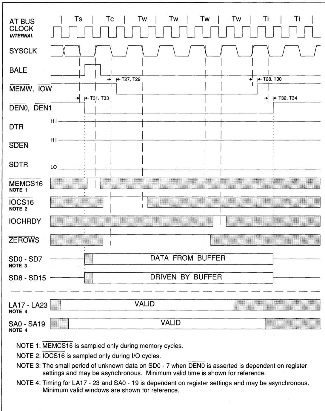
FIGURE 12-25. AT BUS I/O OR MEMORY WRITE: 8-BIT, EVEN BYTE, DEFAULT TIMING
