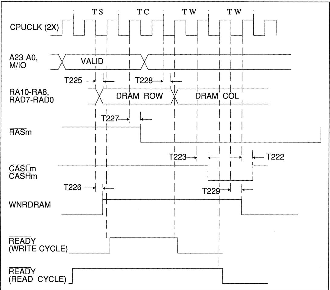
FIGURE 12-1. 80286 - PAGE MODE FIRST ACCESS READ/WRITE
