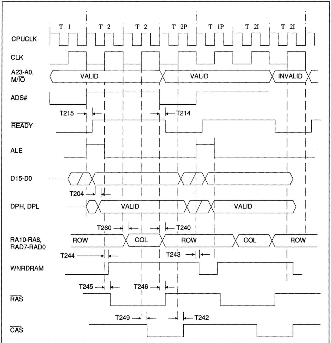
FIGURE 12-19. 80386SX - NON-PAGE MODE 00, 1 WAIT STATE WRITE (PIPELINE)
