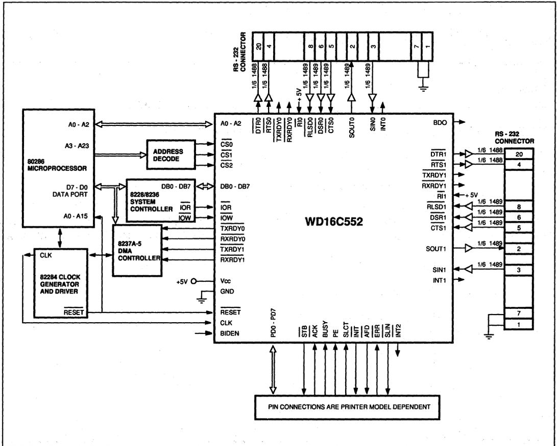
FIGURE 8-2. TYPICAL 16-BIT MICROPROCESSOR/RS-232 TERMINAL INTERFACE USING THE WD16C552
