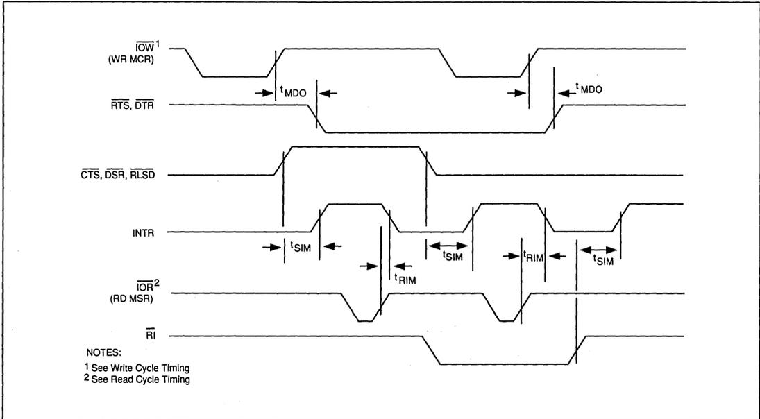
FIGURE B-3. MODEM CONTROL TIMING
