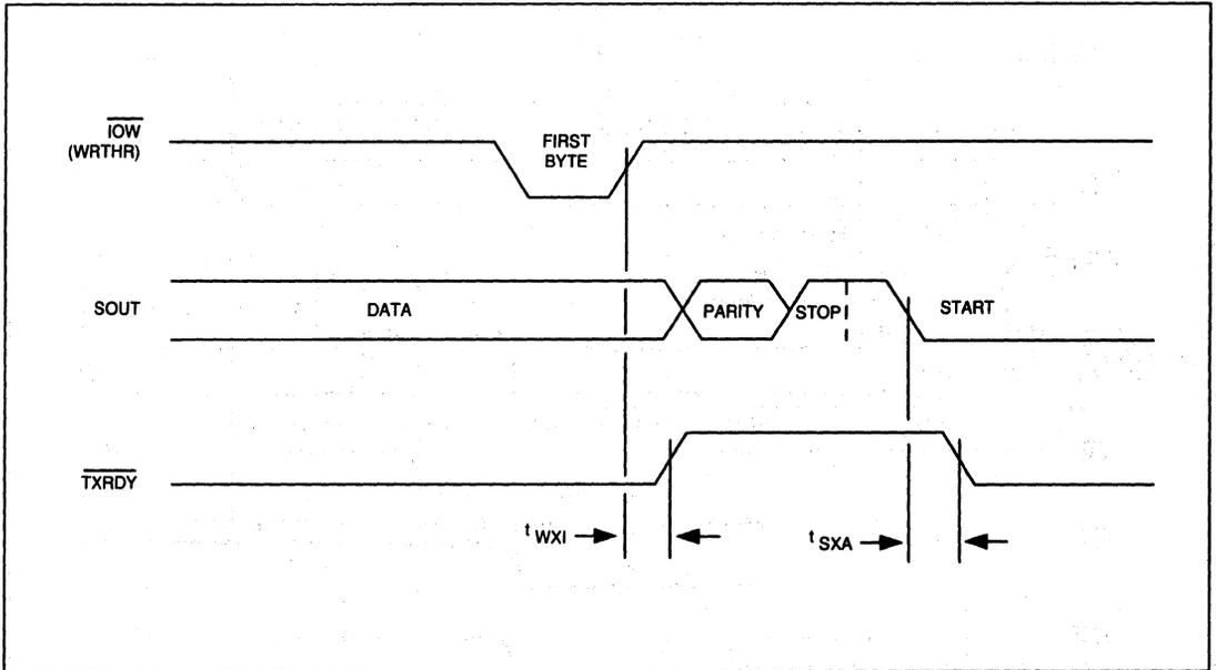
**FIGURE B-10. TRANSMITTER DMA MODE 0 TIMING**
