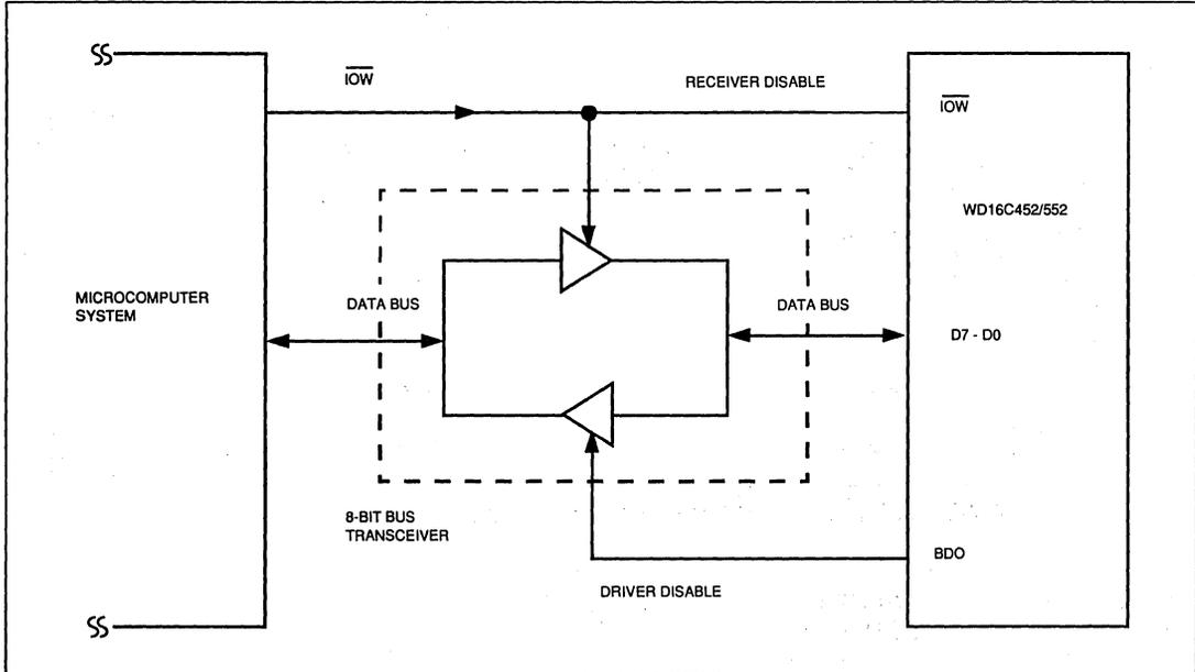
FIGURE 8-1. TYPICAL INTERFACE FOR A HIGH-CAPACITY DATA BUS
