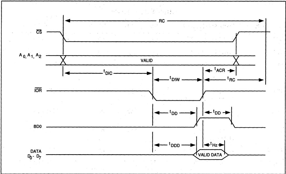
FIGURE B-4. READ CYCLE TIMING
