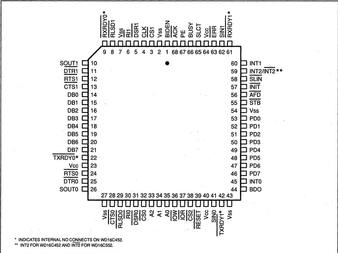
FIGURE 2-1. WD16C452/WD16C552 68-PIN QUAD ASSEMBLY
