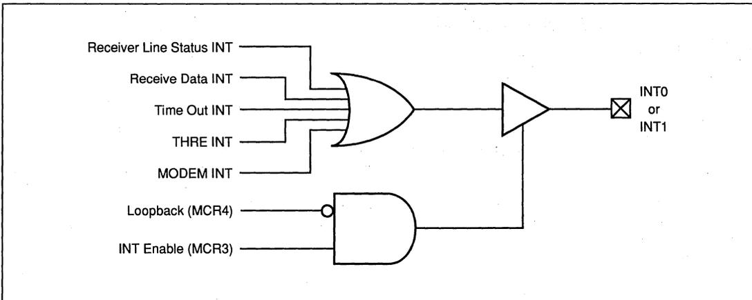
FIGURE 5-1. INTERRUPT SIGNAL LOGIC
