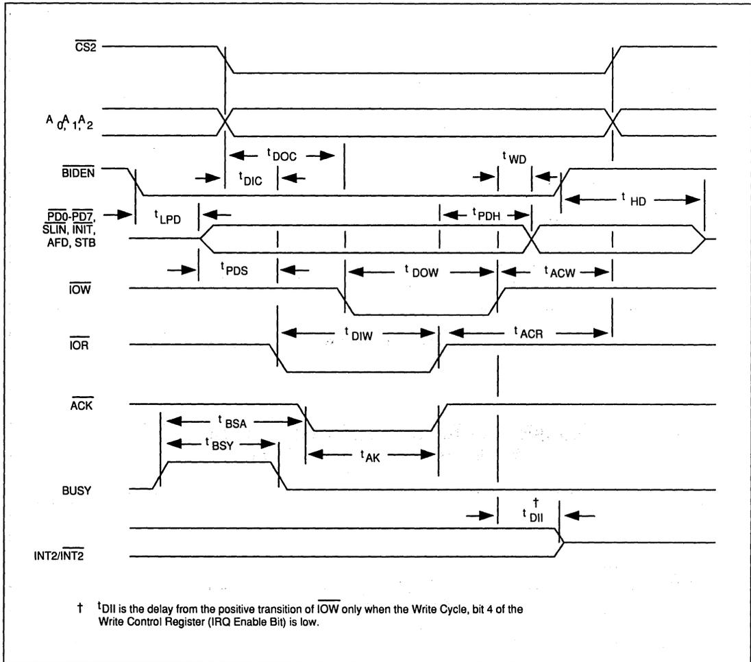
FIGURE B-12. PARALLEL PORT TIMING
