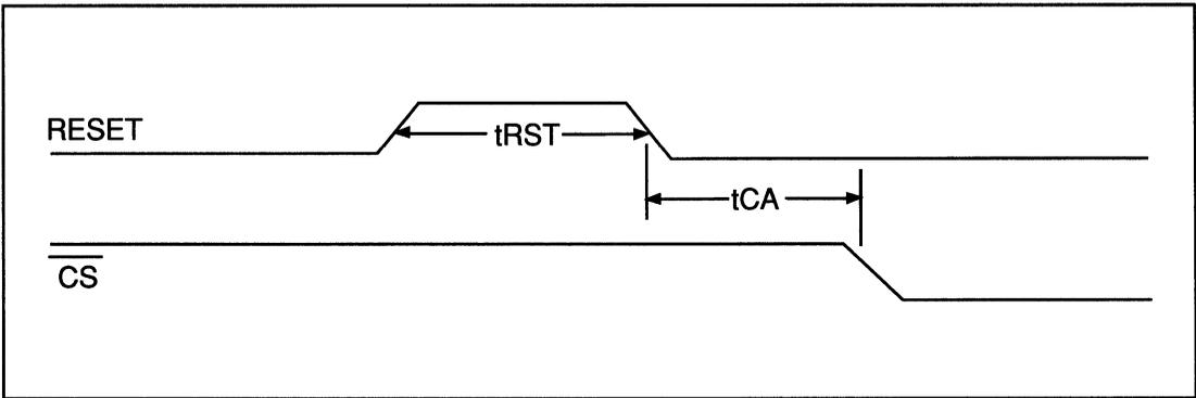
FIGURE 11. RESET TIMING
