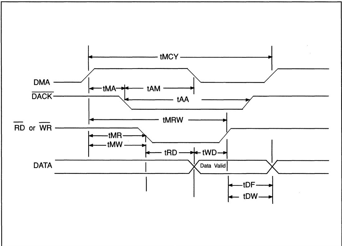
FIGURE 9. DMA TIMING
