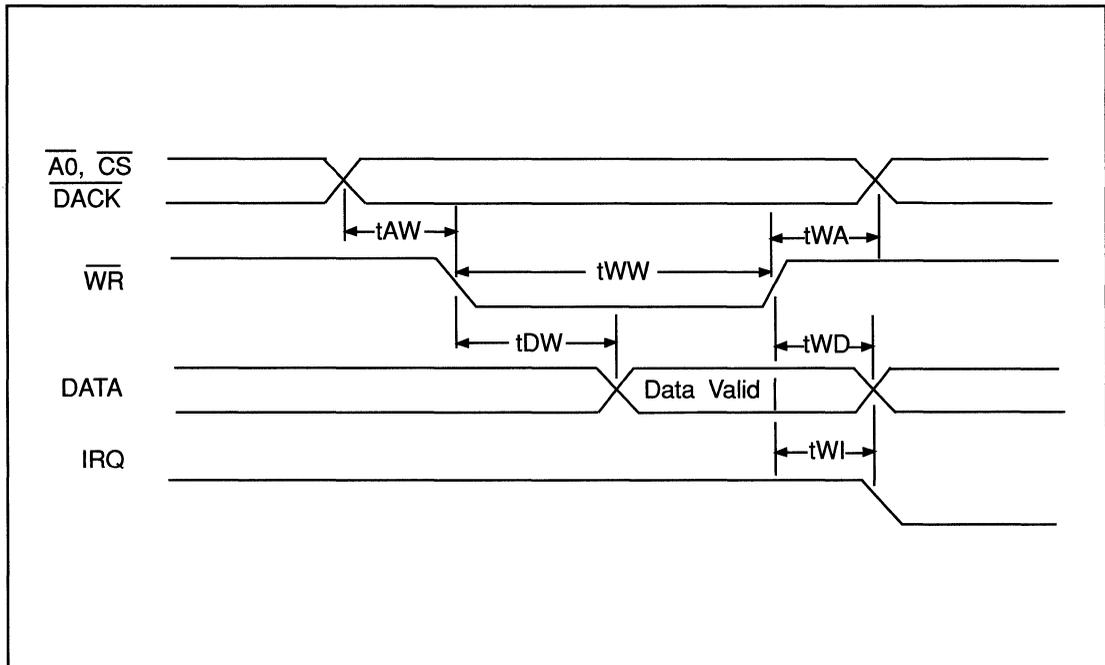
FIGURE 8. WRITE TIMING
