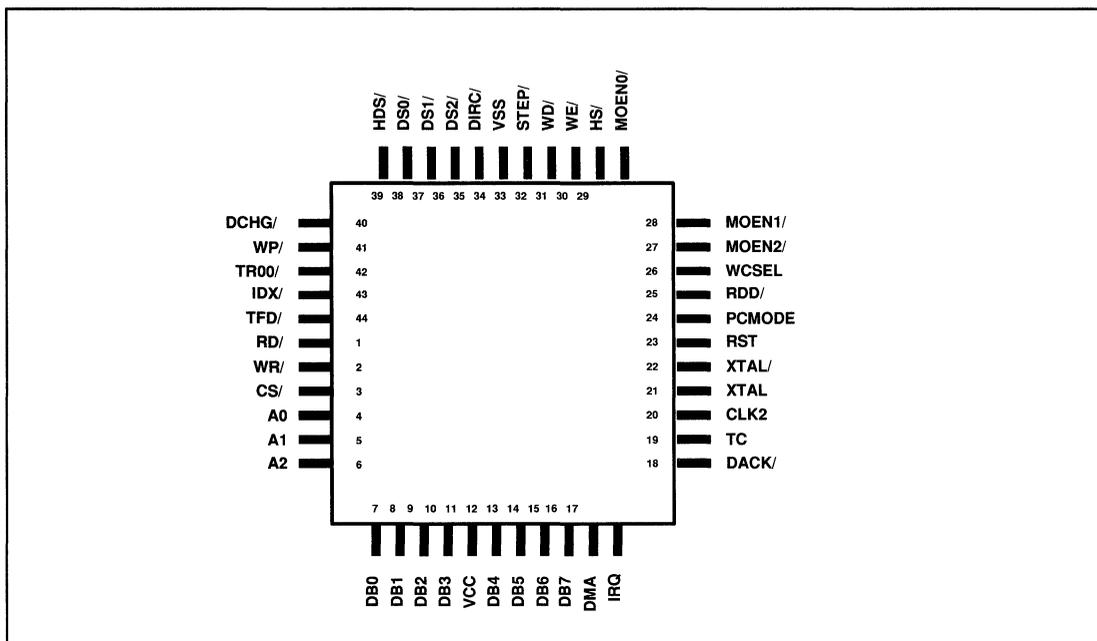
FIGURE 5. WD57C65 44-PIN PLCC
