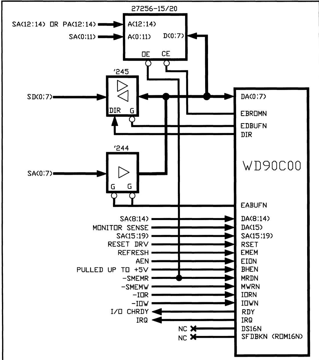
FIGURE 12. 8-BIT PC/AT INTERFACE WITH 8-BIT BIOS
