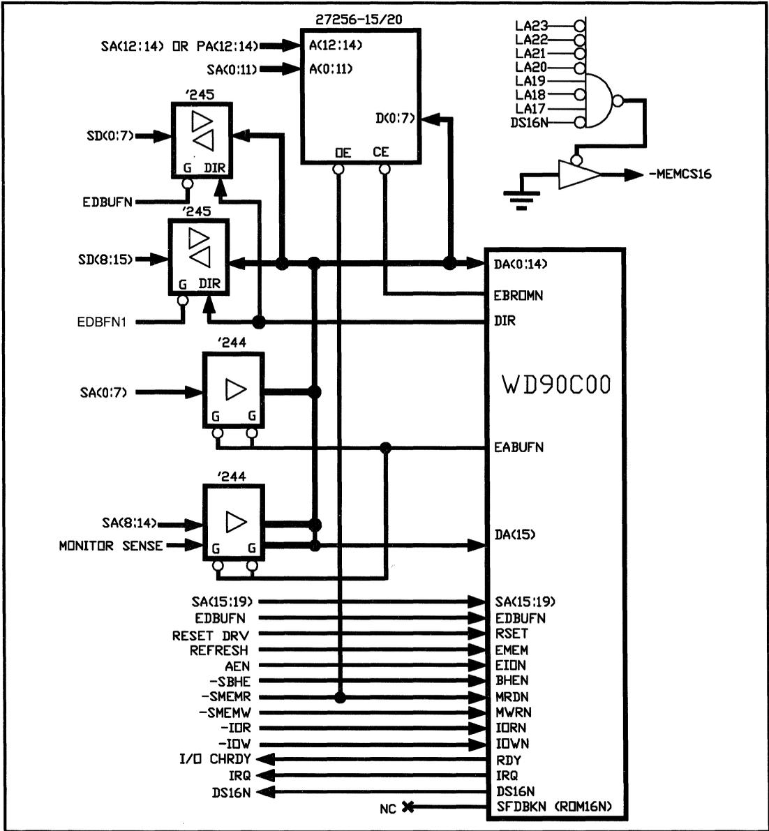
FIGURE 13. 16-BIT PC/AT INTERFACE WITH 8-BIT BIOS
