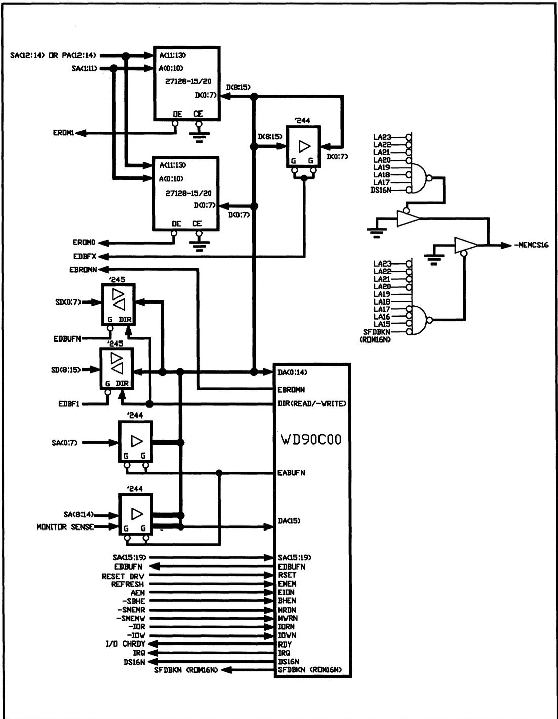
FIGURE 14. 16-BIT PC/AT INTERFACE WITH 16-BIT BIOS
