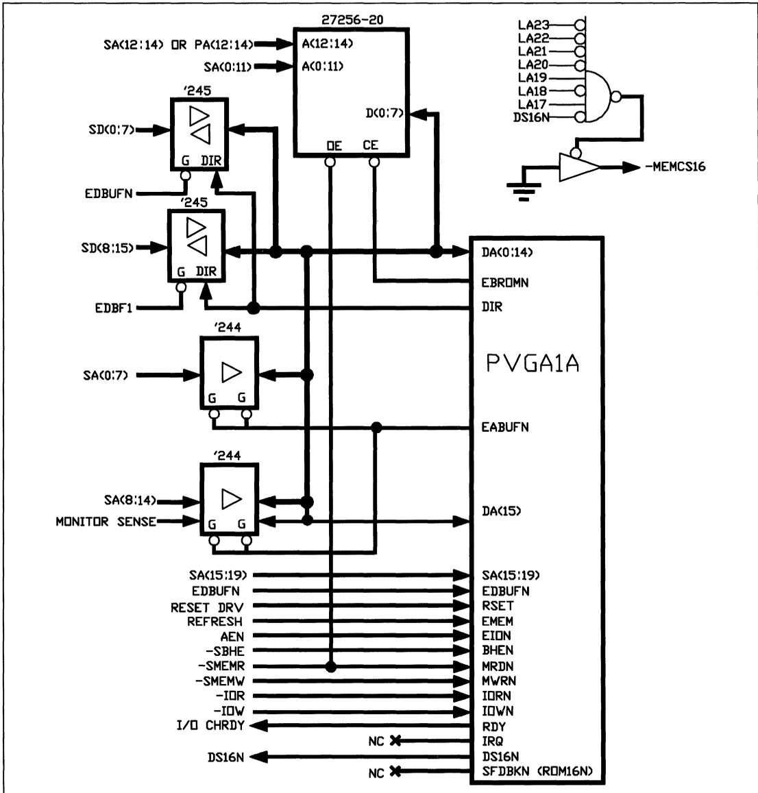
Figure 18. 16-Bit PC/AT Interface With 8-Bit BIOS
