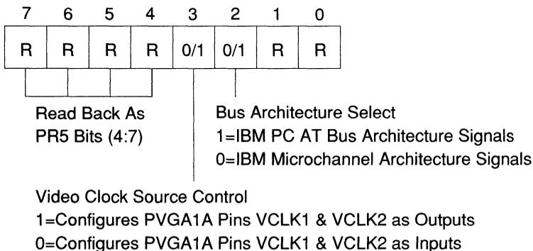
Bits CNF (2:3) are latched internally at power on reset from the corresponding memory data bus pins MD (2:3), connected to the external pullup or pulldown resistors. Pullup resistor sets MD(2:3) to logic 1. Note, that the configuration bits (2:3) are not readable since they are latched after power up. However, the configuration register bits (4:7) are readable after power up as PR5 bits (4:7). They appear as general purpose read only status bits in the PR5 register.
