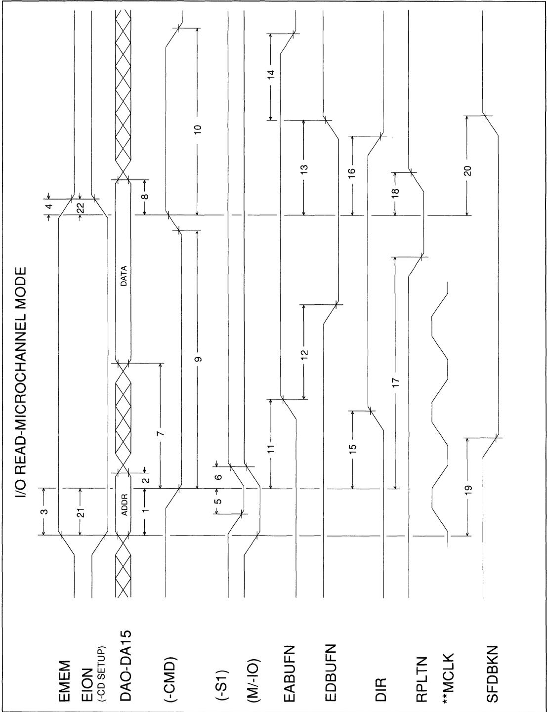
Figure 7. I/O Read - Micro Channel Mode
