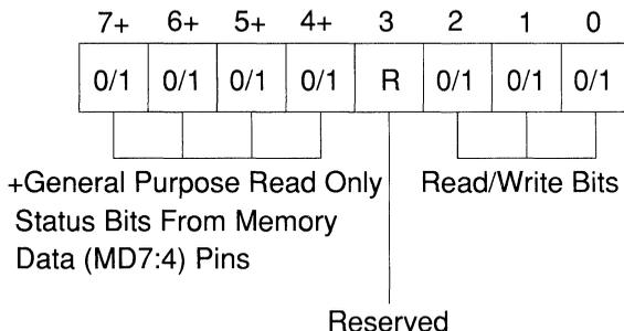
**NOTE:** += Pull Down Resistors Set These Bits To Logic 1
