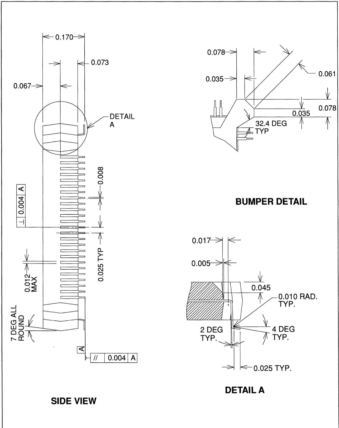
Figure 28. 100 Pin JEDEC Plastic Flat Package (PFP)
