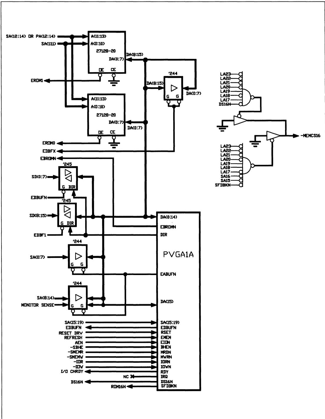
Figure 19. 16-Bit PC/AT Interface With 16-Bit BIOS
