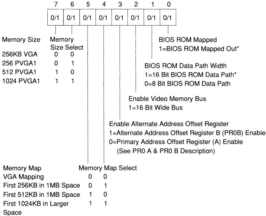
**NOTE:** \* = A Pull Up Resistor On MD(0) Or MD(1) Line Sets These Bits To 0 At Power On Reset
