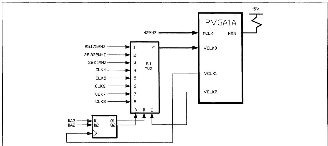
Figure 25. External Multiplexing of the Video Clocks
