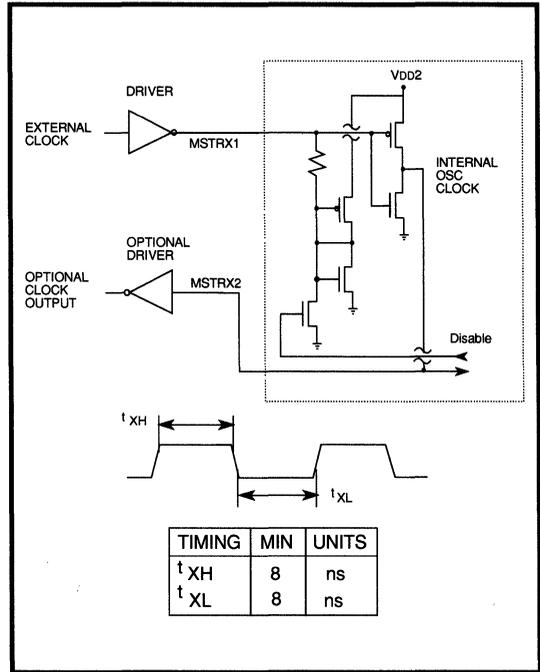
FIGURE 8-1. EXTERNAL CLOCK INPUT (48 MHz MAX.)
