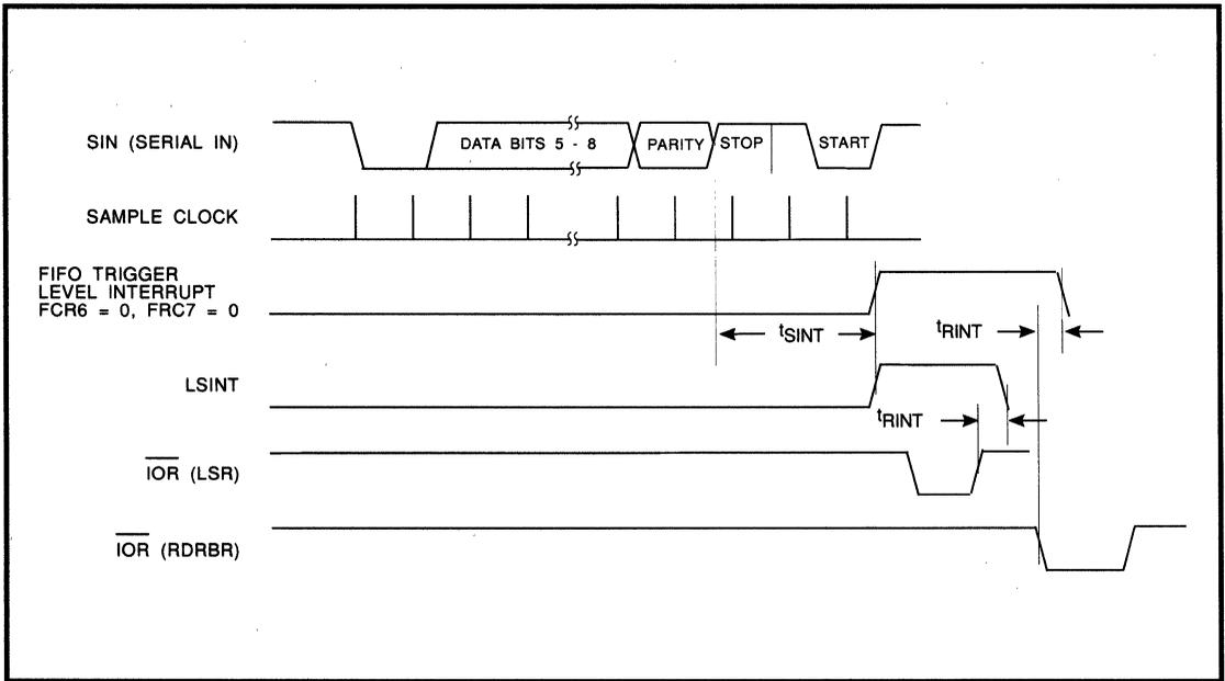
FIGURE 6-6. RCVR FIFO SIGNAL TIMING FOR FIRST BYTE
