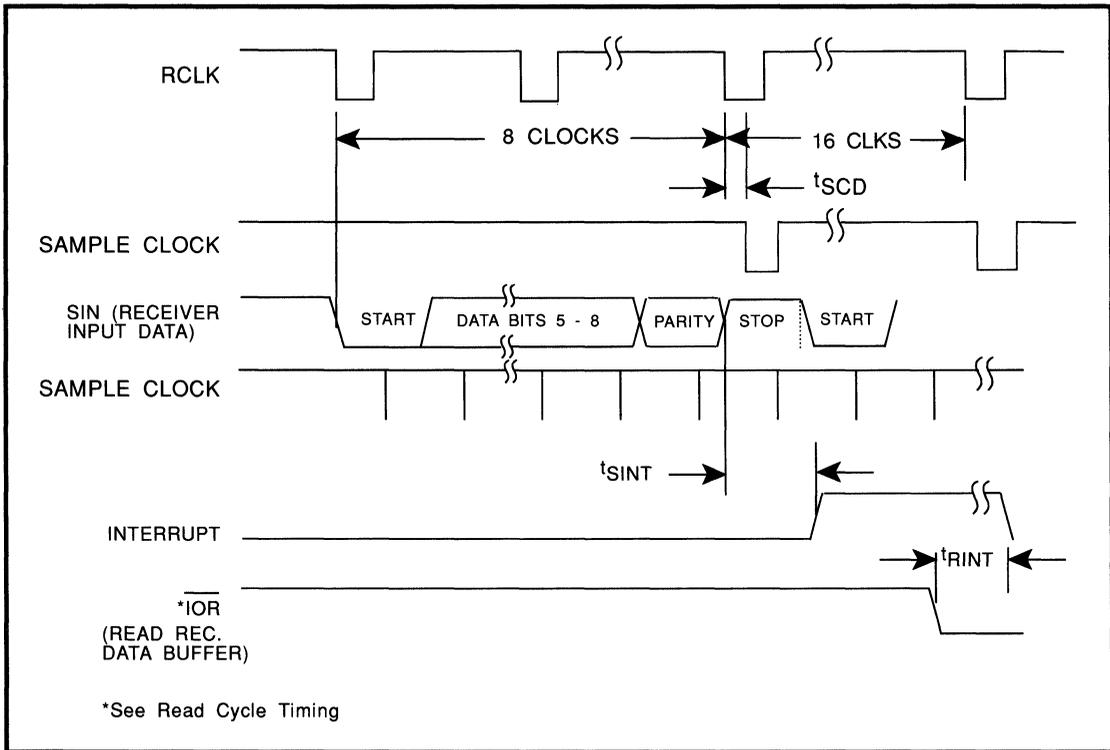
FIGURE 6-1. RECEIVER TIMING
