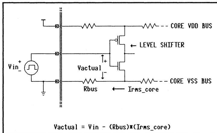
Additionally, enough power must be applied to handle the DC requirements of the output buffers and the average operating current of the array core.
