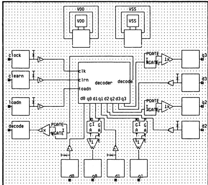
Three-state, bidirectional, open drain and open source pad control signals should be explicitly named (Figure 10). Refer to the VTIschematic manual for the syntax of legal signal names. Also, all three-state, bidirectional, open drain and open source output buffers must be driven by a pad driver. The output pad's NGATE and PGATE pins must be connected to a single driver cell's NGATE and PGATE pins respectively.
