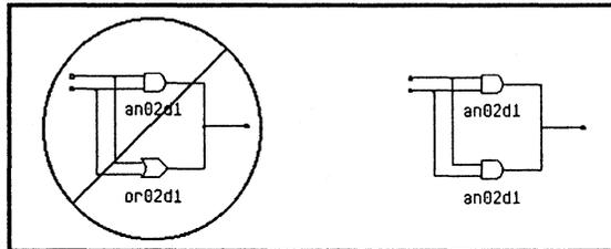
If a signal is driven by macros in parallel but whose input signals are not common, the VLSI netlist screener produces an error message unless the macros are three-state. This restriction prevents contention:
