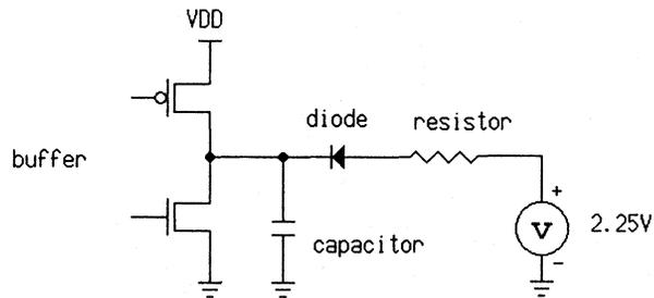
The resistor and voltage network causes the output buffers to sink or source the appropriate amount of current during AC performance simulations. For sourcing current, the diode in the above figure points the opposite direction.
