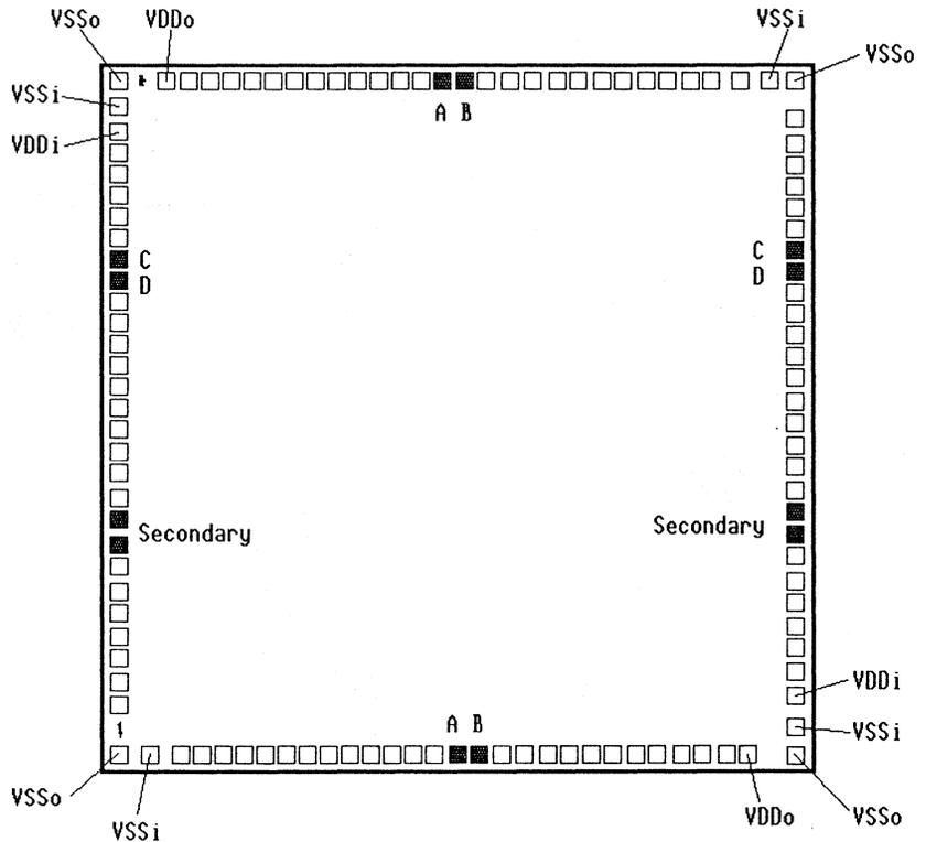
If you choose the recommended split power bus arrangement, place a PCVDD1 macro in the A position and a PCVSS1 macro in the B position. Use PCVDD2 and PCVSS2 on the vertical sides of the array, as shown, in locations C and D respectively. Additionally, for VGT100 arrays, place PCVDD1 and PCVDD2 macros in the two indicated corners of the array.
