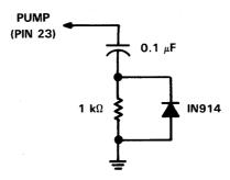
Since 5¼" drives operate at exactly one-half the data rate (250 Kb/sec) the above capacitor should be doubled to 0.2  $\mu$ F or 0.22  $\mu$ F.
