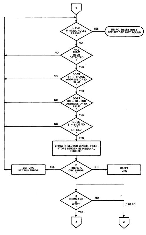
The Type II and III commands for the 2795-97 contain a side select flag (bit 1). When U = 0, SSO is updated to 0. Similarly, U = 1 updates SSO to 1. The chip compares the SSO to the ID field. If they do not compare within 5 revolutions, the interrupt line is made active and the RNF status bit is set.
