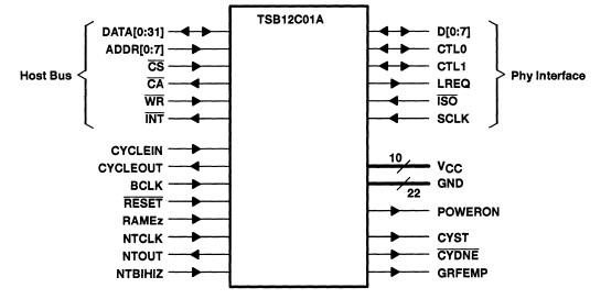
Figure 2–2. TSB12C01A Terminal Functions
