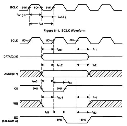
NOTE A: When back-to-back write cycles are done, a maximum of 9 BCLK cycles may be required after the falling edge of  $\overline{CS}$  before  $\overline{CA}$  is asserted (low). DATA[0:31], ADDR[0:7], and  $\overline{WR}$  need to remain valid until  $\overline{CA}$  is asserted (low).
