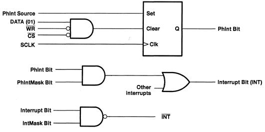
Figure 3–2. Interrupt Logic Diagram Example
