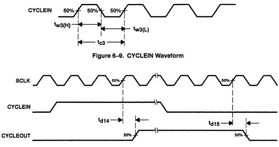
Figure 6–10. CYCLEIN and CYCLEOUT Waveforms
