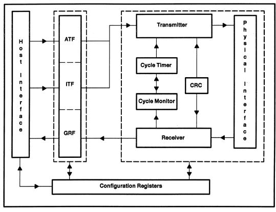
Figure 2–1. TSB12C01A Block Diagram
