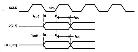
Figure 6-6. Phy-Layer-to-TSB12C01A Transfer Waveforms
