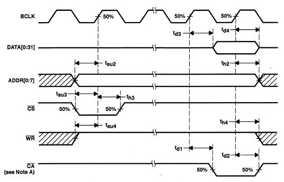
NOTE A: When back-to-back read cycles are done, a maximum of 9 BCLK cycles may be required after the falling edge of  $\overline{CS}$  and before  $\overline{CA}$  is asserted (low). ADDR[0:7] and  $\overline{WR}$  need to remain valid until  $\overline{CA}$  is asserted (low).
