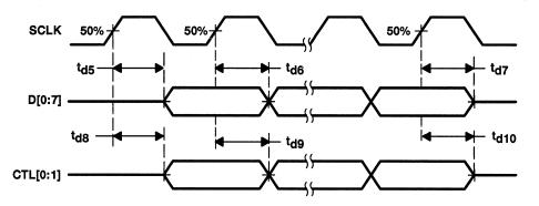
Figure 6–5. TSB12C01A-to-Phy-Layer Transfer Waveforms
