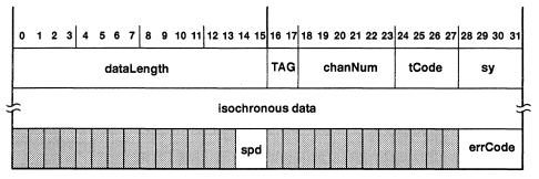
Figure 4-6. Isochronous-Receive Format
