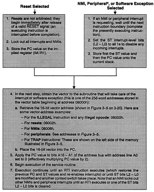
\*Peripheral interrupts must be a level *higher* than the level in the ST interrupt-level bits (L2 - L0) in order to execute. Thus, a level of  $111_2$  locks out any peripheral interrupt.
