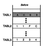
Move (copy) the entire contents (word value) at address TABL1 to address TABL2. Leave the source-address contents unchanged. Consider TABL1 and TABL2 to be on *even address boundaries* in order to work correctly with a move-word instruction.
