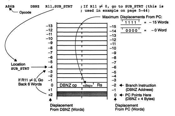
thus, the displacement can redirect execution +2 words (a 0000<sub>2</sub> displacement) or -13 words (1111<sub>2</sub>) from the 17-bit address of the DBNZ instruction (see Figure 5–5). *In any case, the branch must be negative* — *to a previous address (lower memory address)*.
