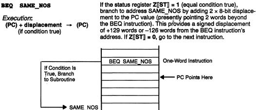
For Bcond, BRBIT0, and BRBIT1, a signed 8-bit value is added to the PC as address lines A8–A1 to redirect execution flow from the executing instruction's 17-bit *physical memory address*. For the DBNZ instruction, a *fourbit unsigned* value in bits 7–4 of the instruction word is *subtracted* from the PC's corresponding value for address lines A4–A1. The following table shows the displacement from the *physical address* of the PC.
