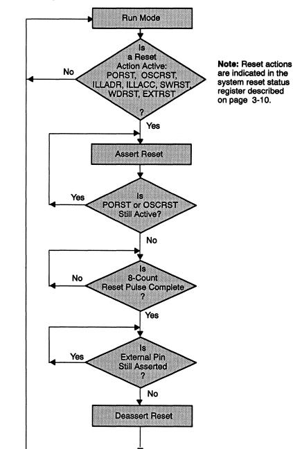
Figure 3–2. Reset State Diagram — Normal Run Mode
