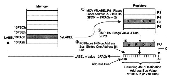
This method can also be used to set up the indirection register for the FMOV instruction. The bits in the indirection register (either the source or destination) are a word address to be applied to address bits A16—A1.
