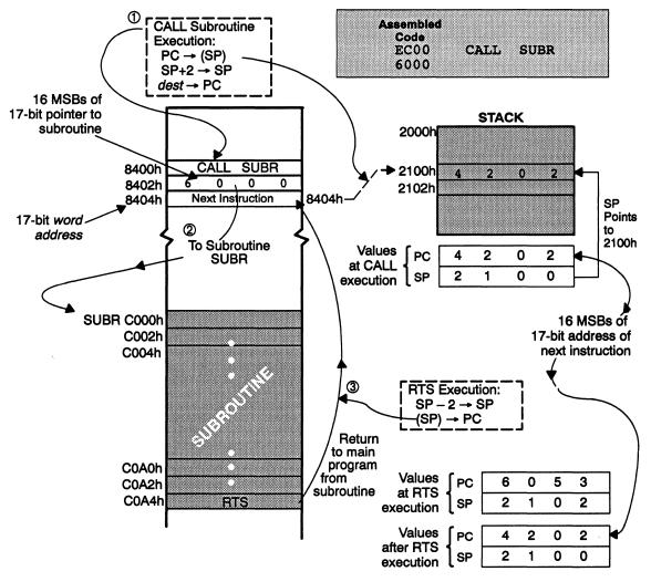
Figure 2-6. Example of Stack Use to and From a Subroutine
