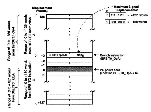
Figure 5-3. BRBIT0 and BRBIT1 Instruction Displacements
