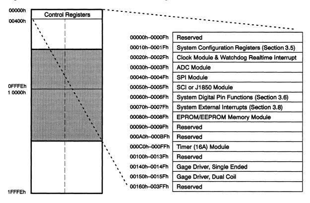
Figure 2–11. Location and Names of Control Registers
