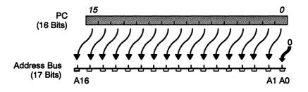
Because of a pipeline architecture, the PC typically points to a memory address *two words beyond the currently executing instruction or to its extension word.* This relationship is graphically shown in Figure 2–4.
