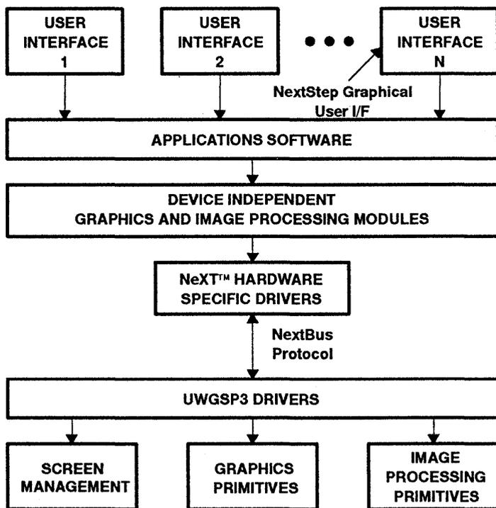
Figure 2. UWGSP3 Software Architecture
