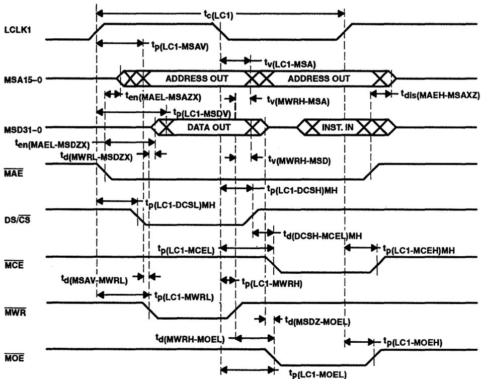
NOTE: This example shows a data write followed by an instruction read. Timing for multiple code writes would be similar. This option for using DS/CS as data space chip enable and MCE as code space chip enable is invoked by setting the MEMCFG bit high in the configuration register. When MEMCFG is high, DS/CS and MCE rise after every clock edge. In this mode, DS/CS and MCE may not both be active (low) at the same time.
