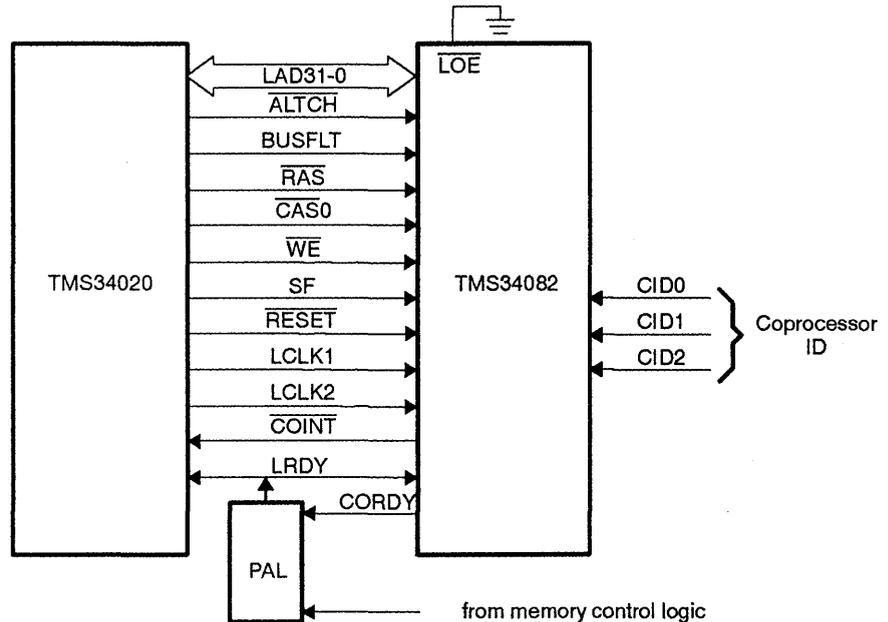
CORDY from the TMS34082 is logically ORed with other ready signals from the system to form the TMS34020 LRDY input ready signal. Note that LRDY connects to both the TMS34020 and the TMS34082 inputs.
