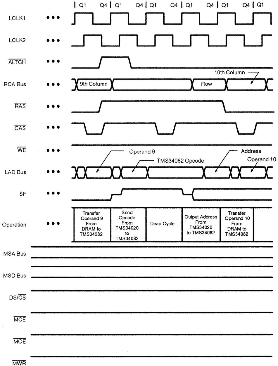
Figure 5-15. 3 × 3 Matrix Multiply Using External SRAM for Data Space and Code Space (Mode 3) (Continued)
