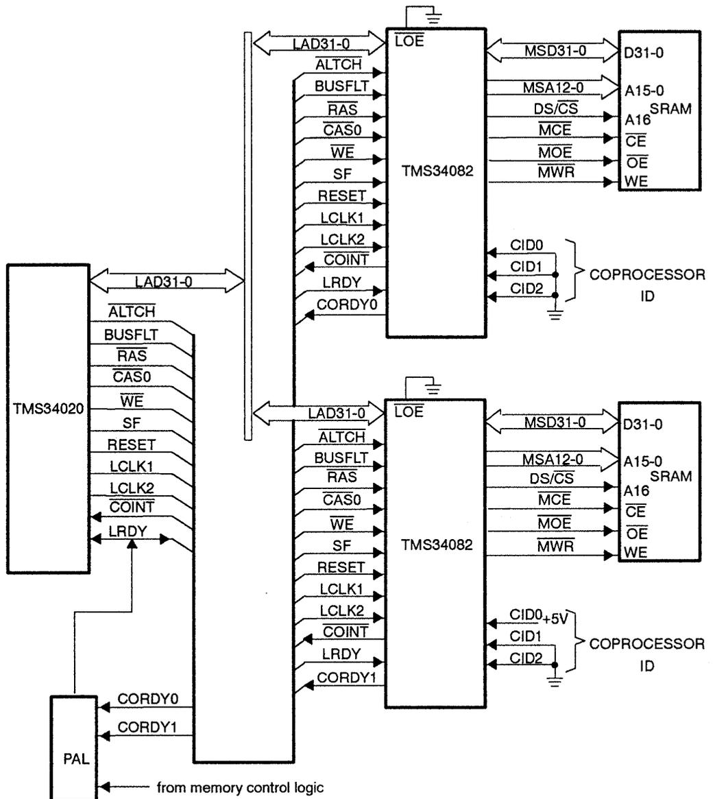
When  $CID2-0 = 100_2$ , the TMS34020 broadcasts the instruction to all coprocessors. Broadcast reads by the TMS34082s are not permitted and are ignored.
