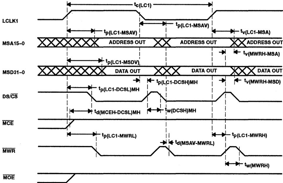
NOTE: This example shows multiple data writes. Timing for multiple code writes would be similar. This option for using DS/CS as data space chip enable and MCE as code space chip enable is invoked by setting the MEMCFG bit high in the configuration register. When MEMCFG is high, DS/CS and MCE rise after every clock edge. In this mode, DS/CS and MCE may not both be active (low) at the same time.
