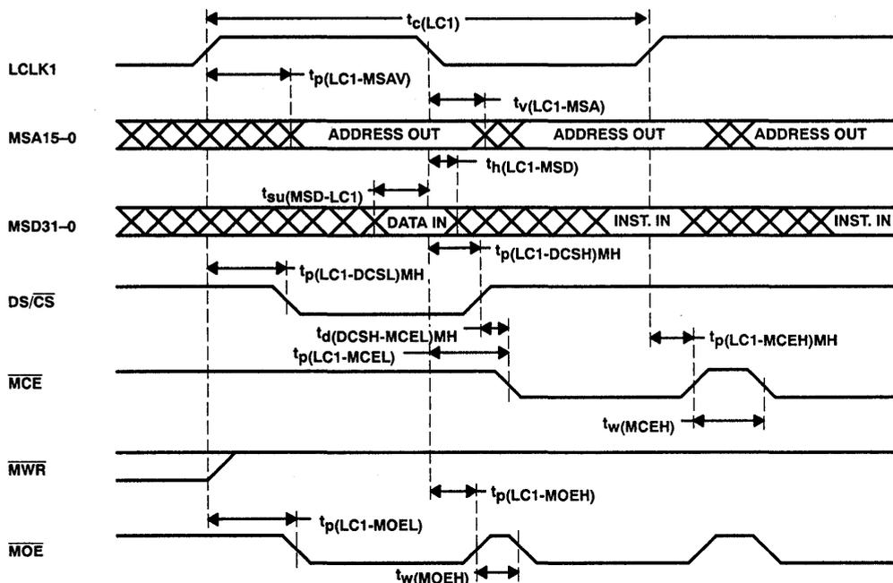
NOTE: This example shows a data read followed by an instruction read followed by an instruction read. This option for using DS/CS as data space chip enable and MCE as code space chip enable is invoked by setting the MEMCFG bit high in the configuration register. When MEMCFG is high, DS/CS and MCE rise after every clock edge. In this mode, DS/CS and MCE may not both be active (low) at the same time.
