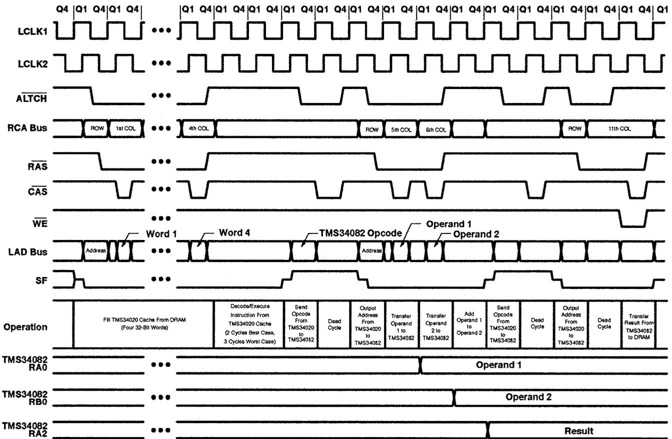
Note: Assume instructions are not in TMS34020 cache, TMS34082 pipeline registers turned on (PIPES1=0) and output registers turned off (PIPES2=1) DRAM page mode accesses.
