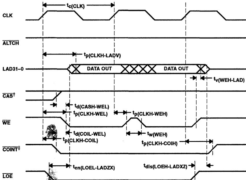
† When the LADCFG bit is high,  $\overline{LOE}$  high places  $\overline{CAS}$  and  $\overline{WE}$  (as well as the LAD bus) in high impedance.
