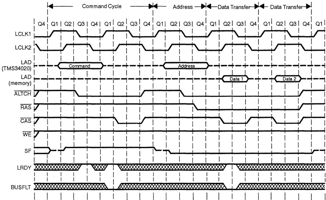
When the TMS34082 is transferring data to memory, the TMS34020 outputs the memory address on the LAD bus. An extra clock cycle, called a spacer, is then inserted before the TMS34082 outputs data. The spacer is added to allow time for the TMS34020 to stop driving the LAD bus and the TMS34082 to set up valid data on LAD.
