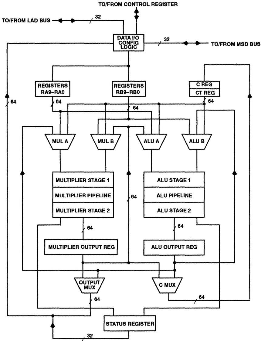
Figure 8. FPU Core Functional Block Diagram
