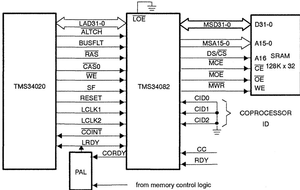
CC is a condition code input and may be used as an external input for branch conditions in external code. It is not used in internal instructions.
