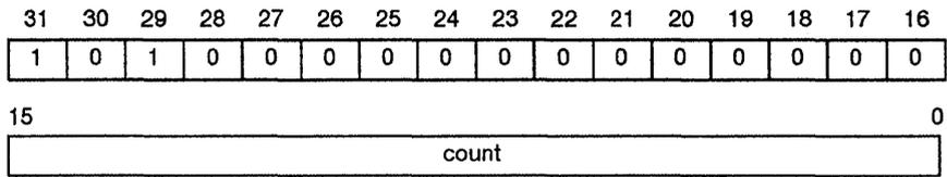
**Description** This instruction loads the LOOPCT register with the value specified by count. If the register is loaded with 0, the loop would execute 64K times.
