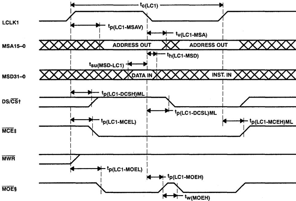
† The setting of DS/CS determines whether the value on the MSD bus is an instruction or data.
