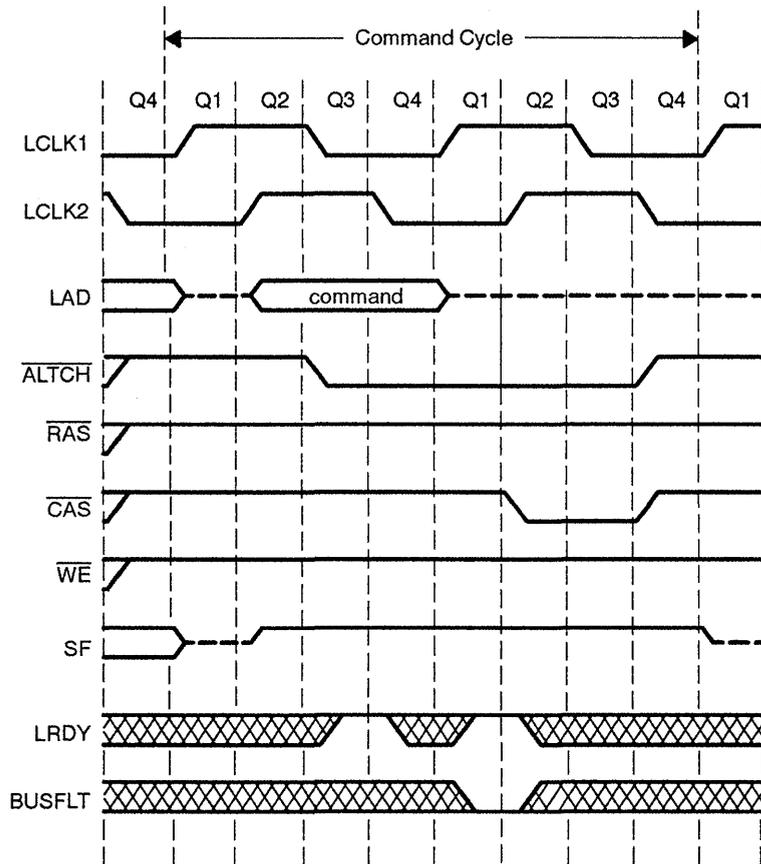
If operands are required from DRAM/VRAM, the TMS34020 sets up the appropriate DRAM/VRAM address and timing. The data is then transferred directly between the TMS34082 and DRAM/VRAM.
