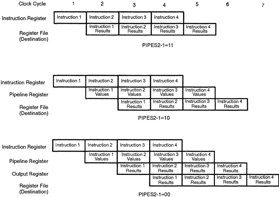
Both sets of pipeline registers are controlled by the PIPES2 and PIPES1 bits in the configuration register. When the device is powered up or reset, the intermediate pipeline registers are enabled (PIPES1=0) and the output registers are transparent (PIPES2=1). For internal instructions, control logic sets the pipeline registers as needed and restores them to their previous configuration after the instruction is completed.
