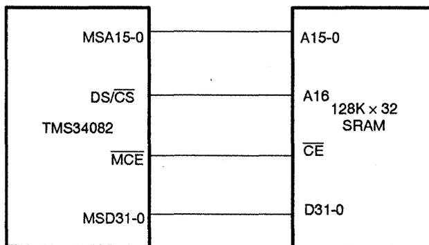
When MEMCFG is high,  $\overline{MCE}$  becomes the code space chip enable and  $DS/\overline{CS}$  the data space chip enable. Both are active low. This may eliminate the need for an external inverter on  $DS/\overline{CS}$ . Figure 4-8 show this configuration.
