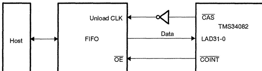
The TMS34082 only drives the LAD bus during instructions that output an address or data. The LAD bus drivers are disabled at any other time.
