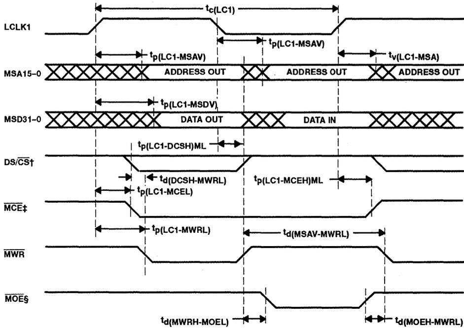
† The setting of DS/CS determines whether the value on the MSD bus is an instruction or data.
