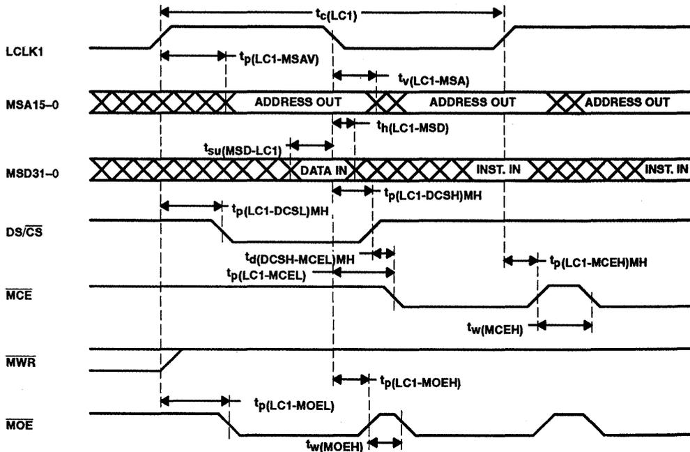
NOTE: This example shows a data read followed by an instruction read followed by an instruction read. This option for using DS/CS as data space chip enable and MCE as code space chip enable is invoked by setting the MEMCFG bit high in the configuration register. When MEMCFG is high, DS/CS and MCE rise after every clock edge. In this mode, DS/CS and MCE may not both be active (low) at the same time.
