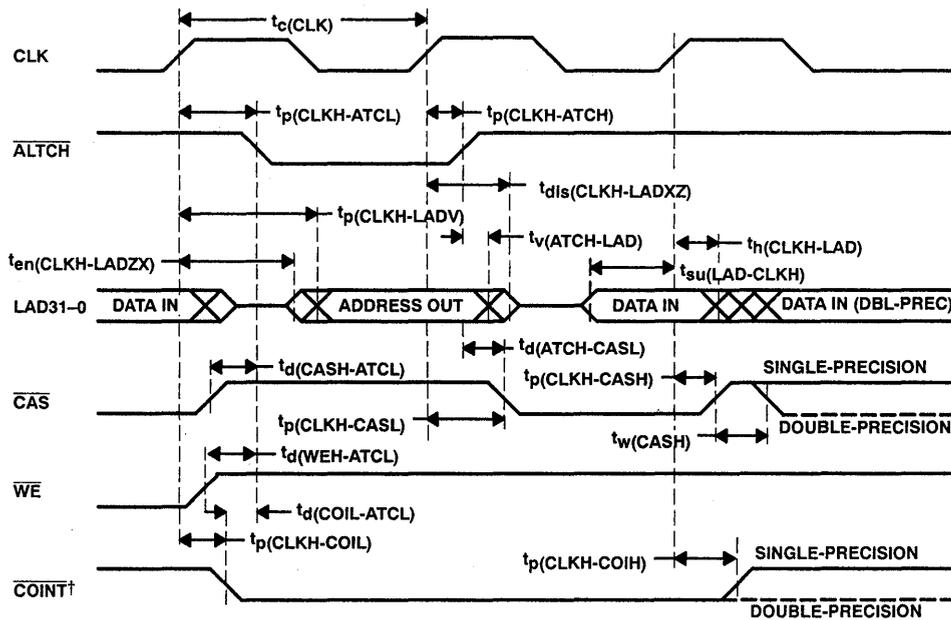
†  $\overline{\text{COINT}}$  timing is for LADCFG high only. When the LADCFG bit is set high in the configuratin register,  $\overline{\text{COINT}}$  is controlled by bit 1 of the LAD move instruction instead of the set mask instruction.
