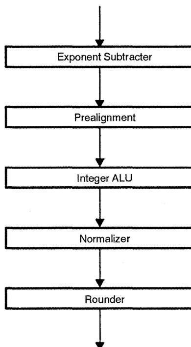
Integer processing in the ALU includes both arithmetic and logical operations in either 2s complement numbers or unsigned integers. The ALU performs addition, subtraction, comparison, logical shifts, logical AND, logical OR, and logical XOR. Format conversions and wrapping/unwrapping of denormals are also done by the ALU.
