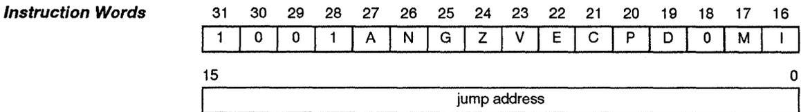
**Description** Jump conditional to the specified subroutine address. During a jump instruction, no FPU operations are performed.
