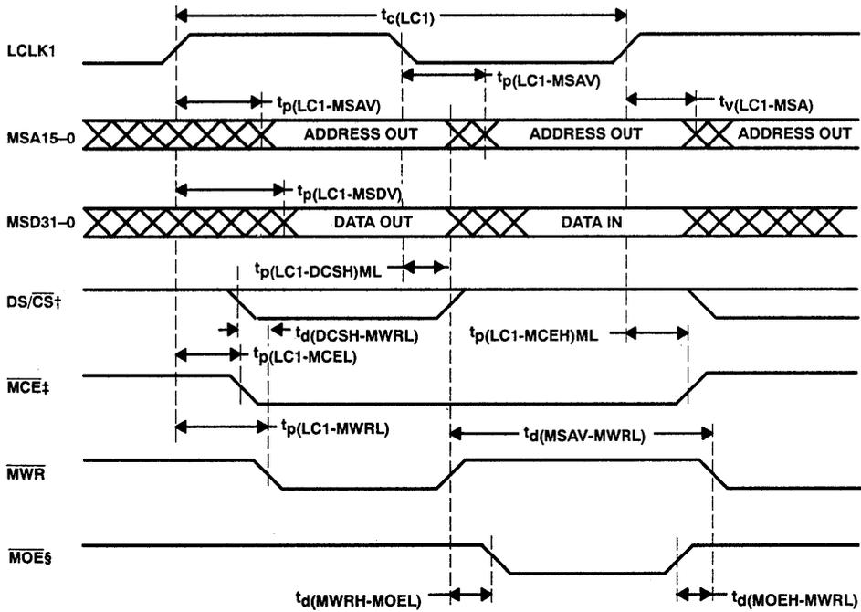
† The setting of DS/ $\overline{CS}$  determines whether the value on the MSD bus is an instruction or data.
