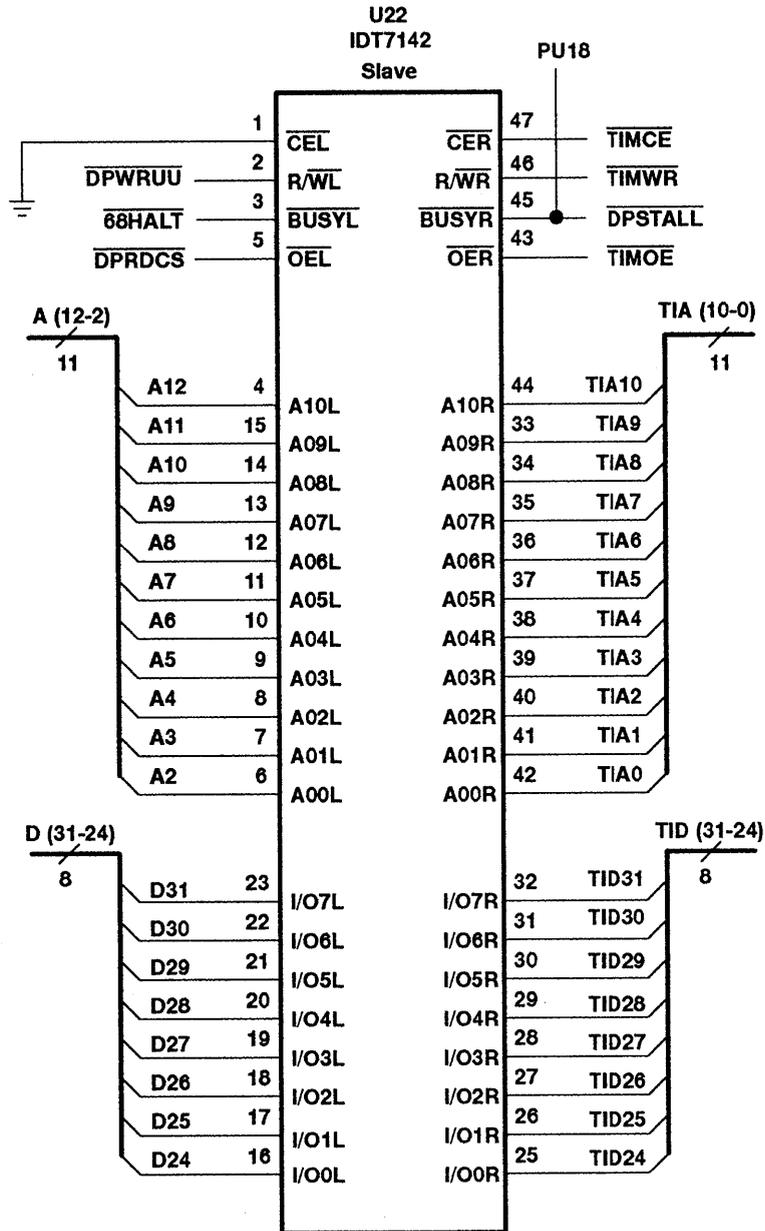
Figure 24. FIFO Logic DP-SRAM, Details of U22
