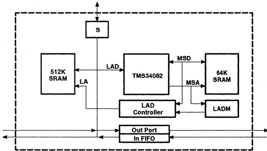
Figure 3. PE Architecture
