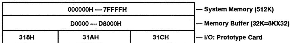
Figure 6. PC/AT Interface: I/O and Memory Addressing
