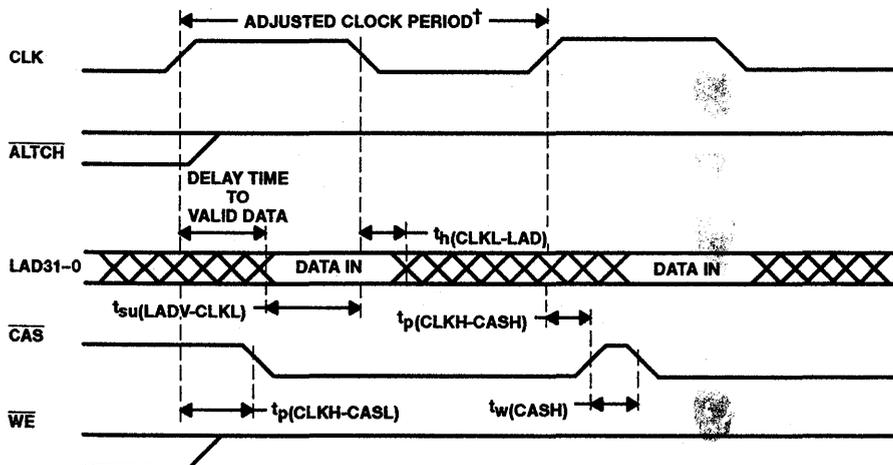
† This mode permits data input which does not meet the minimum setup before CLK high. For immediate data input, CLK must be high for more than 20 ns. This input mode cannot be used to input data for divides and square roots.
