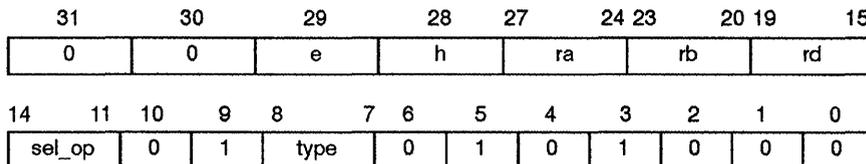
**Description** This instruction shifts the value in ra to the left by the number of bit positions indicated in rb. Zeros are shifted into the least significant bit location.
