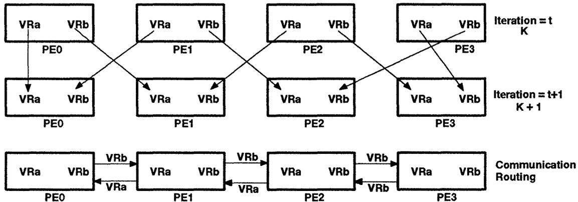
Figure 5. Parallel Jacobi Updating on a Systolic Architecture
