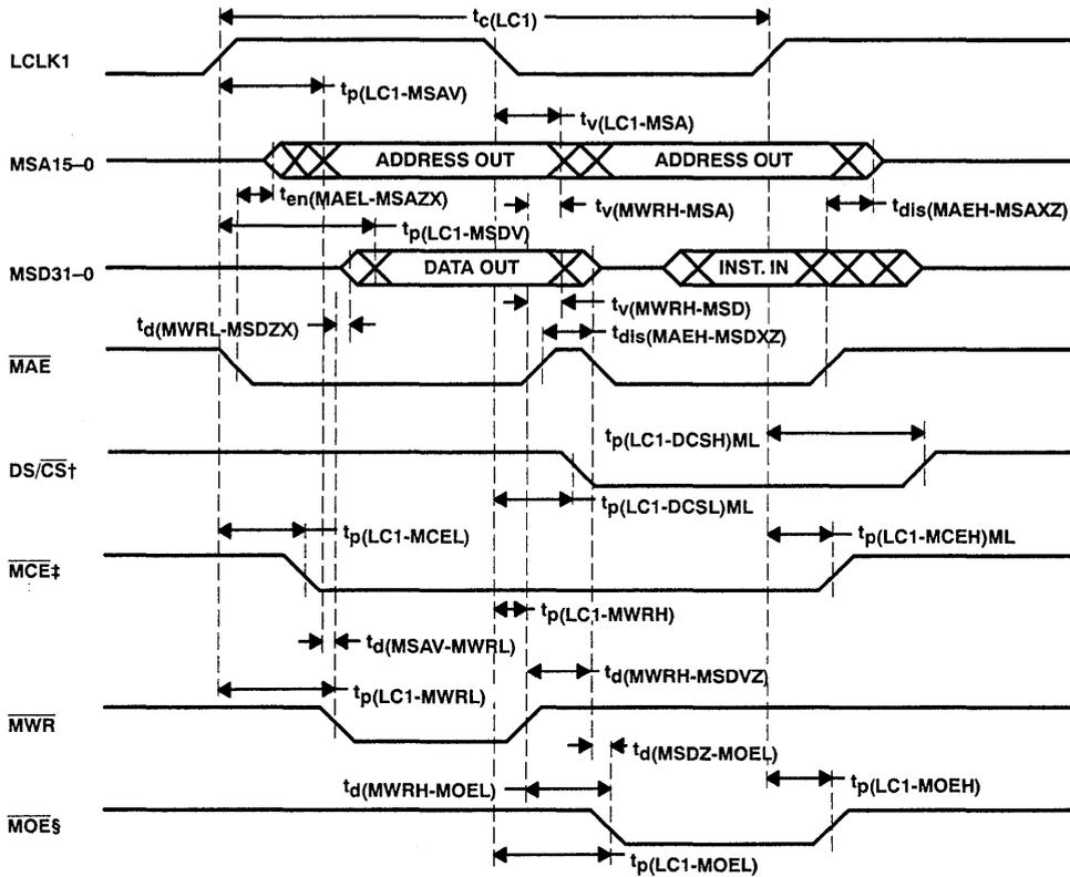
† The setting of DS/CS determines whether the value on the MSD bus is an instruction or data.
