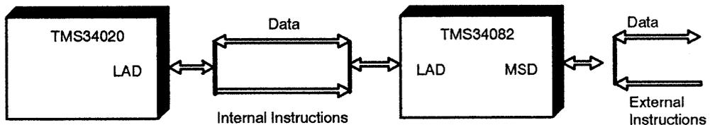
In host-independent mode, the TMS34082 is controlled by external instructions input on the MSD bus.
