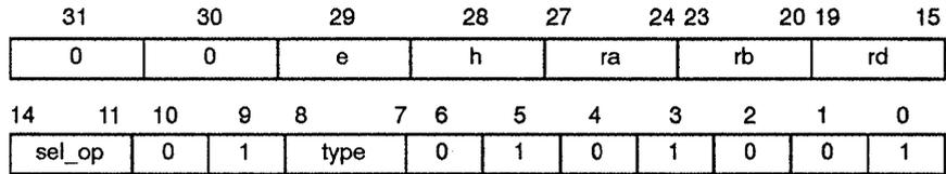
**Description** This instruction shifts the value in ra to the right by the number of bit positions indicated in rb. Zeros are shifted into the most significant bit location.
