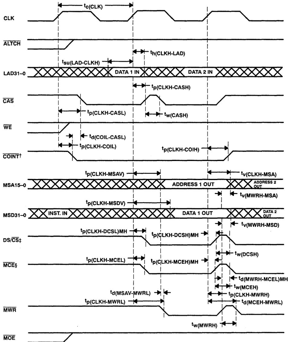
†  $\overline{\text{COINT}}$  timing is for LADCFG high only. When the LADCFG bit is set high in the configuration register,  $\overline{\text{COINT}}$  is controlled by bit 1 of the LAD move instruction instead of the set mask instruction.
