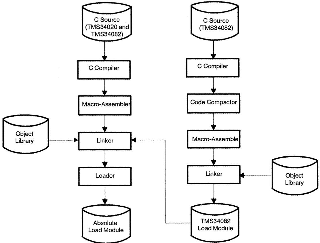
TMS340 Family Software Code Generation Tools (used for generating TMS34020 code and TMS34082 internal instructions)
