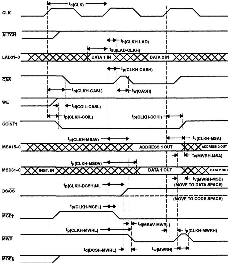
† COINT timing is for LADCFG high only. When the LADCFG bit is set high in the configuration register,  $\overline{\text{COINT}}$  is controlled by bit 1 of the LAD move instruction instead of the set mask instruction.
