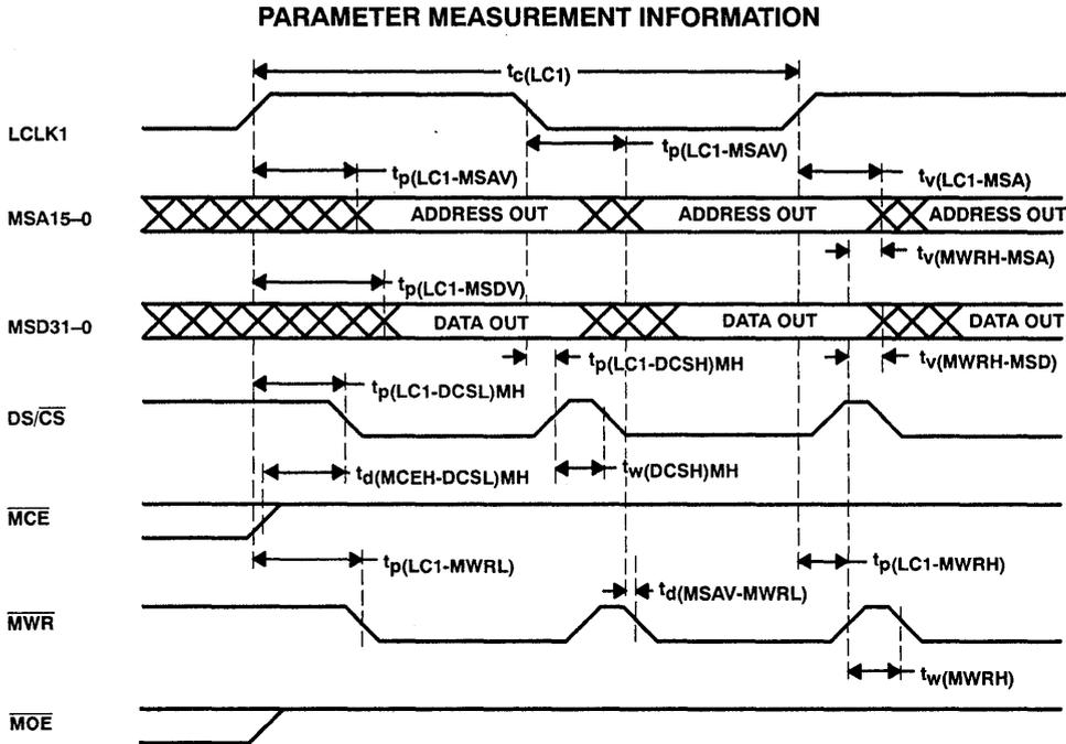
NOTE: This example shows multiple data writes. Timing for multiple code writes would be similar. This option for using DS/CS as data space chip enable and MCE as code space chip enable is invoked by setting the MEMCFG bit high in the configuration register. When MEMCFG is high, DS/CS and MCE rise after every clock edge. In this mode, DS/CS and MCE may not both be active (low) at the same time.
