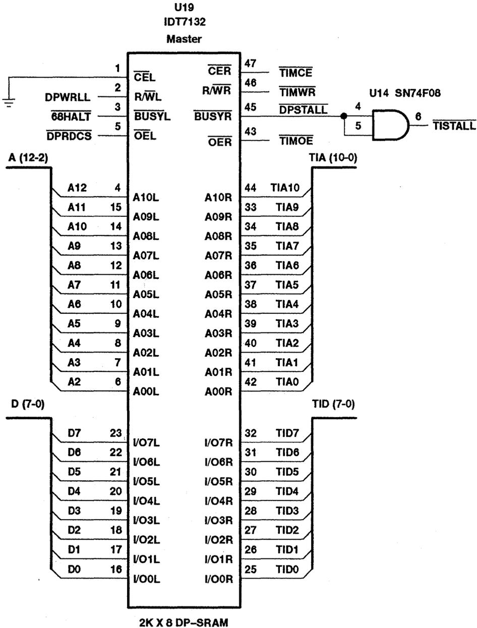
**Figure 20. 8K x 8 SRAM DP-SRAM, Details of U14 and U19**
