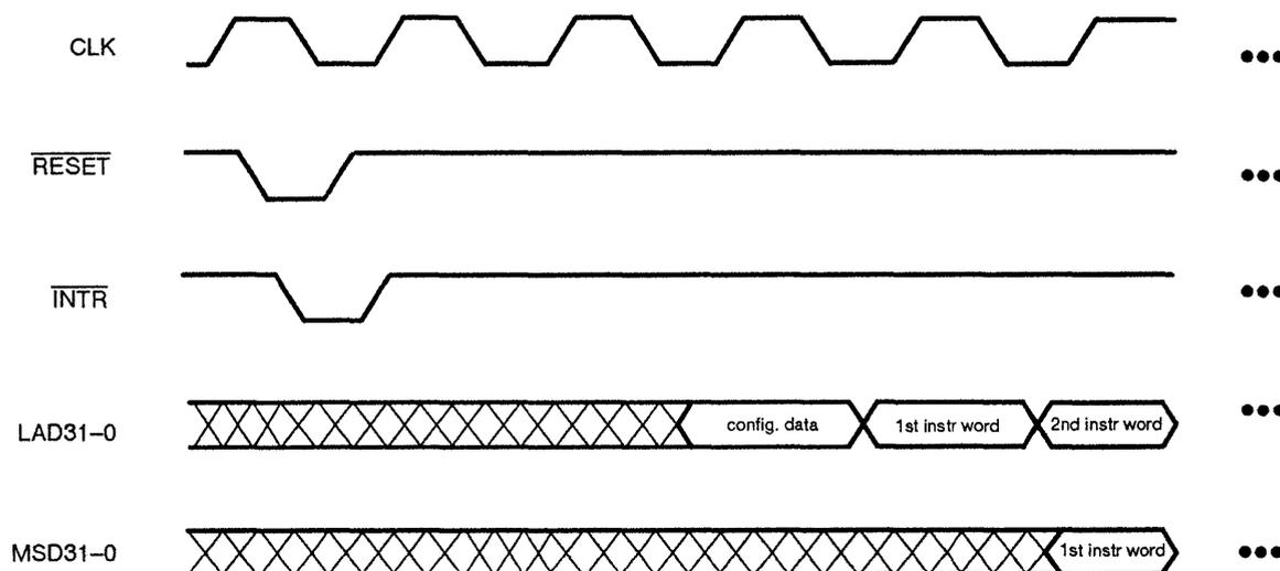
Loader operation begins on the second clock cycle after  $\overline{\text{RESET}}$  and  $\overline{\text{INTR}}$  return high. The first word is read into the configuration register on the rising edge of the third clock. Each successive rising edge loads an instruction word. The instruction word is output on the MSD bus one clock cycle after it is input on the LAD bus.
