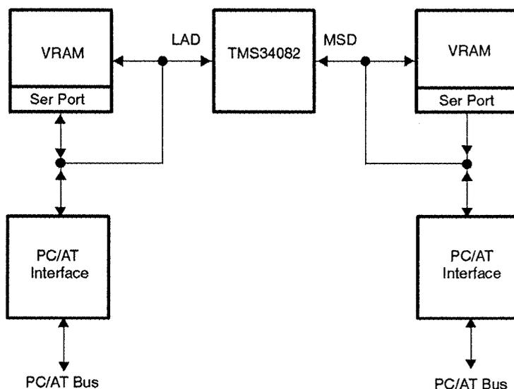
Built on a PC/AT card occupying a single slot, the TMS34082 Demonstration Board features:
