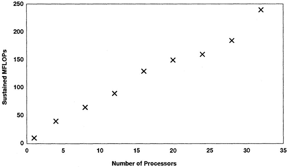
Figure 7. 128 x 128 Matrix Multiplication on P-Processor Systems
