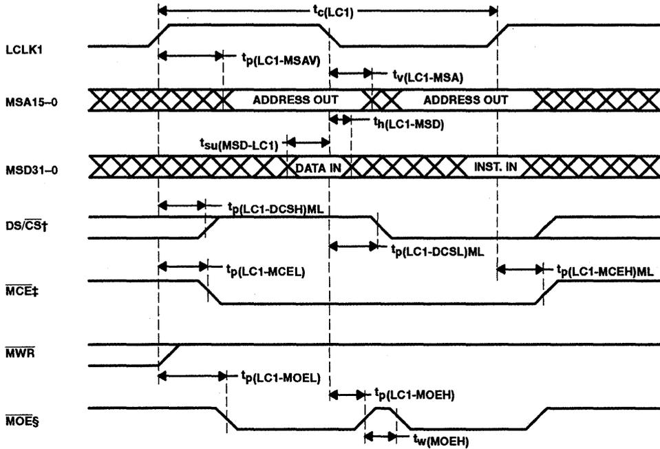
† The setting of  $DS/\overline{CS}$  determines whether the value on the MSD bus is an instruction or data.
