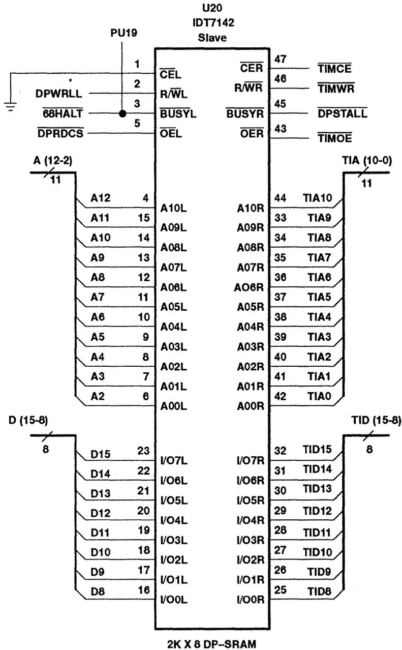
Figure 22. 8K x 8 SRAM DP-SRAM, Details of U20
