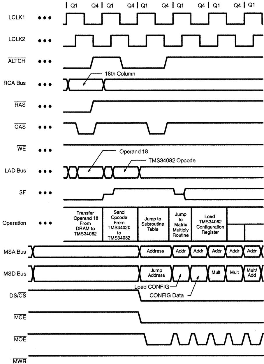
Figure 5-15 3x3 Matrix Multiply Using External SRAM for Data Space and Code Space (Mode 3) (Continued)
