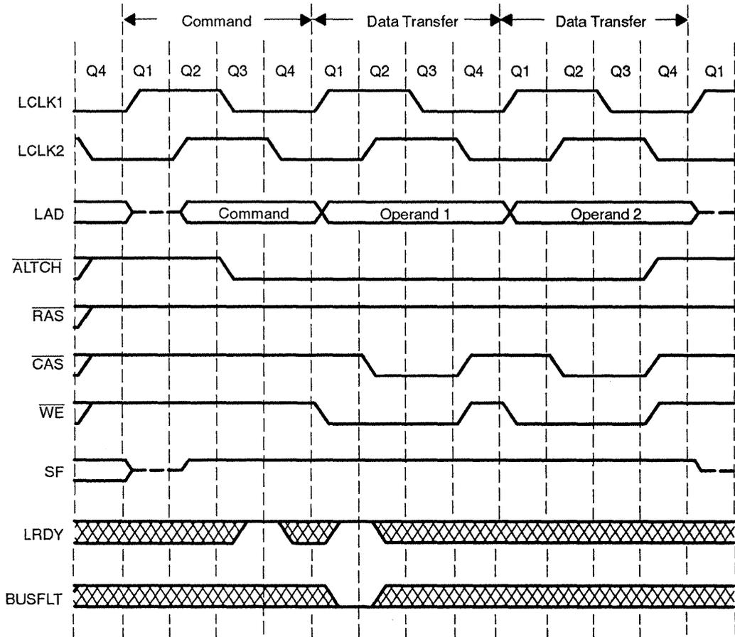
Figure 5-5. Transferring from the TMS34082 to a TMS34020 Register
