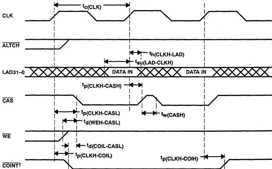
†  $\overline{\text{COINT}}$  timing is for LADCFG high only. When the LADCFG bit is set high in the configuration register,  $\overline{\text{COINT}}$  is controlled by bit 1 of the LAD move instruction instead of the set mask instruction.
