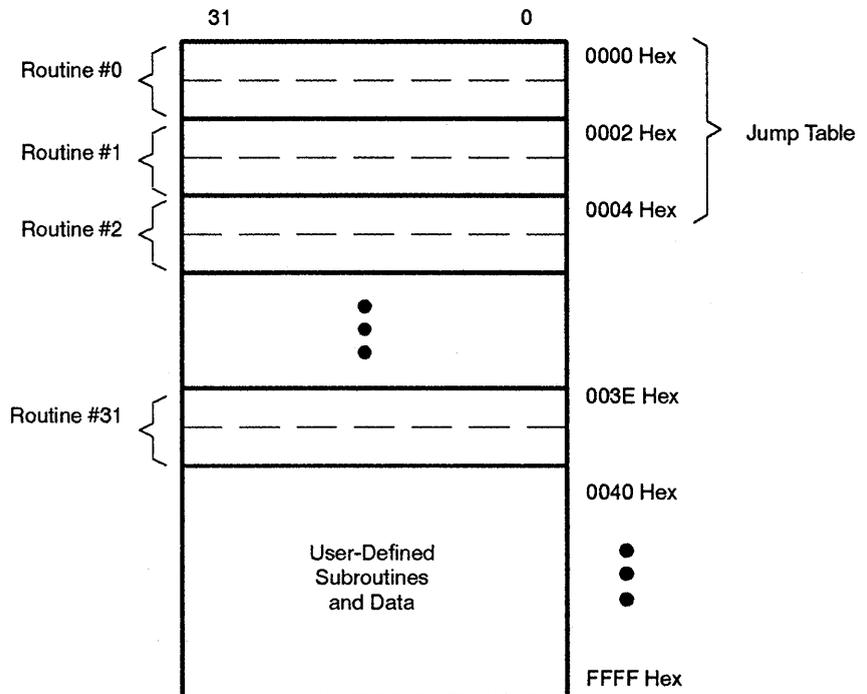
Figure 5–14 illustrates how an external subroutine would execute. The final instruction in the subroutine should be a return from subroutine (RTS). This puts the TMS34082 in an idle mode, waiting for the next instruction from the TMS34020.
