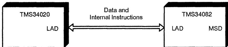
In the host-independent mode, an internal instruction can be executed by jumping to the proper internal ROM address. Chapter 8 of this manual shows the correct syntax for the JSR (jump to subroutine) and CJSR (conditional jump to subroutine) instructions.
