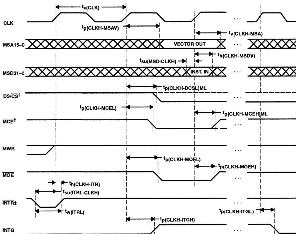
† Dotted lines show  $\overline{\text{DS}}/\overline{\text{CS}}$  and  $\overline{\text{MCE}}$  for MEMCFG high.
