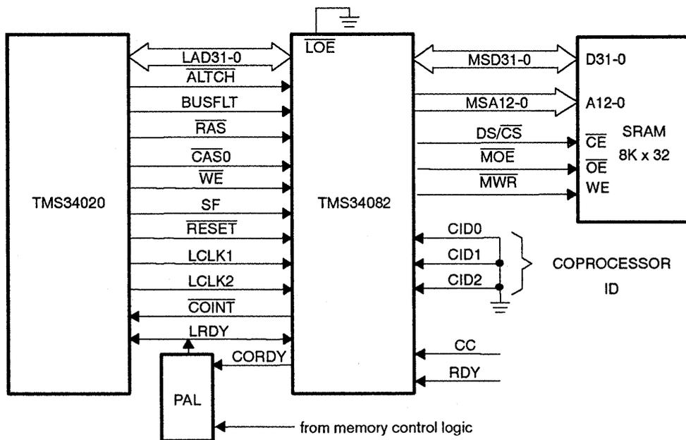
The maximum amount of external memory directly addressable by the TMS34082 is 64K words of program code and 64K words of data as shown in Figure 5-13. This comes out to 512K bytes total. When additional memory is necessary, segmentation or paging techniques can be utilized.
