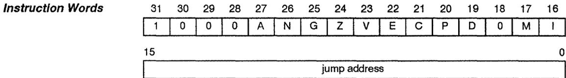
**Description** Jump conditional to the specified branch address. During a jump instruction, no FPU operations are performed.
