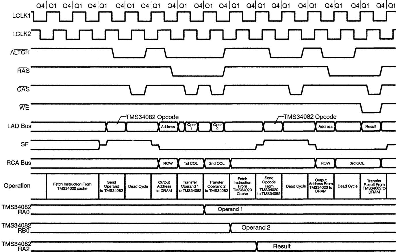
Note: Assume instructions are in TMS34020 cache, TMS34082 pipeline registers turned on (PIPES1=0) and output registers turned off (PIPES2=1), DRAM page mode accesses.
