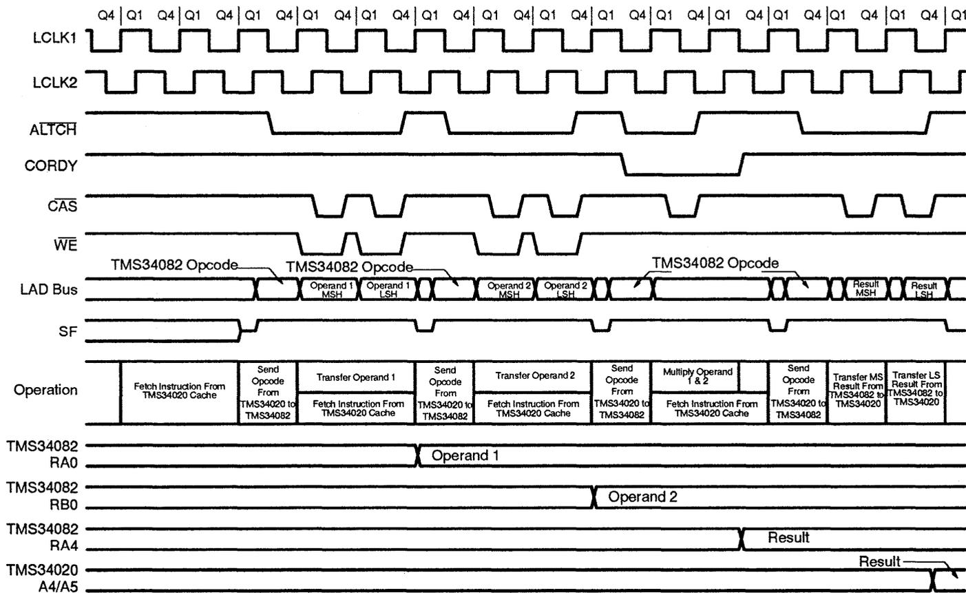
Note: Assume instructions are in TMS34020 cache, TMS34082 pipeline registers turned on (PIPES1=0) and output registers turned off (PIPES2=1), TMS34082 load order is MSH, then LSH.
