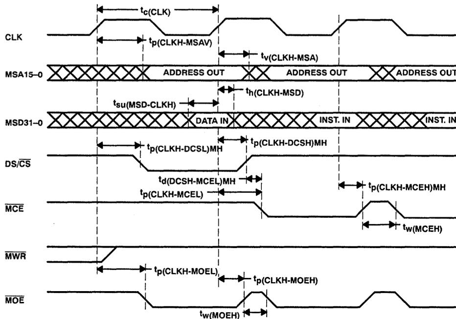
NOTE: This example shows a data read followed by an instruction read followed by an instruction read. This option for using  $\overline{DS/CS}$  as data space chip enable and  $\overline{MCE}$  as code space chip enable is invoked by setting the MEMCFG bit high in the configuration register. When MEMCFG is high,  $\overline{DS/CS}$  and  $\overline{MCE}$  rise after every rising clock edge. In this mode,  $\overline{DS/CS}$  and  $\overline{MCE}$  may not both be active (low) at the same time.
