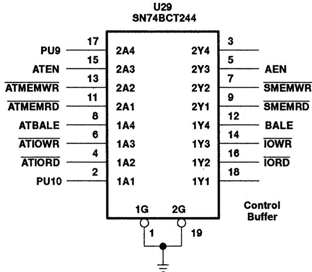
**Figure 10. PC/AT I/F and Control, Details of U29**
