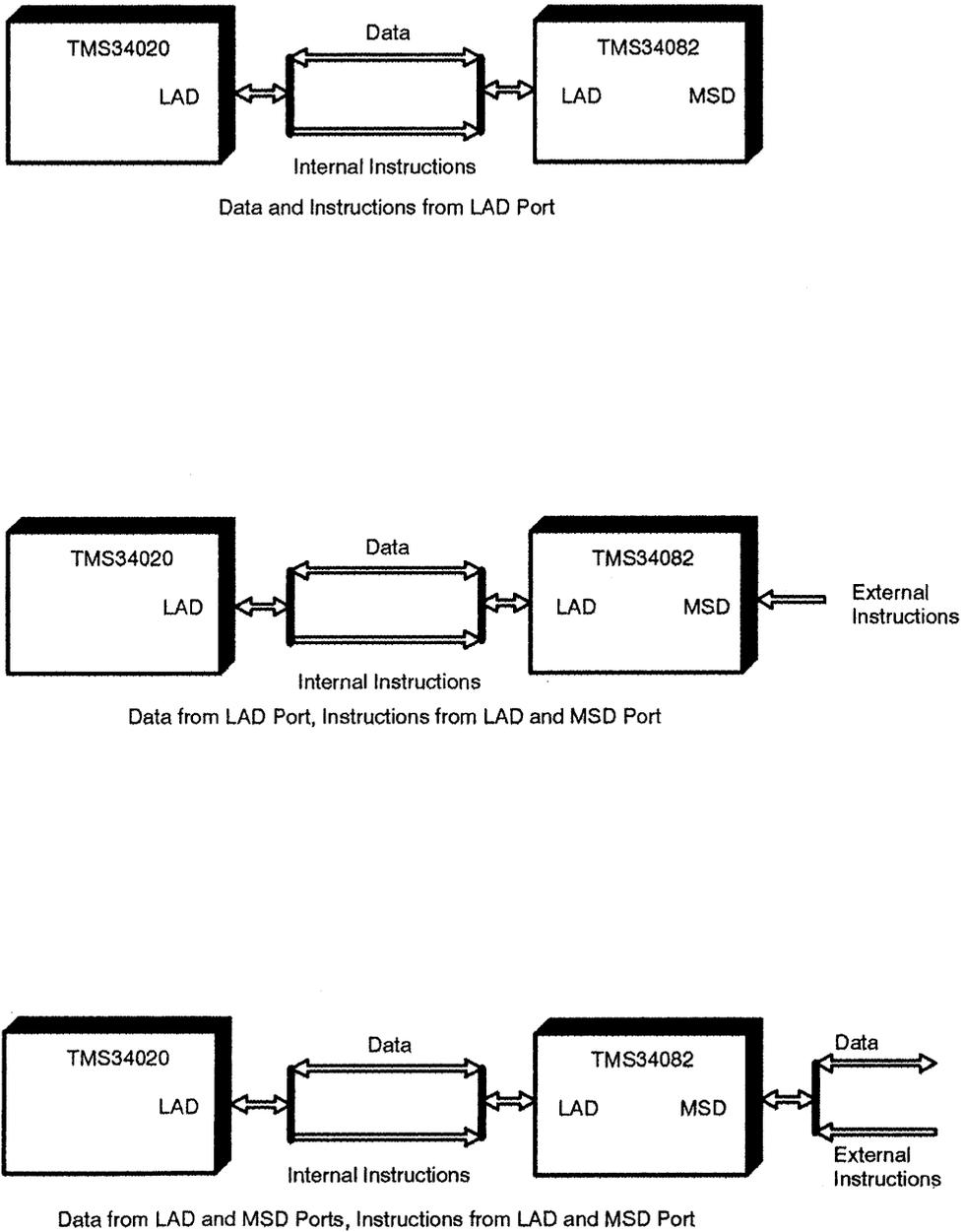
Figure 1-3. Host-Independent Mode Bus Architectures
