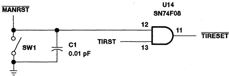
Figure 25. FIFO Logic, Details of U14
