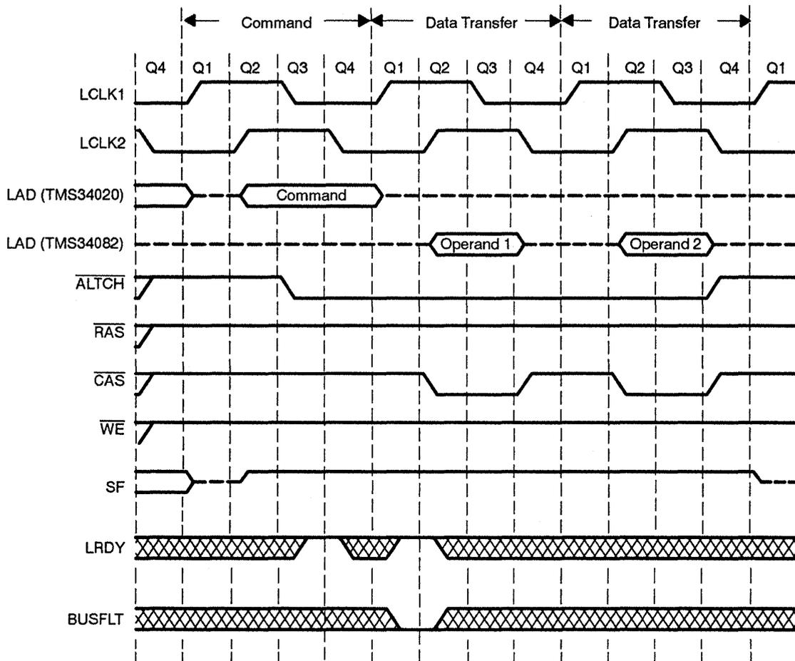
Figure 5-6. Transferring Memory to the TMS34082
