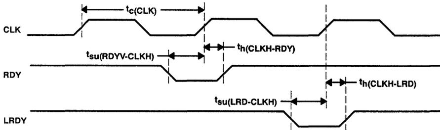
NOTE: When either RDY or LRDY is set low and the setup time before CLK high is observed, the device is stalled for one or more clock cycles, until RDY or LRDY is set high again. During a wait state, internal states and status are preserved and output signals do not change. LRDY can be used in this manner only in the host-independent mode.
