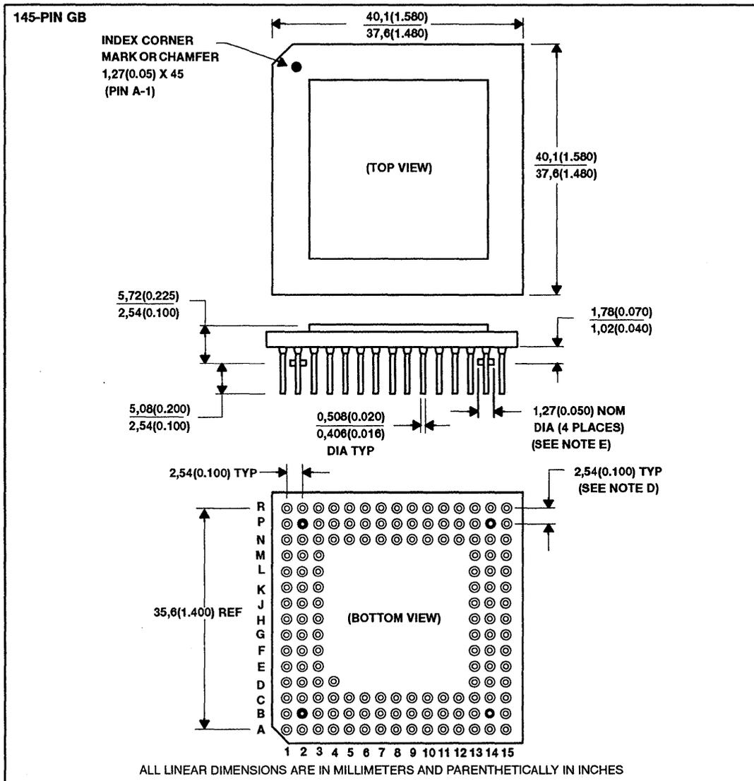
NOTES: D. Pins are located within 0,13 (0.005) radius of true position relative to each other at maximum material condition and within 0,457 (0.018) radius of the center of the ceramic.
