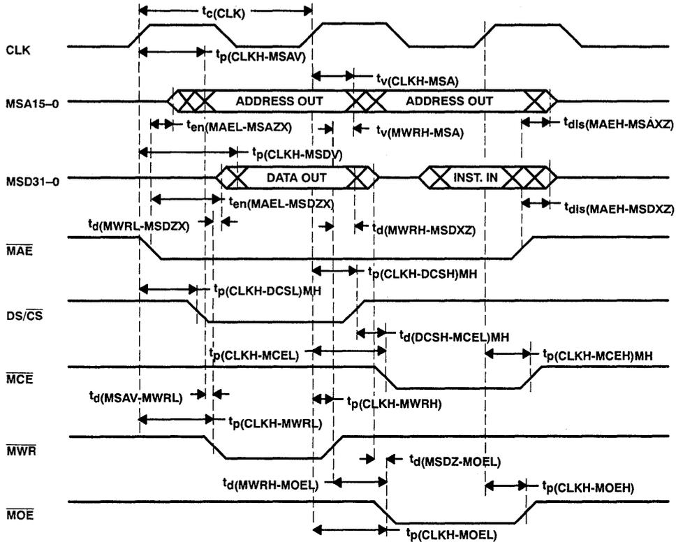
NOTE: This example shows a data write followed by an instruction read. Timing for multiple code writes would be similar. This option for using DS/CS as data space chip enable and MCE as code space chip enable is invoked by setting the MEMCFG bit high in the configuration register. When MEMCFG is high, DS/CS and MCE rise after every rising clock edge. In this mode, DS/CS and MCE may not both be low at the same time.
