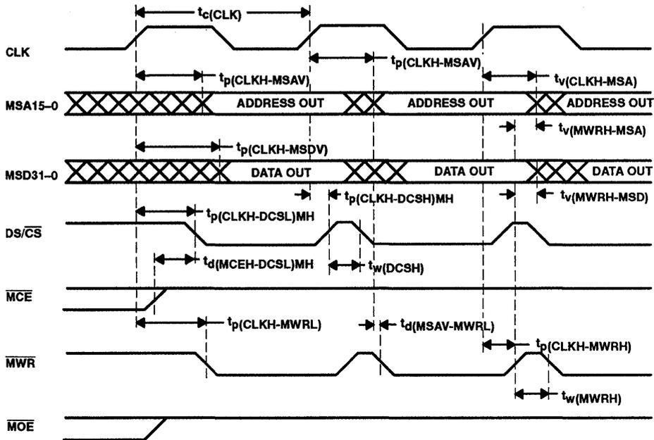
NOTE: This example shows multiple data writes. Timing for multiple code writes would be similar. This option for using DS/CS as data space chip enable and MCE as code space chip enable is invoked by setting the MEMCFG bit high in the configuration register. When MEMCFG is high, DS/CS and MCE rise after every rising clock edge. In this mode, DS/CS and MCE may not both be active (low) at the same time.
