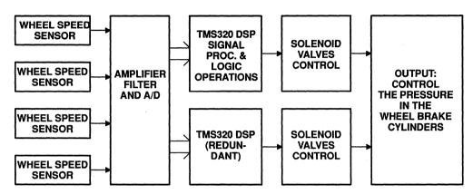
Figure 21. Anti-Lock Braking System (ABS) Block Diagram
