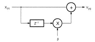
Figure A-1. One Zero FIR Filter.
