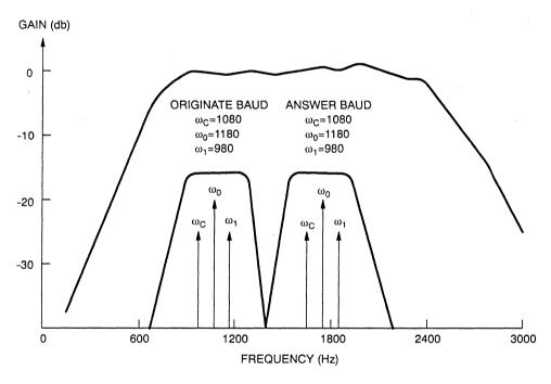
Figure 1. Spectral Response of a Typical Telephone and a V.21 Splitband Modem
