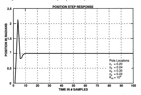
Figure 11. PID Controller Step Response for System's Third Pole Locations
