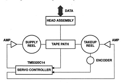
Figure 18. Block Diagram of a Tape Drive Controller
