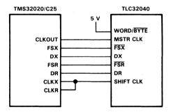
Figure 3-1. AIC Interface to TMS32020/C25
