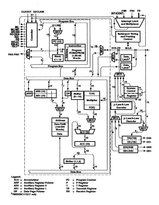
Figure 5. TMS320C17/E17 Block Diagram
