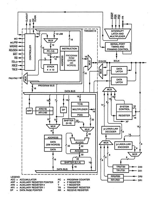
Figure 2. TMS320C17/E17 Block Diagram
