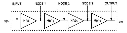
Figure 5. Four Op-Amp Block Diagram
