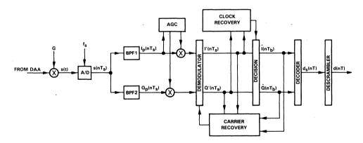
Figure 5. Modem Receiver Block Diagram
