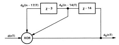
Figure 4. Signal Flowgraph of Transmitter Scrambler
