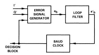
Figure 19. Baud Clock Alignment Block Diagram
