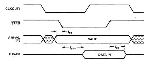
As shown in Figure 13, the EPROMs are not enabled until  $\overline{STRB}$  goes low. Since the address has been valid for at least  $t_{su} = 13$  ns before  $\overline{STRB}$  goes low, valid data appear on the data bus  $t_{a(S)} = 25$  ns (max) later. The EPROMs are disabled with  $\overline{STRB}$  going high, and their output buffers enter a high-impedance state,  $t_{dis} = 25$  ns (max) later. Therefore, no bus conflict occurs even if the memory read cycle is followed by a write cycle.
