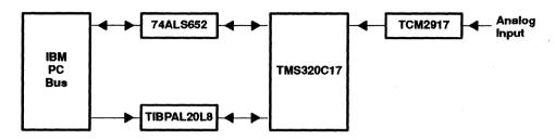
Figure 6. PC Tone Detector Circuit Diagram—Block Level
