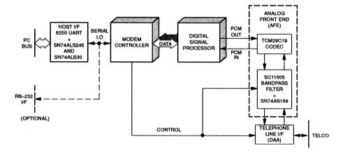
Figure 3. Block Diagram of Modem System Components
