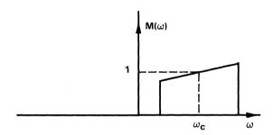
Figure A-2. Spectrum after Modulation
