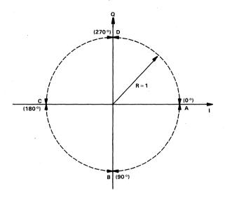
Figure 2. Signal Constellation for the Bell 212A/V.22
