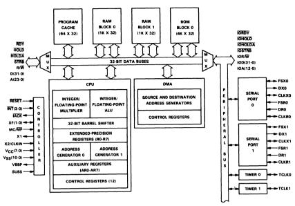
Fig. 7. TMS320C30 functional block diagram.
