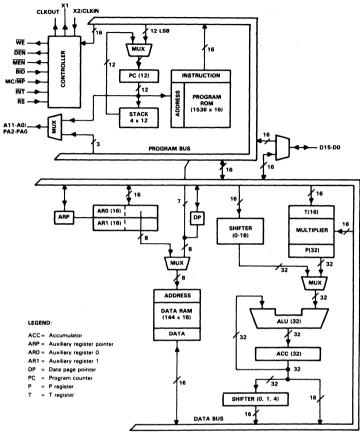
Fig. 4. TMS320C10 functional block diagram.
