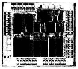
Capable of 10 million operations per second, the newest member of the TMS320 family can serve as an inexpensive alternative to bit-slice processors or custom ICs in digital signal processing applications.
