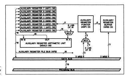
Figure 3. Auxiliary register file.
