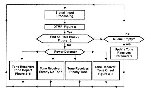
Figure 4. Tone Detector Flow Chart - Top Level
