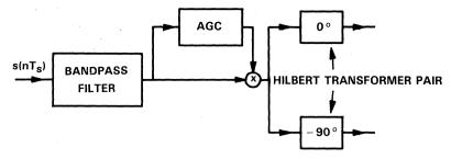
Figure 26. Alternative Modem Receiver Input Configuration
