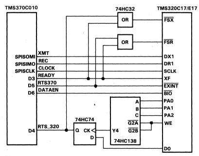
Figure 5. Stand-Alone TMS320C17/E17/TMS370 Serial Interface
