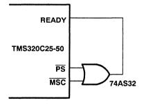
Applications having sufficiently simple address partitioning can make use of one or more levels of standard logic gates to generate READY. The circuit shown in Figure 4 has the following wait-state map:
