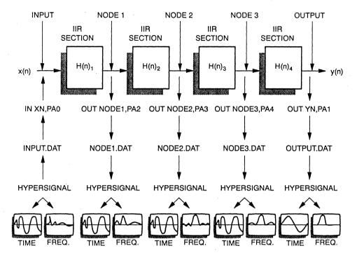
Figure 6. Four Second-Order IIR Structures
