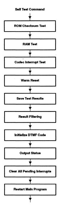
Figure 14. Tone Receiver Flow Chart - Self Test
