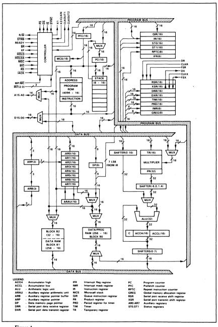
Figure 1. TMS320C25 block diagram.
