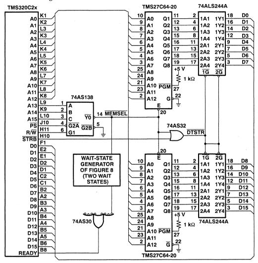
Figure 16. Interface of the TMS27C64-20 to the TMS320C2x
