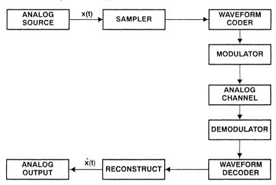
Figure 7. A Typical Communication Channel
