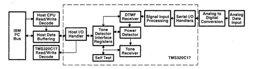
Figure 3. Tone Detector Functional Block Diagram
