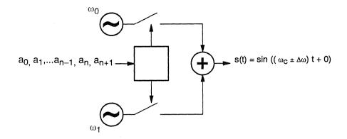
Figure 7. Functional Model of an FSK Modulator
