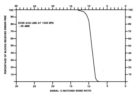
(a) PERCENTAGE OF BLOCKS RECEIVED ERROR-FREE BY THE TMS32010 MODEM VS. SNR WITH THE BELL MODEM TRANSMITTING
