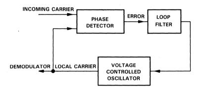
Figure 8. Carrier Recovery Phase-Locked Loop
