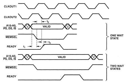
With this arrangement, READY is driven by a multiple-input NAND gate. This can be a standard gate such as a 74AS30 or can be part of the logic implemented by a high-speed programmable logic device. The output of this gate is low unless at least one of the inputs is low. The propagation delay of READY decode logic selecting zero wait-state devices in addition to the NAND delay
