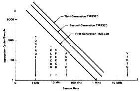
Fig. 3. Number of instruction cycles/sample versus sample rate for the TMS320 family.
