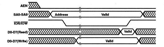
Figure 18. PC Bus Activity I/O Read or Write
