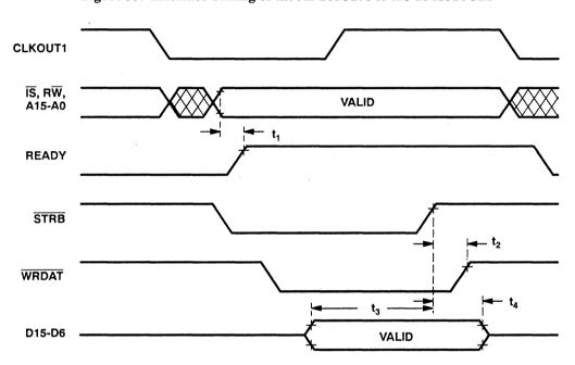
Figure 33. Interface Timing of the ADDAC100 to the TMS320C2x
