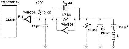
The 74AS04 inverter in Figure 26 provides the 180-degree phase shift that a parallel oscillator requires. The 4.7-k $\Omega$  resistor provides the negative feedback that keeps the oscillator in a stable
