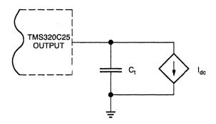
An equivalent load connected to each device output during the TMS320C25  $I_{CC}$  measurement is shown in Figure 5. Note that when the output is high, the device sources  $(V_{OH}-2.15)/825 = 303 \, \mu A$  at  $V_{OH}=2.4 \, V$ . The device sinks  $(2.15-V_{OL})/825=2.12 \, mA$  at  $V_{OL}=0.4 \, V$  when the output is low. When the output is switching, the output buffer drives  $100 \, pF$  of capacitance in addition to the resistor current.
