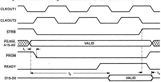
Figure 22. Interface Timing for Accesses of TMS27C64-15 to the TMS320C25-50
