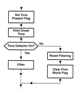
Figure 9. Power Detector Flow Chart—Tone Onset
