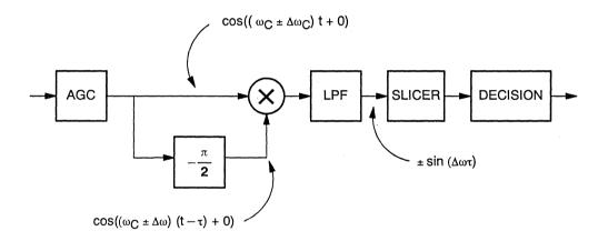
Figure 8. FSK Demodulator
