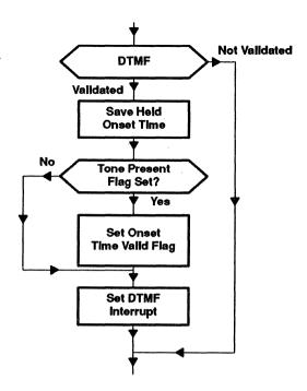
Figure 8. DTMF Receiver Flow Chart
