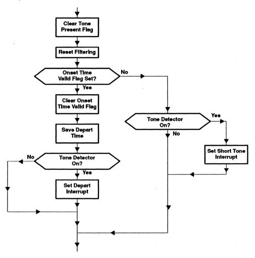
Figure 11. Power Detector Flow Chart—Tone Departure
