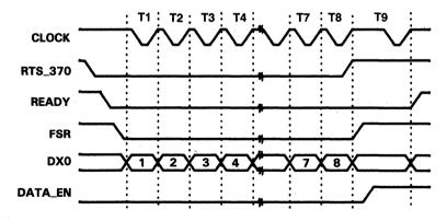
Figure 8. Timing Diagram for TMS370C010 to TMS320C17/E17 Transmission
