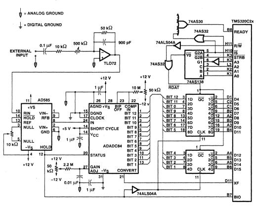
Figure 30. Interface of the ADADC84 to the TMS320C2x
