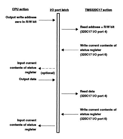
Figure 19. Host Write Cycle
