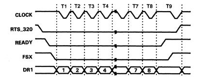
Figure 9. Timing Diagram for TMS320C17/E17 to TMS370C010 Transmission
