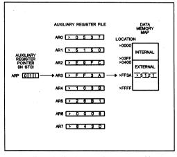
Figure 5. Example of indirect auxiliary register addressing.
