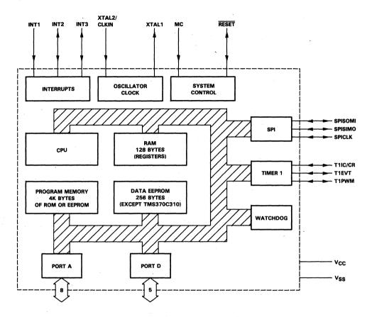
Figure 6. TMS370C010 Block Diagram
