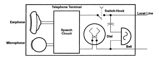
Figure 1. Pulse Dialing Telephone
