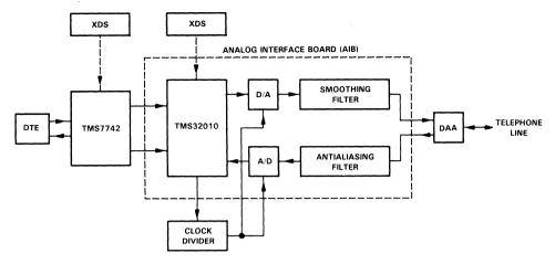
Figure 11. Modem Hardware Block Diagram
