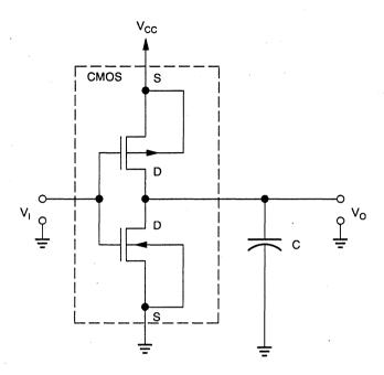
If the input voltage is fixed at a logic high or logic low level, one of the two inverter transistors will be non-conducting (off) while the other has a highly conductive channel (on). Under this condition, the supply current is equal to the negligibly small P-N junction leakage current through the off device.
