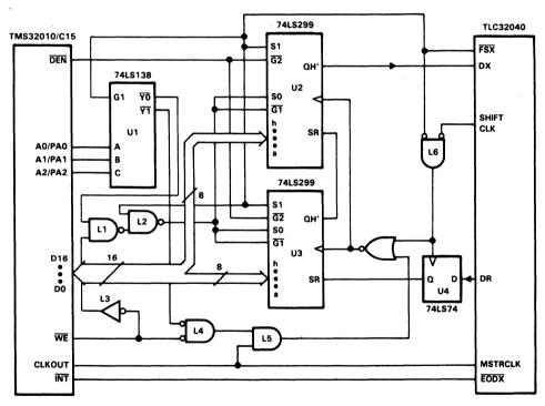
Figure 2-1. AIC Interface to TMS32010/E15
