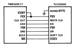
Figure 4-1. AIC Interface to TMS320C17
