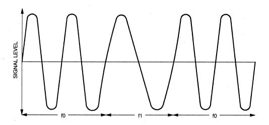
Figure 2. FSK Signal Transmission
