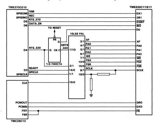
Figure 11. Serial Interface with CODEC
