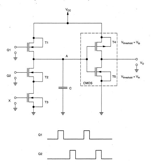
Again, this high-current condition is not of concern in static logic circuits, and is only of concern in dynamic logic circuits at very low clock frequency. The minimum input clock frequency of the TMS320C25 is specified at 6.7 MHz. This lower limit is orders of magnitude higher than the frequency at which adverse mechanisms in dynamic logic come into play; its choice was driven by other practical considerations such as test time minimization.
