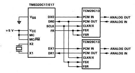
Figure 4. Simple TMS320C17/E17/CODEC Interface
