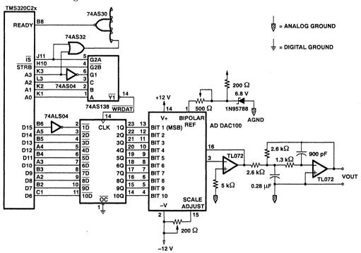
Figure 32. Interface of the ADDAC100 to the TMS320C2x
