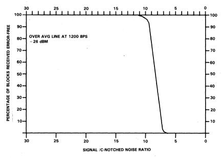
(b) PERCENTAGE OF BLOCKS RECEIVED ERROR-FREE BY THE AT&T MODEM VS. SNR WITH THE BELL MODEM TRANSMITTING
