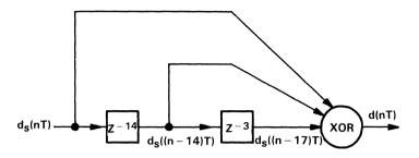
Figure 7. Signal Flowgraph of Receiver Descrambler
