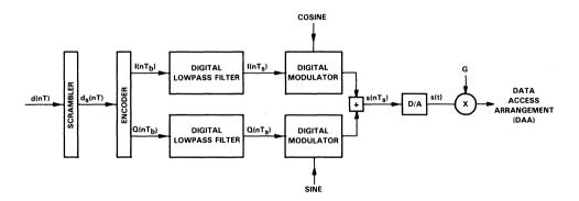
Figure 3. Modem Transmitter Block Diagram
