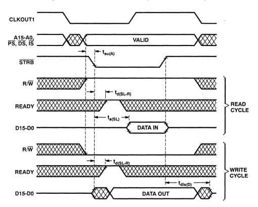
Figure 20. TMS320C25-50 Memory Read and Write Cycle
