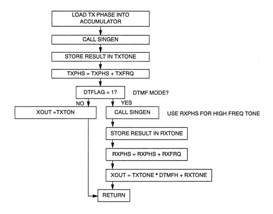
Figure 6. Flowchart of Subroutine FSKTX
