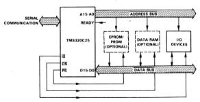
Fig. 6. Minimal processing system with external data RAM and PROM/EPROM.
