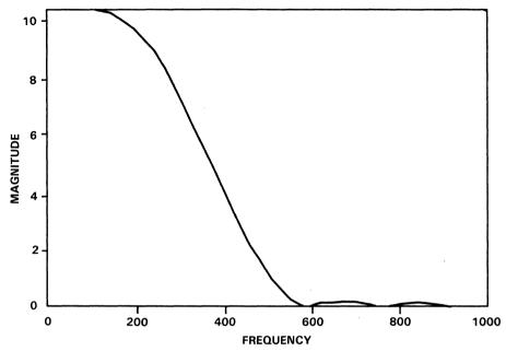
Figure 13. Frequency Response Characteristics of Transmit Lowpass Filters
