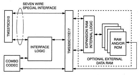
Figure 1. Block Diagram of TMS320C17/E17/TMS370C010 System
