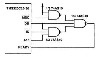
Note that this circuit just meets the READY specification of the TMS320C25-50 with READY guaranteed valid no later than 9 ns from address valid.
