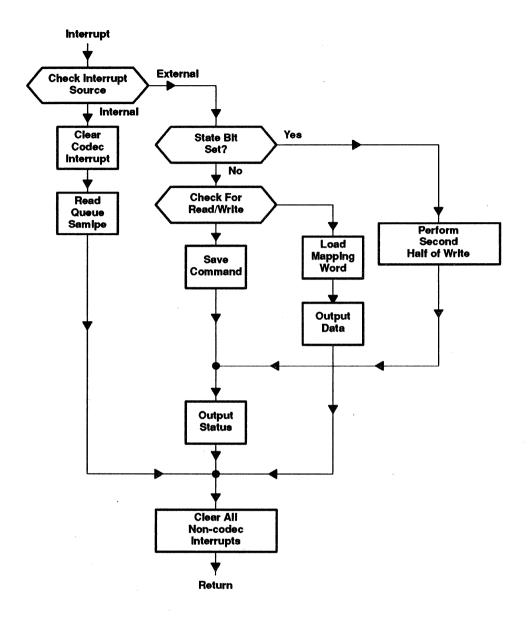
Figure 13. I/O (Interrupt Handler) Flow Chart
