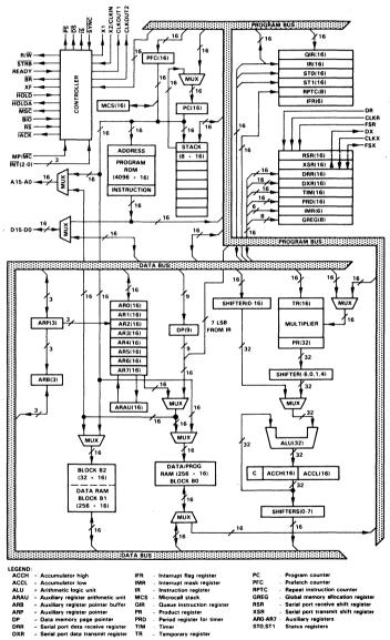
Fig. 5. TMS320C25 functional block diagram.
