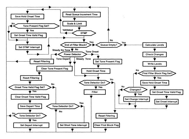
Figure 15. Tone Detector Flow Chart (Detailed)
