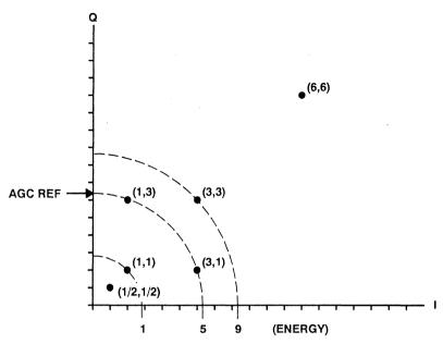
In Figure 3, constellation points (3,3) and (1,1) with respective energy contents of 9 and 1 felie outside the reference level of 5. A window function is then necessary so that the AGC does not treat these energy variations around the nominal energy as distortions induced by the communication channel.
