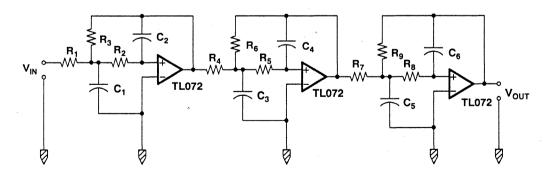
The design of Figure 34 is used to implement the antialiasing and smoothing filtering operations in the TMS32010 Analog Interface Board. The cutoff frequency of this filter depends on the values of the passive components. The values of these components for several cutoff frequencies are shown in Table 15.[3]
