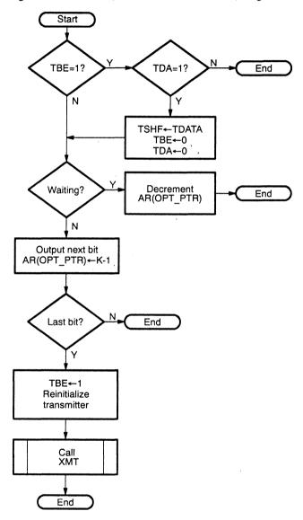
Figure 4. Transmitter Routine
