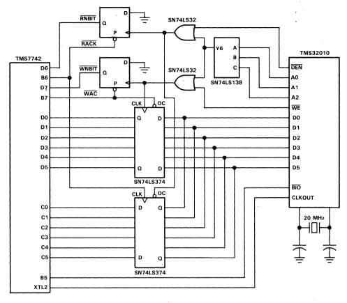
Figure 12. TMS7742 and TMS32010 Interface
