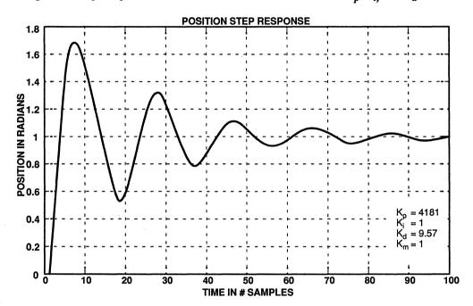
Figure 6. Step Response of the PID Controller with Second Set of  $K_p$ ,  $K_i$ , and  $K_d$  Values
