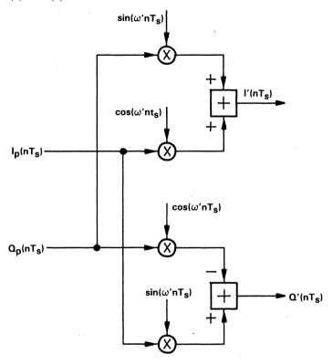
Figure 6. Demodulator Structure
