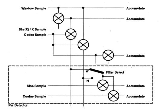
Figure 10. FIR Filter Structure
