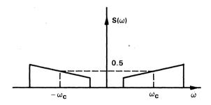
Figure A-3. Transmitted Spectrum
