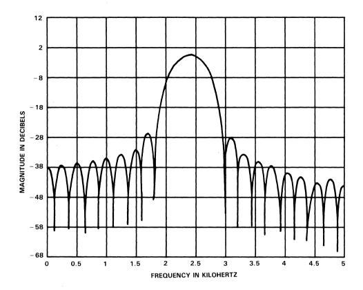
Figure 15. Frequency Response of Receiver Bandpass Filters
