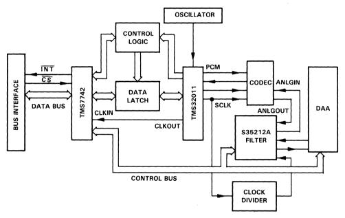
Figure 25. Modem Hardware Block Diagram Using a Codec for the A/D and D/A Conversions
