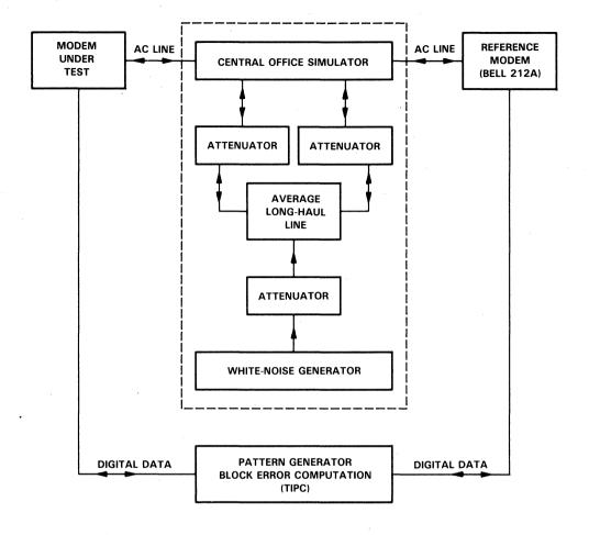
Figure 21. Modem Testing Equipment
