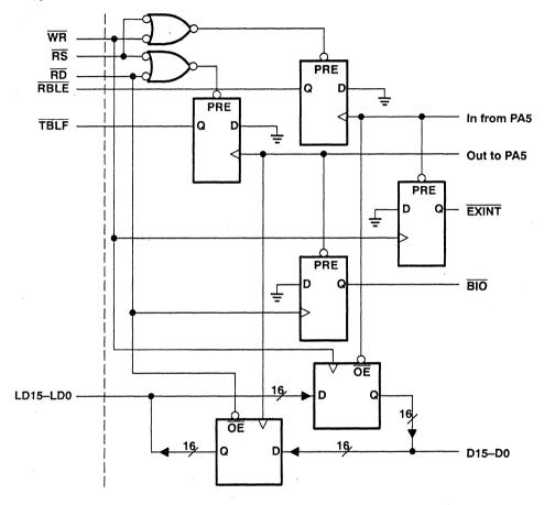
Figure 24. TMS320C17/E17 Simplified Coprocessor Port Logic Diagram
