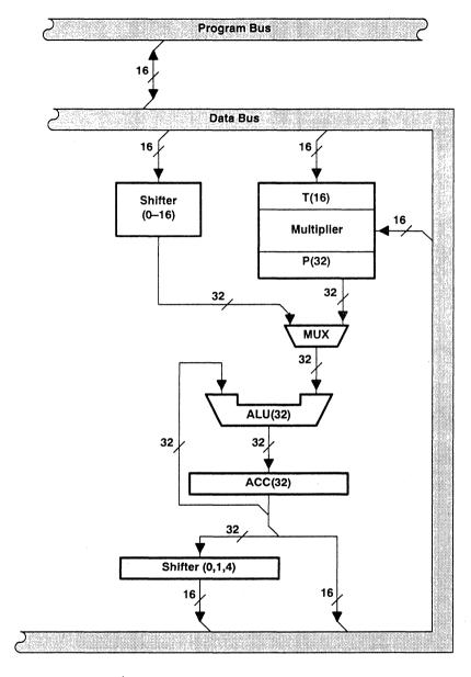
Figure 16. Central Arithmetic Logic Unit (CALU)
