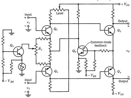
Fig. 8.17. D-c differential amplifier.
