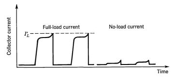
Fig. 34.5. Dual-transformer converter: typical collector currents.
