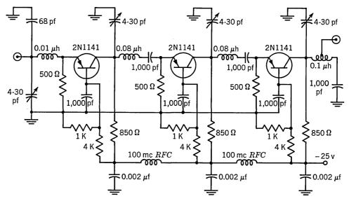
0.08 and 0.1  $\mu$ h coils are 3 and 4 turns respectively of No. 18 tinned bus wire,  $^{1}/_{4}$ " diameter
