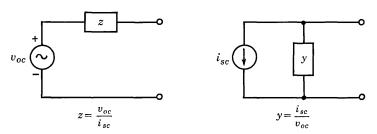
Fig. 6.1. Two-terminal network.
