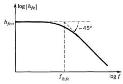
Fig. 19.8.  $|h_{fe}|$  vs. frequency.
