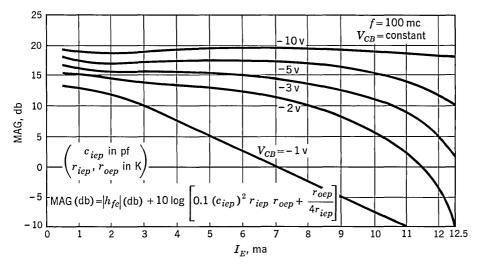
Fig. 24.6. Maximum available power gain vs.  $I_E$ .
