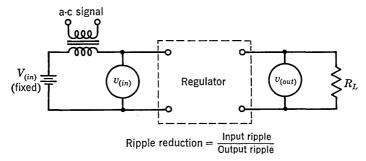
Fig. 9.22. Ripple reduction test circuit.
