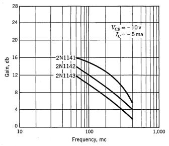
Fig. 20.6. Common-base unilateralized RF power gain.
