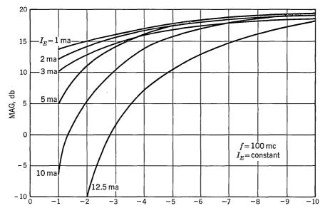
Fig. 24.7. Maximum available power gain vs.  $V_{\it CB}$ .
