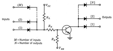
Fig. 29.17. Basic NAND TDL circuit.
