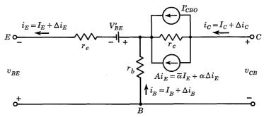
Fig. 8.1. Equivalent circuit for direct current and low-frequency alternating current (NPN).
