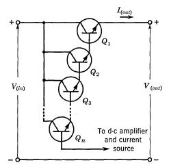
Fig. 9.9. Compound connection used as series control element.
