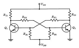
Fig. 27.1. Basic flip-flop.
