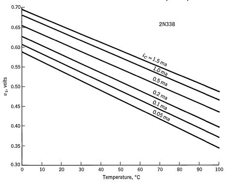
Fig. 8.7. Equivalent input voltage drift, single-ended stage silicon transistor.
