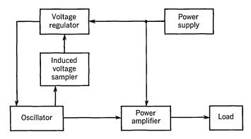
Fig. 35.1. Block diagram of 60-cycle power inverter.
