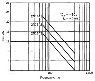
Fig. 20.8. Common-emitter unilateralized RF power gain.
