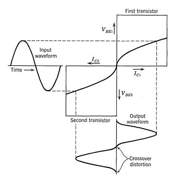
Fig. 17.1. Composite transfer characteristic for unbiased stage.
