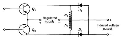
Fig. 35.2. Induced-voltage-sensing circuit.
