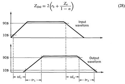
Fig. 29.26. Typical input and output waveforms for a transistor switch.
