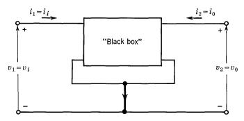
Fig. 6.3. Three-terminal network: a special case.
