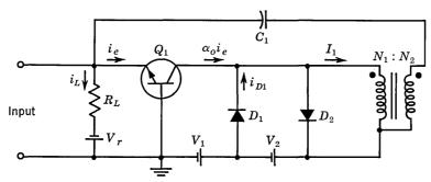
Fig. 33.2. Common-base nonsaturating triggered blocking oscillator.
