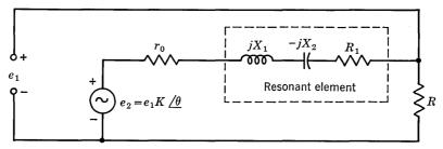
Fig. 12.6. Simplified schematic of feedback oscillator.
