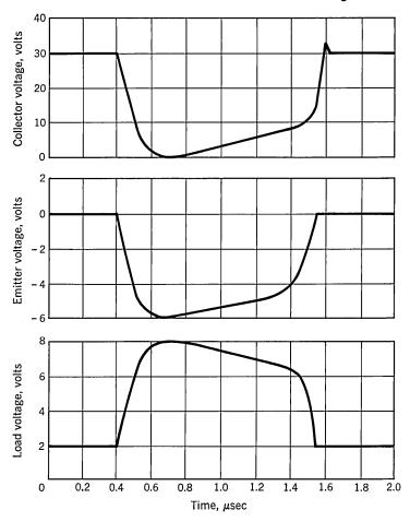
Fig. 33.5. Blocking-oscillator waveforms with 100-ohm load.
