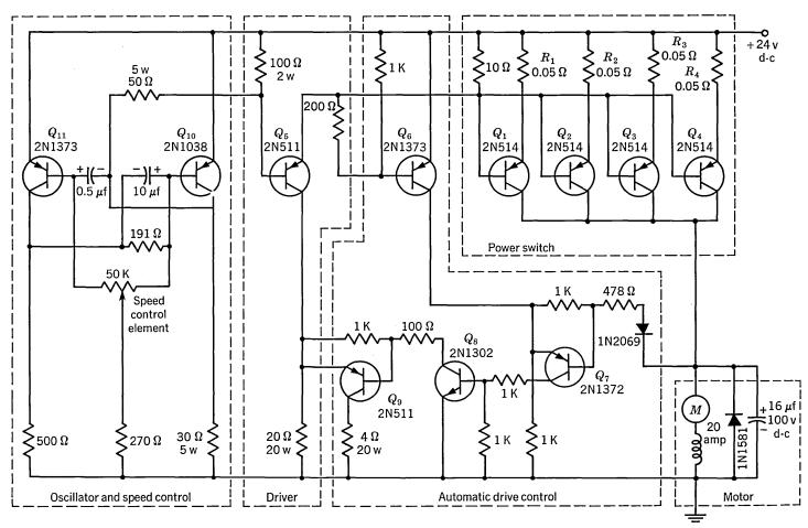
Fig. 37.3. Complete schematic diagram of speed-control system.
