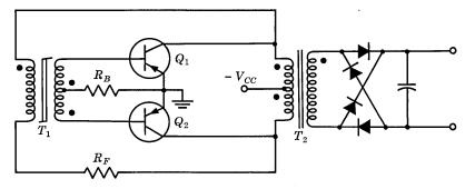
Fig. 34.4. Basic dual-transformer converter.
