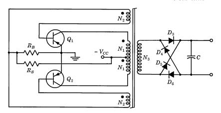
Fig. 34.7. Type A converter.
