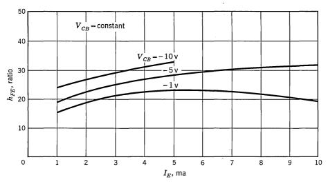
Fig. 24.17. D-c forward current transfer ratio ( $h_{FE}$ ) vs.  $I_{E}$ .
