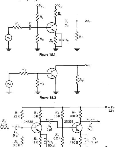
Fig. 15.3. Two-stage cascaded CE audio amplifier.
