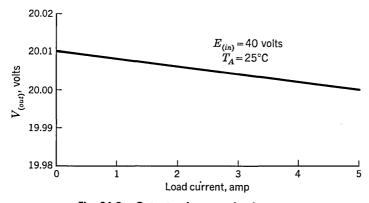
Fig. 36.9. Output voltage vs. load current.
