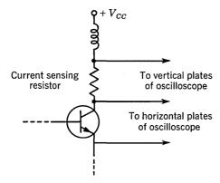
Fig. 31.2. Measurement of load line.
