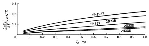
Fig. 8.12.  $\Delta \bar{\alpha} I_E/\Delta T$  vs.  $I_C$ .
