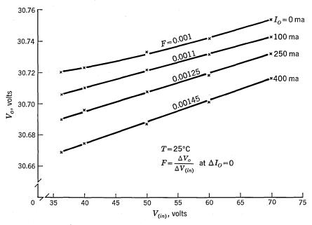
Fig. 9.15.  $V_o$  vs.  $E_{(in)}$  for circuit of Fig. 9.14.
