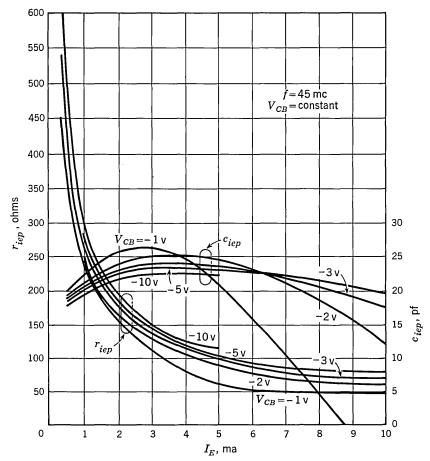
Fig. 24.12. Parallel component of input resistance and capacitance vs. emitter current (at f = 45 mc).
