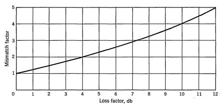
Fig. 20.13. Loss factor vs. mismatch factor.
