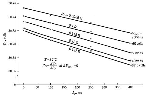
Fig. 9.16.  $V_o$  vs.  $I_o$  for circuit of Fig. 9.14.
