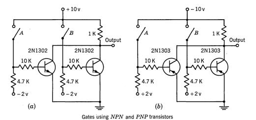
Fig. 29.9. Basic logic circuits using parallel transistors.
