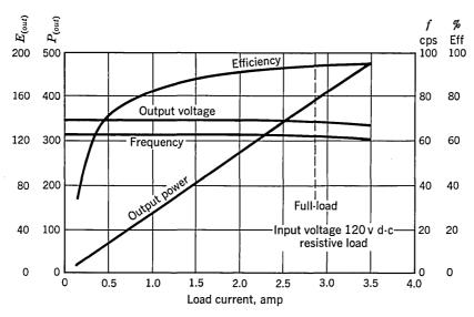
Fig. 35.16. 400-watt inverter operating characteristics.
