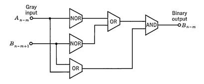
Fig. 39.5. Gray-to-binary converter module.
