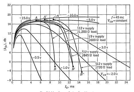
Fig. 24.11.  $h_{fe}$  vs.  $I_E$  (at f = 45 mc).
