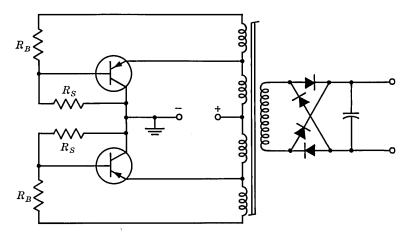
Fig. 34.3. Common-collector autotransformer configuration.
