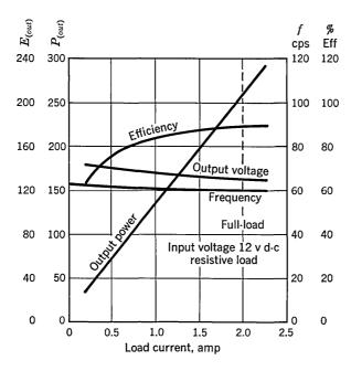
Fig. 35.15. 250-watt inverter operating characteristics.
