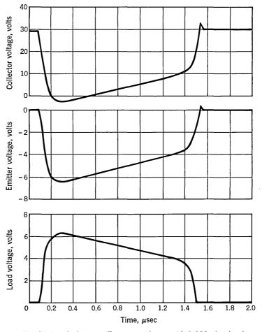
Fig. 33.4. Blocking-oscillator waveforms with 1,000-ohm load.
