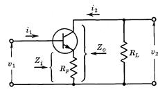
Fig. 19.1. Simplified series feedback circuit.
