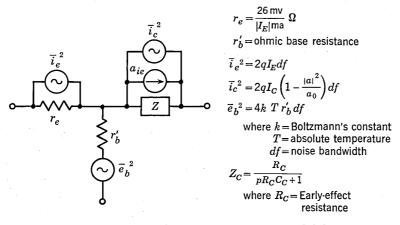
Fig. 21.1. Noise equivalent circuit of transistor, and definitions.
