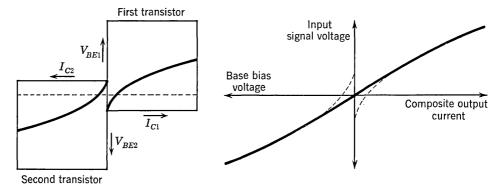
Fig. 17.2. Composite transfer characteristic for biased stage.
