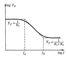
Fig. 19.14.  $Y_F$  vs. frequency.
