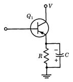
Fig. 29.35. Emitter-follower driving a capacitive load.
