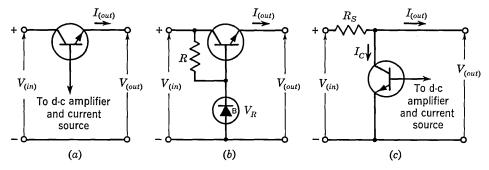
Fig. 9.8. Regulator control elements: (a) series regulator; (b) emitter-follower regulator; (c) shunt regulator.
