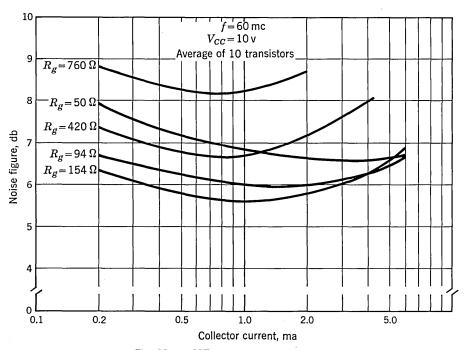
Fig. 21.7. NF vs.  $I_{Cr}$  transistor 2N743.
