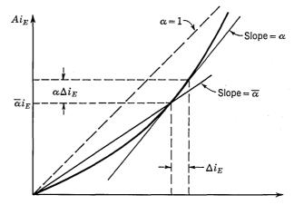
Fig. 8.3. Collector current generator static characteristic.
