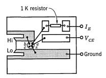
Emitter and collector terminals of transistor socket are fitted into Erie type 2405-102 feed-through capacitors. Shield terminal is wired to ground
