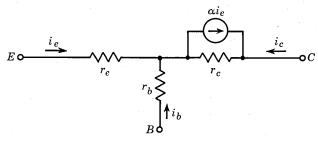
Fig. 6.10. T-equivalent circuit, common base.
