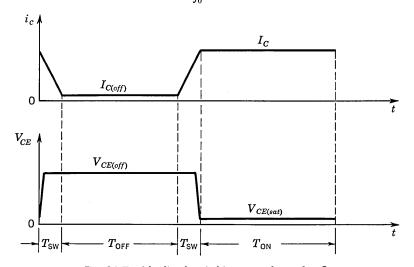
Fig. 36.7. Idealized switching waveforms for  $Q_9$ .
