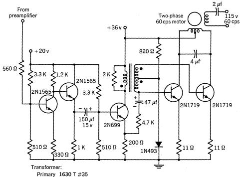
Secondary 1020 T #29 Bifilar wound Laminations El 75 SL14 5 x 5 interleaved
