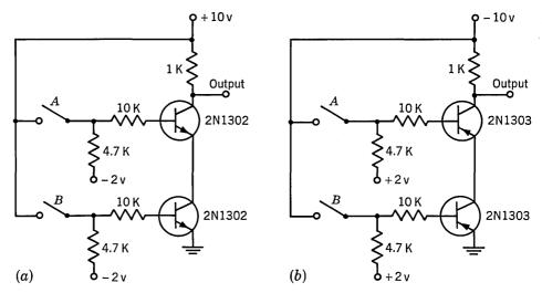
Gates using NPN and PNP transistors and gate for normally open switches or gate for normally closed switches Note: Phase inversion of input
