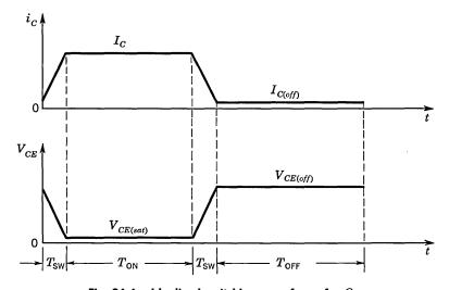
Fig. 36.6. Idealized switching waveforms for  $Q_8$ .
