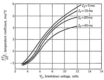
Fig. 9.3. Temperature coefficient vs. breakdown voltage: 1N746 series.
