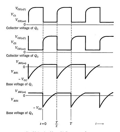
Fig. 28.5. Astable multivibrator waveforms.
