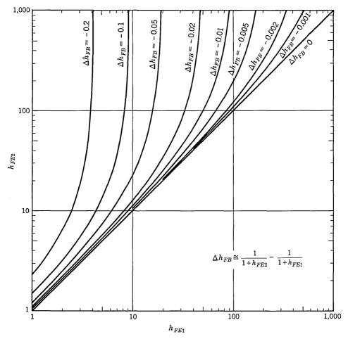
Fig. 7.16.  $\Delta h_{FB}$  vs.  $\Delta h_{FE}$ .
