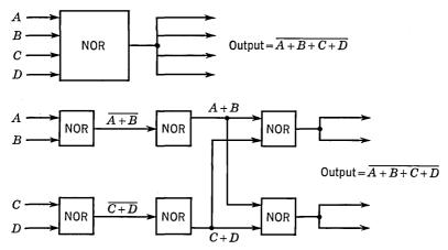
Fig. 29.7. Four-input, four-output NOR logic.
