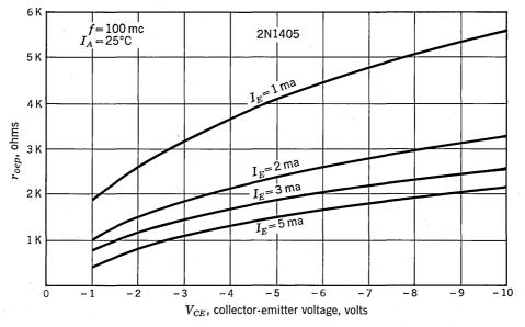
Fig. 4.22. Equivalent short-circuit common-emitter parallel output resistance  $r_{oep}$  at 100 mc.
