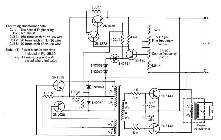
Fig. 35.5. 200-watt 60-cycle inverter.
