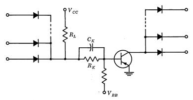
Fig. 29.20. NAND logic with speedup capacitor.
