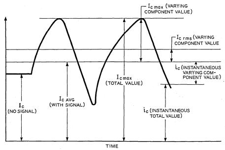
Figure 1. Chart of Collector Current Versus Time
