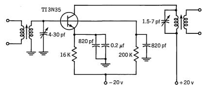
Fig. 20.26. One stage of the amplifier.
