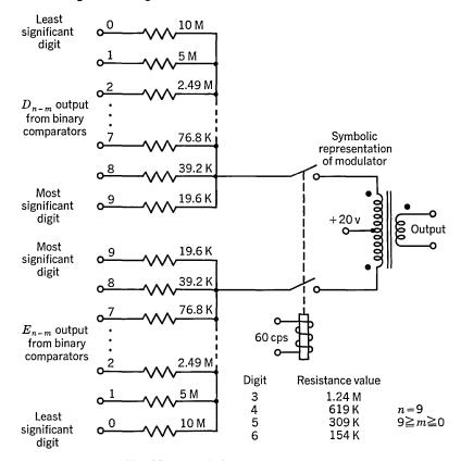
Fig. 39.7. Digital-to-analog converter.
