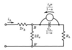
Fig. 29.28. Composite equivalent circuit.
