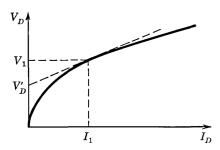
Fig. 17.8. Diode forward characteristic.
