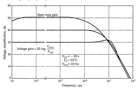
Fig. 19.23. Typical frequency response of wideband amplifier in Fig. 19.22.
