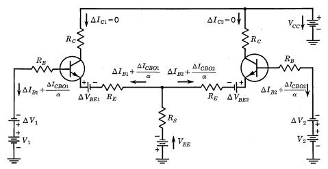
Fig. 8.19. Common-emitter amplifier configuration.
