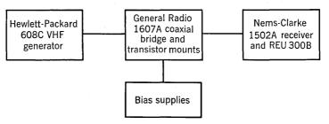
Fig. 20.21. Test-equipment block diagram.
