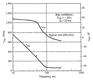
Fig. 4.18.  $c_{iep}$  and  $r_{iep}$  vs. frequency: type 2N1141.
