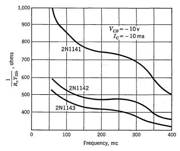
Fig. 20.16. Parallel output resistance common base vs. frequency.
