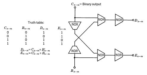
Fig. 39.6. Binary comparator module.
