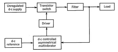
Fig. 36.1. Block diagram of switching regulator.
