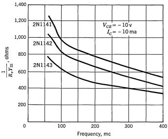
Fig. 20.19. Parallel output resistance common emitter vs. frequency.
