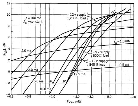
Fig. 24.2.  $h_{fe}$  vs.  $V_{CB}$  (at f = 100 mc).
