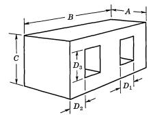
Fig. 34.19. Transformer core.
