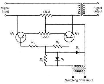
Fig. 10.7. Practical design for transistor chopper.
