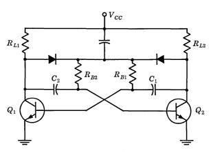
Fig. 28.6. Sure-starting astable multivibrator.
