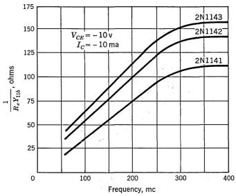
Fig. 20.17. Parallel input resistance common base vs. frequency.
