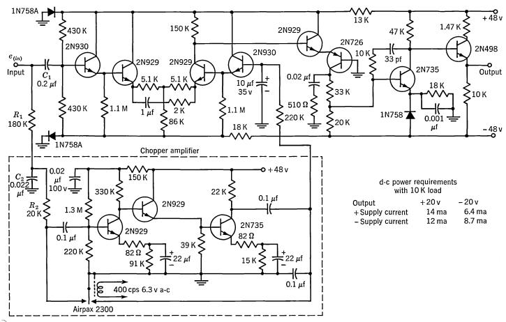
Fig. 14.2. Chopper-stabilized d-c operational amplifier.
