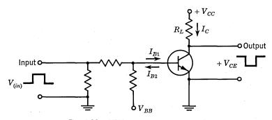
Fig. 4.28. NPN common-emitter switch.
