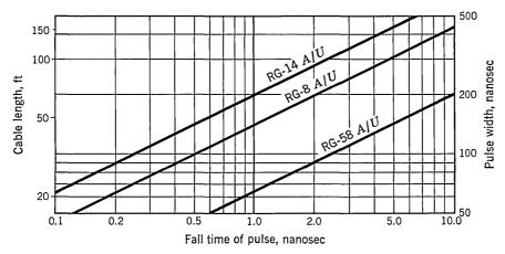
Fig. 5.32. Fall time of pulse vs. pulse width.
