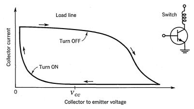
Fig. 31.3. Switch with inductive load.
