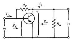
Fig. 19.2. Simplified shunt feedback circuit.
