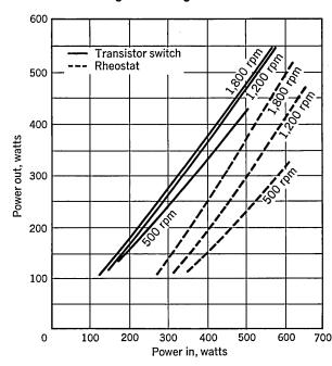
Fig. 37.7. Control element: power out vs. power in (speed = constant).
