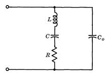
Fig. 22.8. Equivalent circuit of a quartz crystal.
