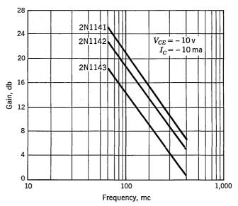
Fig. 20.7. Common-emitter unilateralized RF power gain.
