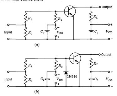
Fig. 5.38.  $BV_{EBO}$  protection circuit.
