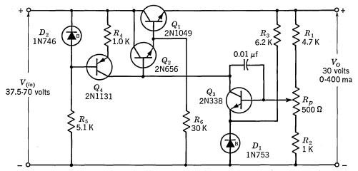
Fig. 9.14. Typical series regulator using transistor-type preregulator.
