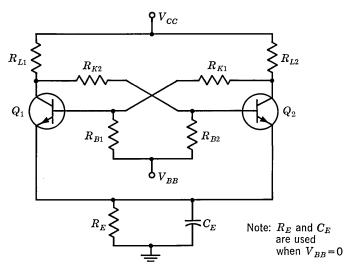
Fig. 28.1. Basic flip-flop with emitter bias.
