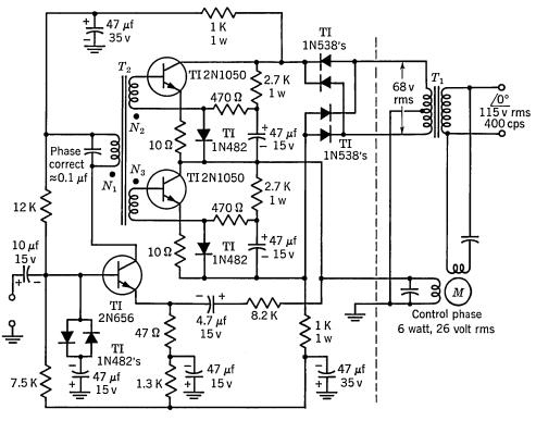
Transformers:  $T_1$  400 cps 12-watt power transformer step-down 115 volt to 68 volt c.t.  $T_2$  400 cps 65-mw driver transformer. Turns ratio  $N_1:N_2:N_3=2:1:1$  Primary current = 10 ma d-c. Primary inductance = 1.5 hy.
