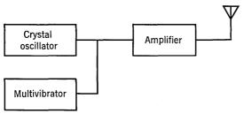
Fig. 26.1. Transmitter block diagram.
