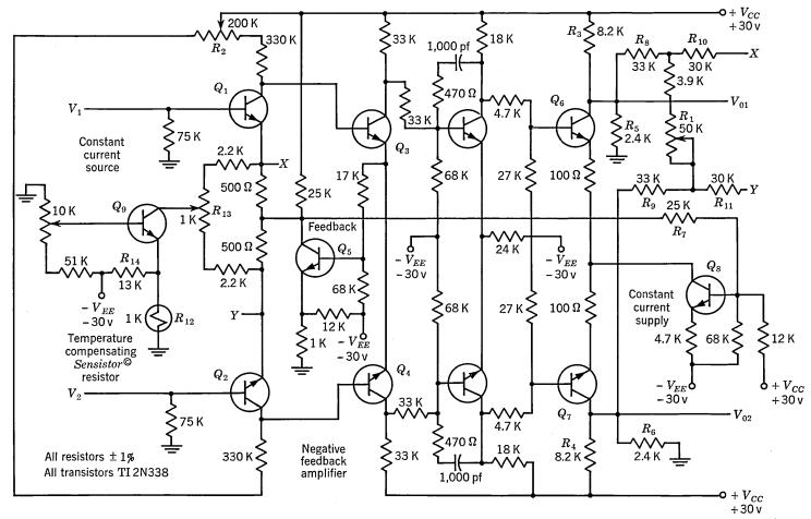
Fig. 8.18. Differential amplifier circuit.
