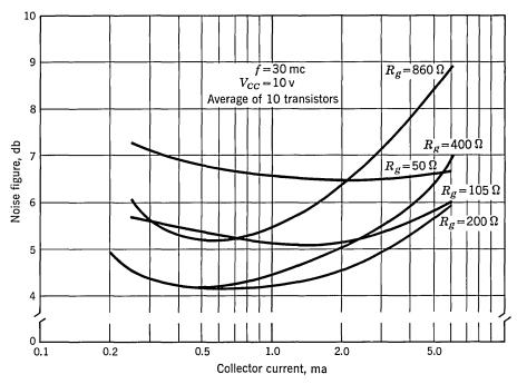
Fig. 21.6. NF vs.  $I_{Cr}$  transistor 2N743.
