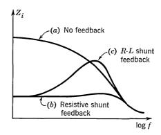
Fig. 19.16. Input impedance vs. frequency.
