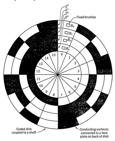
Fig. 39.2. Binary-coded disk.
