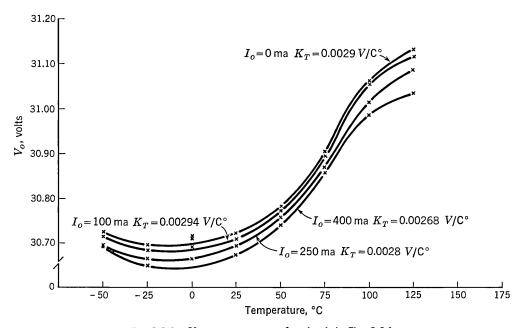
Fig. 9.17.  $V_o$  vs. temperature for circuit in Fig. 9.14.
