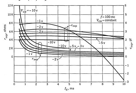
Fig. 24.5. Parallel component of output resistance and capacitance (common emitter) vs. emitter current.
