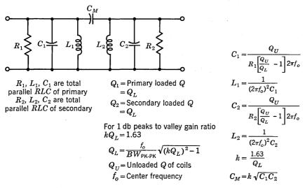
Fig. 20.3. Design equations for capacitive coupling.
