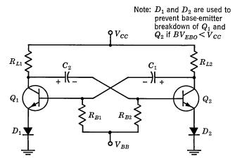
Fig. 28.4. Basic astable multivibrator.
