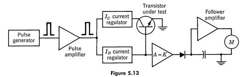
The pulse test circuit used at Texas Instruments is built up using the above described circuit elements. Figure 5.13 shows a simplified drawing of the complete pulse  $V_{BE}$  test circuit.
