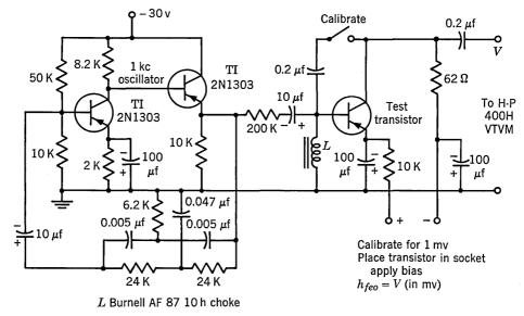
Fig. 21.9.  $h_{feo}$  at 1-kc test circuit.
