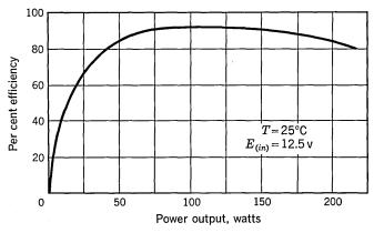
Fig. 35.10. Efficiency vs. power output.
