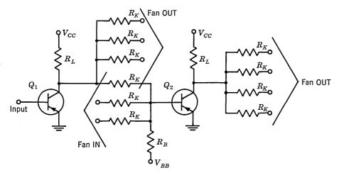
Fig. 29.11. Connection of TRL circuits.
