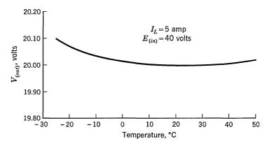
Fig. 36.10. Output voltage vs. temperature.
