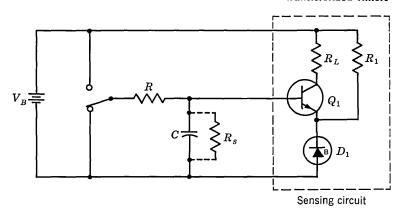
Fig. 30.2. Transistorized RC timing circuit.
