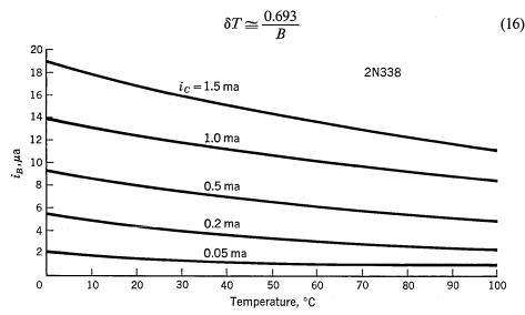
Fig. 8.9. Equivalent input current drift, single-ended stage silicon transistor.
