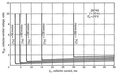
Fig. 4.24. Contours of constant transadmittance,  $|y_{fe}|$ .
