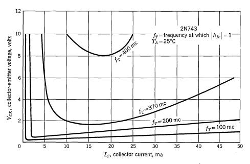
Fig. 4.27. Contours of constant-gain-bandwidth product,  $f_T$ .
