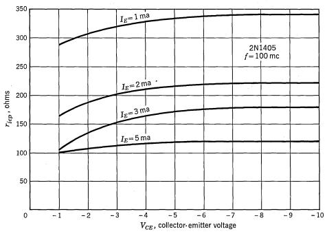
Fig. 4.19. Equivalent short-circuit common-emitter parallel input resistance  $r_{iep}$ .
