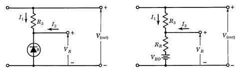
Fig. 9.5. A reference element and its equivalent circuit.
