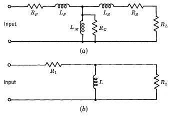
Fig. 34.2. Approximate transformer equivalent circuits.
