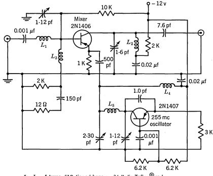
$L_1$ ,  $L_2$  4 turns #18 tinned buss on  $^3/_8$ " dia Teflon® rod
