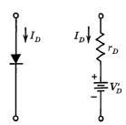
Fig. 17.9. Diode equivalent circuit.
