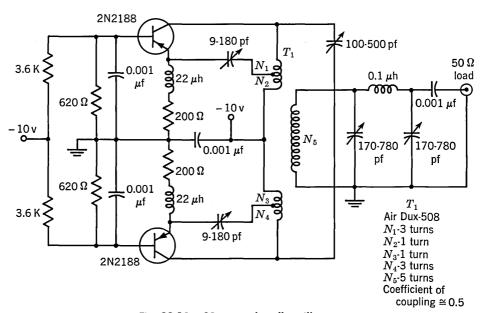
Fig. 22.10. 23-mc push-pull oscillator.
