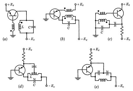
Fig. 12.2. Some basic transistor oscillators using external feedback.
