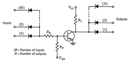
Fig. 29.14. Basic NOR TDL circuit.
