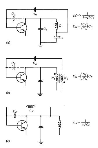
Fig. 20.1. Methods of unilateralization: (a) capacitance bridge circuit; (b) capacitance tap circuit; (c) inductive feedback circuit.
