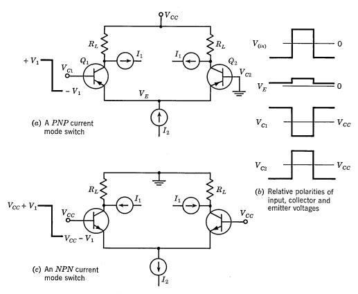
Fig. 29.22. Current mode switches.
