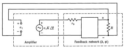
Fig. 12.5. Block diagram of feedback-type oscillator.
