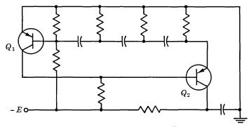
Fig. 12.4. Phase-shift-type oscillator.
