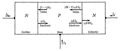
Fig. 4.8. One-dimensional transistor model.
