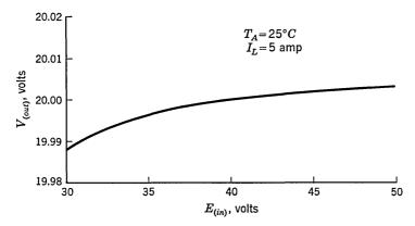
Fig. 36.8. Output voltage vs. d-c input voltage.
