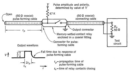
Fig. 5.31. Coaxial pulse generator.
