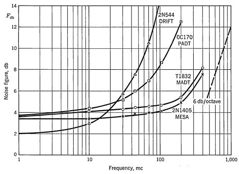
Fig. 21.5. Experimental values for transistor noise figure vs. frequency for four types of germanium high-frequency transistors.  $R_g=$  50 ohms,  $I_E=$  1.5 ma,  $V_{CB}=-$ 9.0 volts.
