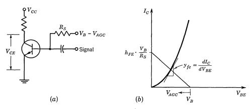
Fig. 11.3. Typical  $y_{FE}$  curve.
