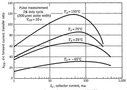
Fig. 4.7.  $h_{FE}$  vs.  $I_C$  characteristics of 2N697.
