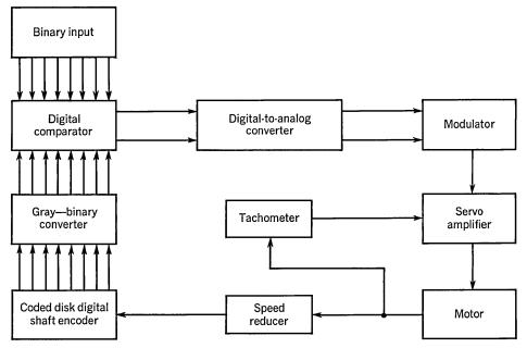
Fig. 39.1. Block diagram of digital servo system.
