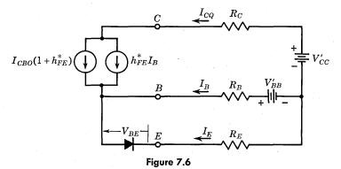
**Setting the Bias.** By combining the internal and external equivalent circuits as in Fig. 7.6, an expression for the bias-point collector current,  $I_{CQ}$ , can be obtained. From Fig. 7.6,
