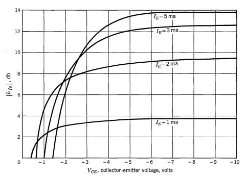
Fig. 4.25. Short-circuit common-emitter forward current transfer ratio  $\left|h_{\it fe}\right|$  at 100 mc.
