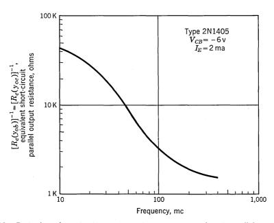
Fig. 4.21. Equivalent short-circuit common-emitter (or common-base) parallel output resistance vs. frequency.
