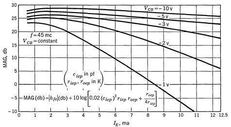
Fig. 24.14. Maximum available power gain vs.  $I_E$  (at f= 45 mc).
