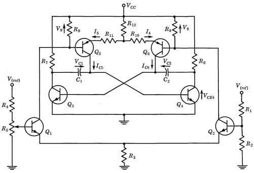
Fig. 36.2. D-c controlled asymmetrical multivibrator.
