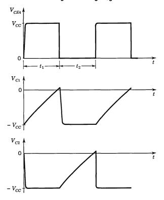
Fig. 36.3. Multivibrator voltage waveform.
