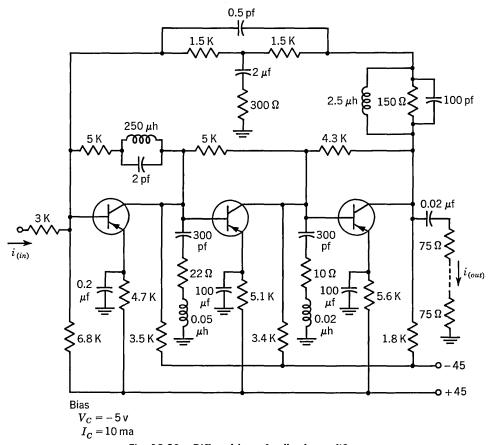
Fig. 19.20. Diffused-base feedback amplifier.
