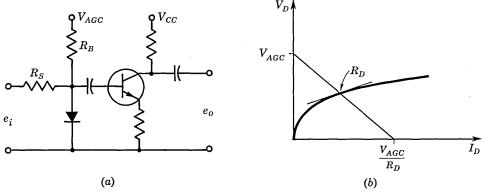
Fig. 11.4. (a) AGC circuit; (b) diode characteristics.
