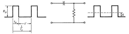
Fig. 5.36. D-c shift with capacitor coupling.
