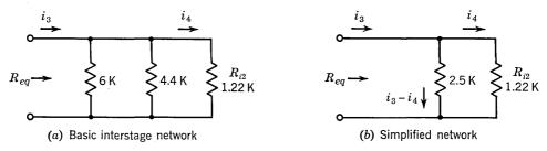
Fig. 15.7. Interstage network of a two-stage cascaded CE audio amplifier.
