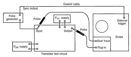
Fig. 5.28. Typical switching time test setup.
