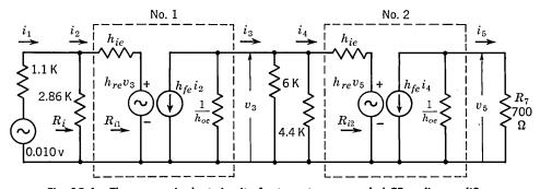
Fig. 15.4. The a-c equivalent circuit of a two-stage cascaded CE audio amplifier.
