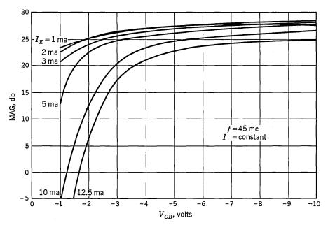
Fig. 24.15. Maximum available power gain vs.  $V_{\it CB}$  (at f= 45 mc).
