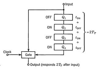
Fig. 4.31. Propagation time.
