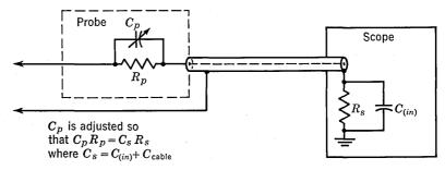
Fig. 5.39. Probe compensation circuit.
