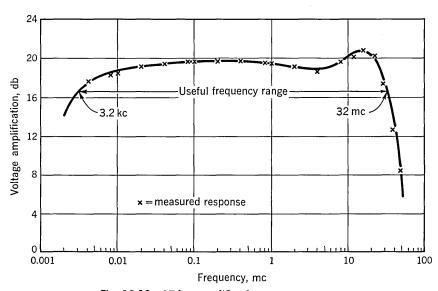
Fig. 19.19. Video amplifier frequency response.
