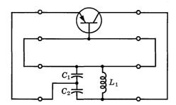
Fig. 22.3. The Colpitts type circuit.
