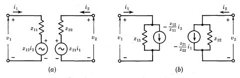
Fig. 6.8. z-parameter equivalent circuit.
