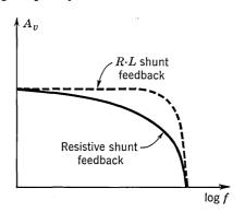
Fig. 19.17.  $A_V$  vs. frequency: resistive feedback.
