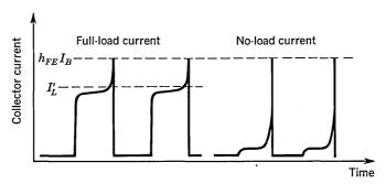
Fig. 34.6. Single-transformer converter: typical collector currents.
