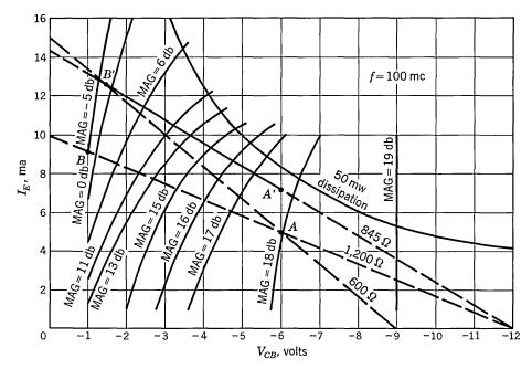
Fig. 24.8. 100-mc MAG curves for variation in operating point.
