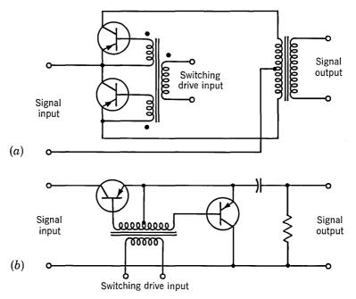
Fig. 10.6. Simple transistor-chopper circuits.
