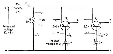
Fig. 35.7. Equivalent oscillator bias circuit.
