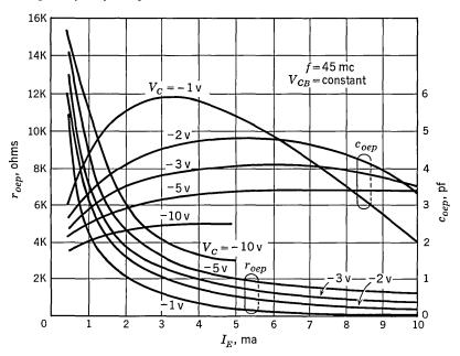
Fig. 24.13. Parallel component of output resistance and capacitance (common emitter) vs. emitter current (at  $f=45~{\rm mc}$ ).
