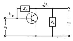
Fig. 19.3. Shunt feedback equivalent circuit.
