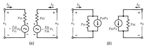
Fig. 6.9. y-parameter equivalent circuit.
