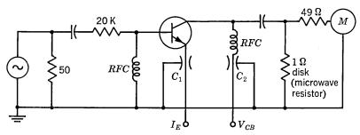
Fig. 5.21. High-frequency  $h_{fe}$  test set.
