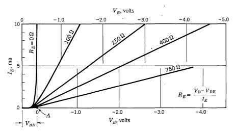
Fig. 24.18. D-c transconductance linearization.
