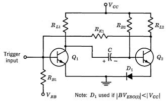
Fig. 28.8. Basic monostable multivibrator.
