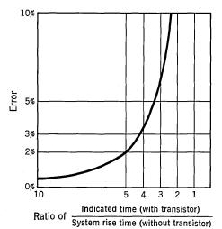
Fig. 5.30. Test system error.
