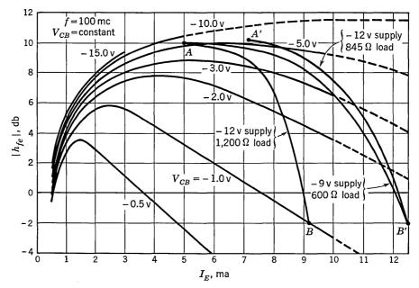
Fig. 24.3.  $h_{fe}$  vs.  $I_E$  (at f = 100 mc).
