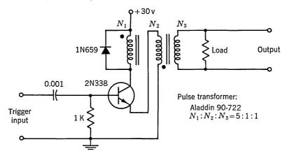
Fig. 33.3. Common-base blocking oscillator.
