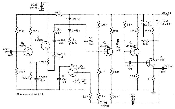
Fig. 11.6. Low-noise low-level amplifier.
