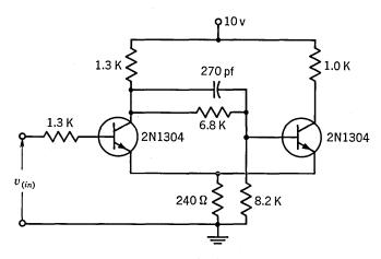
Fig. 28.11. Typical Schmitt trigger.
