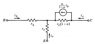
Fig. 6.11. T-equivalent circuit, common emitter.
