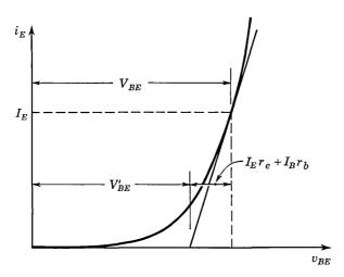
Fig. 8.2. Emitter-base diode forward characteristic.
