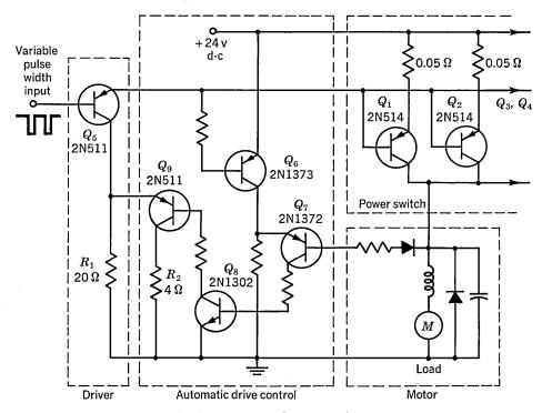
Fig. 37.4. Automatic drive-control circuit.
