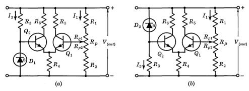
Fig. 9.7. Differential amplifier comparison elements with sampling and reference elements: (a) low output voltage; (b) high output voltage.
