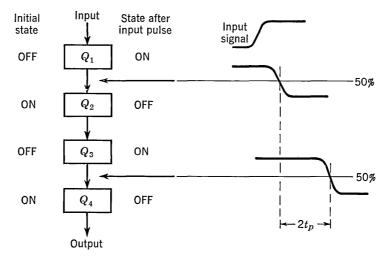
Fig. 4.30. Block diagram showing propagation time.
