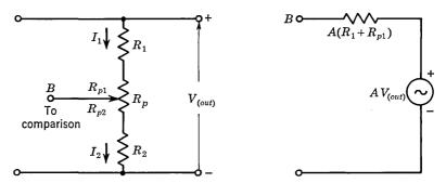
Fig. 9.2. Sampling element and its Thévenin equivalent circuit.
