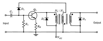
Fig. 33.1. Common-emitter triggered blocking oscillator.
