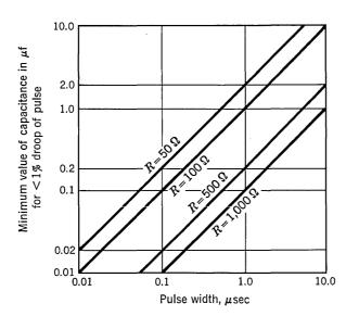
Fig. 5.35. Minimum value for coupling capacitor.
