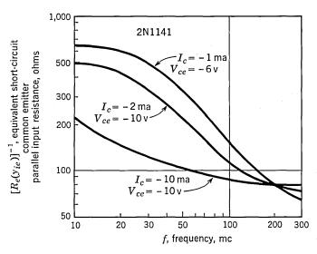
Fig. 4.23. Equivalent short-circuit common-emitter parallel input resistance vs. frequency.
