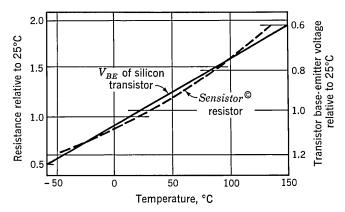
Fig. 8.20. Temperature characteristics of silicon resistor element.
