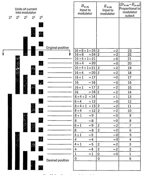
Fig. 39.8. Operation of demodulator.
