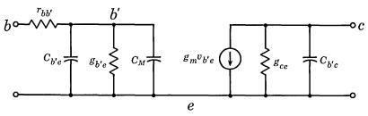
Fig. 4.13. Modified hybrid- $\pi$  circuit.
