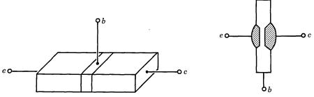
Fig. 1.2. Grown-junction-type transistor.
