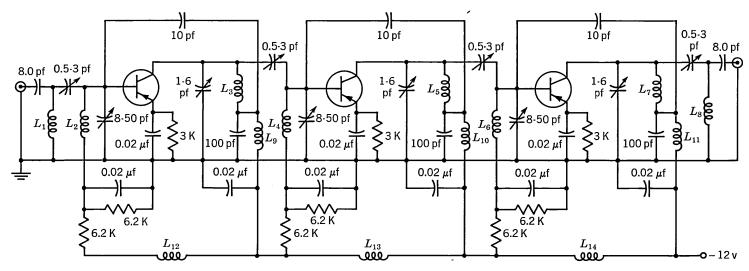
$L_1$ ,  $L_8$  -3.5  $\mu$ h 23 turns #36 heavy Formvar closewound on Cambion LS-9 form  $L_2$ ,  $L_4$ ,  $L_6$ -0.53  $\mu$ h 9 turns #36 heavy Formvar space  $^{1}/_{62}$ " apart on Cambion LS-9 form  $L_3$ ,  $L_5$ ,  $L_7$ -5.3  $\mu$ h 29 turns #36 heavy Formvar closewound on Cambion LS-9 form  $L_9$ - $L_{14}$  -15  $\mu$ h rfc
