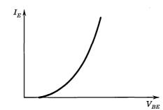
Fig. 23.7. Input diode characteristic curve.
