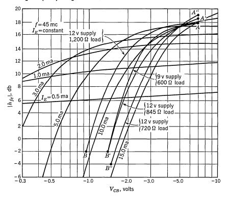
Fig. 24.10.  $h_{fe}$  vs.  $V_{CB}$  (at f = 45 mc).
