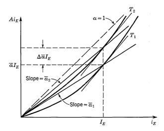
Fig. 8.4. Effect of temperature on collector current generator.
