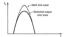
Fig. 17.4. Distortion from  $h_{FE}$  fall-off.
