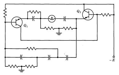
Fig. 12.3. Bridge-type oscillator.
