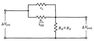
Fig. 9.20. A voltage divider used to determine F.
