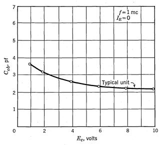
Fig. 4.16.  $C_{ob}$  vs.  $E_C$ : types 2N1141, 2N1142, and 2N1143.
