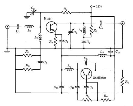
Fig. 23.4. Circuit configuration of mixer design example.
