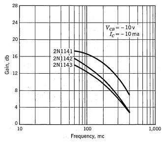
Fig. 20.5. Common-base unilateralized RF power gain.
