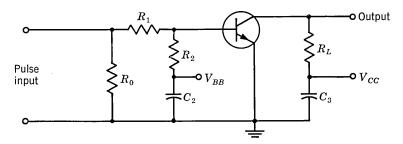
Fig. 5.37. Bypass capacitors.
