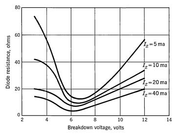
Fig. 9.4. D-c diode resistance vs. breakdown voltage: 1N746 series.
