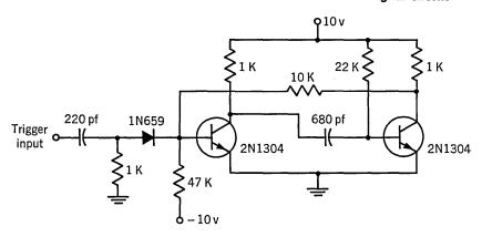
Fig. 28.9.  $10-\mu$ sec monostable multivibrator.
