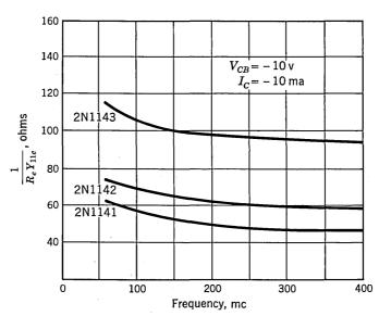
Fig. 20.20. Parallel input resistance common emitter vs. frequency.
