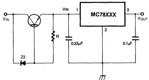
$$V_{IN} = V_I - (V_Z + V_{BE})$$
