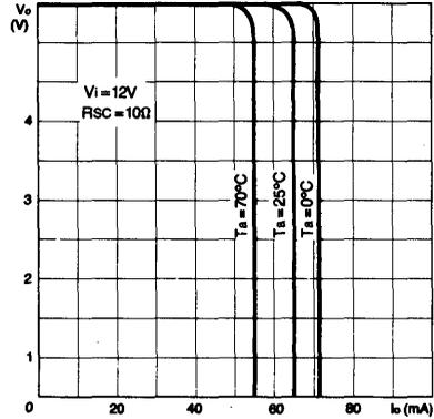
Fig. 10 LOAD REGULATION CHARACTERISTICS WITHOUT CURRENT LIMITING
