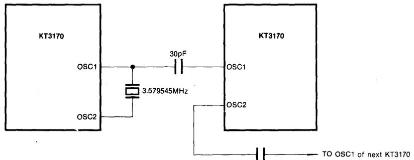
Fig. 4 Oscillator Connection
