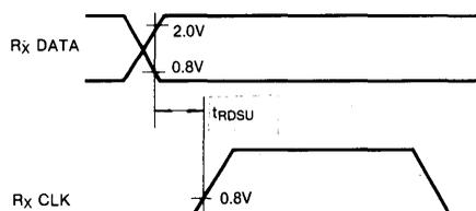
Fig. 4 Receive Data Setup Time (+1 Mode)
