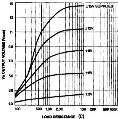
Fig. 8 NEGATIVE OUTPUT VOLTAGE SWING vs LOAD RESISTANCE
