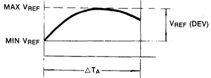
where  $\Delta T_A$  is the rated operating free-air temperature range of the device.
