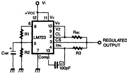
Note:  $R3 = R1 \cdot R2 / (R1 + R2)$  for minimum temperature drift.
