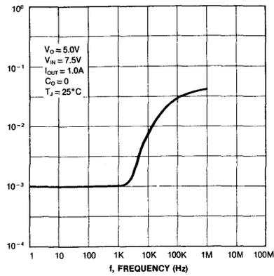
Fig. 3 RIPPLE REJECTION  $V_S$  FREQUENCY
