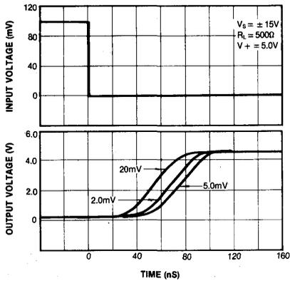
Fig. 8 RESPONSE TIME FOR VARIOUS INPUT OVERDRIVER
