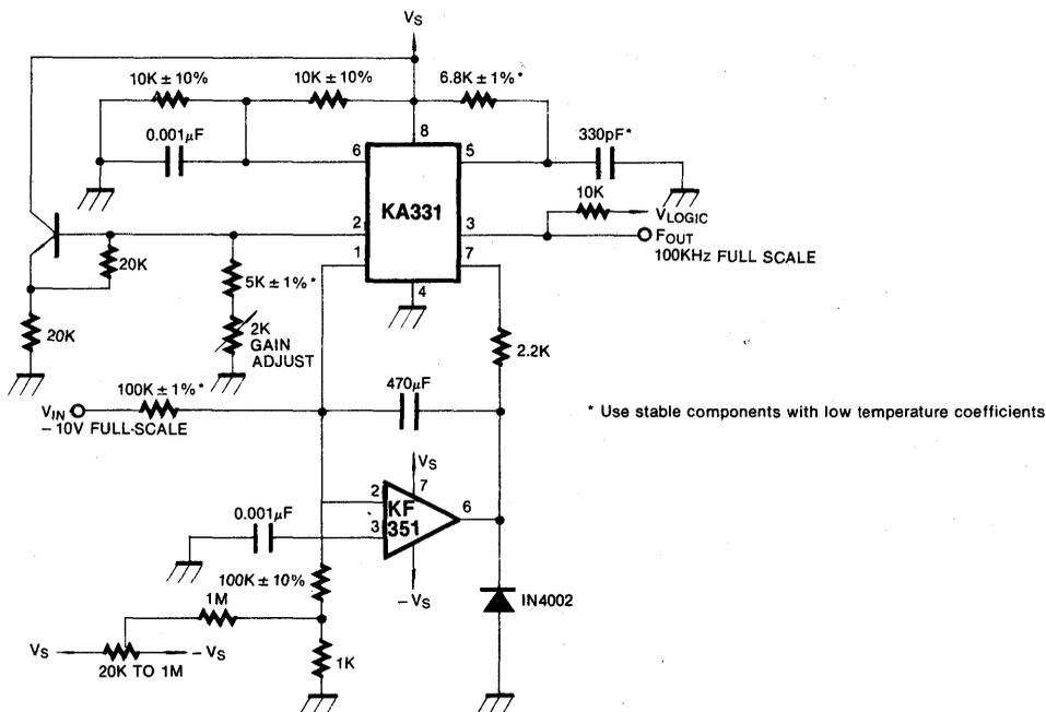
Fig. 2 Simple Frequency-to-Voltage Converter, 10KHz Full-Scale
