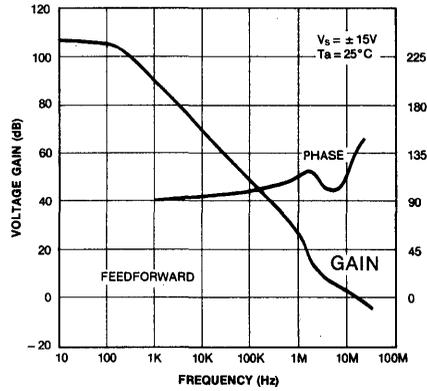
Fig. 17 LARGE SIGNAL FREQUENCY RESPONSE
