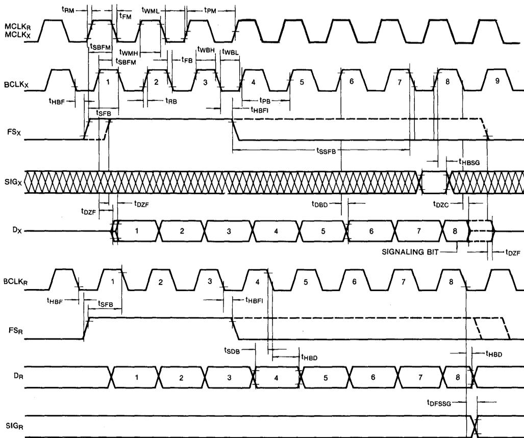
Fig. 3 Long Frame Sync Timing
