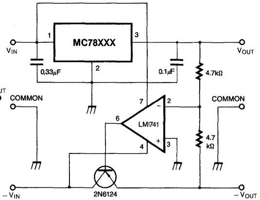
Fig. 14 Split Power Supply ( $\pm 15V - 1A$ )
