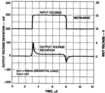
Fig. 7 LOAD TRANSIENT RESPONSE
