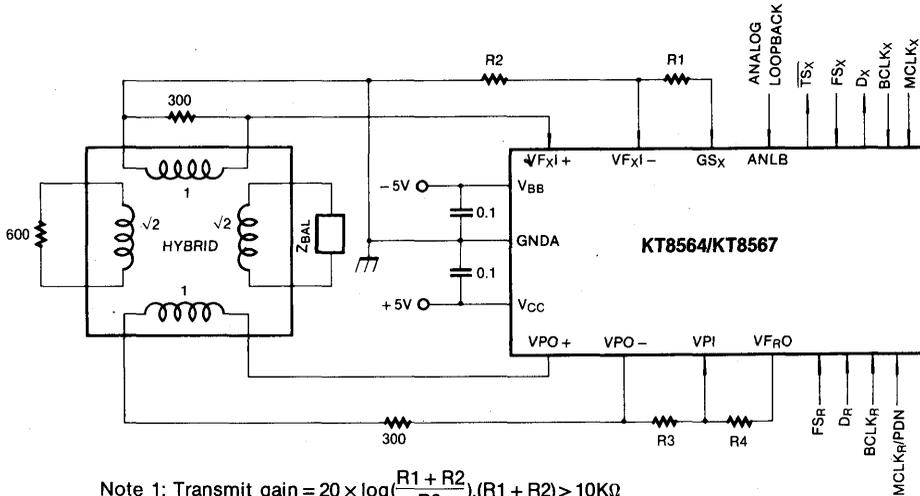
Note 1: Transmit gain =  $20 \times \log\left(\frac{R1 + R2}{R2}\right)$ ,  $(R1 + R2) \geq 10K\Omega$
