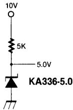
Fig. 9 5.0V REFERENCE WITH MINIMUM TEMPERATURE COEFFICIENT
