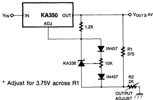
Fig. 16 ADJUSTABLE REGULATOR WITH IMPROVED RIPPLE REJECTION
