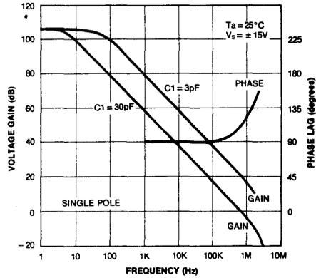
Fig. 9 LARGE SIGNAL FREQUENCY RESPONSE
