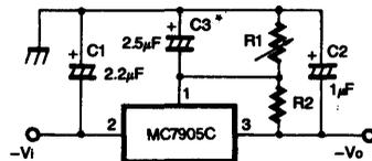
$$V_o = V_{XX} \cdot \frac{R_1 + R_2}{R_2}$$
