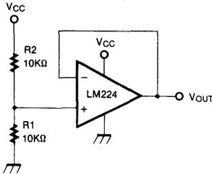
Fig. 14 Non-Inverting DC Gain
