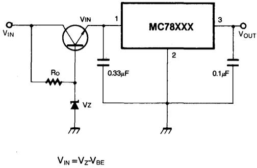
Fig. 19 High Output Voltage Regulator
