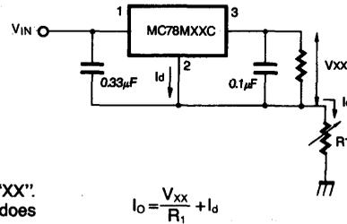
Fig. 3 Circuit for increasing output voltage
