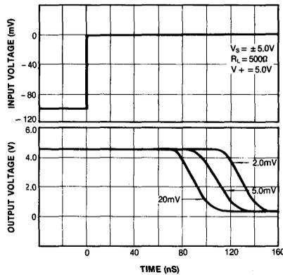
Fig. 5 RESPONSE TIME FOR VARIOUS INPUT OVERDRIVER
