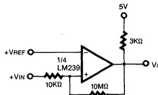
Fig. 8 Inverting comparator with Hysteresis
