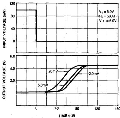
Fig. 6 INPUT CHARACTERISTICS
