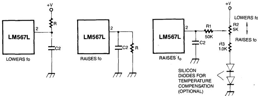
Fig. 7. Detection Band Skew Adjustment
