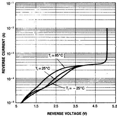
Fig. 6 TEMPERATURE DRIFT
