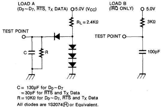
Fig. 9 Bus Timing Test Loads
