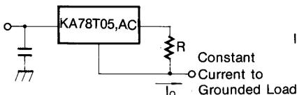
The KA78T05 regulator can also be used as a current source when connected as above. In order to minimize dissipation, the KA78T05 is chosen in this application. Resistor R determines the current as follows:
