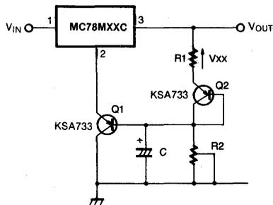
Note: Q2 is connected as a diode in order to compensate the variation of the Q1 V<sub>BE</sub> with the temperature. C allows a slow rise-time of the V<sub>o</sub>
