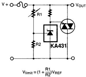
FIGURE 17—OVER-VOLTAGE/UNDER-VOLTAGE PROTECTION CIRCUIT
