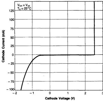
Fig. 5 CATHODE CURRENT VS CATHODE VOLTAGE
