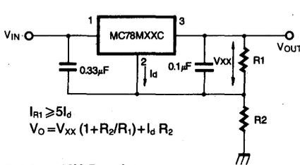
Fig. 4 Adjustable output regulator (7 to 30V)
