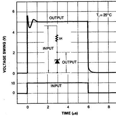
Fig. 5 REVERSE CHARACTERISTICS
