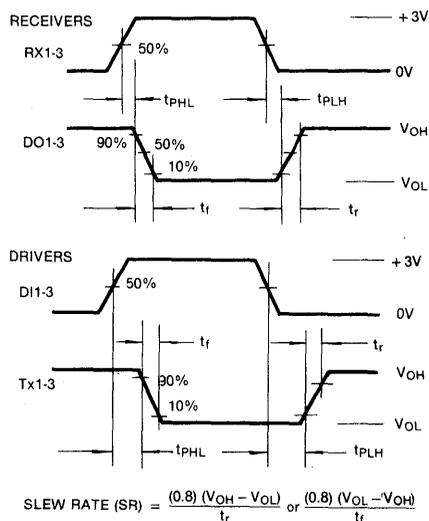
Fig. 2 Switching Characteristics
