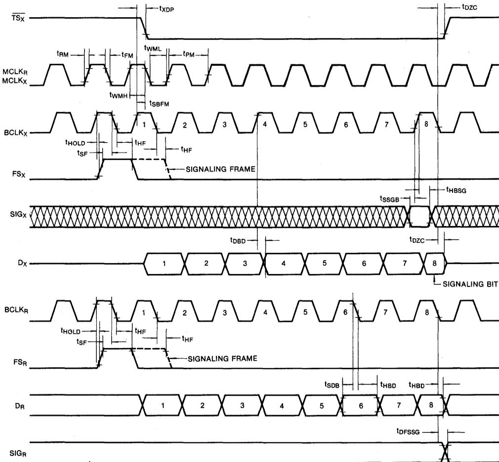
Fig. 2. Short Frame Sync Timing
