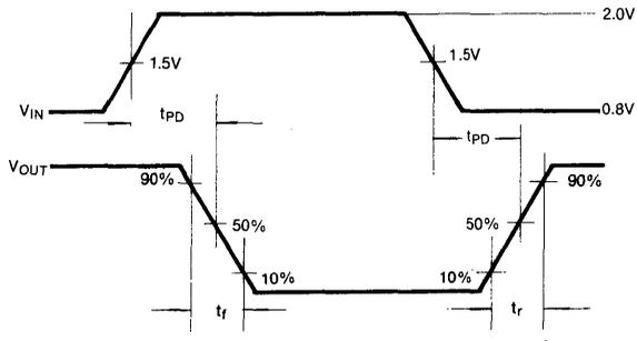
Fig. 2 Switching Waveforms
