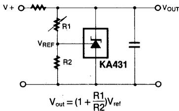
FIGURE 12—SINGLE-SUPPLY COMPARATOR WITH TEMPERATURE-COMPENSATED THRESHOLD
