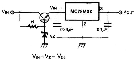
Fig. 10 Reducing power dissipation with dropping resistor
