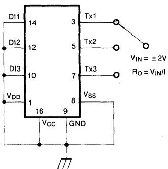
Fig. 1 Power Off Source Resistance
