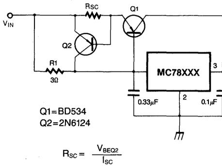
Fig. 13 Tracking Voltage Regulator
