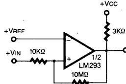
**Fig. 8 Inverting comparator with Hysteresis**
