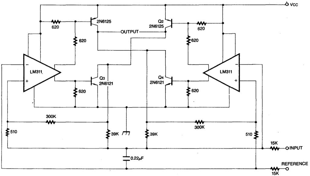
Fig. 2 | Relay Driver with Strobe
