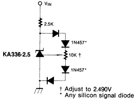
Fig. 7 Trimmed 4V to 6V reference with temperature coefficient of breakdown voltage independent
