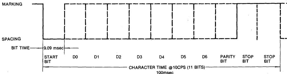
Fig. 10 110 Baud Serial ASCII Data Timing
