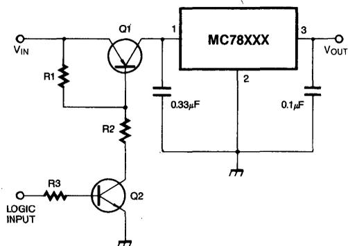
Fig. 23 Power AM Modulator
