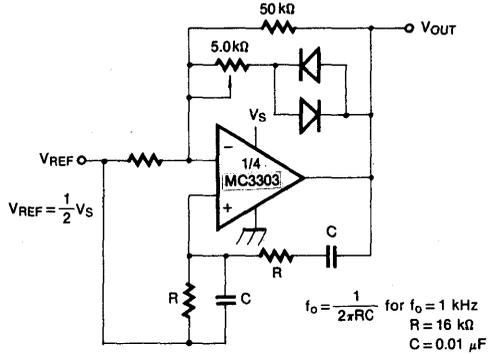
$$f_o = \frac{1}{2\pi RC} \text{ for } f_o = 1 \text{ kHz}$$
