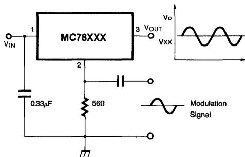
Note: The circuit performs well up to 100 KHz.
