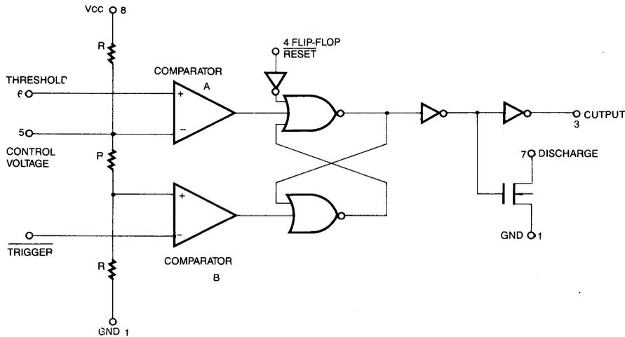
This block diagram reduces the circuitry down to its simplest equivalent components. Tie down unused inputs.
