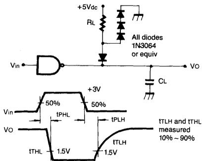
$C_L = 15\text{pF}$  = total parasitic capacitance, which includes probe and wiring capacitances
