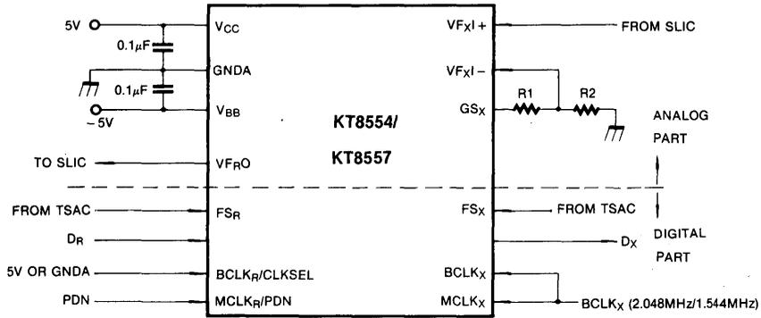
Note: XMIT gain =  $20 \times \log\left(\frac{R1 + R2}{R2}\right)$ ,  $(R1 + R2) > 10K\Omega$ .
