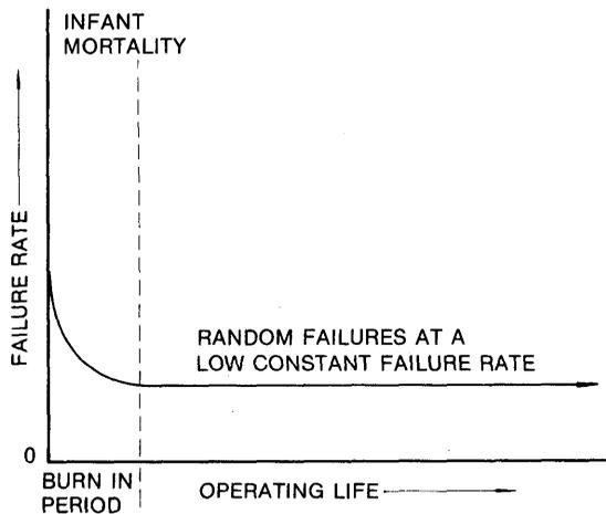
Reliability theory assumes that devices fail according to the above curve. When a group of devices is manufactured a small portion of the units will be inherently weaker than the average. These weak units will probably fail during the first few hours of operation—hence the term "infant mortality." If the units are burned-in however, thereby allowing the weak units to fail, there is a much lower probability that those finally put into system use will fail.
