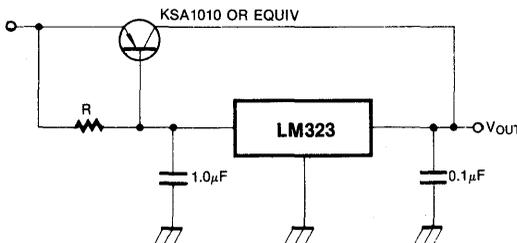
The LM323 can be current boosted with a PNP transistor. The KSA1010 provides current to 15 amperes. Resistor R in conjunction with the V<sub>BE</sub> of the PNP determines when the pass transistor begins conducting; this circuit is not short-circuit proof. Input-output differential voltage minimum is increased by the V<sub>BE</sub> of the pass transistor.
