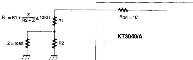
Receive Filter Output Gain Adjustment
