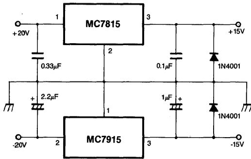
Fig. 15 Negative Output Voltage Circuit
