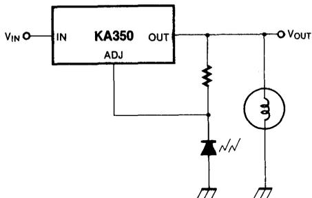
Fig. 15 PRECISION POWER REGULATOR WITH LOW TEMPERATURE COEFFICIENT
