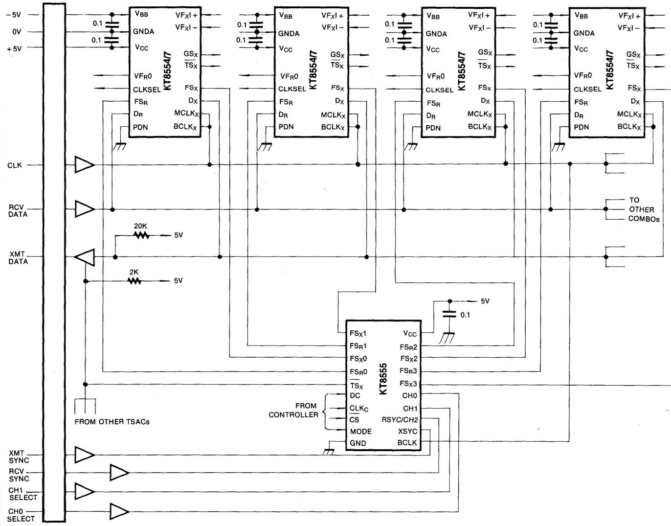
Fig. 3 Digital Interconnections on a Typical Synchronous Line Board
