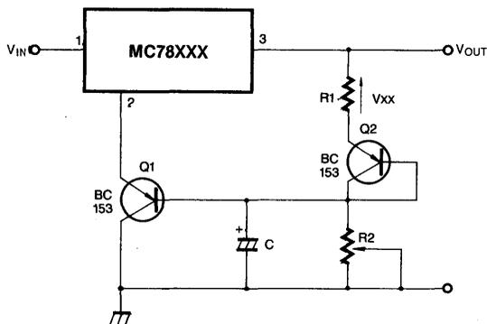
Note: Q2 is connected as a diode in order to compensate the variation of the Q1 V<sub>BE</sub> with the temperature. C allows a slow rise-time of the V<sub>o</sub>
