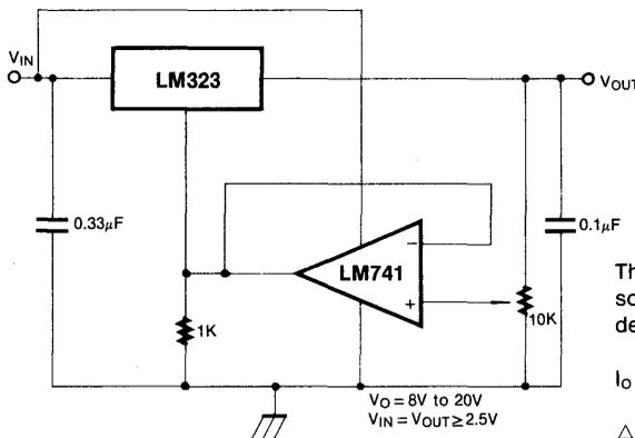
The addition of an operational amplifier allows adjustment to higher or intermediate values while retaining regulation characteristics. The minimum voltage obtainable with this arrangement is 3.0 volts greater than the regulator voltage.
