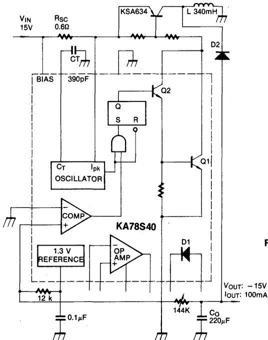
Fig. 4. Typical inverting operation ( $T_a = 25^\circ\text{C}$ )
