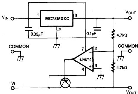
Fig. 9 High input voltage circuit
