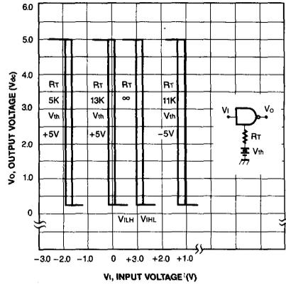
Fig. 7 — MC1489A INPUT THRESHOLD VOLTAGE ADJUSTMENT
