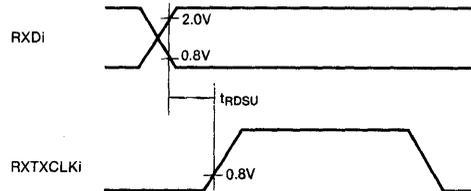
Fig. 4 Receive Data Setup Time (+1 Mode)
