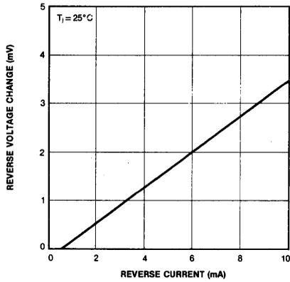
Fig. 2 REVERSE CHARACTERISTICS
