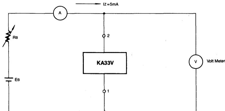
Fig. 2 Measuring Circuit for Dynamic Resistance
