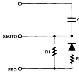
$$t_{GTP} = (RpC) \ln(V_{DD}/V_{DD} - V_{TST})$$
