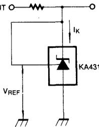
**Fig. 2 Test Circuit for  $V_{KA} \geq V_{REF}$**
