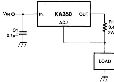
Fig. 26 ADJUSTING MULTIPLE ON-CARD REGULATORS WITH SINGLE CONTROL\*
