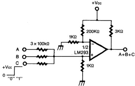
Fig. 13 Large fan-in AND gate
