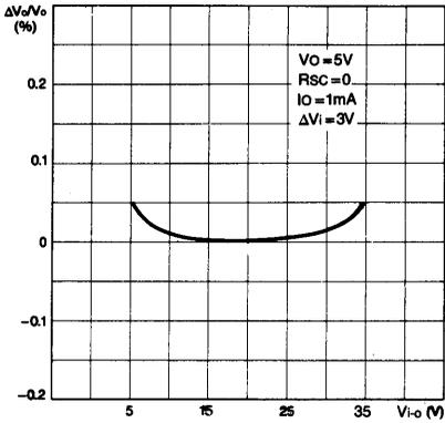
Fig. 14 LOAD REGULATION—VOLTAGE DROP
