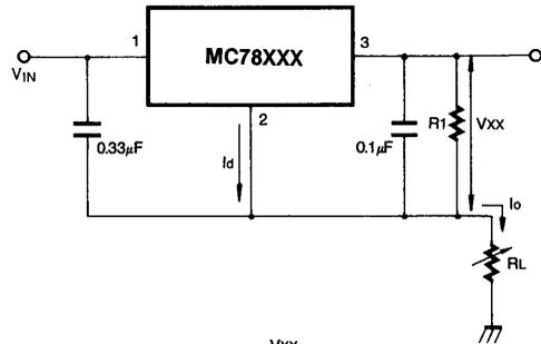
$$I_o = \frac{V_{XX}}{R_1} + I_d$$
