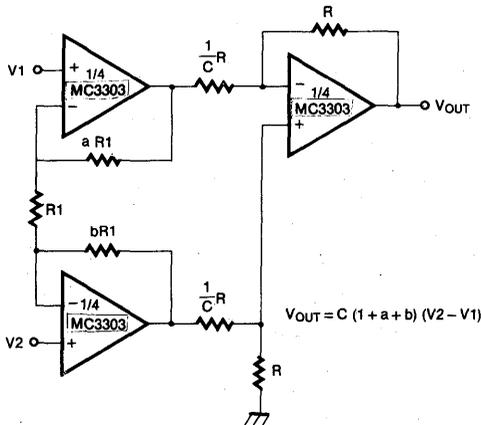
$$V_{OUT} = C(1 + a + b)(V_2 - V_1)$$
