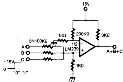
Fig. 13 Large fan-in AND gate
