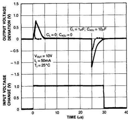
Fig. 10 LOAD TRANSIENT RESPONSE
