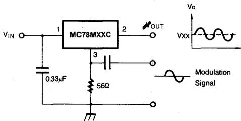
Note: The circuit performs well up to 100 KHz.
