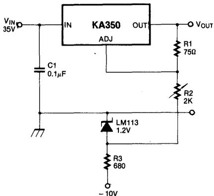
Fig. 19 5V LOGIC REGULATOR WITH ELECTRONIC SHUTDOWN\*
