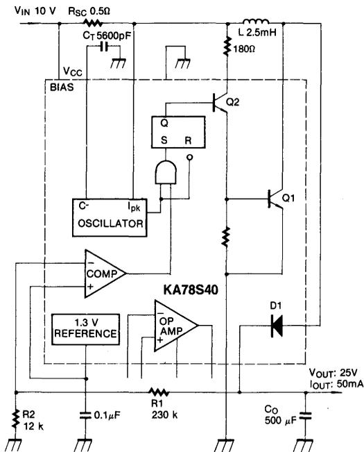
Fig. 3. Typical step-up operation ( $T_a = 25^\circ\text{C}$ )
