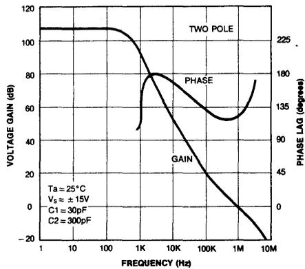
Fig. 13 LARGE SIGNAL FREQUENCY RESPONSE
