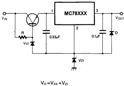
Fig. 21 Reducing Power Dissipation with Dropping Resistor
