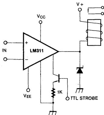
Fig. 3 | Digital Transmission Isolator
