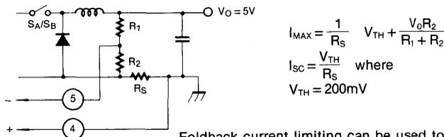
Foldback current limiting can be used to reduce power dissipation under shorted output conditions
