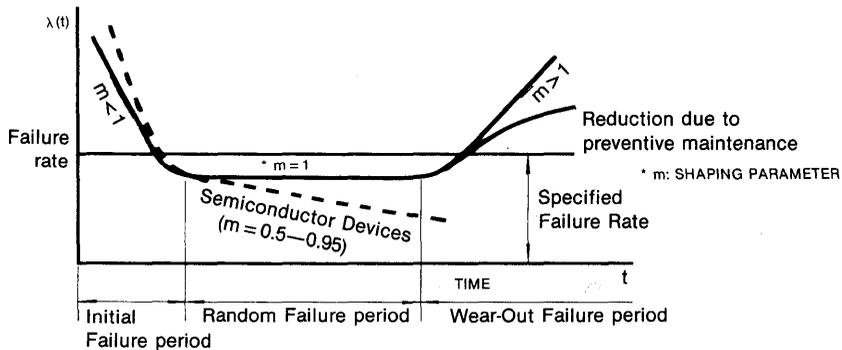
Figure 3. Failure Rate Curve ("Bath Tub Curve")
