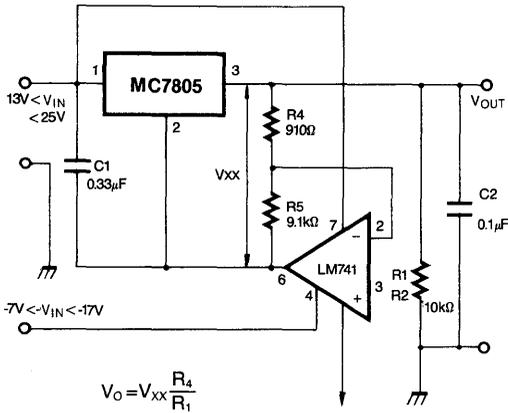
Fig. 11 High Current Voltage Regulator
