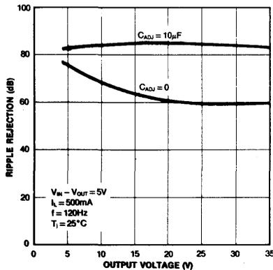
Fig. 6 RIPPLE REJECTION
