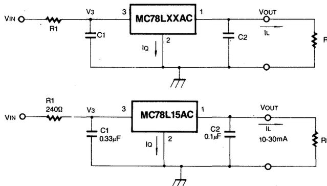
When it is necessary to operate a MC78LXXAC regulator with a large input-output differential voltage, the addition of series resistor R1 will extend the output current range of the device by sharing the total power dissipation between R1 and the regulator.
