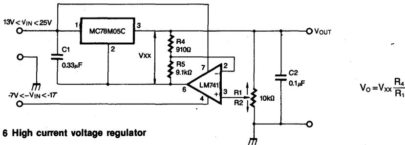
Fig. 6 High current voltage regulator
