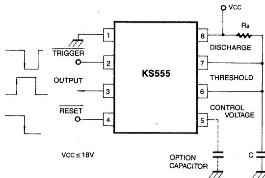
Fig. 3. Monostable Operation
