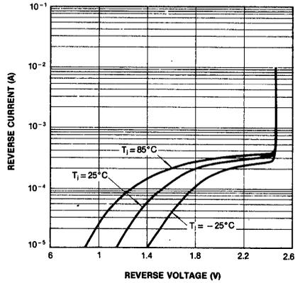
Fig. 3 TEMPERATURE DRIFT
