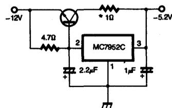
\* Optional dropping resistor to reduce the power dissipated in the boost transistor.
