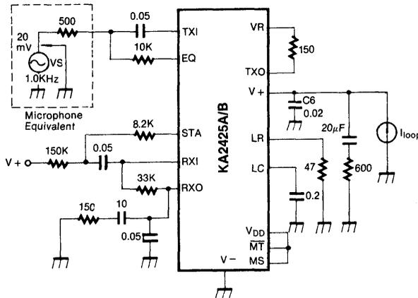
Fig. 4 AC Impedance, Receive and Sidetone Cancellation Test
