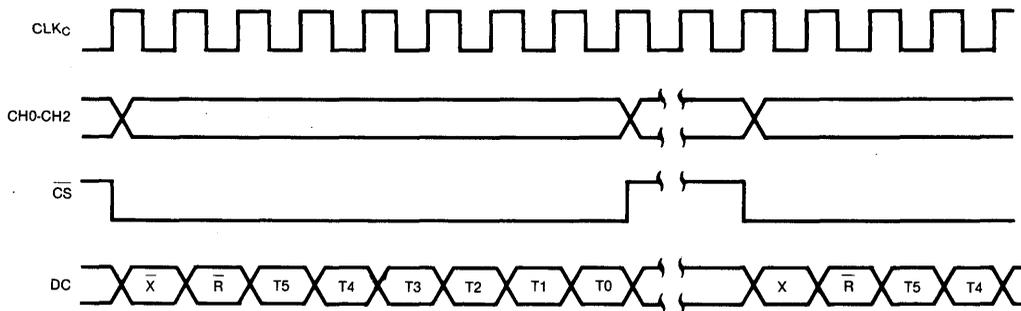
**Fig. 2 Control Data Timing**
