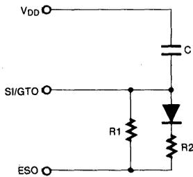
$$t_{GTP} = (R1C) \ln(V_{DD}/V_{DD} - V_{TST})$$
