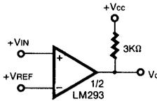
**Fig. 7 Non-inverting comparator with Hysteresis**
