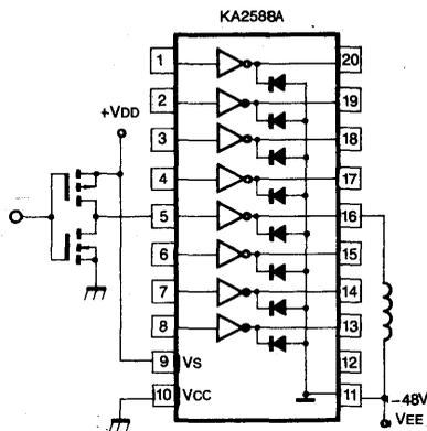
Telecommunication Relay Driver (Positive Logic)
