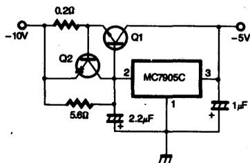
Fig. 5 — Typical ECL system power supply (-5.2V/4A)
