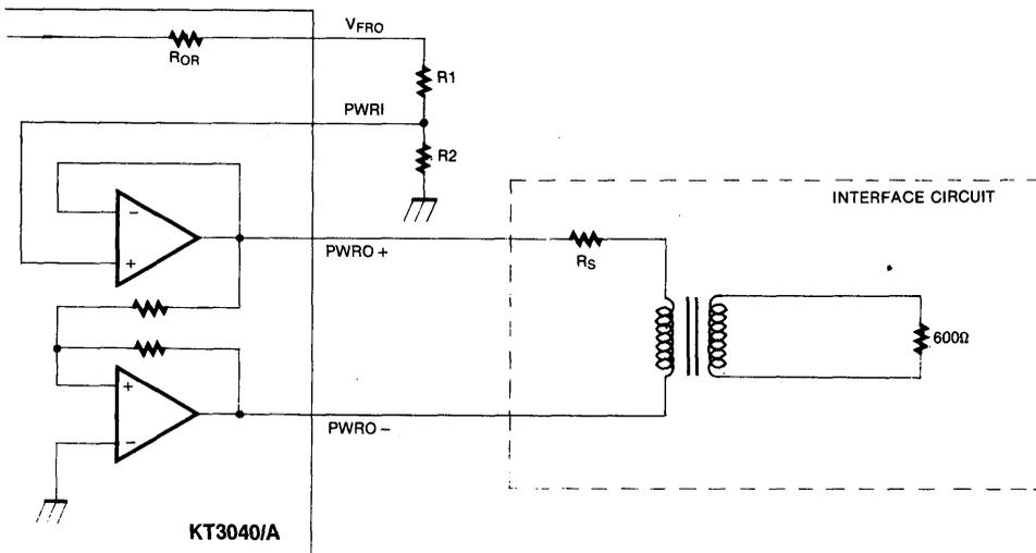
Typical Connection of Output Driver Amp
