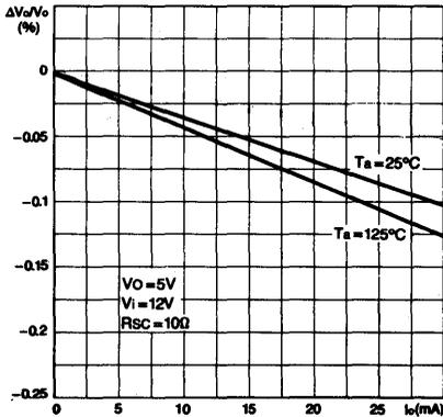
Fig. 8 CURRENT LIMITING CHARACTERISTICS
