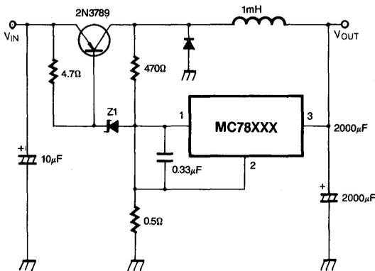
Fig. 17 High Input Voltage Circuit
