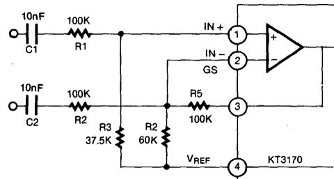
$$R3 = R2R5 / (R2 + R5), \text{ VOLTAGE GAIN} = R5/R1$$
