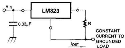
The LM323 regulator can also be used as a current source when connected as above. Resistor R determines the current as follows:
