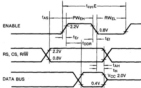
Fig. 7 Bus Read Timing Characteristics (Read information from UART)
