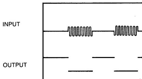
Response to 100mV<sub>rms</sub> tone burst.  $R_L = 1K\Omega$
