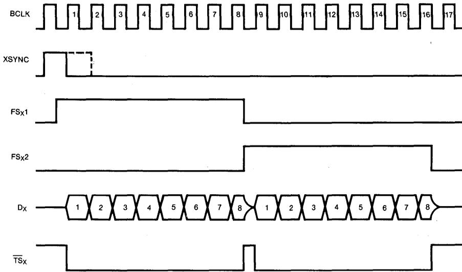
**Fig. 1 Transmit Data Timing**
