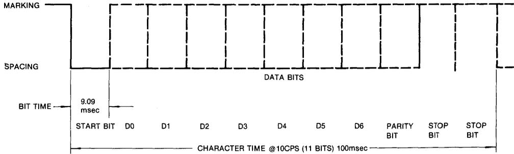
Fig. 10 110 Baud Serial ASCII Data Timing
