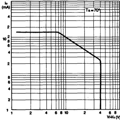
Fig. 9 CURRENT LIMITING CHARACTERISTICS VS. JUNCTION TEMPERATURE
