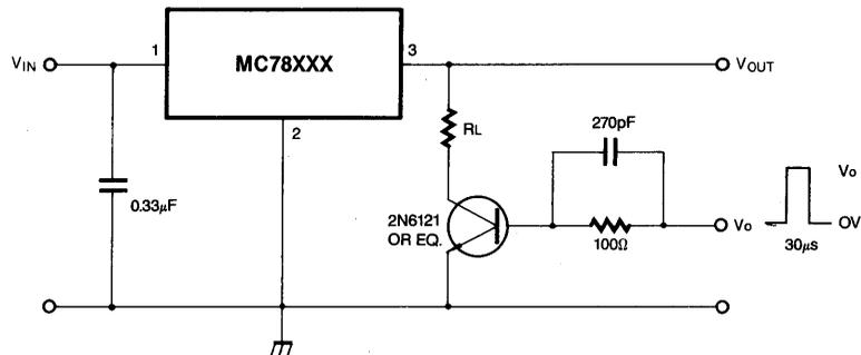
Fig. 5 Ripple Rejection
