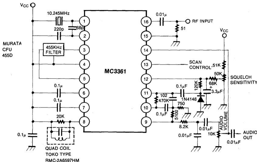
In the above typical application, the audio signal is recovered using a conventional quadrature FM detector. The absence of an input signal is indicated by the presence of noise above the desired audio frequencies. This "noise band" is monitored by an active filter and a detector. A squelch trigger circuit indicates the presence of noise (or a tone) by an output which can be used to control scanning. At the same time, an internal switch is operated which can be used to mute the audio.
