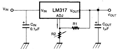
$$V_{OUT} = 1.25V (1 + \frac{R_2}{R_1}) + I_{adj} R_2$$
