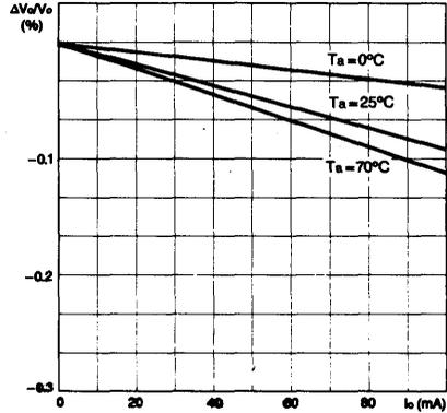
Fig. 12 LOAD REGULATION CHARACTERISTIC WITH CURRENT LIMITING
