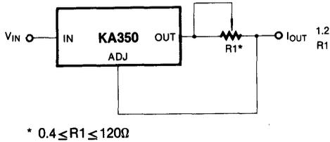
Fig. 21 1.2V - 20V REGULATOR WITH MINIMUM PROGRAM CURRENT
