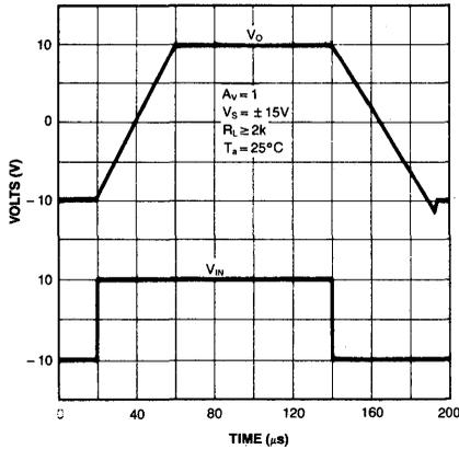
Fig. 10 SMALL SIGNAL PULSE RESPONSE
