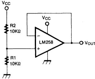
Fig. 14 Non-Inverting DC Gain
