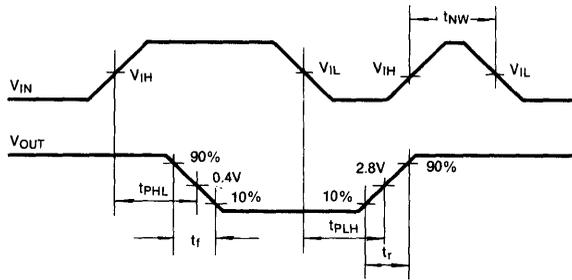
Fig. 2 Switching Waveforms
