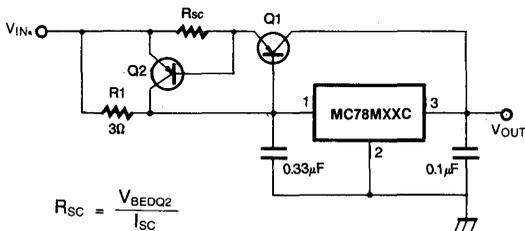
Fig. 8 Tracking voltage regulator
