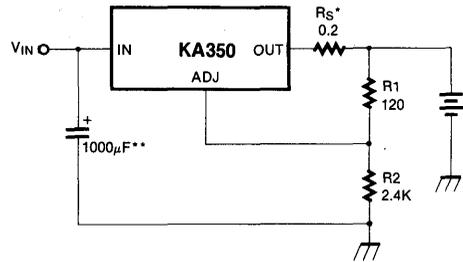
\*  $R_s$  – sets output impedance of charger  $Z_{OUT} = R_s (1 + \frac{R_2}{R_1})$
