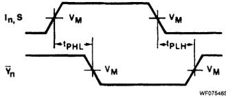
Waveform 1. Propagation Delay Data ( $I_n$ ), Select (S) To Output ( $Y_n$ )
