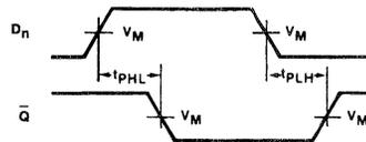
**Waveform 6. Data To Output Delays**
