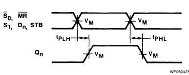
Waveform 1. Propagation Delay For Non-Inverting Outputs
