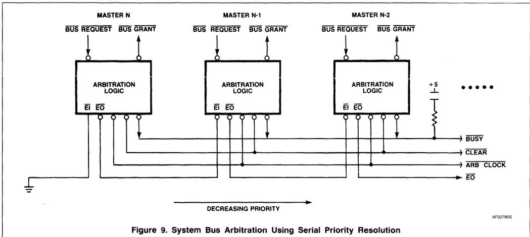
Figure 9. System Bus Arbitration Using Serial Priority Resolution
