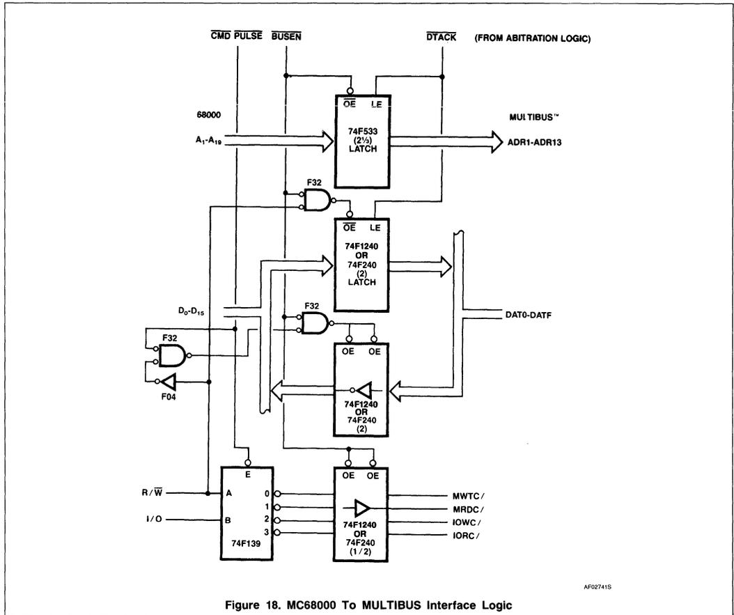
Figure 18. MC68000 To MULTIBUS Interface Logic
