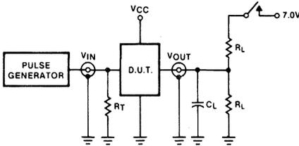
Test Circuit For 3-State Outputs ('F630)
