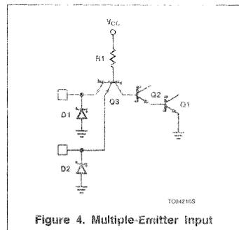
Figure 4. Multiple-Emitter Input
