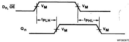
Waveform 1. Propagation Delay For Data To Output
