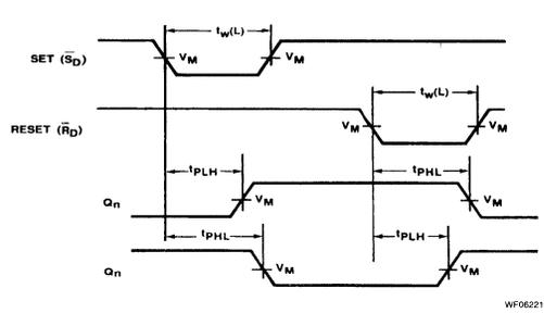
Waveform 2. Set And Reset To Output Delays, Set And Reset Pulse Widths
