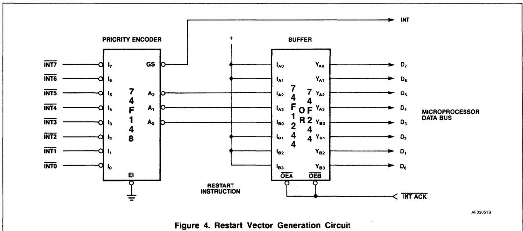
Figure 4. Restart Vector Generation Circuit
