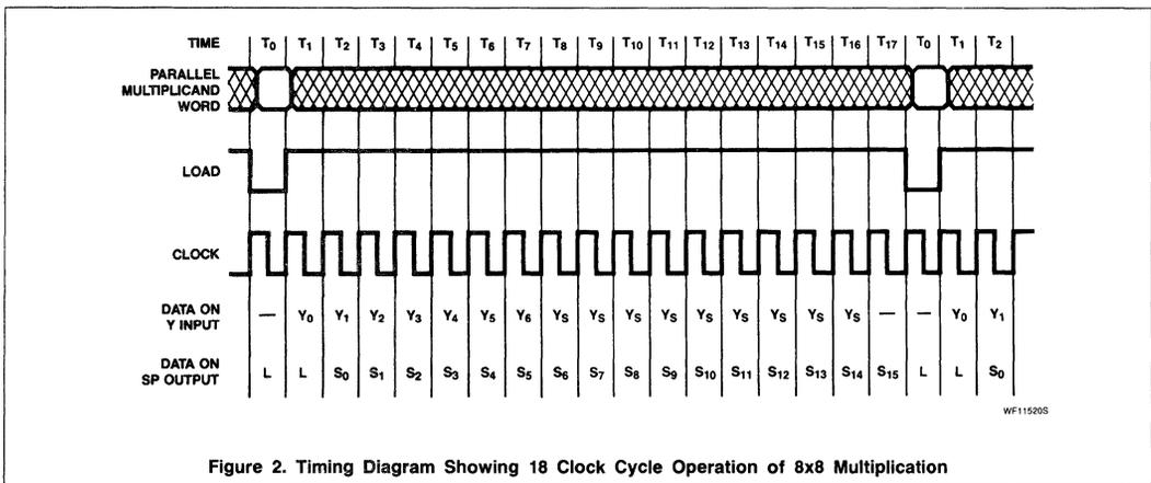
Figure 2. Timing Diagram Showing 18 Clock Cycle Operation of 8x8 Multiplication
