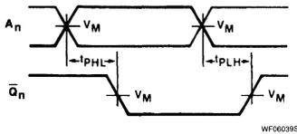
Waveform 3. Propagation Delay For Output Select Address Input ( $A_n$ ) To Decoder Outputs ( $\overline{Q}_n$ )
