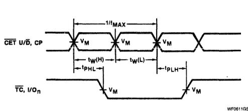
**Waveform 1. Clock To Output Delays, Clock Pulse Width, And Maximum Clock Frequency**
