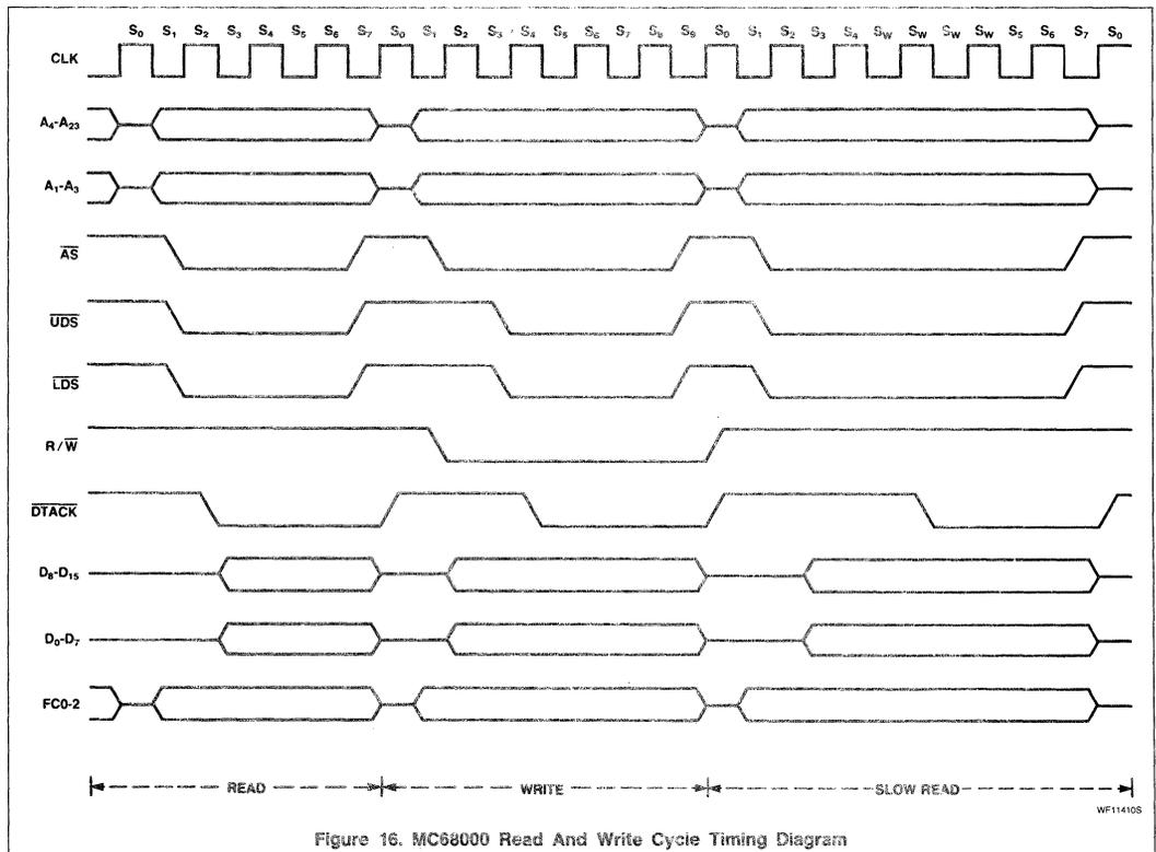
Figure 16. MC68000 Read And Write Cycle Timing Diagram
