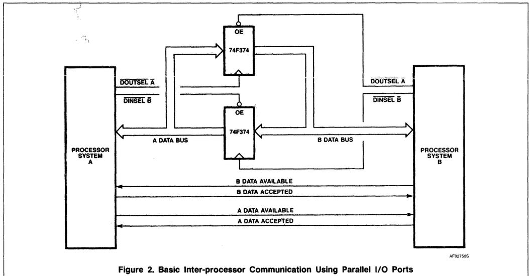
Figure 2. Basic Inter-processor Communication Using Parallel I/O Ports
