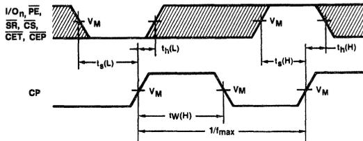
**Waveform 5. Data Set-up And Hold Times**
