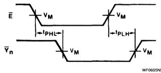
Waveform 4. For Non-Inverting Outputs
