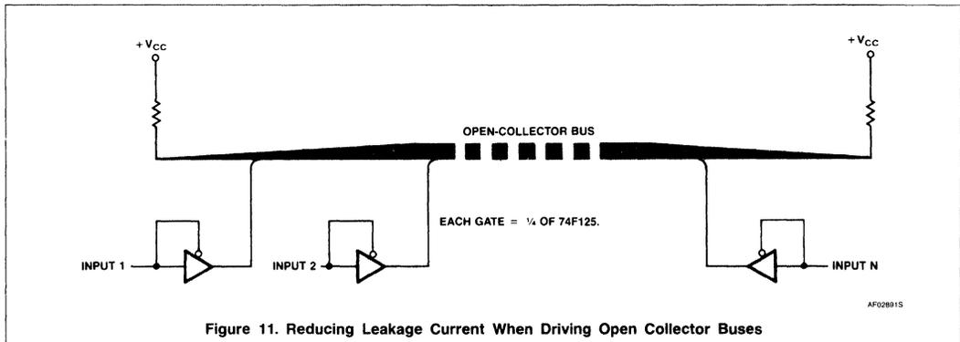
Figure 11. Reducing Leakage Current When Driving Open Collector Buses
