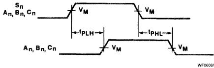
Waveform 1. Propagation Delay Select, Busses To Busses
