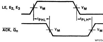
Waveform 1. Propagation Delay For Chip Enable Inputs ( $E_2, E_3$ ) And Latch Enable Input ( $LE$ ) To Write Acknowledge ( $\overline{ACK}$ ) And Decoder ( $\overline{Q}_n$ ) Outputs
