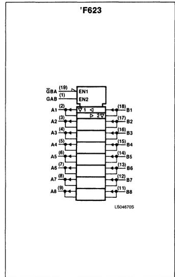
These devices allow data transmission from the A bus to the B bus or from the B bus to the A bus, depending upon the logic levels at the Enable inputs ( $\bar{G}BA$  and  $GAB$ ). The Enable inputs can be used to disable the device so that the buses are effectively isolated.
