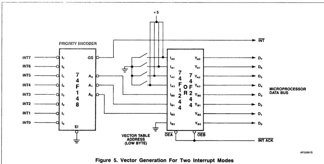
**Figure 5. Vector Generation For Two Interrupt Modes**
