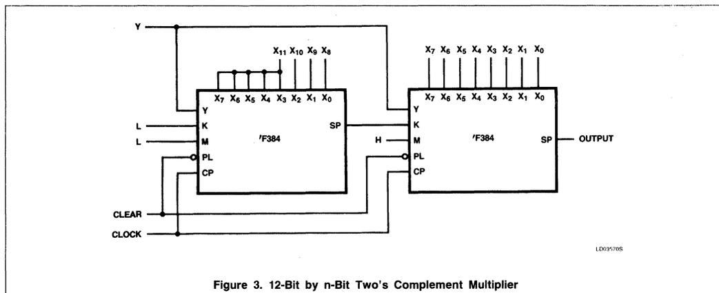
Figure 3. 12-Bit by n-Bit Two's Complement Multiplier
