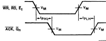
Waveform 2. Propagation Delay For Chip Enable Input ( $E_1$ ) To Decoder Outputs ( $\overline{Q}_n$ ) And Write Acknowledge Inputs ( $\overline{WR}, \overline{RD}$ ) To Acknowledge Output ( $\overline{ACK}$ )
