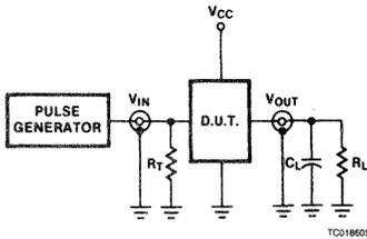
Test Circuit For Totem-Pole Outputs
