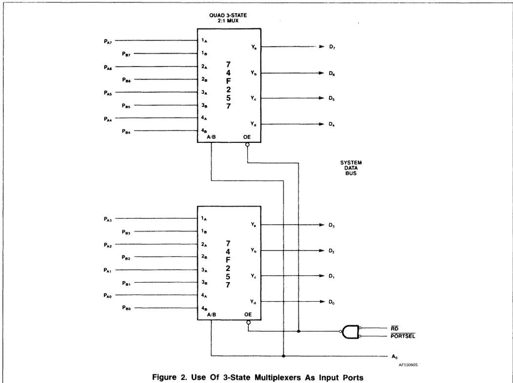
Figure 2. Use Of 3-State Multiplexers As Input Ports
