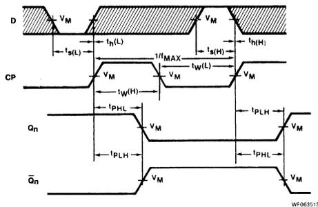
Waveform 1. Clock To Output Delays, Data Set-up And Hold Times, Clock Pulse Width
