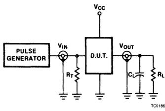
**Test Circuit For Totem-Pole Outputs**
