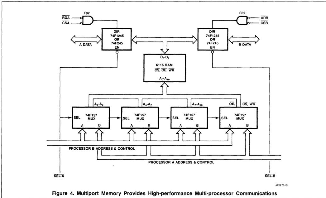
Figure 4. Multiport Memory Provides High-performance Multi-processor Communications
