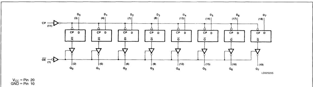
When  $\overline{OE}$  is LOW, the latched or transparent data appears at the outputs. When  $\overline{OE}$  is HIGH, the outputs are in the HIGH impedance "off" state, which means they will neither drive nor load the bus.
