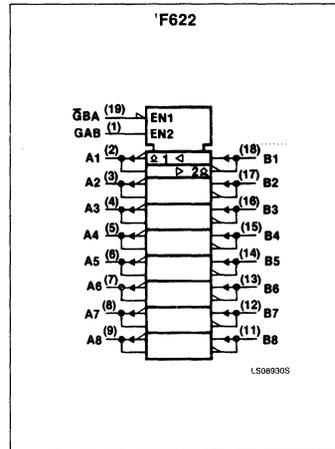
These devices allow data transmission from the A bus to the B bus or from the B bus to the A bus, depending upon the logic levels at the Enable inputs ( $\overline{G}BA$  and  $GAB$ ). The enable inputs can be used to disable the device so that the buses are effectively isolated
