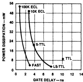
Figure 1. The Speed/Power Spectrum
