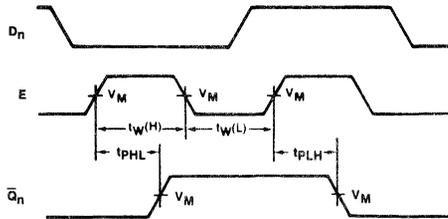
**Waveform 7. Latch Enable To Output Delays**
