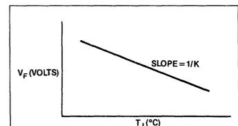
Figure 2. Forward Voltage — Junction Temperature Characteristics of a Semiconductor Junction Operating at a Constant Current. The K Factor is the Reciprocal of the Slope
