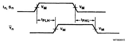
Waveform 2. For Non-Inverting Outputs
