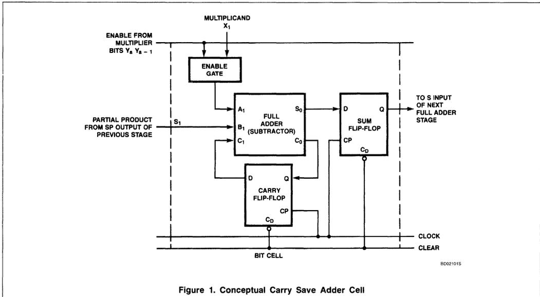
Figure 1. Conceptual Carry Save Adder Cell
