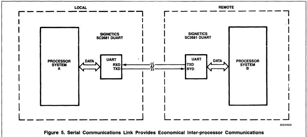
Figure 5. Serial Communications Link Provides Economical Inter-processor Communications
