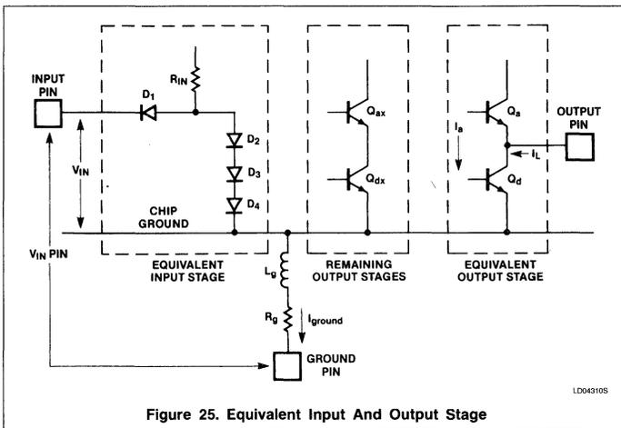
Figure 25. Equivalent Input And Output Stage
