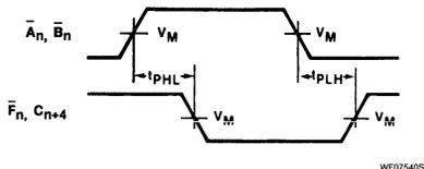
Waveform 1. Propagation Delay For Operands To Carry Output And Outputs
