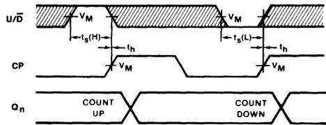
Waveform 6. Up/Down Control Set-up And Hold Times
