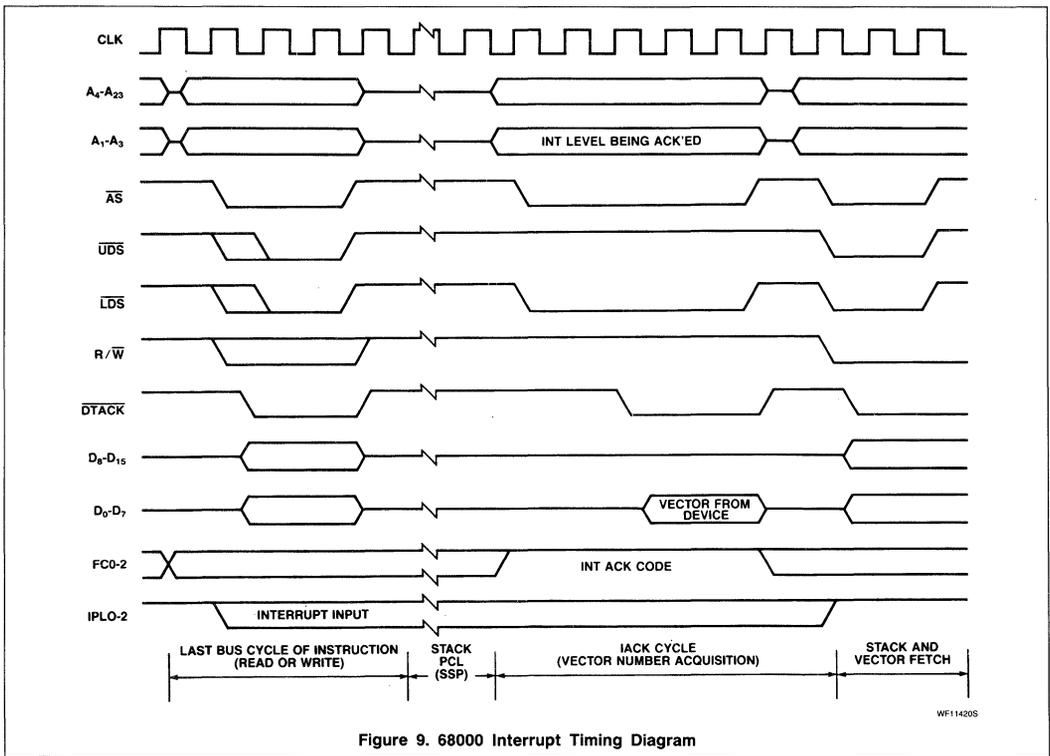
Figure 9. 68000 Interrupt Timing Diagram
