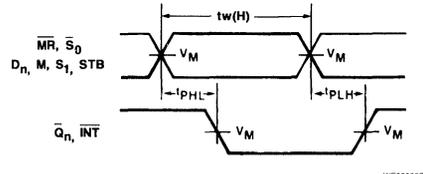
Waveform 2. Propagation Delay For Inverting Outputs Disable Time From HIGH Level
