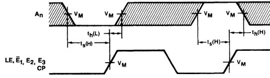
Waveform 4. Data Set-up And Hold Times For Output Select Address Inputs ( $A_n$ ) To Latch Enable Inputs ( $LE$ ) And Chip Enable Inputs ( $\overline{E}_1, \overline{E}_2, \overline{E}_3$ )
