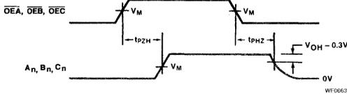
Waveform 3. 3-State Output Enable Time To HIGH Level And Output Disable Time From HIGH Level From HIGH Level
