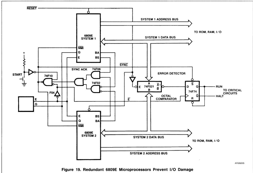
Figure 19. Redundant 6809E Microprocessors Prevent I/O Damage
