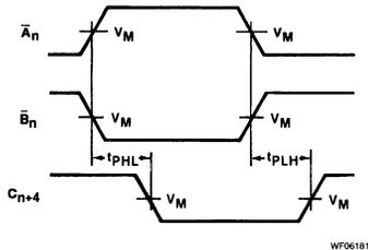
Waveform 4. Propagation Delays For Operands Carry Output
