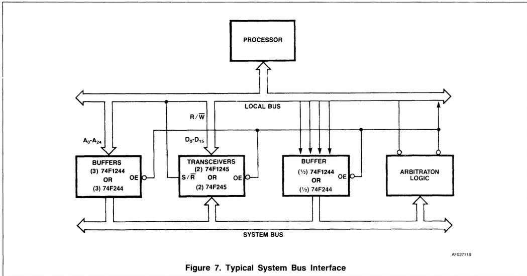
Figure 7. Typical System Bus Interface
