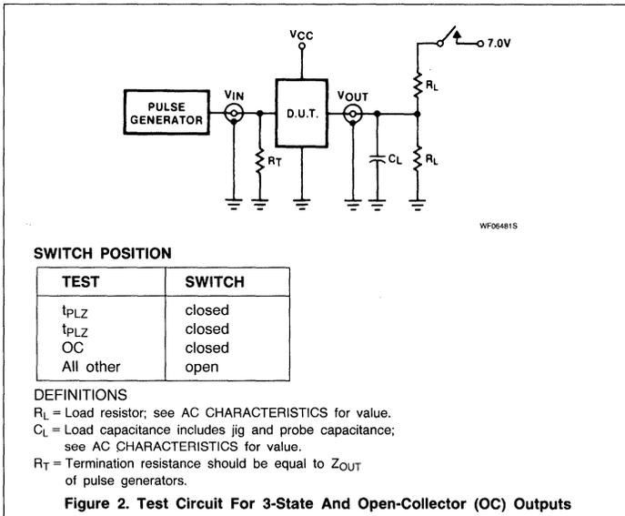
Good, high-frequency wiring practices should be used in constructing test jigs. Leads on the load capacitor should be as short as possible to minimize ripples on the output waveform transitions and to minimize undershoot. Generous ground metal (preferably a ground plane) should be used for the same reasons. A  $V_{CC}$  bypass capacitor should be provided at the test socket, also with minimum lead
