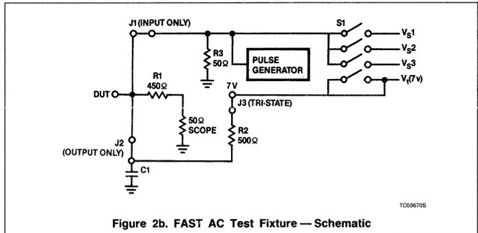
Figure 2b. FAST AC Test Fixture — Schematic
