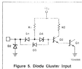
Figure 5. Diode Cluster Input
