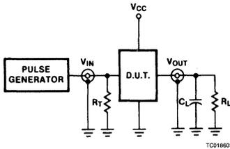
Test Circuit For Totem-Pole Outputs
