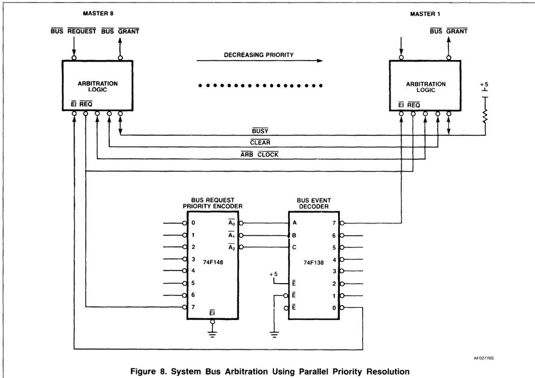
Figure 8. System Bus Arbitration Using Parallel Priority Resolution
