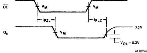
**Waveform 2. 3-State Output Enable Time To LOW Level And Output Disable Time From LOW Level**
