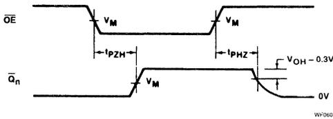
**Waveform 1. 3-State Output Enable Time To HIGH Level And Output Disable Time From HIGH Level**
