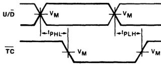
Waveform 3. Propagation Delays U/D Control To Terminal Count Output
