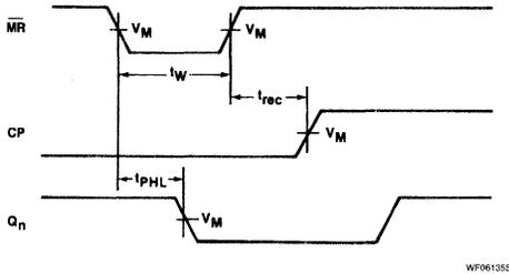
Waveform 3. Master Reset Pulse Width, Master Reset To Output Delay and Master Reset To Clock Recovery Time ('F160A, 'F161A)
