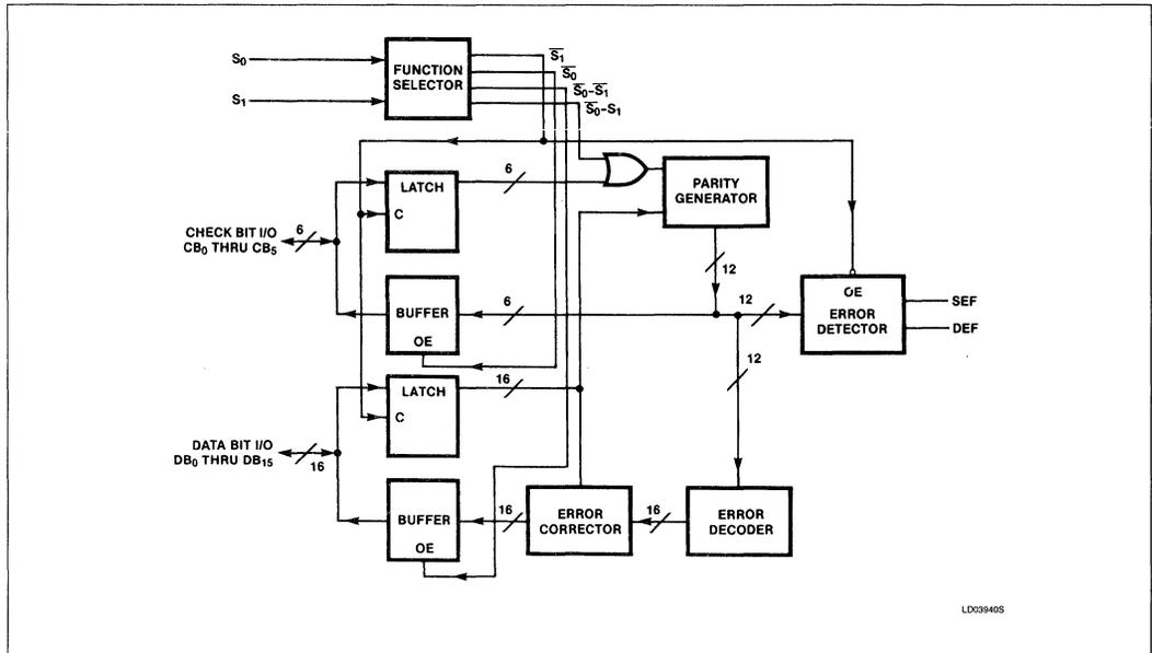
This check word is stored along with the data word during the memory write cycle. During the memory read cycle, the 22-bit words from memory are processed by the EDACs to determine if errors have occurred in memory.
