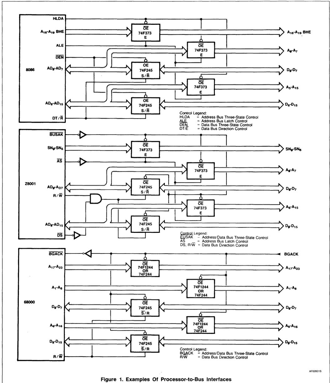
Figure 1. Examples Of Processor-to-Bus Interfaces
