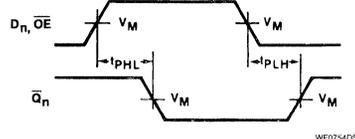
Waveform 2. Propagation Delay For Data To Output
