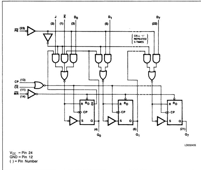
The J and  $\bar{K}$  inputs provide the flexibility of the J- $\bar{K}$  type input for special applications and, by tying the two pins together, the simple D-type input for general applications.
