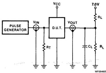
Test Circuit For Open Collector Outputs ('F631)
