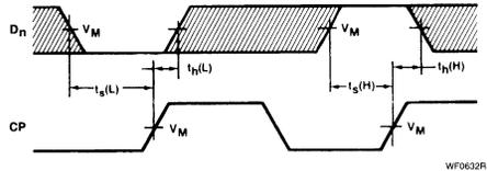
**Waveform 2. Data Set-up And Hold Times**
