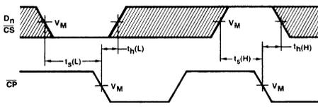
**Waveform 6. Data Set-up And Hold Times**
