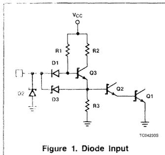
Figure 1. Diode Input
