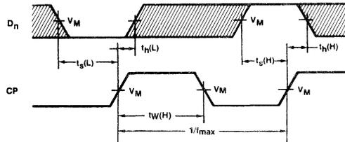
**Waveform 4. Data Set-up And Hold Times**
