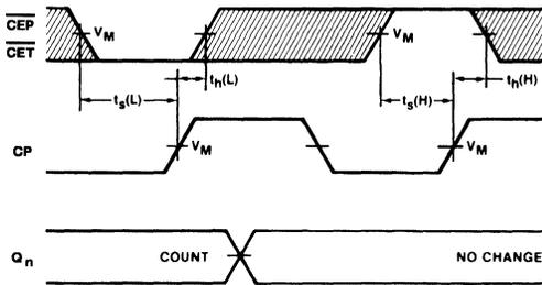
Waveform 5. Count Enable Set-up And Hold Times
