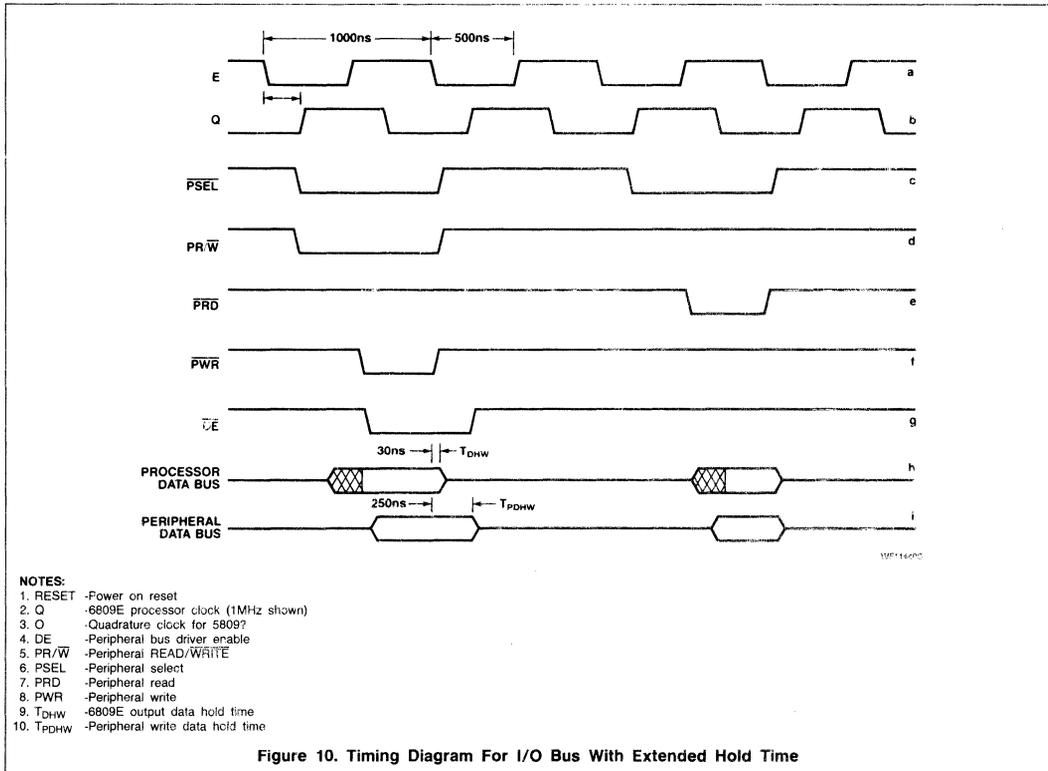
Figure 10. Timing Diagram For I/O Bus With Extended Hold Time
