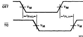
Waveform 2. Propagation Delays CET Input To Terminal Count Output
