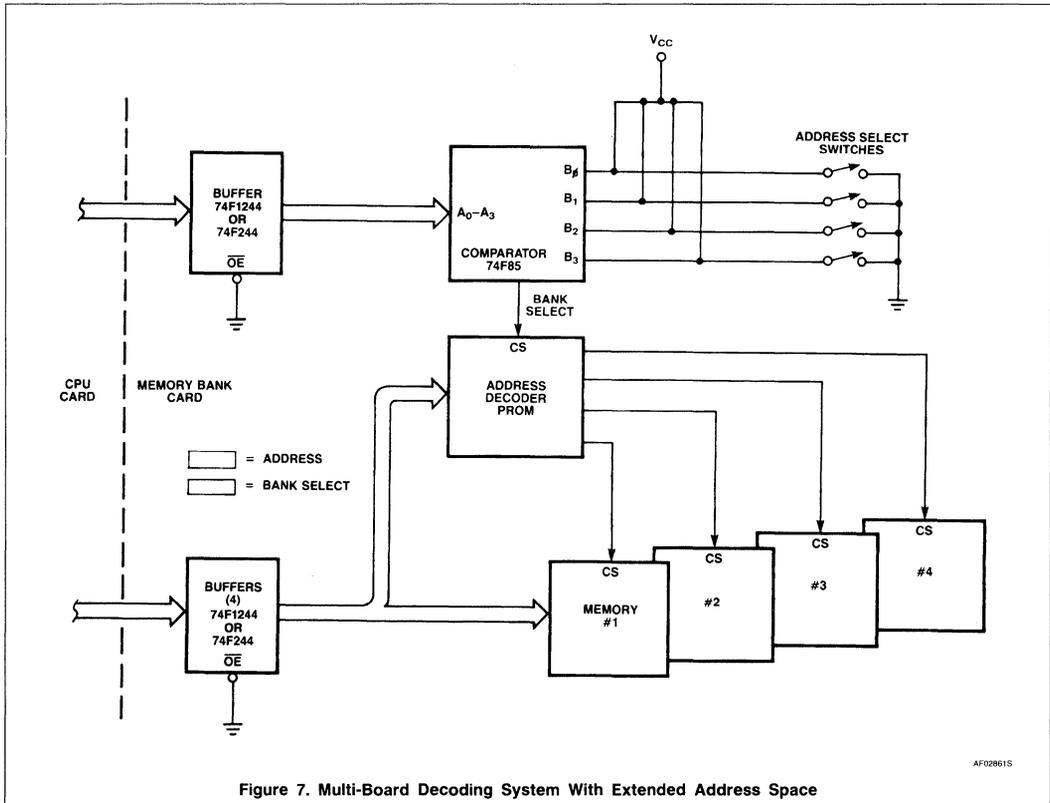
Figure 7. Multi-Board Decoding System With Extended Address Space
