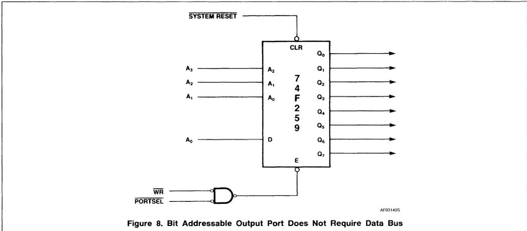
Figure 8. Bit Addressable Output Port Does Not Require Data Bus
