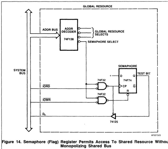
Figure 14. Semaphore (Flag) Register Permits Access to Shared Resource Without Monopolizing Shared Bus
