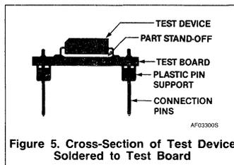
Figure 5. Cross-Section of Test Device Soldered to Test Board
