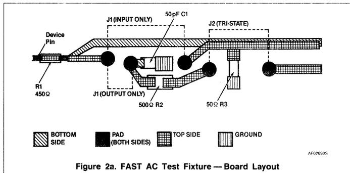
Figure 2a. FAST AC Test Fixture — Board Layout
