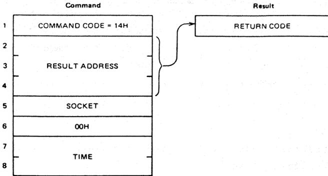
The WAIT RCV command specifies the time during which the socket set up by the SETUP RCV command is to await reception of a message packet.
