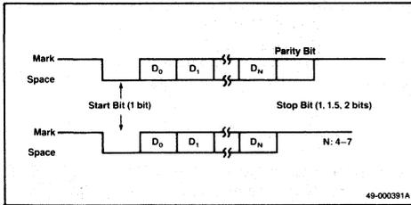
The start bit of the receive data indicates the start of the data. The stop bit indicates the end of the data block. When a data block is received, the MPSCC detects the start and stop bits, checks the parity bit, and deletes these bits from the data block. Therefore, the MPSCC transfers only data  $D_0$  through  $D_N$  to the host system.
