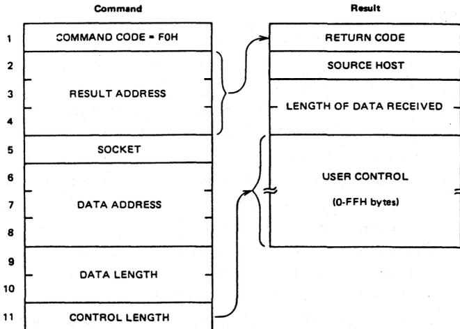
The SETUP RCV command readies a socket to receive message packets.
