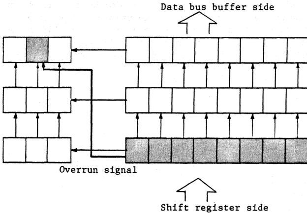
Fig. 3-5 Rx Overrun Error Bit Set Timing
