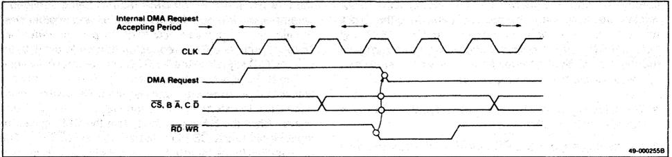
Figure 6-7. Example of MPSCC and μPD8237A Interface
