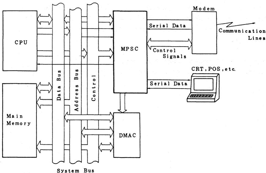
Figure 1.1 Example of configuration of system using MPSC
