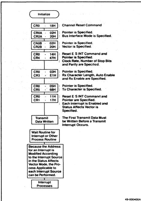
Figure 5-3. Interrupt Process
