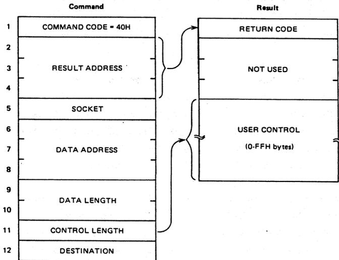
The SEND command transmits messages from memory to the other nodes through the network.
