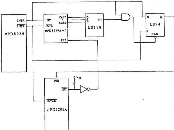
Figure 3.12 (b)  $\mu$ PD7201A and  $\mu$ PD8259A-2 connection example (reference circuit)
