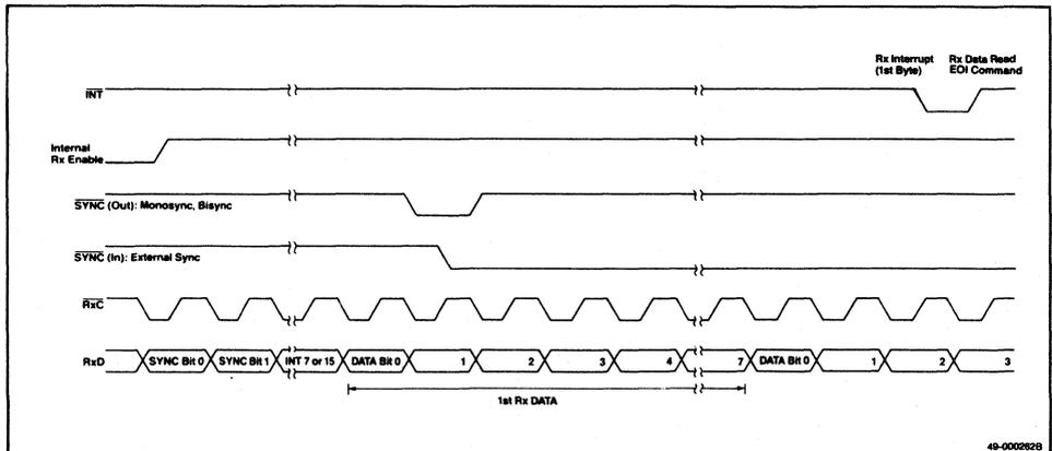
**Figure 6-14 Reception in Synchronous Mode (CRC Calculation)**
