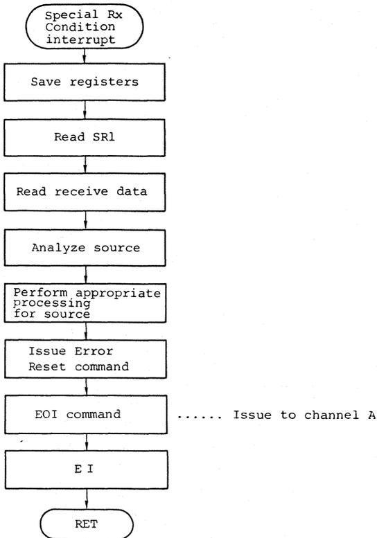
Figure 3.8 Example of Special Rx Condition interrupt processing
