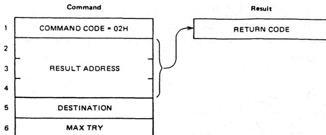
The ECHO command transmits the ECHO packet to the other nodes on the network. With this command, the host system can learn whether the destination node of the ECHO packet exists on the network.
