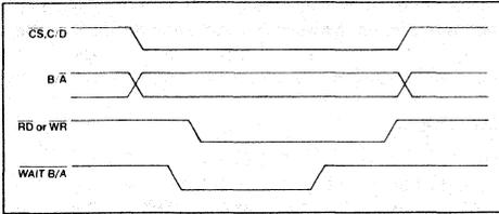
Figure 6-3. Interrupt Timing in Vectored Mode (1)
