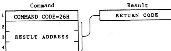
The CLR STAT command clears the contents of event counters to initialize the counters. The counters manage the transmit/receive statistics.
