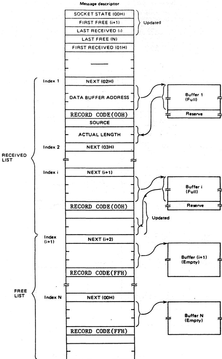
Fig. 4-4 Updated List on Receiving the i-th Packet (by the chip)
