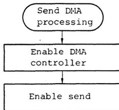
Figure 3.14 (a) Control example of send operation by DMA (main program)
