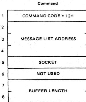
The RCV LIST command sets up a list of message buffers (message descriptor) to allow reception by sockets 80H and 90H. Only socket numbers 80H and 90H are supported by this command. The list provided by the host system when this command is executed is shown in Fig. 4-2. The message descriptor consists of a message list indicating the state of the buffer in which the received message is to be stored and control records which manage the buffer.
