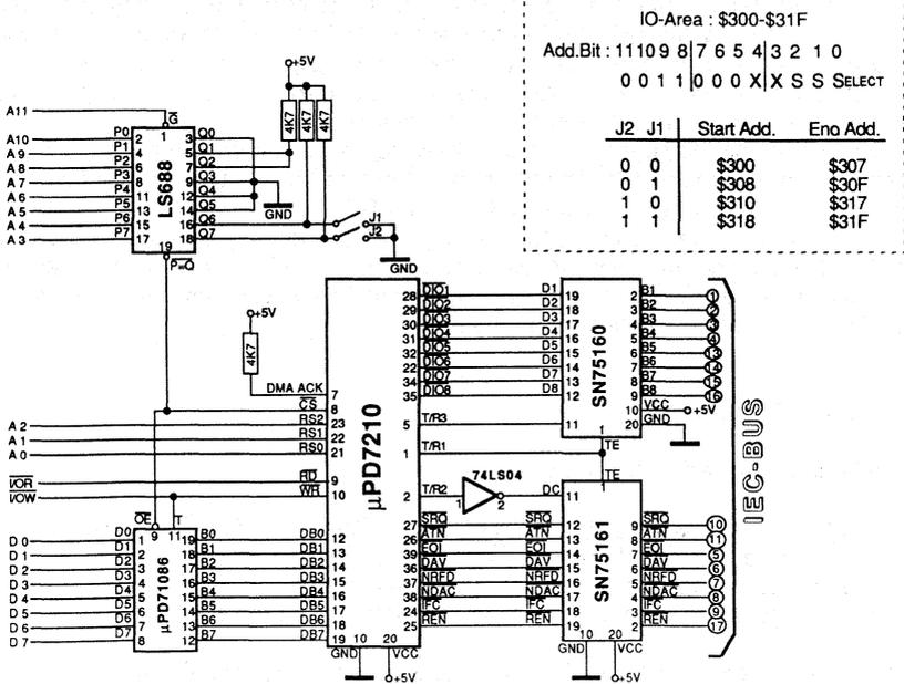
On the other hand the GPIB bus is a very powerful bus by means of communication speed and control protocols. This application note provides a set of routines that allows to handle these protocols. All routines are written in μPD8085 assembly language and can be transferred to any other programming language without problems. Each piece of software is well documented so the user can easily extract those routines which are needed for his application.
