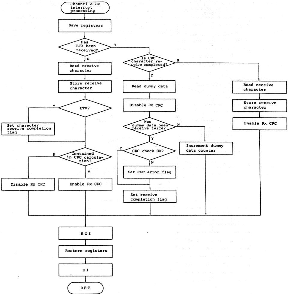
Figure 5.7 Synchronous operation Rx interrupt processing
