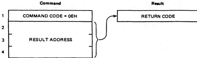
The MONIT OFF command suspends DMA transfer to the ring buffer while the uPD72105 is monitoring the network.
