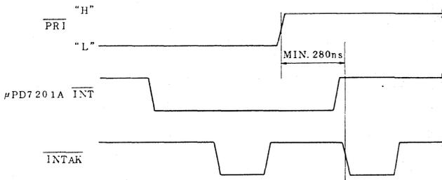
Figure 3.12 (a) Relation between  $\overline{\text{PRI}}$  and  $\overline{\text{INTAK}}$
