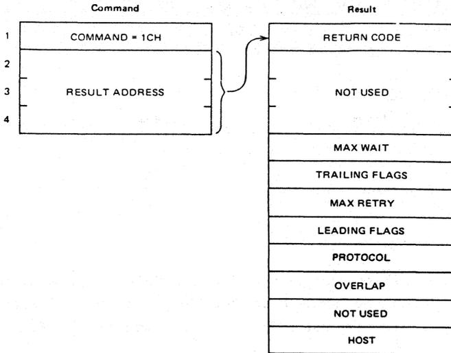
The GET PARM command reads the internal parameters of the μPD72105. To partially modify the internal parameters, the parameters of the SET PARM command can be created by first executing the GET PARAM command and then modifying the result.
