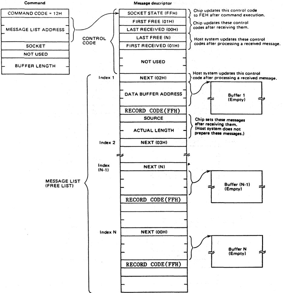
Fig. 4-2 RCV LIST Command List (created by the host system)
