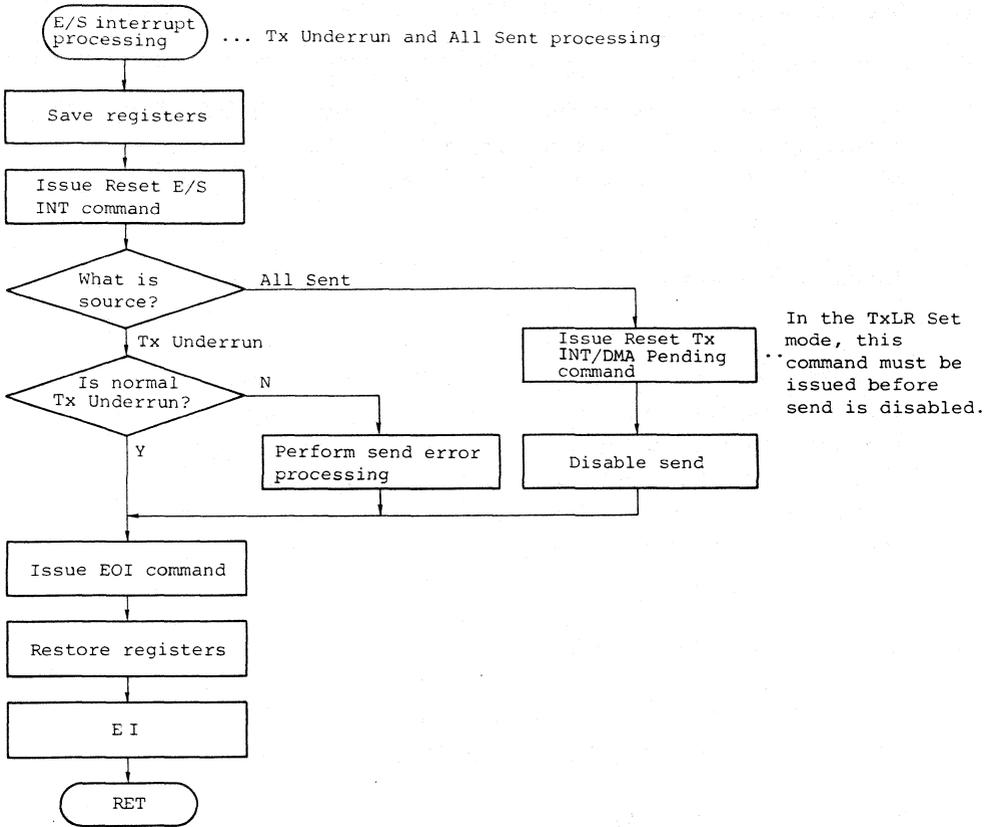
Note) Interrupt processing caused by other E/S sources is omitted.
