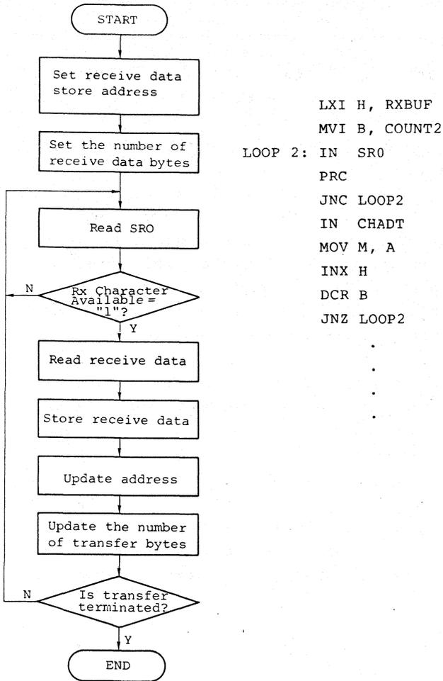
Figure 3.2 Example of send data transfer program using polling
