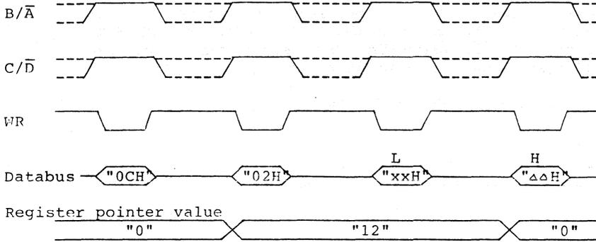
Fig. 3-3 TxBRG Register Setting Sequence
