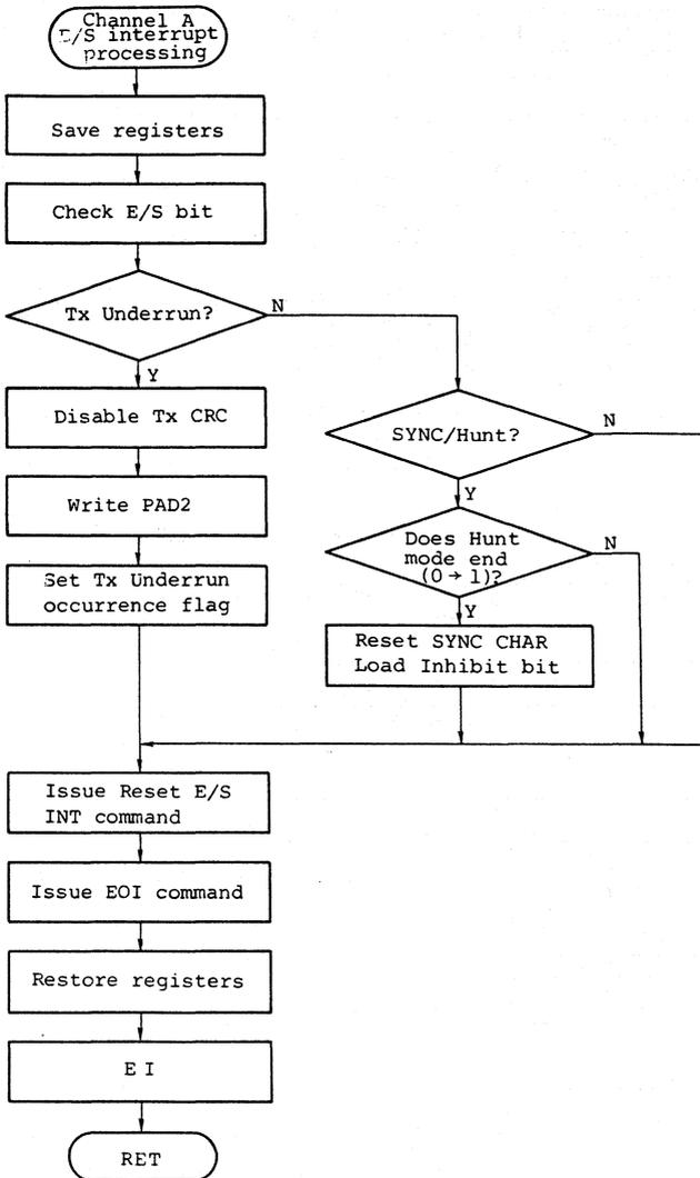
Figure 5.8 Synchronous operation E/S interrupt processing
