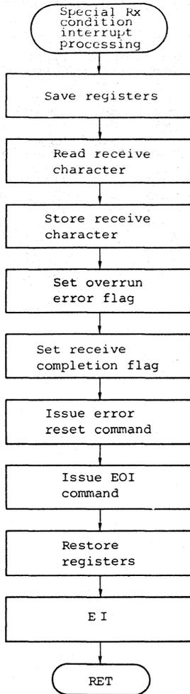
Figure 5.9 Synchronous operation Special Rx Condition interrupt processing
