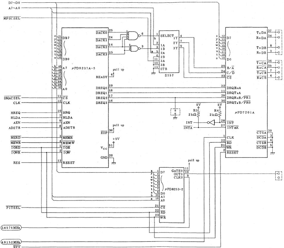
Figure 4.1 (b) μPD7201A application circuit example (reference circuit)
