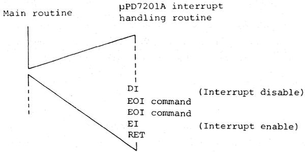
Figure 3.12 (c) Multiinterrupt processing sequence
