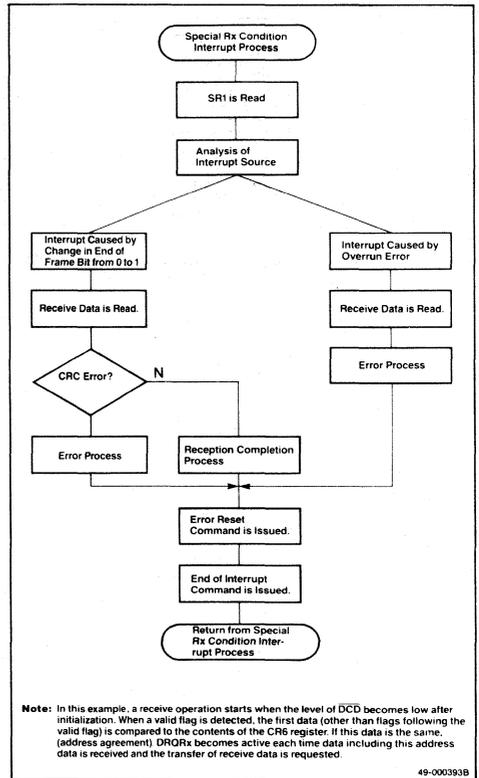
Note: In this example, a receive operation starts when the level of DCD becomes low after initialization. When a valid flag is detected, the first data (other than flags following the valid flag) is compared to the contents of the CR6 register. If this data is the same, (address agreement) DR0Rx becomes active each time data including this address data is received and the transfer of receive data is requested.
