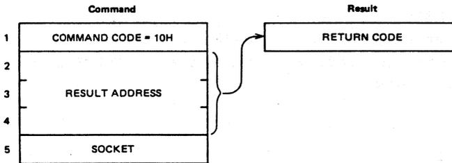
The END RCV command causes the socket that has been set up by the SETUP RCV or RCV LIST command to return to the inactive state.
