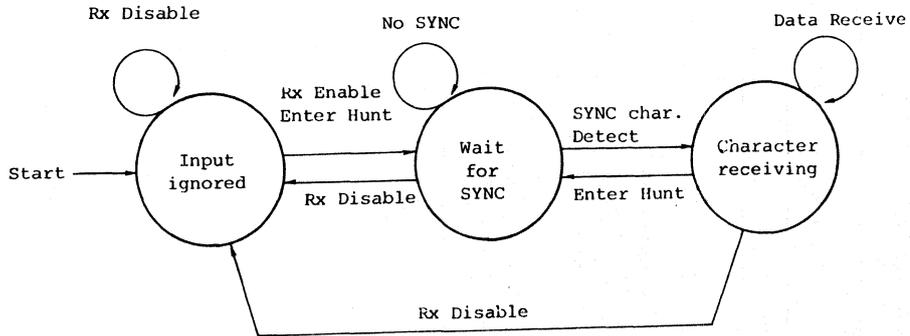
Figure 6.4 SYNC receive state transition diagram
