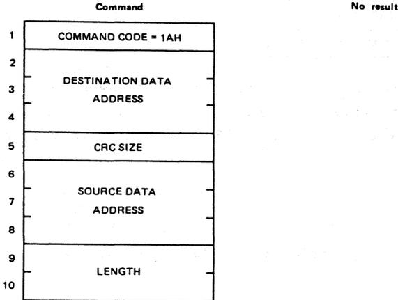
The LOOP BACK command transfers the data held by a buffer in memory via the upD72105 to another buffer in the node. The host system may check the data for changes during transfer by comparing the contents of both the buffers.
