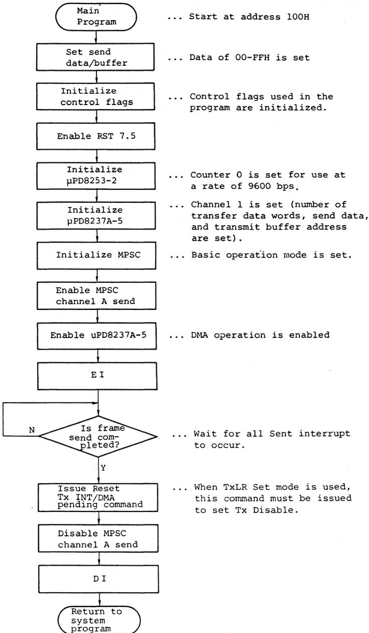
Figure 5.10 (a) HDLC send operation main program
