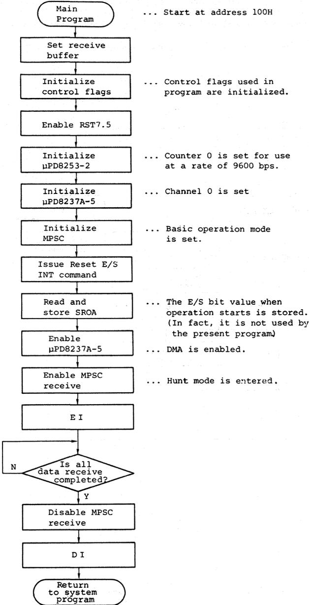
Figure 5.12 (a) HDLC receive operation main program
