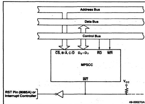
**CHANNEL A IN DMA MODE AND CHANNEL B IN INTERRUPT MODE**
