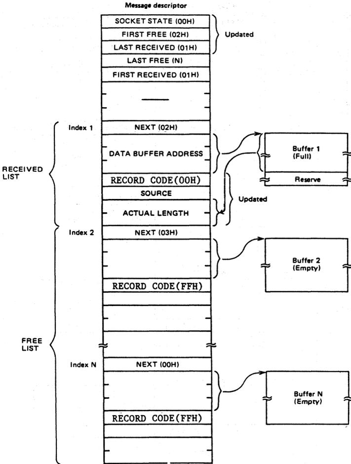
Fig. 4-3 Updated List on Receiving the First Packet (by the chip)
