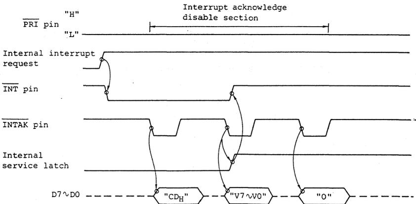
Figure 3.4 Interrupt timing in vector mode (85-1 mode)
