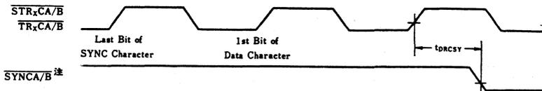
\*: SYNCA/B input must be set to 0 at the rising edge of  $\overline{R_xC}$  after 2 clock cycles following the last bit of SYNC character.
