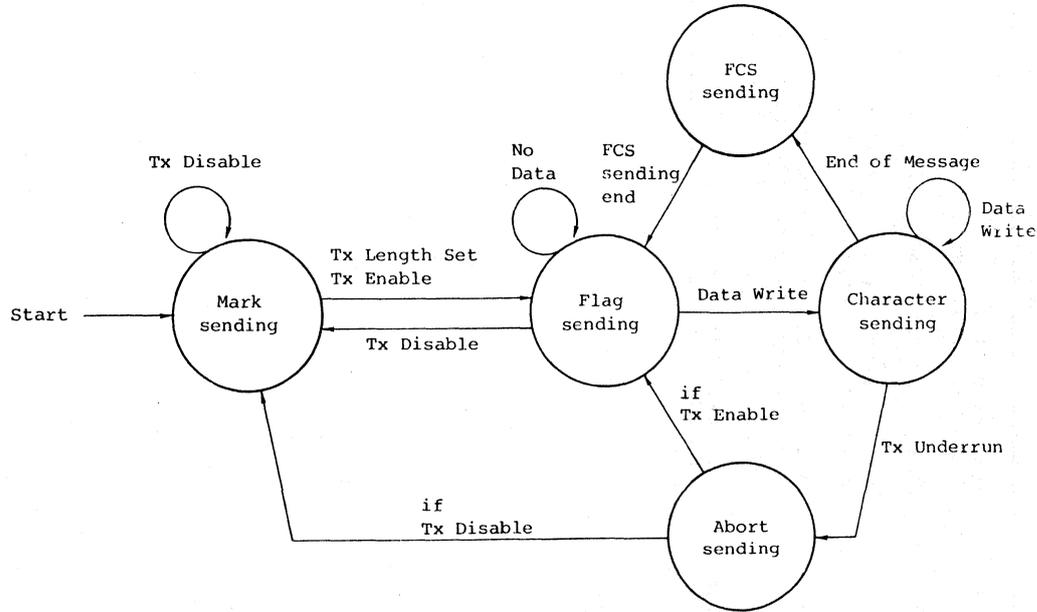
Figure 6.5 HDLC send state transition diagram (when Tx Length Counter is used and CRC exists)
