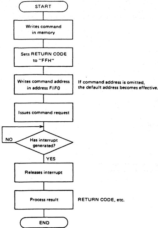
Fig. 5-1 CSMAC Control Flowchart
