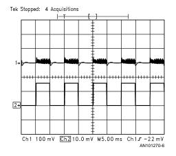
Upper Trace: Output Voltage, 100mV/div Lower Trace: Load Current, 1A/div
