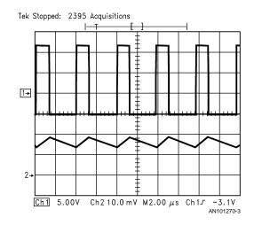
Upper Trace: Switch Voltage, 5V/div Lower Trace: Inductor Current, 2A/div Horizontal: 2µs/div
