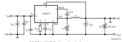
FIGURE 2. LM2673 Positive to Negative Converter
