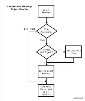
FIGURE 5. CAN Receive Object Handler
