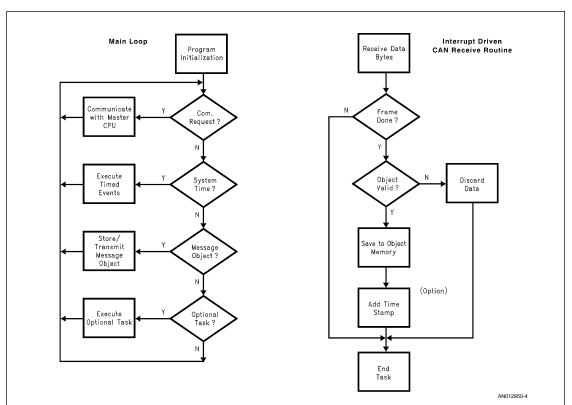
FIGURE 4. Main Program and CAN Receive Interrupt Handler
