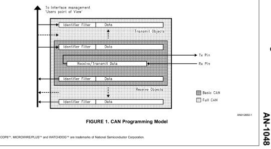
The hardware interface to the processor is provided with either serial links or a paralell interface with message data (identifier, control and data) being accesed on memory mapped address locations, so the user "sees" message data and control information.
